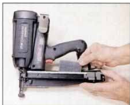
The nail magazine holds two finish nail strips of 50 nails each. Holes in the side show the nails remaining in the magazine.
