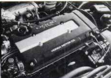
Integra GS-R has smaller, more efficient engine, with highest hp/displacement ratio available in production cars sold in the U.S.
