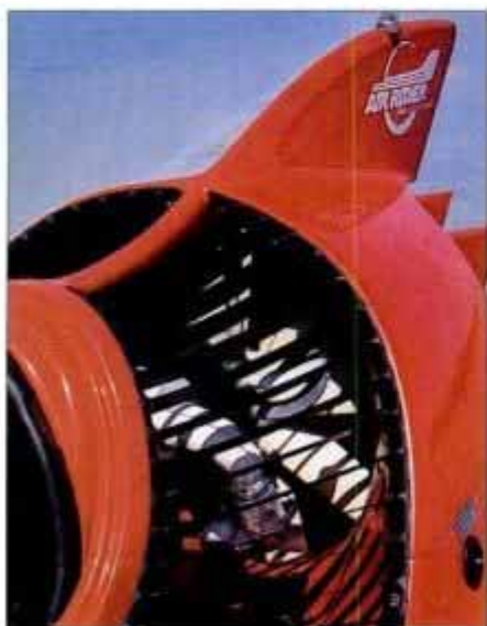
Sand bars don't stop a single-seat Booster (top right). The 2-cycle Goble-Hirth engine pumps out an impressive 54 hp (left). The 9-blade prop is made of Kevlar-reinforced composite (above).
