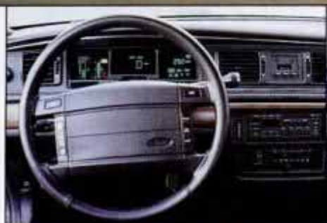
Owners liked control layout, but said that wheel hub blocked instrument panel.
