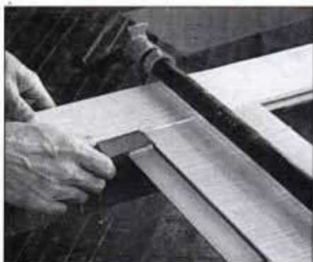
12 Glue and clamp the mullion to the back bottom rail. Check that the assembly is square before leaving it to set up.
