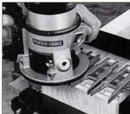
21 Pins are cut in the drawer fronts and backs with the workpiece at horizontal. A vertical board steadies the router.
