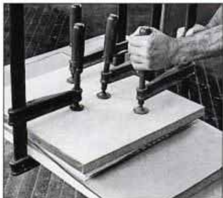
24 Use heavy flakeboard or plywood as cauls to clamp the veneered panels. Place paper between the cauls and panels.
