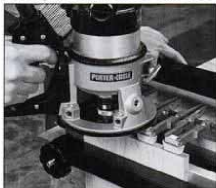
20 Machine-cut dovetails are made with a router and jig. Hold a drawer side vertically in the jig to cut the tails.
