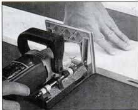
1 Mark the spacing for the biscuits on the stock for the case sides. Place the stock on a tabletop and cut the biscuit slots.
