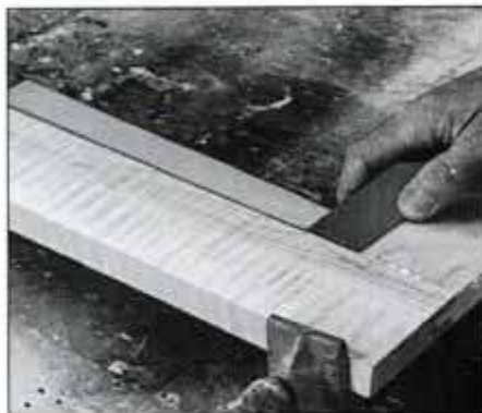
15 Glue and clamp together the drawer frame parts. It's important that each assembly be square and free of twist.
