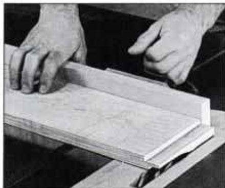
7 Cut tenons on the front and back rails with dado blades in the table saw. Tip the piece on edge to cut the tenon to width.
