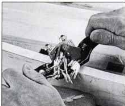
9 Saw the curve on the front rail, and remove the saw marks with a spokeshave. Edge should not need further smoothing.
