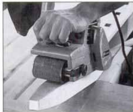
4 Clamp a case leg in a vise. Remove band saw marks and refine the leg's shape using a belt sander.
