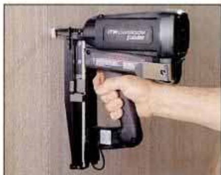
The nailer is suitable for all finish carpentry such as wall paneling. Tool doesn't function unless tip contacts work.
