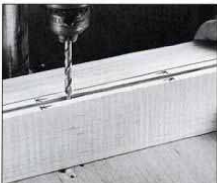
11 Cut the mortises in the top and bottom back rail on the drill press. Square the mortises with a sharp chisel.
