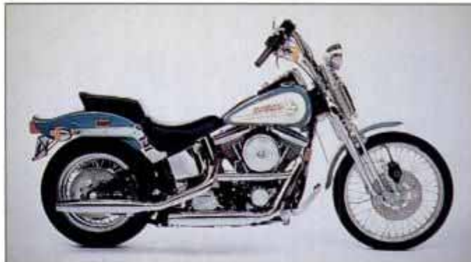
1992 FXSTS Springer Softail carries a '48-style front end.
