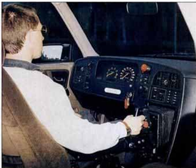
Side-mounted joystick eliminates steering-wheel safety hazard.
