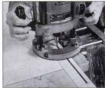
6 Cut the back panel groove in the legs with a plunge router and edge guide. Reset the router's depth to cut rail mortises.
