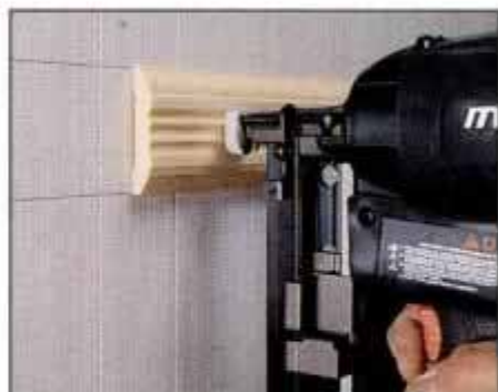
Plastic tip prevents marring work and controls nail depth. Tips are available for nailing flush or setting below surface.
