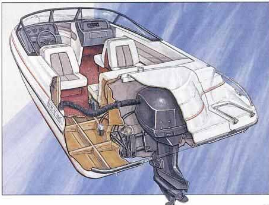
Because it rotates its own profile (above), the OMC Quiet Rider can be mounted beneath a sound-muffling engine cover (right), which is fed by an air-induction hose. Note Eurostyled stern.
