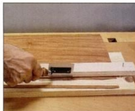
6 Use the edge of a straight board to guide veneer saw. Saw is better than utility knife for cutting with the grain.
