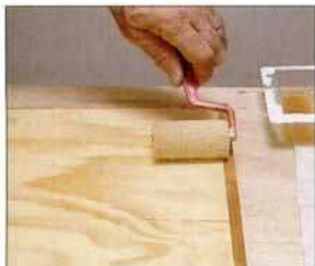
17 Apply two coats of contact veneer glue to both the ground and the back of the veneer. Then wait until glue isn't tacky.
