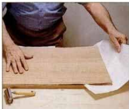
18 Paper sheets between veneer and ground allow alignment. Contact glue takes hold as sheets are pulled away.
