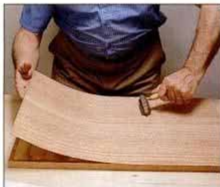
19 Press down the veneer firmly with a small roller. Work from middle toward ends to avoid creating air pockets.
