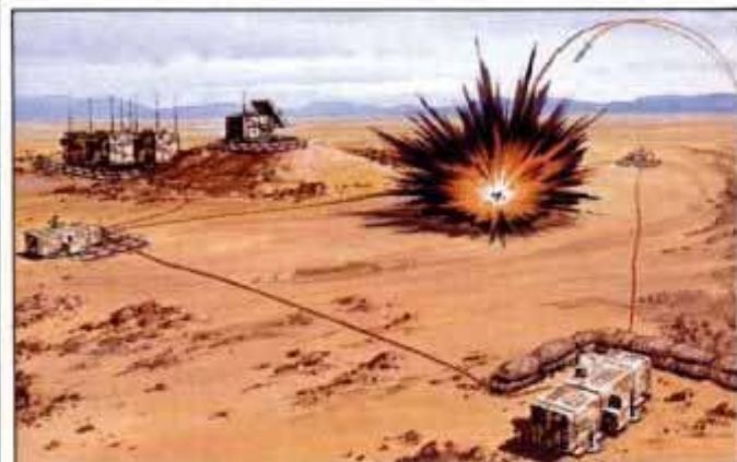
Decoys lure anti-radiation missiles away from radar units.
