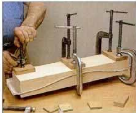
26 Use cutoff from sawing curved ground to act as caul. Several sheets of newspaper over veneer help even out pressure.
