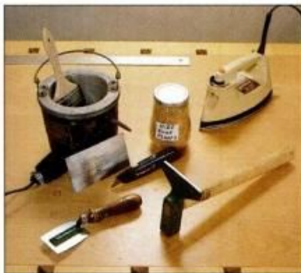
9 Tools for hammer veneering include veneer hammer, saw and utility knife, scraper, glue pot, glue and electric iron.
