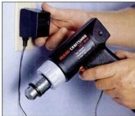
A reversible cordless drill is best for light-duty hole boring and screwdriving. This model recharges in 3 hours.
