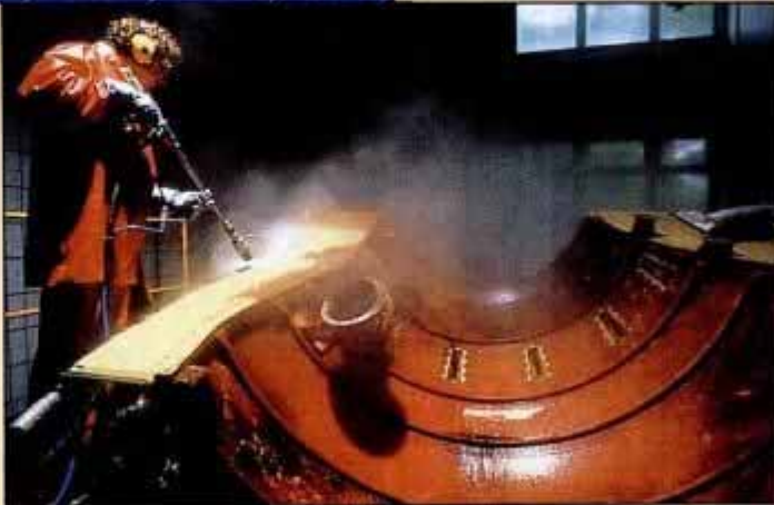
LARPS robot (top) will scour paint from large jets for the Air Force. Lufthansa is testing waterjets on commercial airliners (above).
