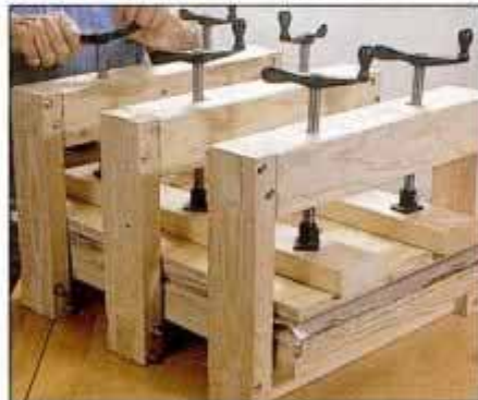
27 For frequent veneering, a shopmade veneer press is handy. This one accommodates work up to 18 x 24 in.
