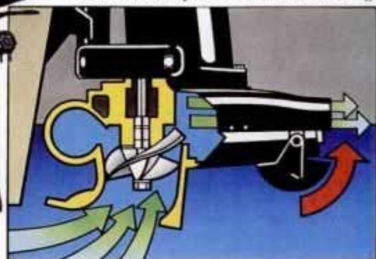
An impeller forces water through a nozzle to create thrust in the new line of Johnson/Evinrude jetdrives.
