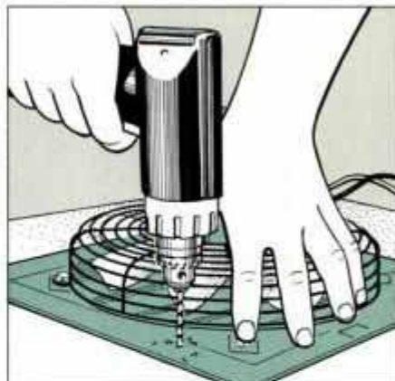
6 Place the shutter housing in the panel. Bore holes for the mounting bolts through the prepunched holes in the housing.
