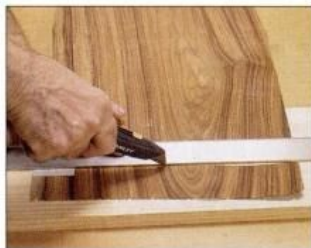
7 Use a utility knife to make clean cross-cuts. A piece of masking tape wrapped at the end of the cut prevents tearout.
