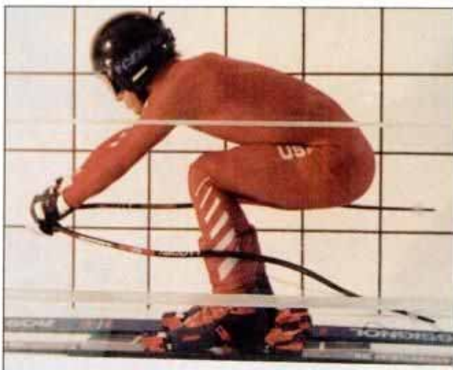
Bill Johnson practices transition from low tuck to turning stance in Calspan wind tunnel. The training helped him win a gold in '84.
