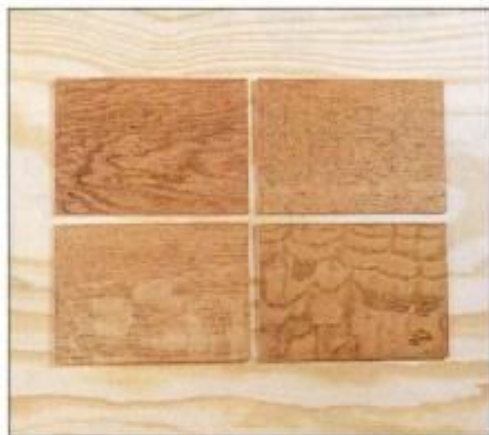
1 Various log cuts (clockwise from top left): flat, rift, half-round and quartered. Plywood panel underneath is rotary cut.
