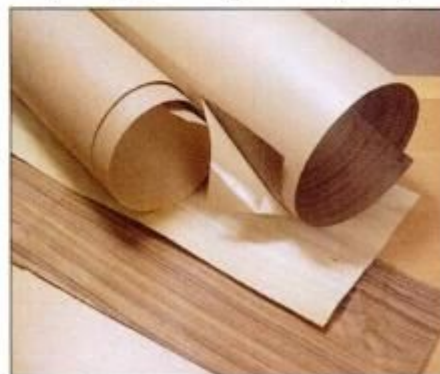
4 Types of veneer (clockwise from top left): paper-backed flexible, adhesive-backed, poplar crossband and standard.
