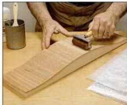
25 Cut veneer slightly oversize and place onto glue-coated ground. Apply pressure by rolling from the center outward.
