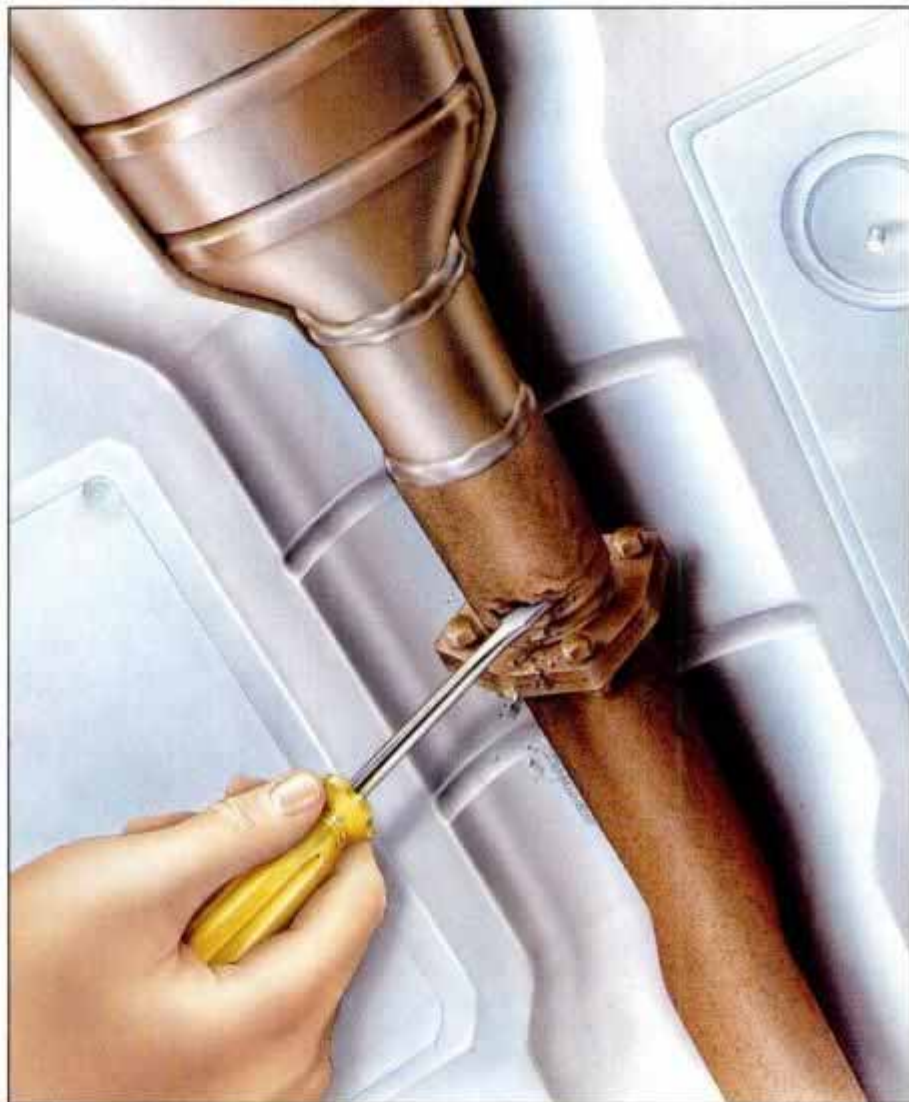
Probe rusty spots of exhaust plumbing to make sure corrosion is only on the surface.
