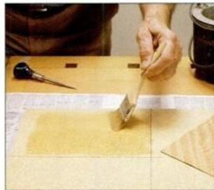
10 After cutting veneers, begin hammer veneering by brushing hot animal glue onto ground. Work one section at a time.
