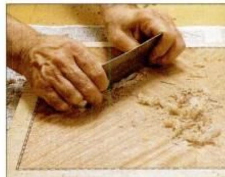
16 Remove surface glue and smooth veneers with a sharp scraper. Then, finish smoothing the panel with sandpaper.
