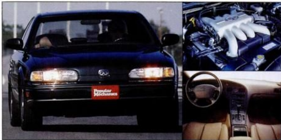
Infiniti Q45 offers subdued, roomy interior and aggressive suspension tuning. Muscle of Q45's twin-cam 32-valve 4.5-liter V8 engine was the favorite of the test crew.
