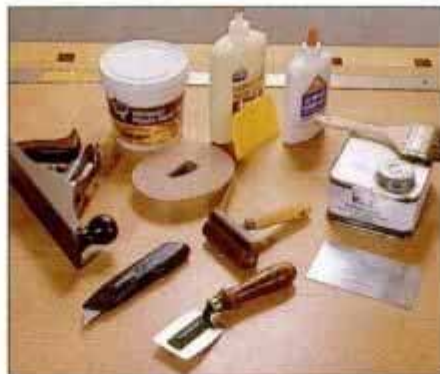
20 Pressure veneering uses standard trimming tools, carpenter's glue and applicator, roller, veneer tape and scraper.
