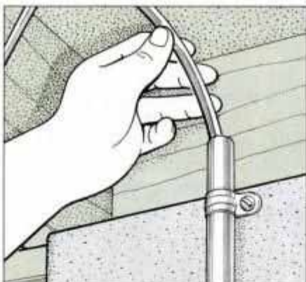
11 Feed 12/2 cable w/g (12-gauge, 2-wire cable with ground) through the conduit and into the switch box.
