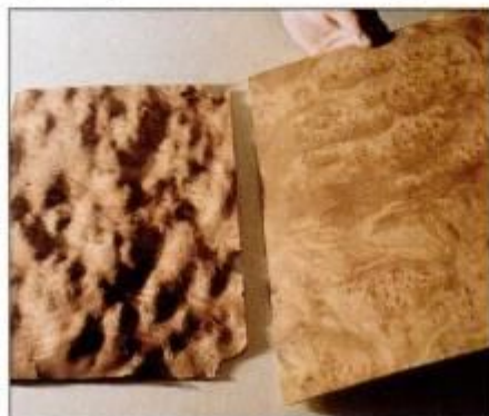
3 Standard burl veneer (left) features typical deformed surface. Flexible veneer of same species comes flattened.
