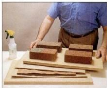
5 To flatten deformed veneer, dampen it with water mist and press between absorbent paper and weighted particleboard.
