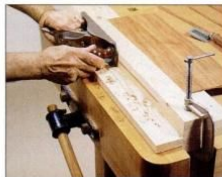
8 To accurately true veneer edges, sandwich veneer between boards and clamp to wider board that supports plane.
