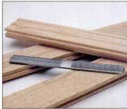
A 4-in-1 combination file/rasp has coarse and fine cutting surfaces on both the flat and half-round sides of the tool.
