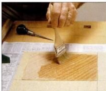
11 Place veneer upside down on the glue and brush hot glue on the underside. Then, turn veneer over and place in position.
