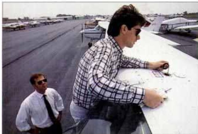
Dave and I do the preflight, checking prop condition, oil and fuel levels, and taking fuel samples to spot water or sediment.
