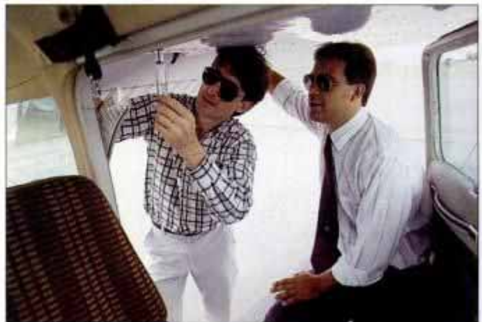
Dave and I do the preflight, checking prop condition, oil and fuel levels, and taking fuel samples to spot water or sediment.
