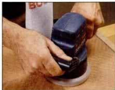
4 Thanks to its pivoting front handle, the sander is easy to control, even in delicate operations such as sanding veneer.
