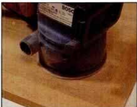
3 Sander's random orbit helps you flush off and smooth edge molding, even when it's perpendicular to the panel's grain.
