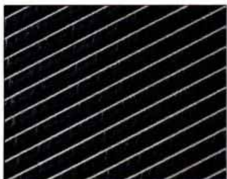
After soaking in sharpening solution for about 35 minutes, the same file now has uniformly sharpened cutting edges.
