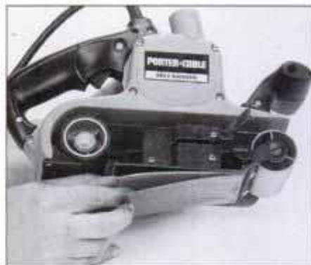
Platen supports belt over sanding area and handles friction of moving belt. P-C model has cork backing pad to cushion platen.
