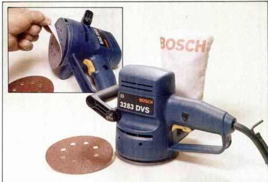
The Bosch variable-speed random orbit sander excels at a variety of sanding, finishing and shaping tasks. Its sanding discs are attached with an easy-to-use hook-and-loop system.
