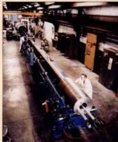
Sandia researchers add third stage to their gun, boosting projectile velocities to orbital speeds.
