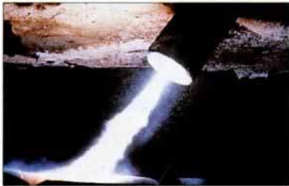
Plasma arc torch, shown in operation at left, could serve as high-efficiency asbestos incinerator in mobile trailer.
