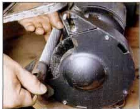
To prepare file for sharpening, it must be thoroughly cleaned of all imbedded particles. Then it's bathed in the degreaser.
