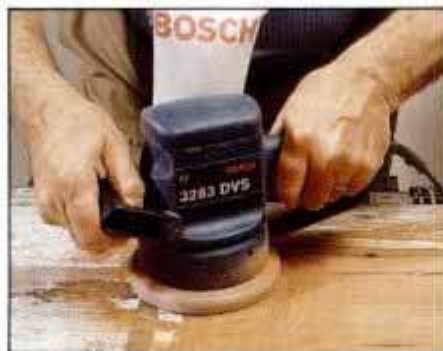
1 The sander is a clean and effective paint-stripping tool when outfitted with dustbag and a coarse-grit disc.
