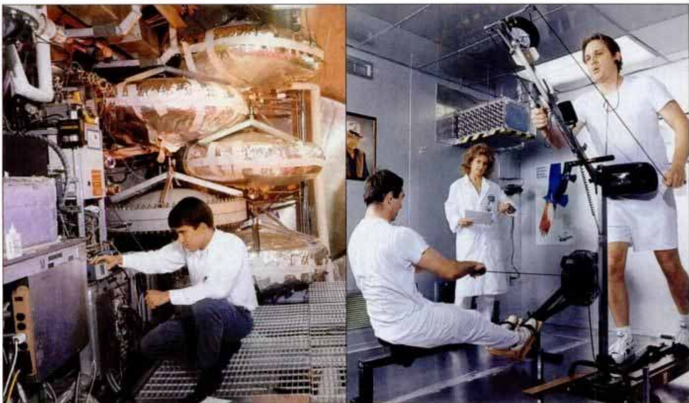
In tests of NASA's Environmental Control and Life-Support System (left), volunteers worked out in a sealed room (right) to supply water for recycling.
