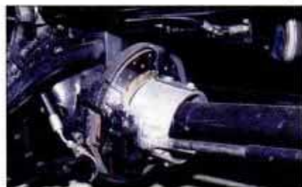
Braking system consists of a 12-in. disc on each differential yoke.
