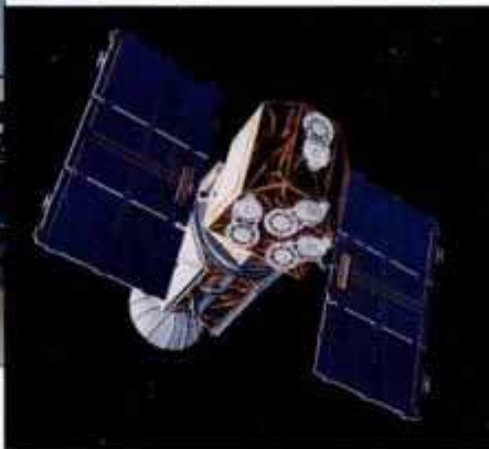
Four telescopes will image near and deep-space objects in extreme ultraviolet radiation.
