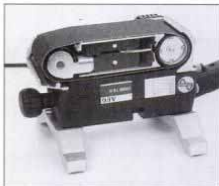
Belt sanders with stand accessories can be used as stationary sanders. Adjustable fences are also available for guiding work.
