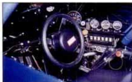
Interior is gutted. Plexiglas firewall allows driver to see into engine compartment.
