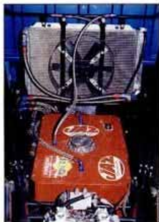
Fuel cell and engine radiator are mounted behind cab for protection.
