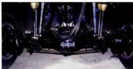
Rear steering is controlled by electric solenoids that control hydraulic pistons.
