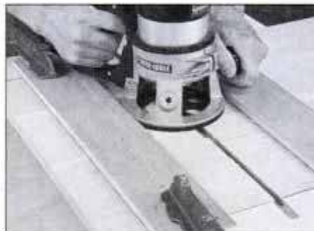
10 Clamp two straightedges across the case sides and rout the dovetail slot, making two passes with the router.
