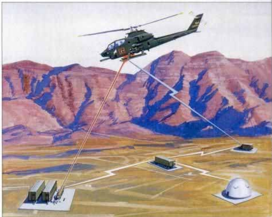
Cobra chopper absorbs brunt of laser beam in threat-surrogate test.
