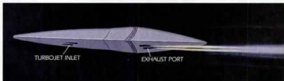
External-combustion ports [top] at mid-fuselage release fuel that burns in cone bounded by shock wave. Conventional jets [above] take over at low Mach numbers.
