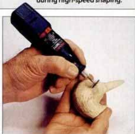
Cordless Minimate is a maneuverable and well-balanced tool that's gripped like a pen during high-speed shaping.
