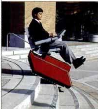
Microprocessor-controlled hydraulics activate tracks and adjust seat on Access power chair.
