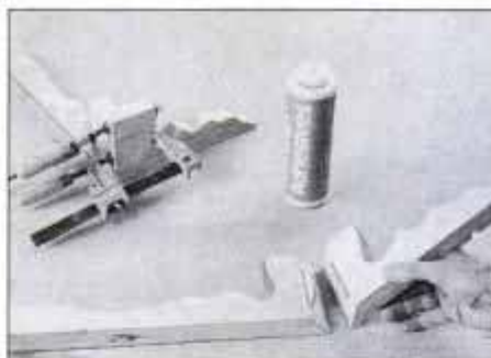
14 Apply glue to miter faces and plate groove. Install the joining plate, and clamp feet together until the glue sets.
