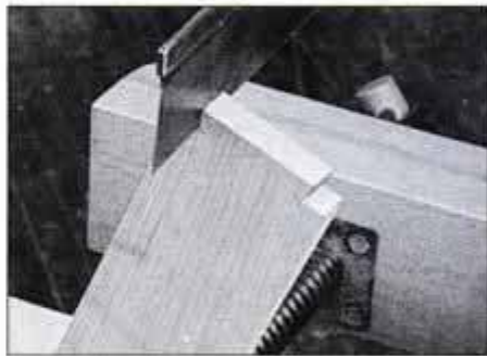
8 Lay out the large dovetails on the stretcher ends. Tip the stretcher at an angle and make the cuts with a dovetail saw.
