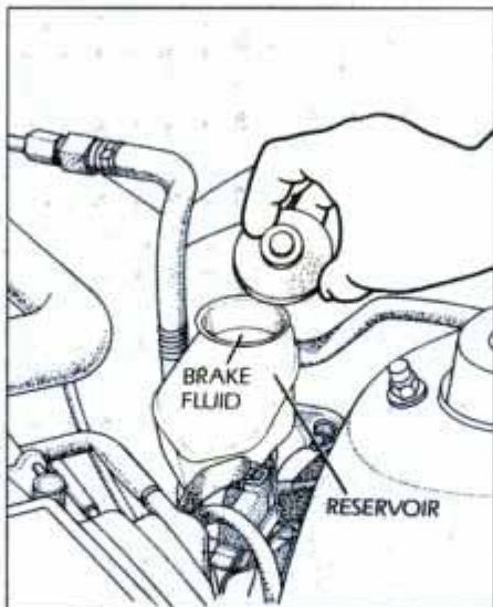
Check the brake master cylinder reservoir for fluid level at regular intervals.
