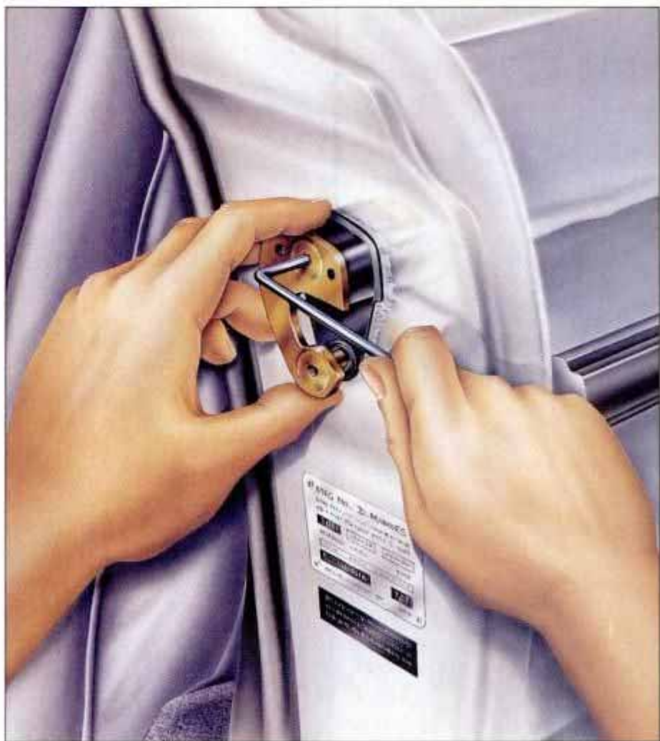
Poorly aligned, ill-closing doors may need to have their striker plates adjusted.
