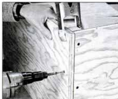
1 Attach end panels to 2 × 2 corner blocks with screws and glue. Then, secure the long sidepieces in the same way.
