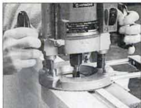
8 Turn benchtop on edge and rout a \frac{1}{8} -in.-wide \times \frac{5}{16} -in.-deep clearance groove for the tail vise upper guide plate.
