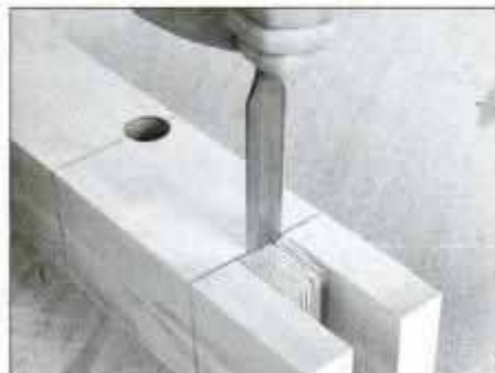
11 Band saw the finger joint slot for the shoulder arm joint. Then, make a series of cuts, and remove waste with chisel.
