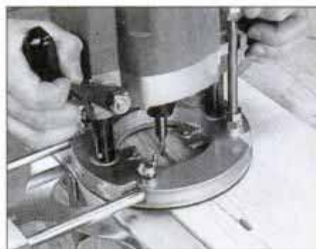
2 Use a router with 3/8-in.-dia. straight bit and edge guide to cut elongated holes for holding chisels, files and rasps.
