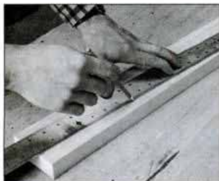
1 After cutting 5/4 \times 4 stock slightly over-size, mark leg tapers with a straightedge and lay out compound angle end cuts.
