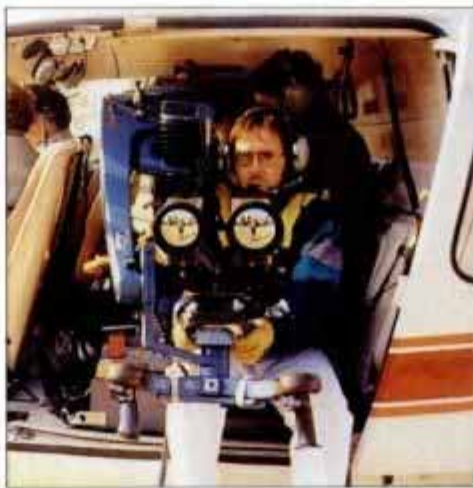
Dual-band infrared scanner peers out of helicopter seeking buried land mines.
