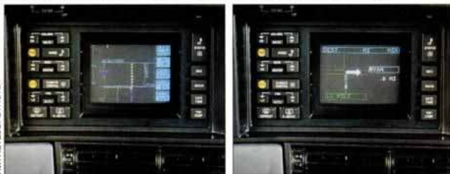
TravTek system now being built into 100 Oldsmobile Troféos uses the car's stock color CRT for map readouts. Steering wheel buttons allow driver inputs while in motion.
