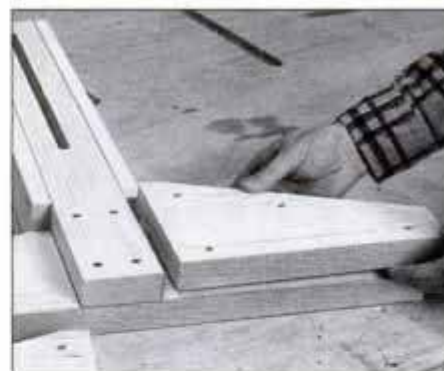
3 Secure angled outer base sections with screws and glue. Outer sections lock channel in place and strengthen base.
