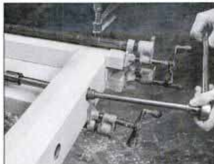
15 Glue and clamp shoulder vise arm to benchtop assembly. Then, secure guide bar end to arm with bolt and washer.
