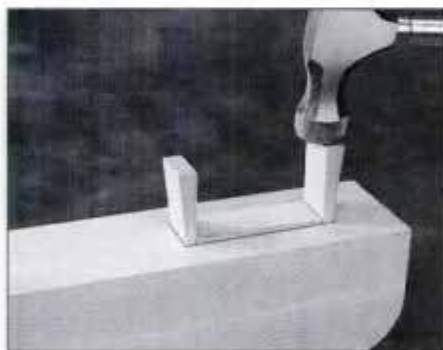
27 Apply glue, and drive wedges in tapered mortises to help lock tenons in place. Trim wedges and tenon ends flush.
