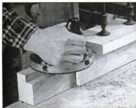
1 Use a router to remove the waste in leg notch. Leave a strip of wood for support that's removed with handsaw or chisel.
