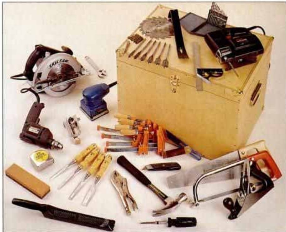
This handsome and durable toolbox is designed to hold all of the tools shown. It features two lift-out trays and a generous storage compartment for power and hand tools.
