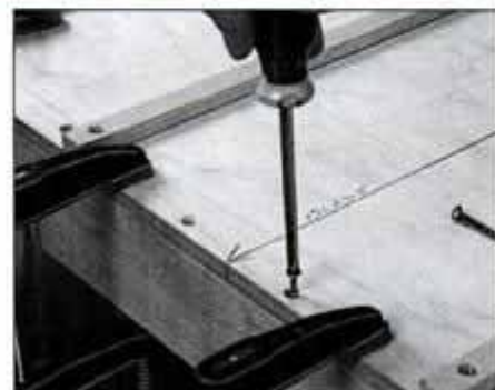
3 Clamp rear fence to bottom panel so it's flush with edge, and attach with screws. Keep screws away from blade line.
