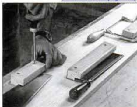
1 Make handsaw blocks from 5/4 pine, and cut rabbet with dado blade. Lay out saws on backboard, and install blocks.
