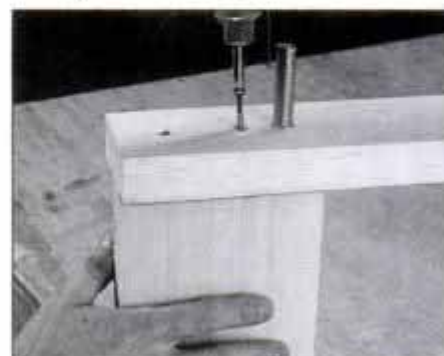
6 Join the roller support sides to the rails. Threaded rod extends through slot for locking stand height.
