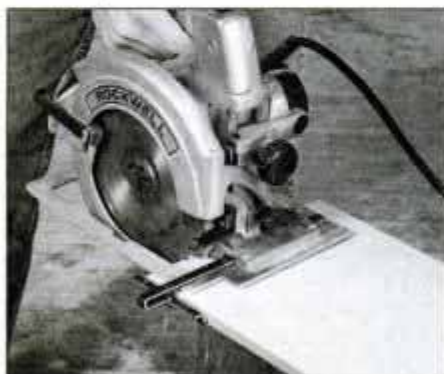
1 Cut plywood to size with a circular saw. Use a straightedge guide for wide pieces and a rip guide for the narrow stock.
