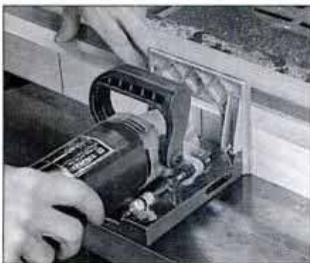
1 Rest plate joiner and stock on a flat surface to ensure accurate slots. Dowels or splines could also be used to join top pieces.
