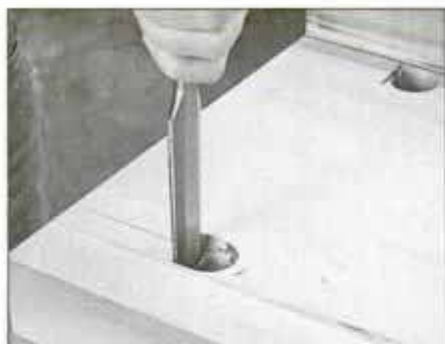
5 Use a chisel to square a washer and nut seat in 1½-in.-dia. × 1¼-in.-deep holes bored to intersect endcap bolt holes.
