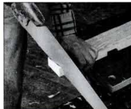
3 Use a handsaw to cut the compound angles on the leg ends. Follow angle layout lines, and trim smooth with plane.
