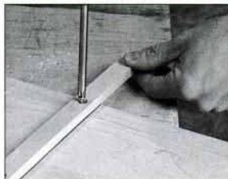
2 Align the guide strips and attach to the bottom of the panel with \frac{3}{4} -in. No. 6 fh screws. Countersink the screw pilot holes.
