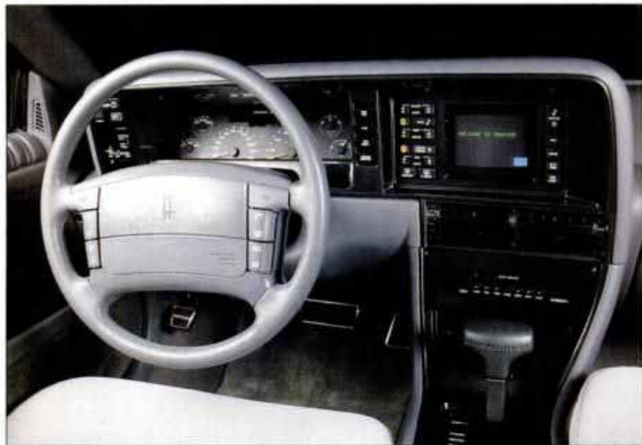
TravTek system now being built into 100 Oldsmobile Troféos uses the car's stock color CRT for map readouts. Steering wheel buttons allow driver inputs while in motion.
