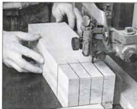
21 Lay out finger joint on tail vise arm pieces. Cut to joint lines on band saw and remove waste with sharp chisel.
