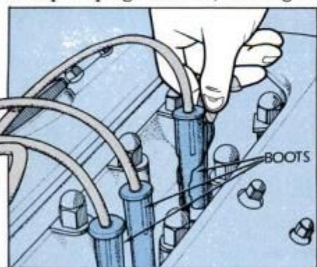
You may need to use a special tool to remove stubborn spark-plug connector boots.
