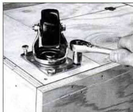
3 Attach swivel casters to 1 × 6 cleats secured to bottom panel. Use \frac{5}{16} -in.-dia. × 1½-in.-long lagscrews and washers.
