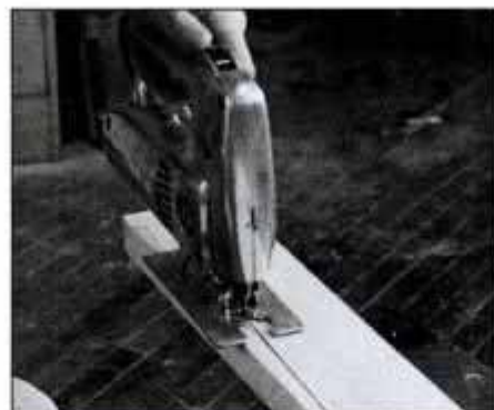
2 Clamp stock to worksurface and cut tapers with a sabre saw. Cut to the waste side of the line, and trim with a plane.
