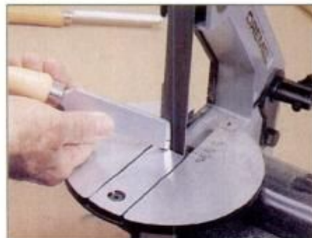
Lathe chisels are quickly sharpened on the belt sander. Unlike wheel grinders, the belt sander produces flat-ground bevels.
