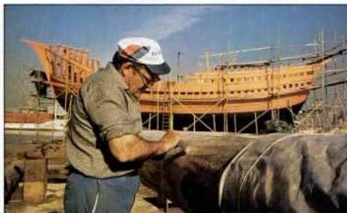
A worker prepares a spar in Barcelona, Spain, where the replica of the Santa Maria was constructed using traditional techniques.
