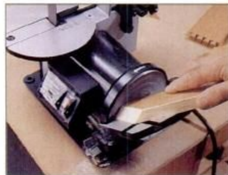
The disc-sander table tilts 45° up or down. In conjunction with the miter gauge, precise compound miters can be sanded.
