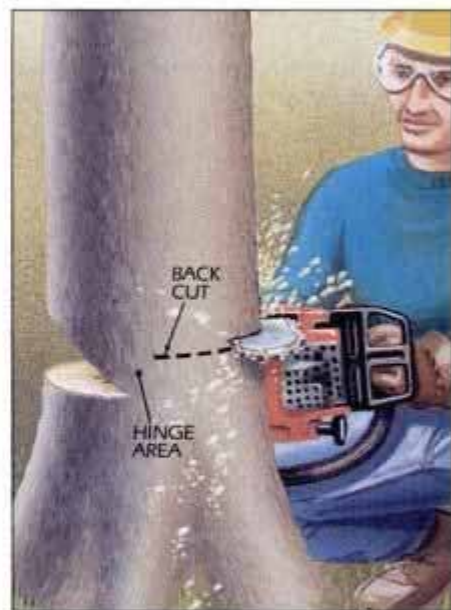
Back cut is slightly above wedge apex. Cut stops about 1/8 of trunk diameter from wedge. Wood at hinge area controls fall.
