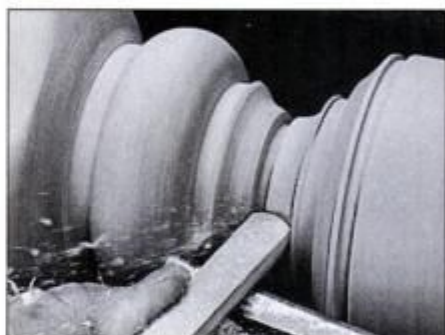
16 Cut beads and coves using depth grooves as guides. Cut cove with a round-nose chisel held straight and pivoted.
