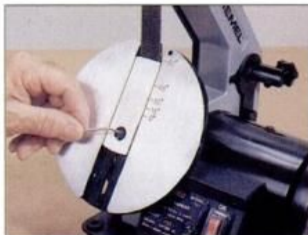
Belt-sander table tilts to 60°. Sliding insert permits adjusting the gap between belt and table to properly support small work.
