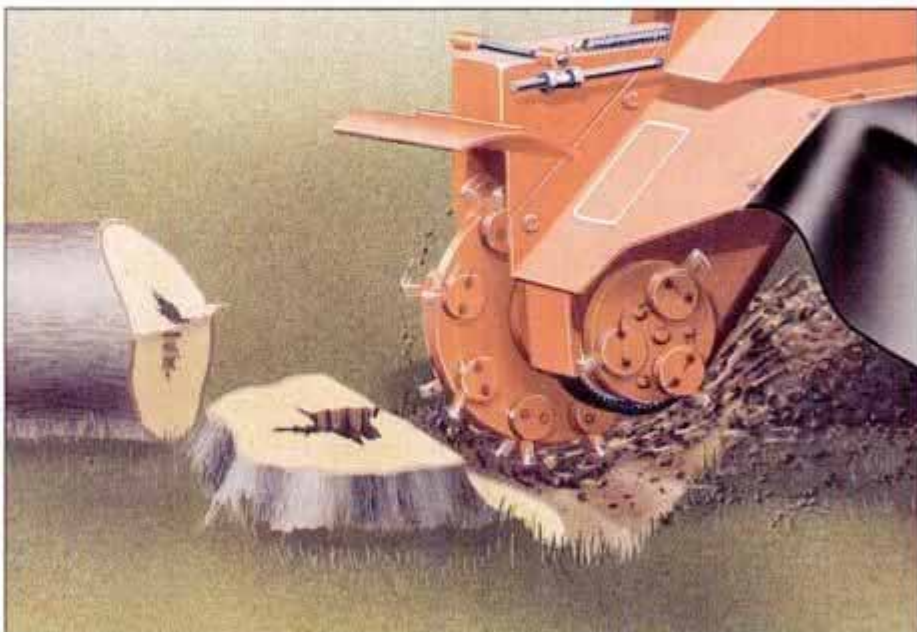
After the tree is down, the stump should be removed. A stump grinder is a powerful, carbide-tipped grinding machine that cuts away the stump to below ground level.
