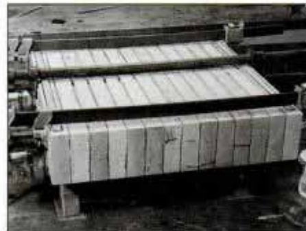
7 Once the glue is dry, glue and clamp the two groups of boards. Keep clamps off top by using thin strips of wood.
