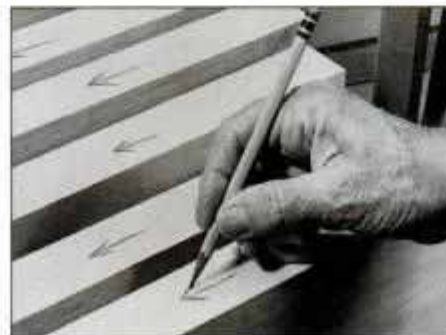
3 Edges become top and bottom surfaces after glue-up. To make surfaces easier to plane, mark and align grain direction.
