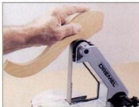
Exposed top idler wheel of belt sander acts like a drum sander for shaping and smoothing inside curves on wood and metal.
