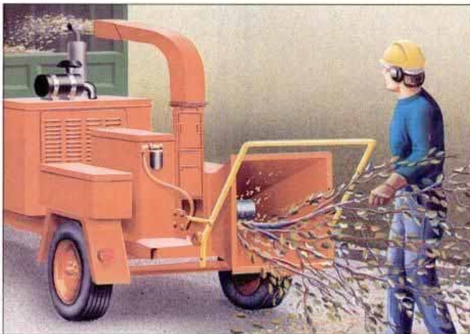
A heavy-duty chipper is the fastest and most efficient tool for clearing tree limbs. The mulch that's produced is fed into a dumptruck or large trailer for disposal.
