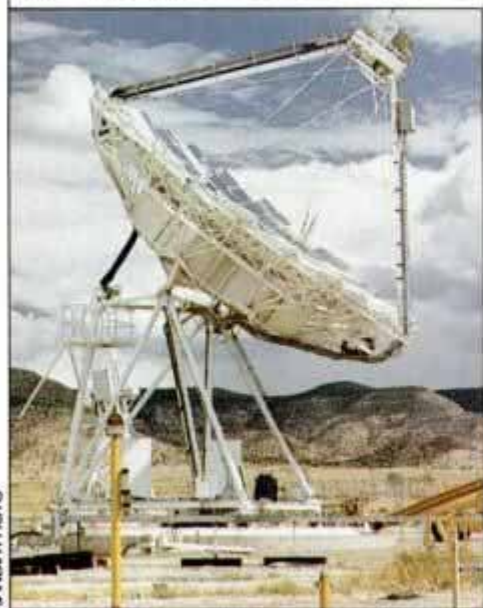
Parabolic mirror focuses sunlight onto pool of liquid sodium for 90% efficiency.
