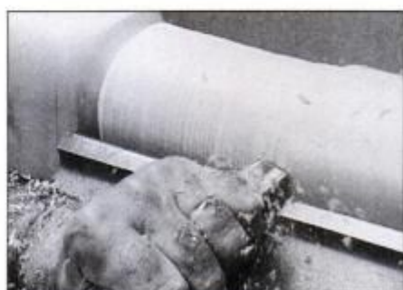
12 Rough the leg into a cylinder. Pivot the gouge to the right, and keep its bevel against the spinning workpiece.
