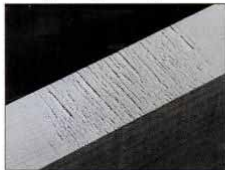
2 Prepare the stock for ripping by jointing one edge. If jointer tears out edge grain, reverse the board end for end.
