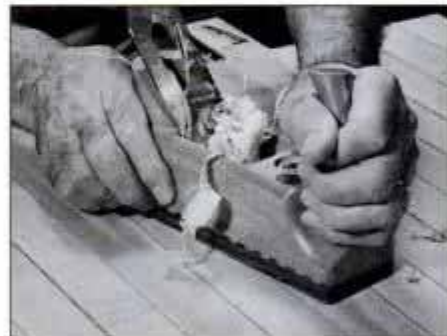
8 Aligning edge grain pays off during surface planing. Scrape off hardened glue, and surface top with a sharp smooth plane.
