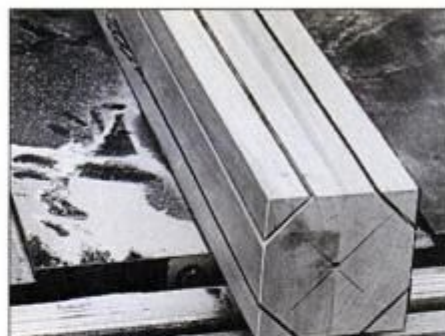
10 To make turning large leg blanks easier, make stopped bevel cuts on the table saw. Cut off scrap strips with a handsaw.
