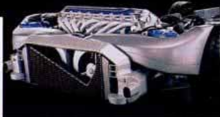
Most unusual feature of Ford Contour front-drive concept car is transverse-mounted inline 8-cylinder engine.
