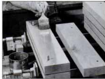
6 Quickly spread plastic resin glue with a short-bristle brush. Glue and clamp together top in at least two groups.
