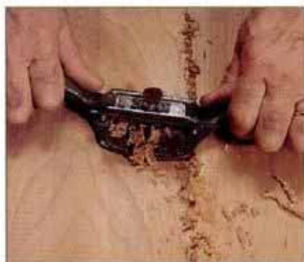
2 Use a sharp cabinet scraper to remove milling marks. A finely set, sharp hand plane will also work. Follow by sanding.
