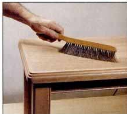
12 Carefully brush the work surface to remove stray abrasive grits when moving from coarser- to finer-grit sandpaper.
