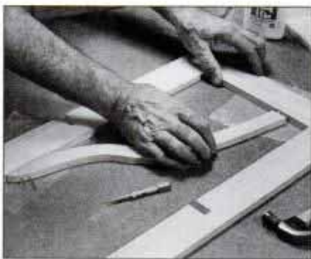
9 Secure slat with glue and two dowel pins at top and two nails at bottom. Drive nails after upper end is seated.
