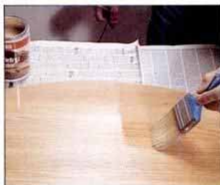
23 When the paste wood filler has thoroughly dried (about 24 hours), sand lightly, wipe clean, and apply a coat of sealer.
