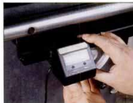
EMS unit slides on L-shaped channel to register fence distance. Unit will measure in .001-in., .005-in. or \frac{1}{32} -in. increments.
