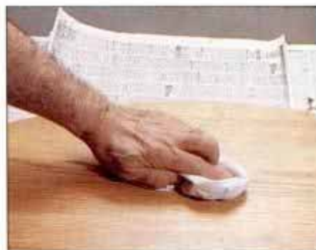
22 After wiping across the grain with a coarse cloth, use a soft cloth to wipe lightly, parallel to the grain direction.
