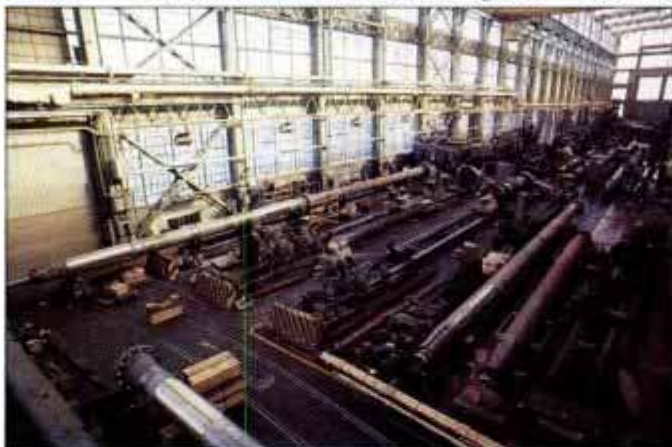
Huge tools at PNSY's machine shop will refurbish the carrier's propeller shafts.
