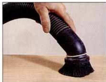
13 Clean and remove most of the excess sanding dust from the work with a vacuum cleaner and brush attachment.
