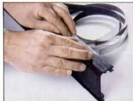
Capacitive tape is applied to L-channel, a Jet-Lock rip fence accessory. EMS unit reads distance based on position on tape.
