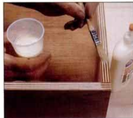
18 Apply water-diluted glue to plywood edges to seal end grain and prevent over-absorption of stain or paint.
