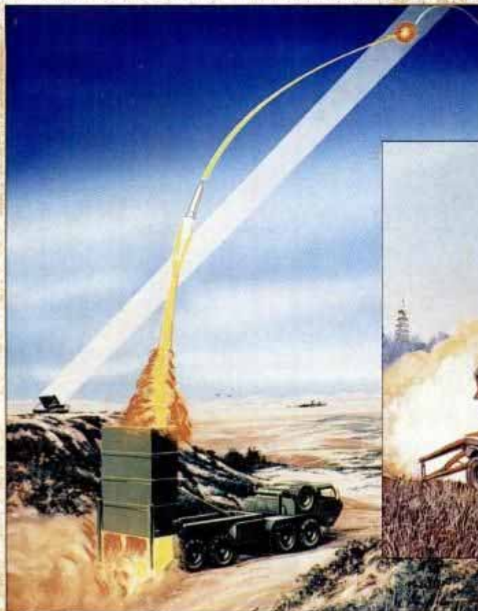
Two-tiered theater missile defense system starts with high-altitude THAAD interceptors (left). To pick off what THAAD misses, fire-and-forget ERINTs (right) blast from Patriot launchers.
