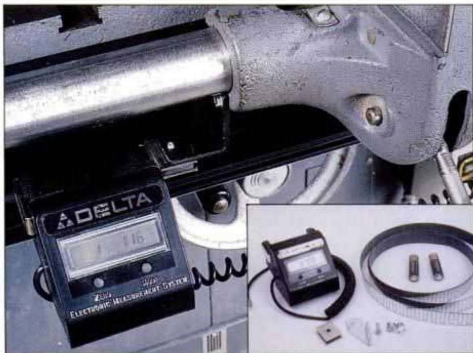
Mounted on a Unisaw with Jet-Lock fence, the Delta Electronic Measurement System accurately displays fence distance. Inset photo shows components for Unifence-equipped saw.
