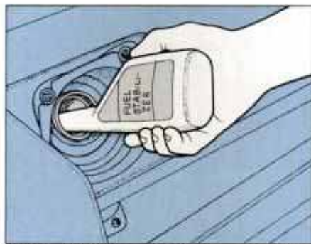
Add fuel-stabilizer additive to prevent varnishes inside the fuel system.
