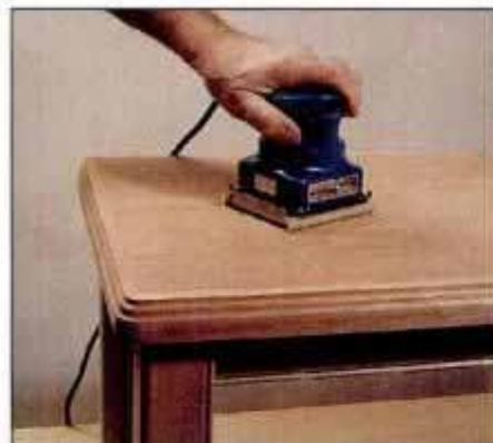
10 Use orbital sander to smooth all flat surfaces before finishing. Start with 100-grit, and work through grades to 220-grit.
