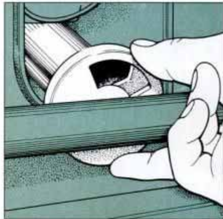
16 Set rotating-cap air-adjustment mechanism by turning cap to increase or decrease size of air-intake opening.
