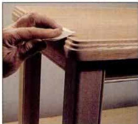
11 Finishes don't hold up well over sharp corners. Always ease corners by lightly sanding them to a slight radius.
