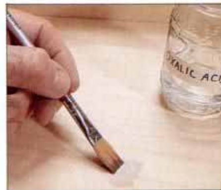
28 Localized stains and discolorations in the wood can be removed by spot bleaching with milder oxalic acid bleach.
