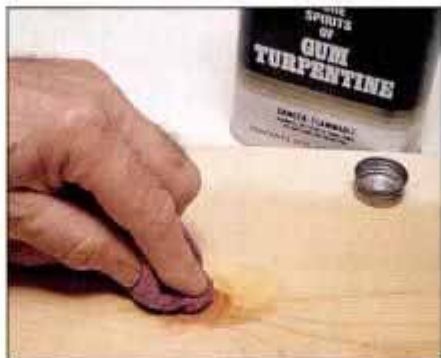
8 Remove sticky, resinous pitch from knots by wiping the knot with a solvent such as turpentine or mineral spirits.
