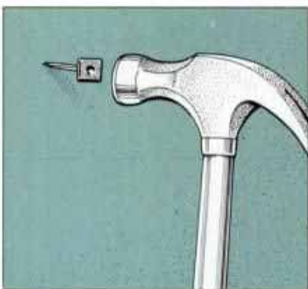
5A Place the pointed tip of the Wall Grabber against the wall. Then, drive the fastener in until it's flush with the surface.
