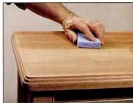
15 If water stain is used, first dampen the wood with a sponge to raise the grain. Let dry, sand lightly, and then stain.
