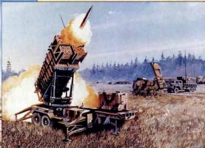
Two-tiered theater missile defense system starts with high-altitude THAAD interceptors (left). To pick off what THAAD misses, fire-and-forget ERINTs (right) blast from Patriot launchers.
