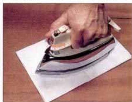
4 Use a damp cloth and hot iron to raise a dent. The steam causes compressed wood fibers to swell back to original size.
