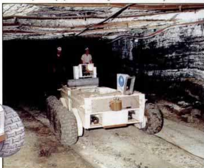
About 8 ft. long, Numbat is driven by twin electric motors, fed by a 48-volt battery. Range is about a mile and a half.
