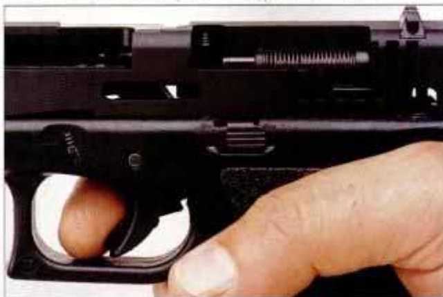
Cutaway shows first safety deactivated by touching trigger.
