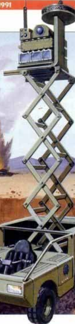
Surrogate Teleoperated Vehicle deploys day and night cameras, microphones, infrared sensor and laser designators on a 15-ft. scissor-lift mast.
