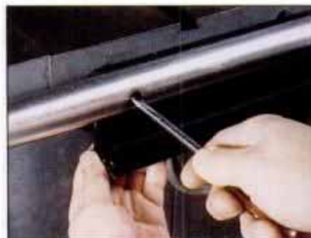
L-shaped channel replaces spacers normally separating guide rail and table. Accessory is necessary for Jet-Lock fences.
