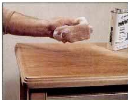
14 After finish sanding and vacuuming, remove all remaining traces of fine wood dust with a naphtha-dampened cloth.
