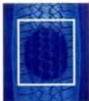
Wet or dry, this is all that touches the road: the contact patch.
