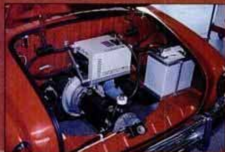
This battery meltdown was caused by a loose connection. VW engine bay shows electric motor bolted to stock transaxle, a common electric-car conversion.
