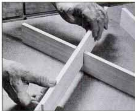
6 Check the half lap for proper fit. The joint should be slightly loose to allow for a couple of coats of finish on both sides.
