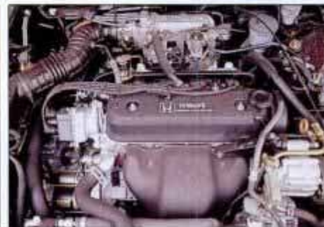
Accord's 2.2-liter sohc 16-valve Four is smoothed by dual balance shafts.
