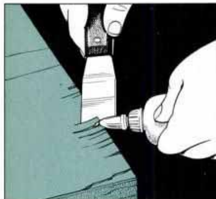
1A Use a putty knife to carefully lift any loose veneer around the damaged area. Apply white glue to reattach the veneer.
