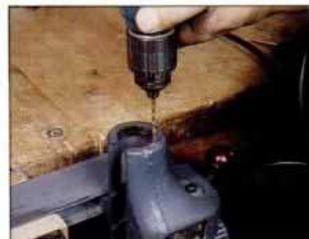
Holes must be drilled in the Jet-Lock fence body for attaching the magnetic bracket that secures the EMS unit to the fence.
