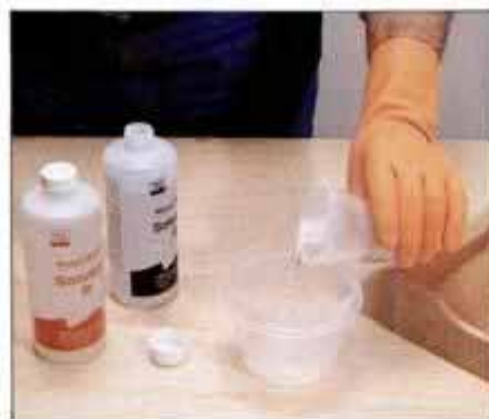
25 Use 2-part bleaches to lighten the wood tone. Wear rubber gloves and goggles, and mix components as directed.
