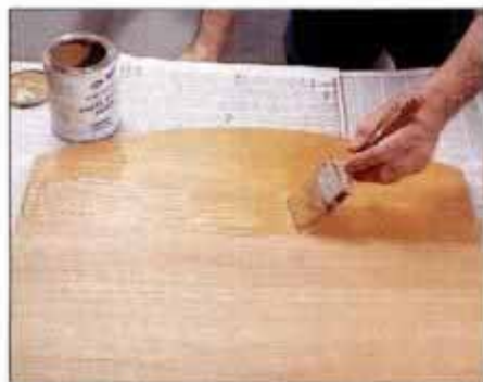
20 Use a stiff brush to apply paste wood filler. Stroke first with the grain, and then across the grain to pack filler into pores.
