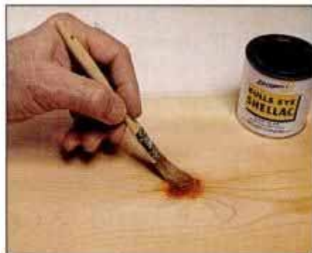
9 Seal knots with undiluted 3-pound-cut shellac. Apply two coats, sanding after each when dry with 220-grit paper.
