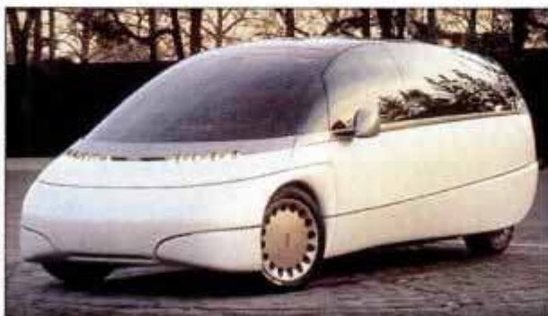
GM’s HX-3 concept car has a small gasoline engine, driving a large alternator to charge its battery pack. It can run in either hybrid gas-electric mode or as a pure electric when necessary.
