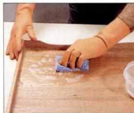
26 Apply the bleach solution with a synthetic sponge, and spread evenly over the surface. Bleaching action is immediate.
