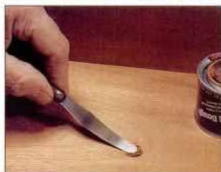
5 To repair small blemishes, use colored wood filler. Avoid over-spreading on coarse-grained woods such as oak.
