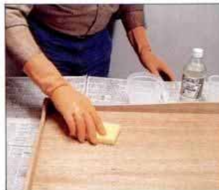
27 Neutralize the bleach residue with a solution of water and white vinegar, or as directed by the bleach manufacturer.
