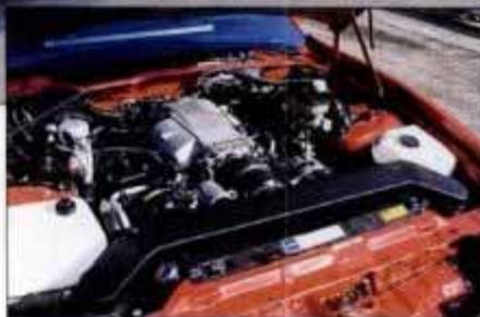
SLP-engineered and GM-built, this modified 350 V8 makes 350 emissions-legal horsepower, 390 ft.-lb. of torque.
