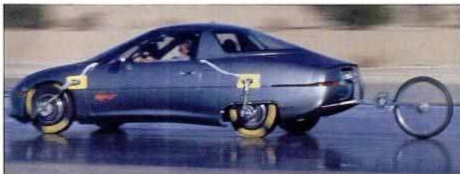
GM's Impact concept car uses conventional lead-acid battery technology.
