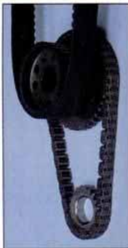
Smaller sprocket on crankshaft drives larger intermediate shaft sprocket, which carries lower camshaft drive-belt sprocket.
