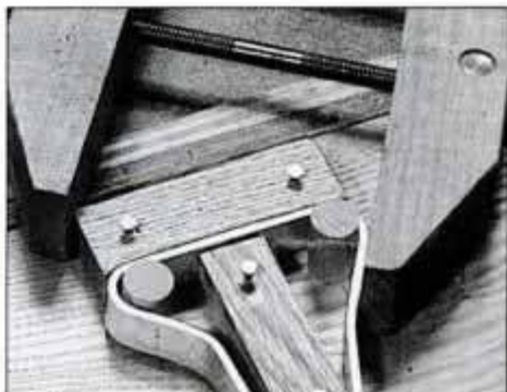
20 Complete handle forming by bending it with parallel jaw clamp. Nail scrap block to jig, and bend piece against block.
