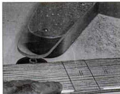
11 Pull slats against rounding-over bit in router table to ease corners. Leave slat edge square where it mounts to stake.
