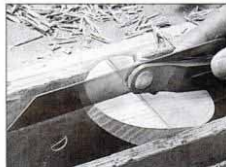
13 Clamp the lower disc in a vise, and bevel its face using a hand plane. Use a sliding T-bevel to gauge surface angle.
