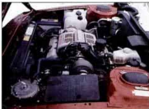
LeSabre's V6 required only a special LPG carburetor and pressure regulator valve for dual fuel use. Standard ECM controls metering.
