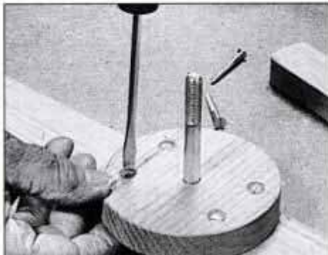
16 To form upper half of the steering assembly, insert the capscrew in disc. Then, glue and screw the disc to the cleat.
