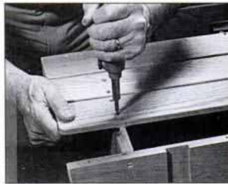
6 Screw together the wagon body using a modest amount of glue. Screw the floorboards to the front and back.
