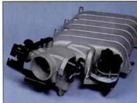
Single throttle body, plenum and upper intake manifold are rubber-isolated from heads by rubber mounts for reducing noise and vibration.
