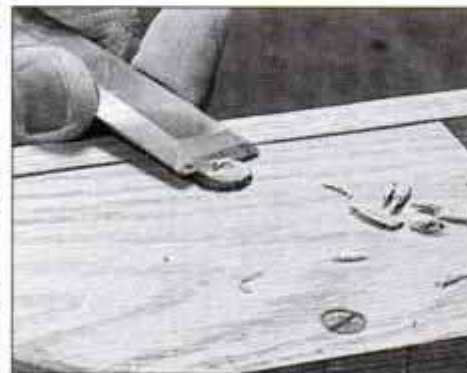
7 Glue and plug lower screwholes in wagon sides. When the glue is dry, pare plugs flush to the sides with a sharp chisel.
