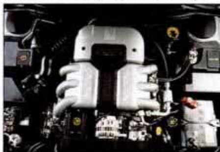
Swoopy styling and excellent cockpit layout help make new Subaru SVX a serious contender in the sports-coupe derby. New dohc 24-valve flat Six engine produces 230 hp.
