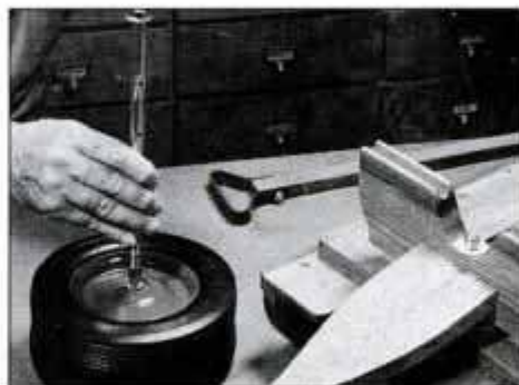
22 When paint on rims is dry, stack wheels as shown and drive axle through both at one time. Fasten axles to bolsters.
