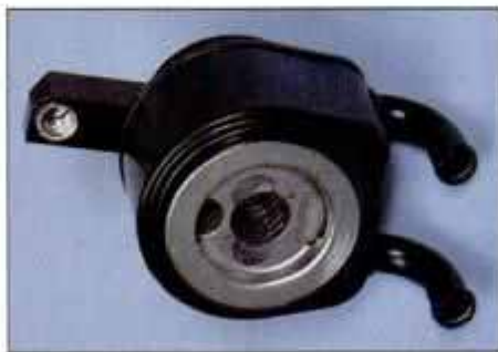
Oil-to-water heat exchanger reduces oil temps under heavy loads, as well as aiding in warmup of oil during cold weather.
