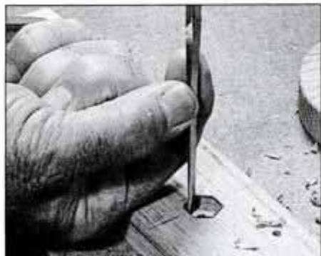
15 Bore a hole in the front cleat, and chisel hole into a hexagon-shaped mortise. Capscrew's hexagon head fits mortise.
