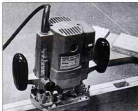
4 Clamp sides together, and use a router and rounding-over bit to soften the corners at the top and bottom of the dados.
