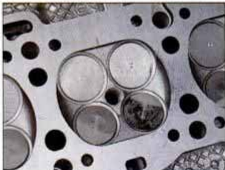
Mild pent-roof combustion chamber with central spark plug has 9.25:1 compression ratio, permitting use of 87-octane fuel.
