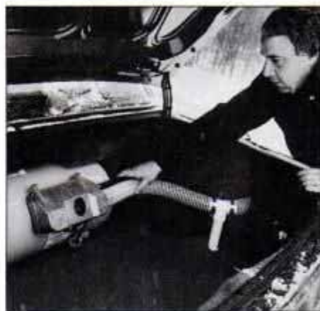
Pressurized LPG tank consumes a sizable portion of LeSabre's generous cargo space.
