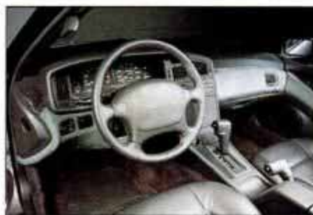
Swoopy styling and excellent cockpit layout help make new Subaru SVX a serious contender in the sports-coupe derby. New dohc 24-valve flat Six engine produces 230 hp.
