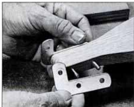
18 Cut handlebar brackets from flat corner plates. Round off the corners and edges, then check them for fit over screws.
