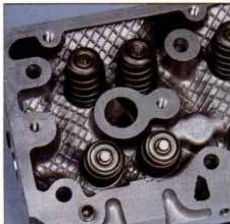
Paired intake and exhaust valves are actuated by lifters riding in cam carrier bolted directly above cylinder head.
