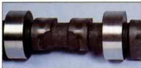
Camshaft lobes are undercut on base circle to make hydraulic lifters rotate slowly and minimize cam noise and lifter wear.
