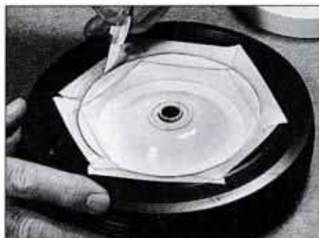
21 Prior to painting, tape over the rim and tire. Silt tape between rim and tire with razor knife. Peel off the tape from the rim.
