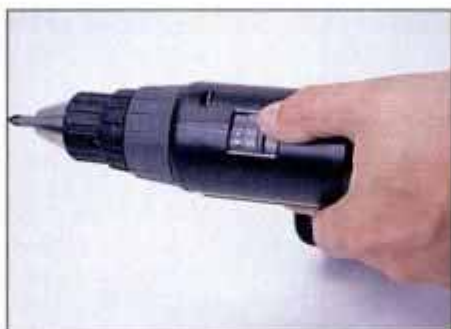
Top-mounted sliding switch shifts gears to change speed range from low (50 to 350 rpm) to high (150 to 1000 rpm).
