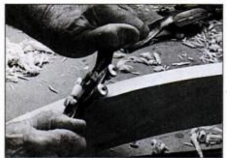
11 Cut the rail's outside curve on the band saw, then use a spokeshave to smooth away the saw marks and refine the curve.
