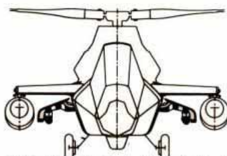
Self deployment: Drop tanks provide 1260-mile range, with two Stingers.
