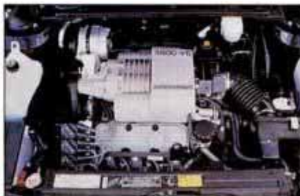
Supercharged 3800 V6 gives Buick Park Avenue Ultra 205 hp, 260 ft.-lb. of torque.
