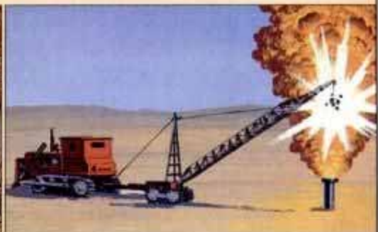
Dozer-pushed Athey wagon clears wreckage and delivers explosives as hose cools debris.
