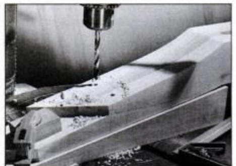
15 Use the drill press to bore pilot holes for the screws that attach armrest to rear leg. Scrap wedge positions the leg.
