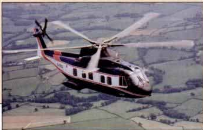
EH101 (below) has four ACSR actuator/strut: between the gearbox and airframe. The result: 75% less vibration.
