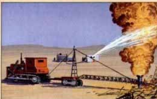
Dozer-pushed Athey wagon clears wreckage and delivers explosives as hose cools debris.
