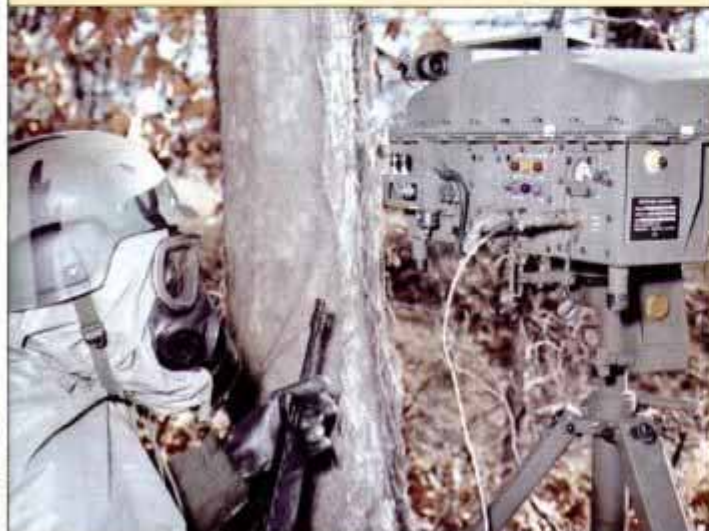
Fuchs N.B.C. recon vehicle (above), an amphibious 6-wheeler, is outfitted with detection gear. XM21 (below) identifies remote toxins from their infrared signature.
