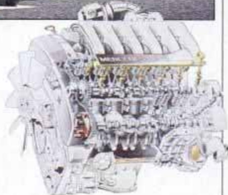
Potent new 408-hp 6.0-liter dohc 48-valve aluminum V12 is also silky smooth.
