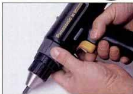
Gray clutch ring behind chuck adjusts maximum torque to one of five settings. A sixth position locks the clutch for boring.
