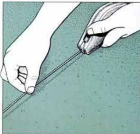
6 Determine the tile layout, then snap two perpendicular chalklines as a guide for laying the first course of tiles.
