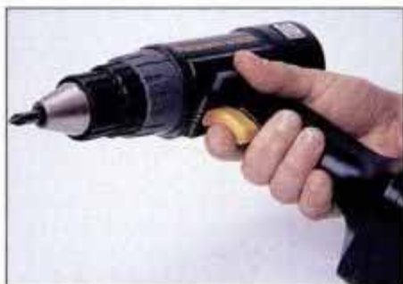
Directly above trigger is FORWARD/REVERSE switch. Keyless chuck has two rings that are tightened against one another.
