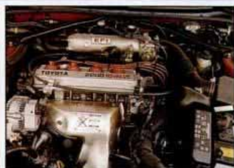
Toyota's 130-hp dohc 16-valve 2.2-liter Four powered 56.5% of Celicas in survey.
