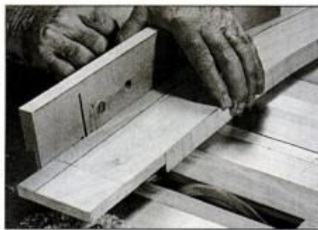
10 On each half of the arched rail, first cut the inside curve. Make a flat edge tangent to the curve, then cut the half lap.
