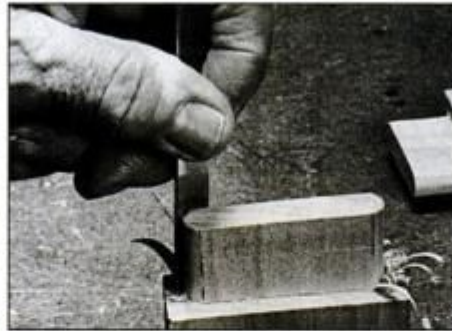
8 Round off edges of tenons with a chisel to fit mortises. Other option is to square the ends of the mortise instead.
