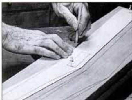
2 Make the patterns for the rear legs, including mortise positions, from cardboard. Trace patterns onto stock.
