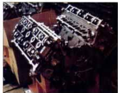
The 300-hp dohc 32-valve aluminum-alloy 4.6-liter V8 will debut in 1993 Mark VIII.
