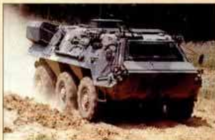
Fuchs N.B.C. recon vehicle (above), an amphibious 6-wheeler, is outfitted with detection gear. XM21 (below) identifies remote toxins from their infrared signature.
