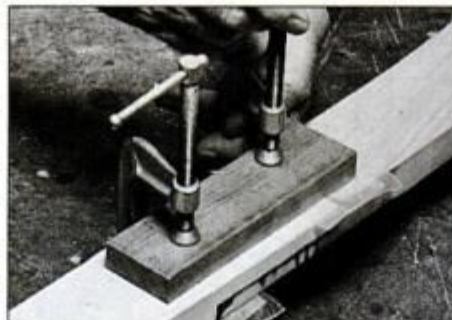
12 Glue and clamp the halves of the arched rail together with blocks on each side. Wax paper keeps glue off blocks.
