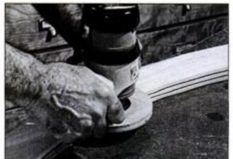
13 Cut the groove in the arched rail using a slotting cutter and router in a series of passes. Clamp stopblock to rail.
