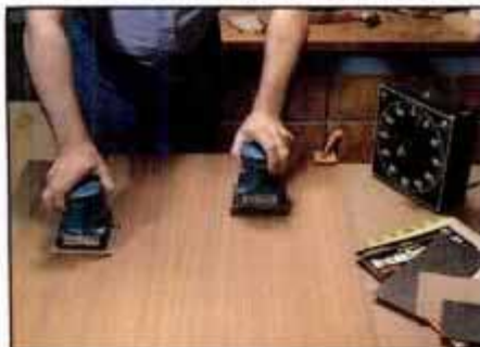
1 Foam-backed and regular sandpaper were equally durable when used on a flat surface during 5-minute sanding test.
