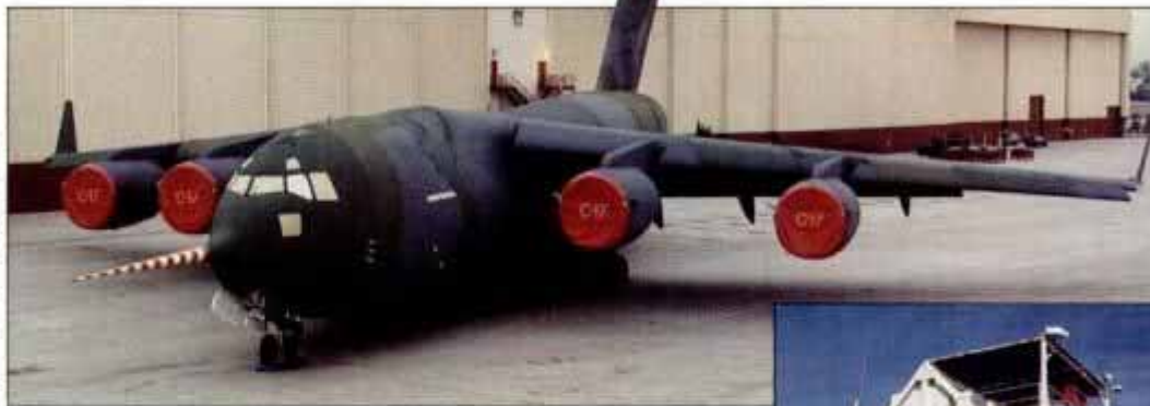
The C-17 (above) relies on winglets and blown-flap system (shown being tested, right) for lift on steep approaches to short runways.
