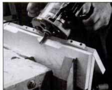
15 Cut chamfers with router and straight bit. Jig holds router at 45°, and small stop-blocks shape chamfer ends.
