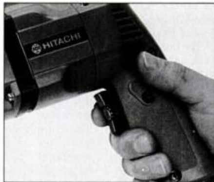
Trigger-lock button is usually under right thumb—lefthanded use is difficult. Note speed dial in trigger (Hitachi and Sears only).
