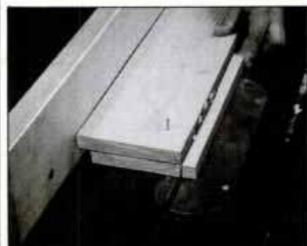
13 Tack a 1 x 6 to a post side so it's aligned with post taper. Hold the guide strip against the table saw fence to saw taper.
