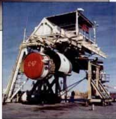
The C-17 (above) relies on winglets and blown-flap system (shown being tested, right) for lift on steep approaches to short runways.
