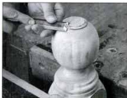
38 After the post is removed from the lathe, saw off waste and trim top of post with sharp chisel. Then sand.
