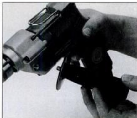
Auxiliary handles are generally attached by threading them into housing side. They provide control in high-torque situations.
