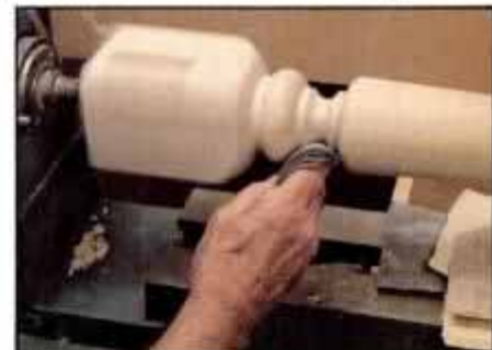
3 The flexible abrasive sheet is ideally suited for sanding lathework. Here, one folded sheet sands cove on table leg.
