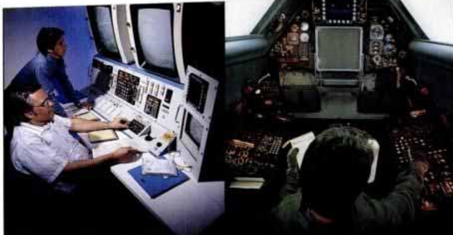
Updated Slinger-Link simulator is the centerpiece of NASA's air crew training program. Instructor's panel (left) governs all displays and controls in the simulated RSO station (right).
