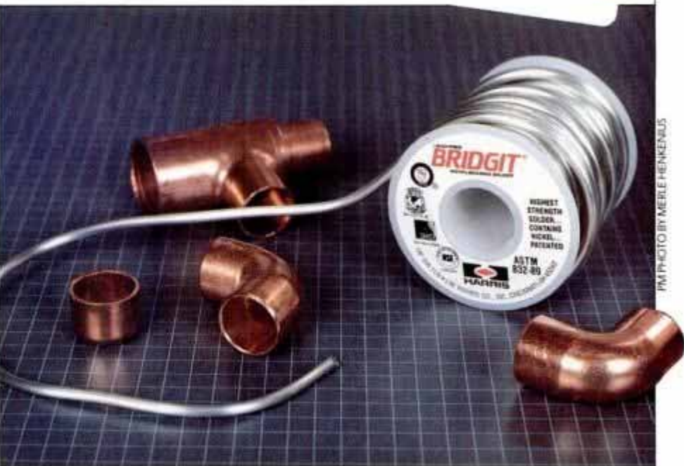
Lead-free solders melt at higher temperatures than the older, mostly lead types. Once you learn how to use them, you'll solder as much as you did before.
