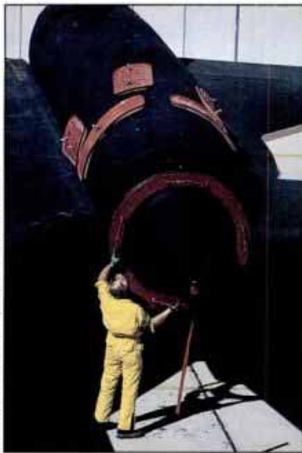
Complex SR-71 maintenance includes work on the mighty J-58s.
