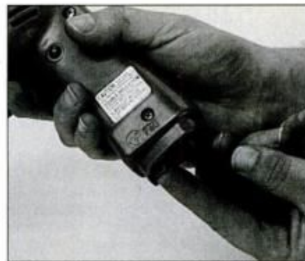
Makita (shown) and Ryobi drills have toggle-type FORWARD/REVERSE switch located at the bottom of the handle.
