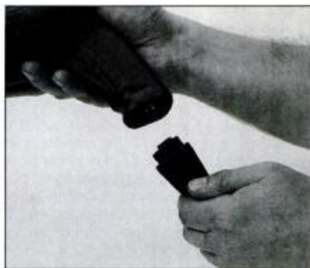
Milwaukee 0224-1 has a plug-in cord to facilitate cord replacement. Note extra-large variable-speed trigger on inside of handle.
