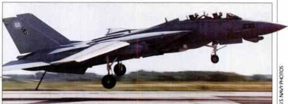
Reengined Tomcat made it through catapult steam ingestion testing (left) and high sink-rate landings (above) at Patuxent River, before beginning carrier suitability tests.
