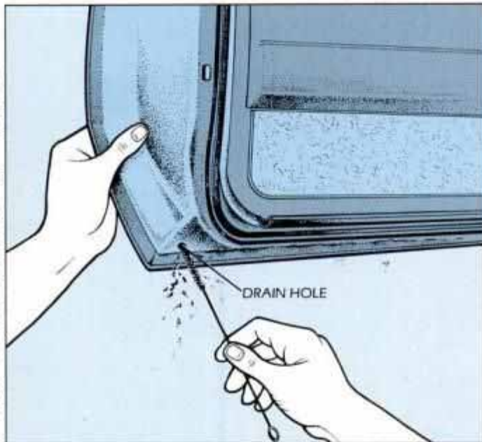
Periodically clean the drain holes in the lower parts of body panels to prevent moisture from accumulating.
