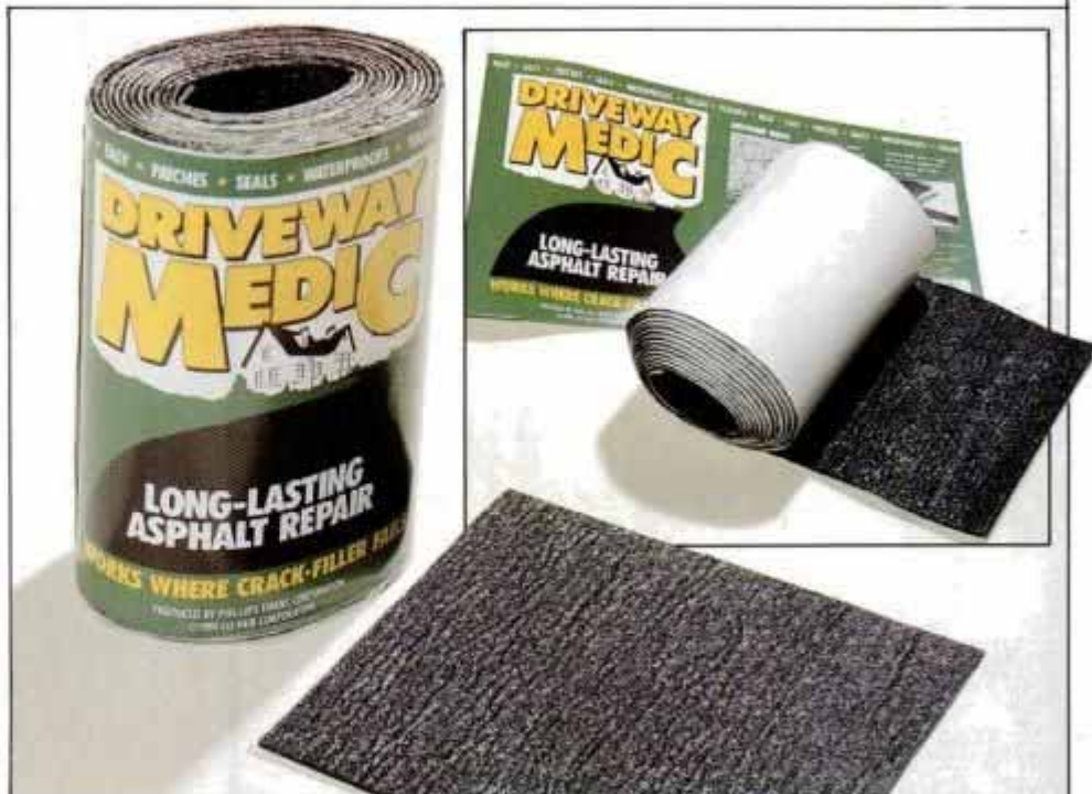
Driveway Medic is a durable adhesive-backed polypropylene fabric impregnated with rubberized asphalt. Apply it over driveway cracks as if it were a piece of tape.
