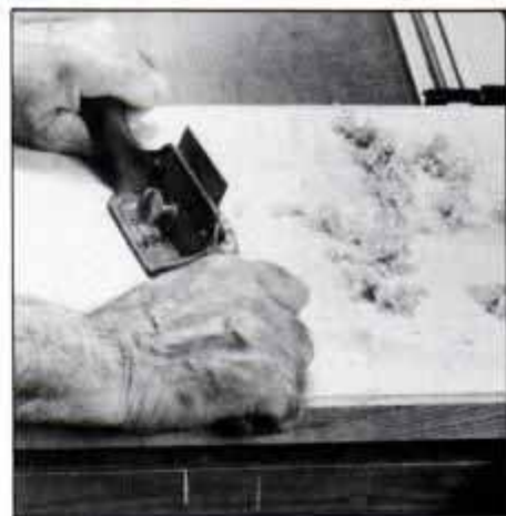
7 After the glue has dried, clean off the surface with a cabinet scraper. This also reduces the amount of sanding necessary.
