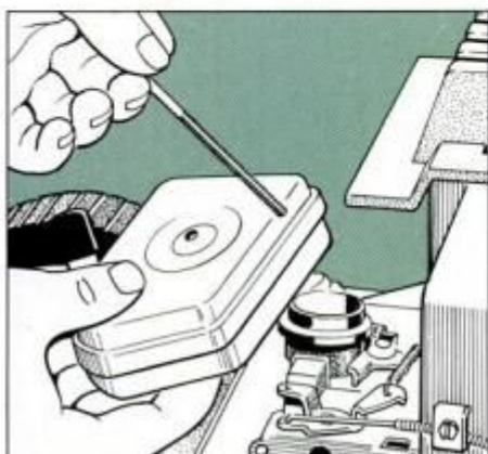
5B Use a screwdriver to loosen the slotted bolt that holds the air cleaner. Clean the filter element or replace it.
