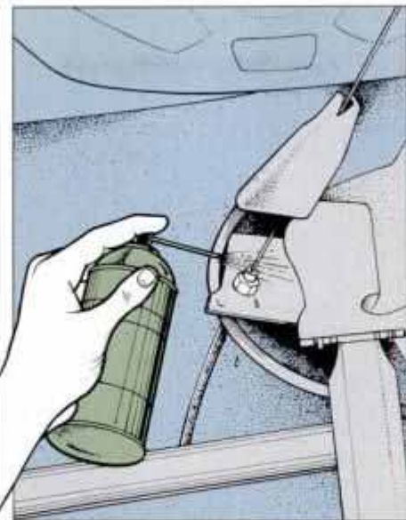
Lubricate handbrake cable and mechanism to prevent corrosion or dragging brakes.
