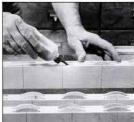
4 Glue the biscuits into one side of each member (except last member). A small squeeze bottle makes dispensing easier.
