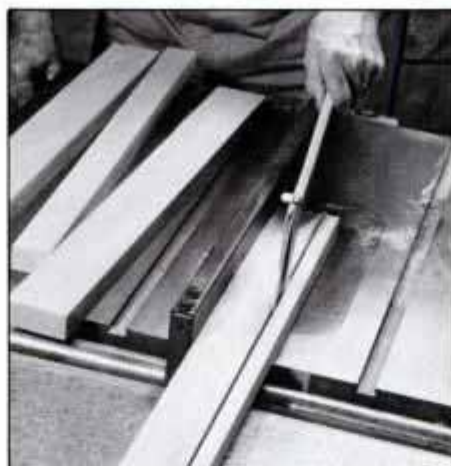
1 Rip wide boards to narrow widths, then reassemble them with their annual rings alternately inverted to prevent warping.
