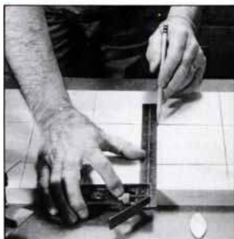
2 Align the pieces and mark for cutout and biscuit slot centerlines. Leave ample clearance for biscuits around the cutout.
