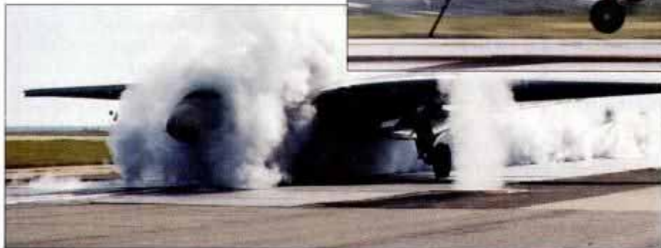
Reengined Tomcat made it through catapult steam ingestion testing (left) and high sink-rate landings (above) at Patuxent River, before beginning carrier suitability tests.
