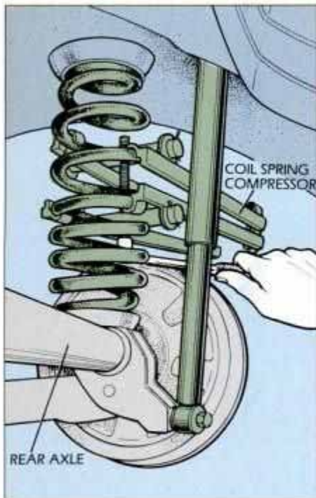
A spring compressor can be rented for the afternoon to replace coil springs.
