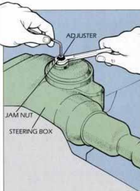
Adjusting your steering box requires an Allen wrench and a box wrench.
