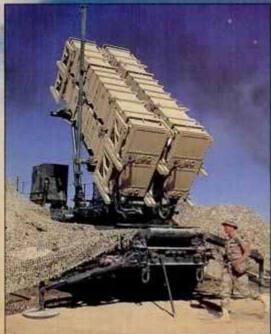
Launcher hot-crew member runs to turn torque tube handles, the last step before missiles can be fired.
