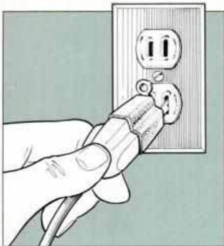
Adapters should not be kept on electrical cords, as shown. They should be attached to the outlet with the covering plate screw.
