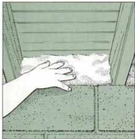
To reduce air infiltration, caulk between the sill and foundation, and install batt insulation between the joists above the sill.
