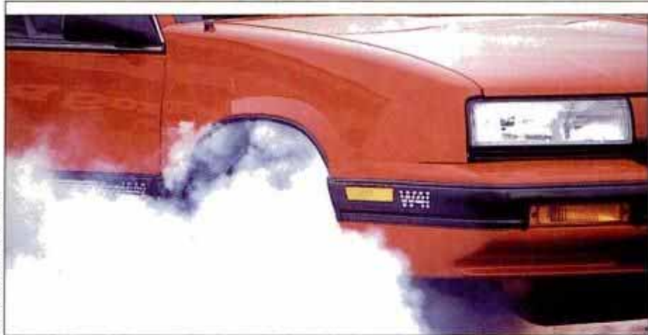
With 190 hp and only 2518 pounds of car, the W41 option on the Olds Cutlass Calais creates plentiful launch power. Injection system tweaks account for most of the gain, 10 hp more than the standard high-output Quad 4.
