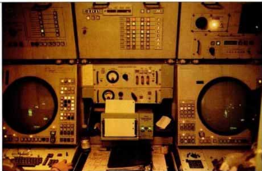
Air war is fought in the ECS (above) by TCA at left and TCO at right. Green lights at top center show launchers okay to fire, and white numbers to right give missile count. At change of shifts, Sgt. Stonestreet briefs ECS crew (below left) and replaces air filters (right).
