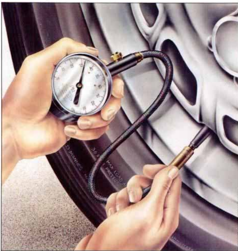
Proper cold inflation pressure is critical to tire performance and lengthening the tire's life.
