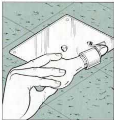
Ceiling light fixtures that provide little clearance around the bulb will easily overheat if improper high-wattage bulbs are used.
