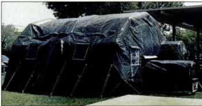
Army's chem-war shelter with airlock deploys from the back of a dedicated HMMWV in less than 20 minutes.
