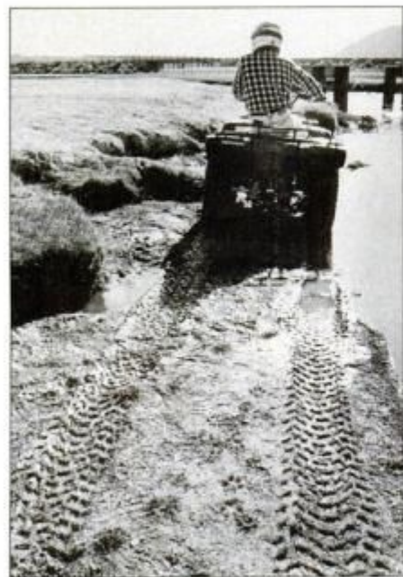
Wide, deep-lug ATV tires leave a lasting impression. Drive around soft, wet soil.
