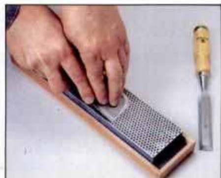
2 Coarse diamond hone shapes plane iron and chisel bevels. Nonwearing surface helps to ensure straight cutting edge on tool.
