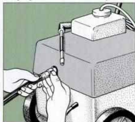
1 Electric power washer uses high-pressure stream of water to remove paint. Attach to water supply with garden hose.
