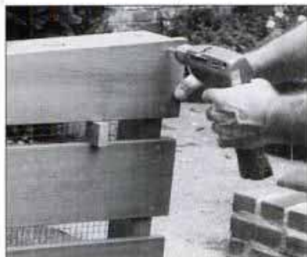
13 Screw slats to end frames. For correct spacing, support each slat while fastening with \frac{1}{2} -in.-wide blocks.
