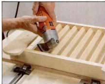
Unique design also permits working in confined spaces such as in between louvers where ordinary sanders can't reach.
