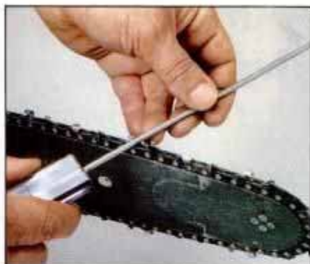
7 Diamond chain-saw file is said to outlast ordinary files. It comes in the extra-coarse grade and in three diameters.
