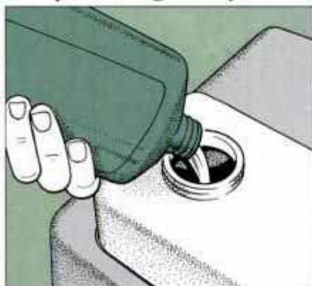
2 On washer with reservoir, pour cleaner into reservoir and set mixture control. Washer mixes cleaner with water stream.
