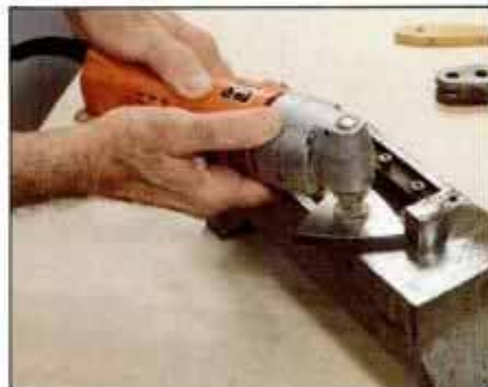
Vigorous metal sanding can overheat Velcro pad. Peel-and-stick pad and adhesive-backed sandpaper are recommended here.
