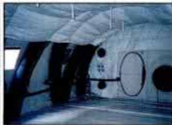
Army's chem-war shelter with airlock deploys from the back of a dedicated HMMWV in less than 20 minutes.
