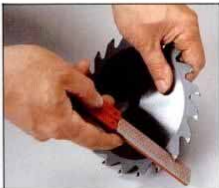
6 Small 4-in. diamond sharpener is handy for touching up faces of dull teeth on carbide-tipped circular-saw blade.
