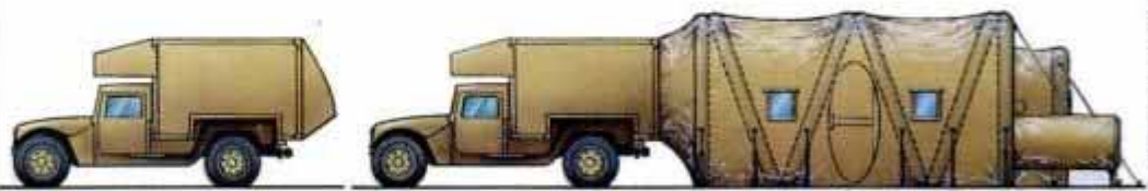
Army's chem-war shelter with airlock deploys from the back of a dedicated HMMWV in less than 20 minutes.
