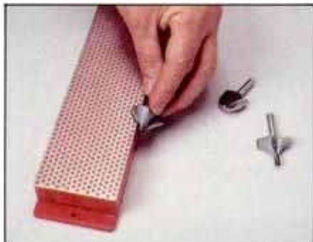
3 High-speed steel and carbide-tipped router bits can be sharpened with industrial diamonds. Hone flat face of cutter.
