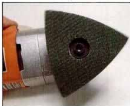
Pad oscillates back and forth through 2° arc at 20,000 oscillations per minute. Pad can be rotated to utilize entire sheet.
