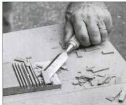
15 Clean out between the kerfs with a sharp chisel. The overlap's depth equals half the stock's thickness.
