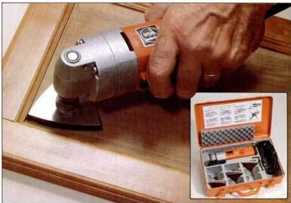
The Fein triangular-pad sander easily sands into corners without marring adjacent surfaces. It comes in a carrying case (inset) with wrenches and Velcro-backed sanding sheets.
