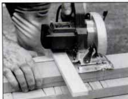
1 For neat crosscuts, make a T-guide from scrap wood. Run saw's shoe against guide for straight and bevel cuts.
