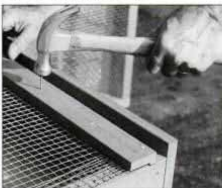
9 Nail front and rear runners to the frame. The rear runner is notched to accommodate the mesh's fold at the corner.
