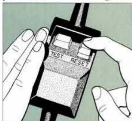
3 Washer units require ground fault circuit interrupters. This model has handy TEST and RESET buttons built into electrical cord.
