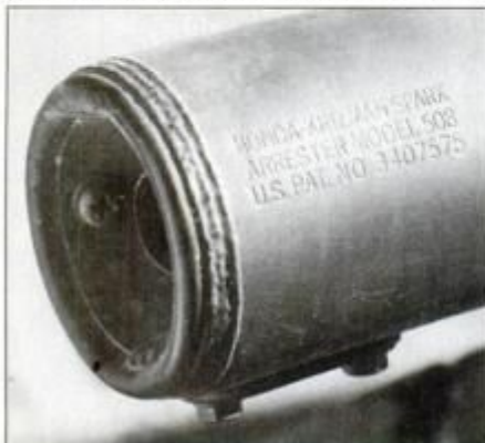
This stock exhaust pipe comes with an approved spark arrester. Don't replace it.
