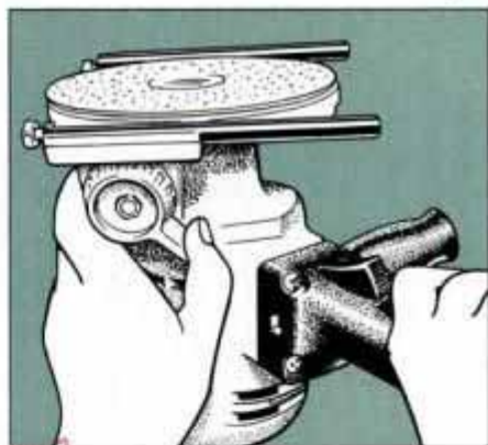
18 Grinder removes paint smoothly because one side of disc is higher. Side knobs raise and lower side support bars.
