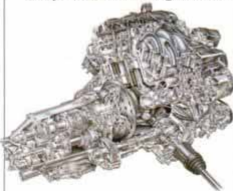
Legend's new 200-hp 3.2-liter sohc 24-valve V6 mounts longitudinally.
