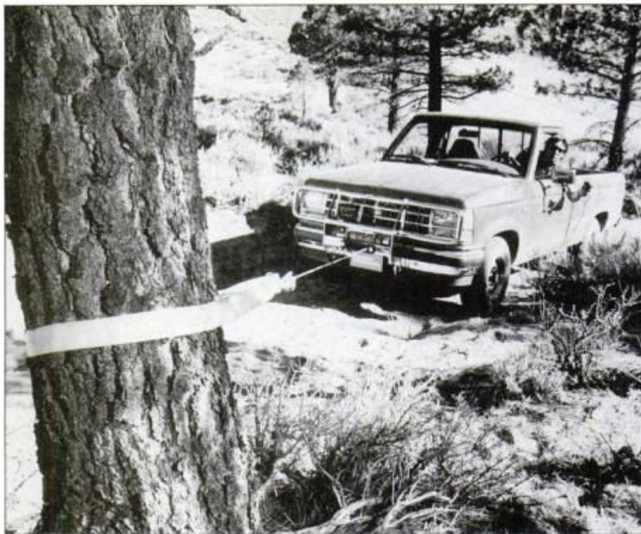
Use a tree-saver strap, instead of bare cable, to prevent bark damage during winching.
