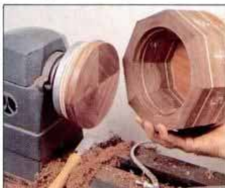
24 Then, attach the bottom piece to lathe faceplate and turn down diameter until the piece fits snugly in bowl rabbet.
