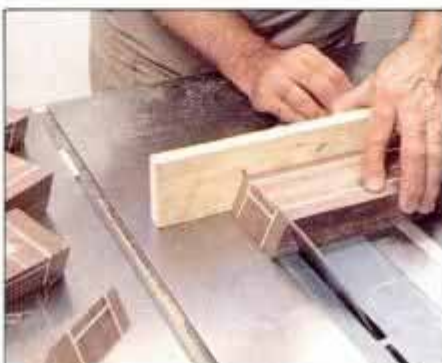
20 Miter laminated stock into eight equal segments. Number each piece in order so grain will be continuous in final assembly.
