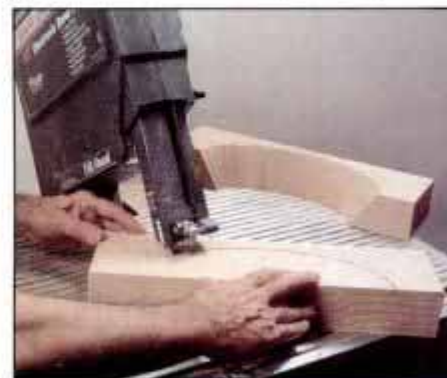
6 After sawing bowl blank along centerline, set band saw for 30° bevel and cut to the inside wall line on each blank half.
