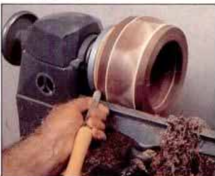
26 Shape the outside profile of the bowl while periodically checking the design. Stop when contour and pattern look right.
