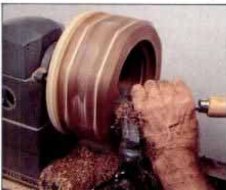
23 Mount bowl blank on lathe and use a skew chisel to shape rabbet on inside bottom edge of ring for bowl bottom.
