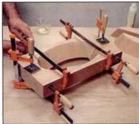
7 Glue the two sections back together to form a single block. Headless nails in waste area serve to keep pieces aligned.
