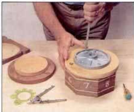
22 Glue plywood discs to top of bowl and to mitered walnut bottom piece. Discs permit work to be secured to lathe faceplate.
