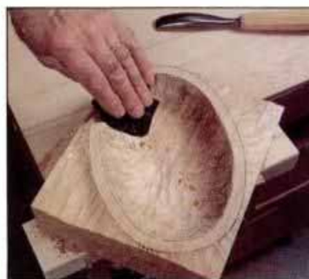
4 Rub carbon paper in bowl to mark high spots for trimming. Shape outside by carving or band sawing at bevel, then sand.
