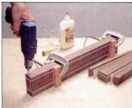
19 Sandwich of contrasting poplar plywood and walnut is made in two stages. Holes for alignment nails go in waste area.
