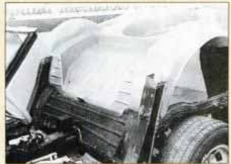
Rear tub assembly installs in stock location of original tub. Note the well in trunk area for 16-in. spare tire.
