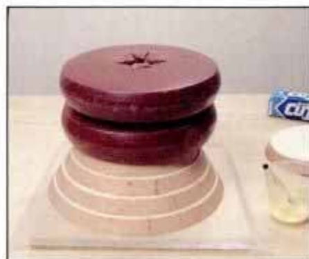
12 Apply glue to all mating surfaces and allow to become tacky before assembling. Then, use weights for uniform pressure.
