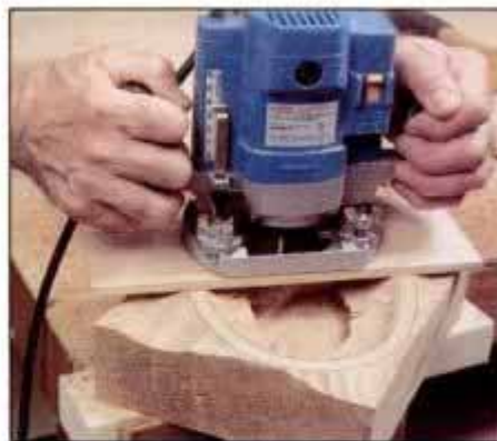
2 Use a router and 3/4-in. corebox bit to quickly remove waste at center. Oversize base supports router on bowl perimeter.
