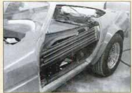
Modified door with repositioned crash beam is test fitted on car. New skin is bonded on to match body contours.
