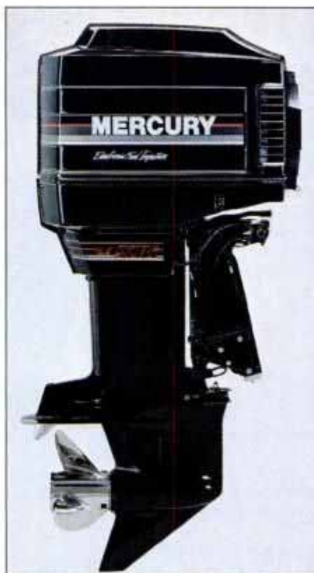
The 2.5-liter XRI continues Merc's industry leadership in electronic fuel injection. Displacement moves up from 142 cu. in. to 153 cu. in.
