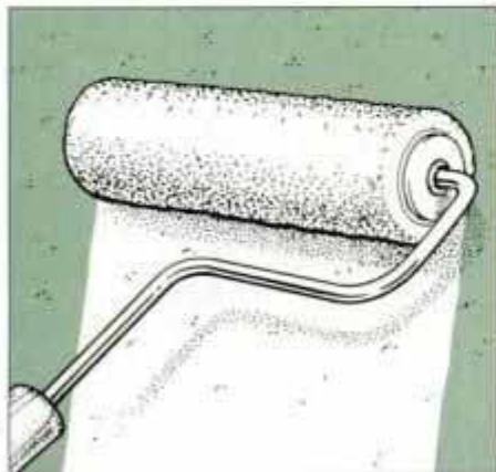
15 Use a roller with a nap length more than ½ in. to paint rough surfaces, like textured stucco walls or ceilings.
