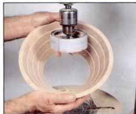
14 For final smoothing, use a large diameter drum sander. Then, glue bottom in place, complete sanding and apply finish.
