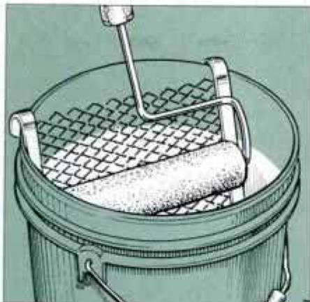
13 To paint a large area, hang a roller screen in a 5-gallon paint pail filled with a couple of gallons of paint.
