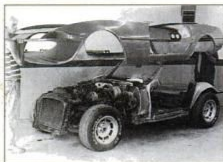
Lightweight, handmade, 1-piece reinforced body is lowered onto chassis and secured by stock mounts.
