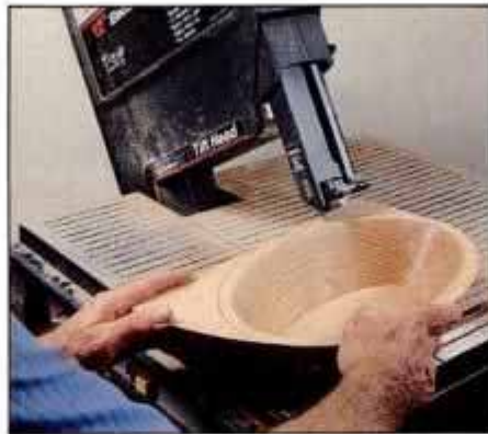
8 After smoothing inside walls and gluing bottom to bowl blank, saw to bowl outside line with the band saw set at 30°.
