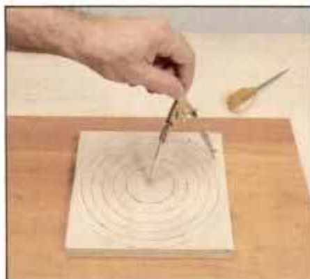
15 Use a compass to lay out the series of circles. Bore a \frac{3}{16} -in.-dia. blade entry hole on each ring for the scroll saw blade.
