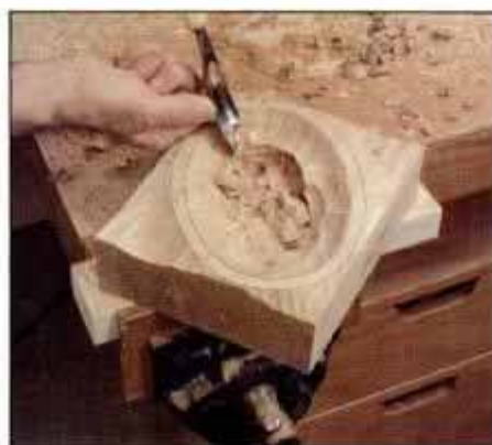
3 After most of the waste has been removed with the router, resume with bent gouge until desired shape is achieved.
