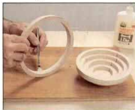
17 Apply glue to contact areas of rings. Align and press each ring into the next and let the glue dry. Clamping is unnecessary.
