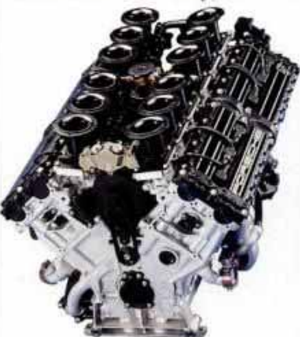
Porsche returns to F1 in '91 with this new 80° V12. The V12 will ride in an Arrows chassis.
