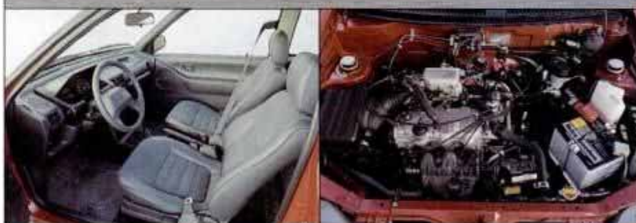
Charade's tiny 3-cylinder engine was rough but willing, and delivered 47.2 mpg on PM econo loop. Front-seat legroom was good, and overall quality was impressive.
