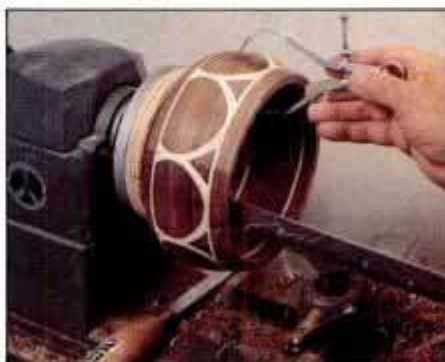
27 Turn inside wall of bowl with bowl scraper or roundnose turning tool. Check wall thickness regularly with caliper.
