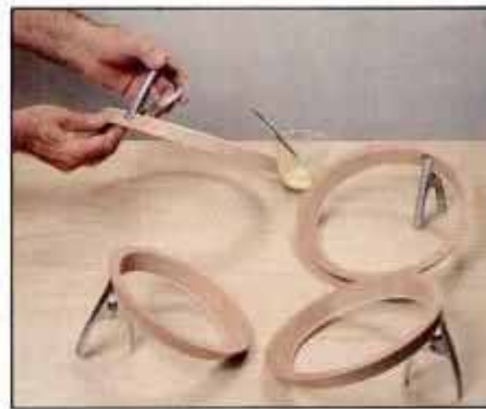
11 Glue together entry cuts on each ring before assembling rings. Small spring clamps apply pressure until glue sets.
