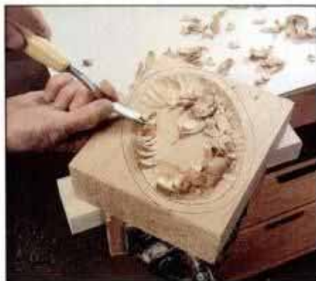
1 Hold carving blank in vise by means of a 2 x 4 screwed to waste area. Bent gouge shapes inside bowl wall near edge.
