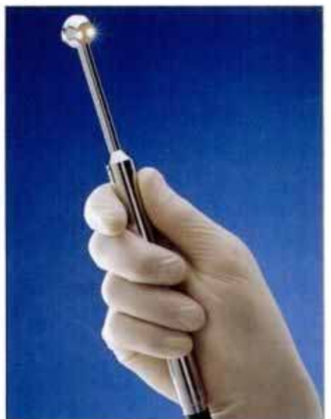
Tiny light, air jet and video camera are incorporated in Fuji DentaCam (above), which produced the image at left.
