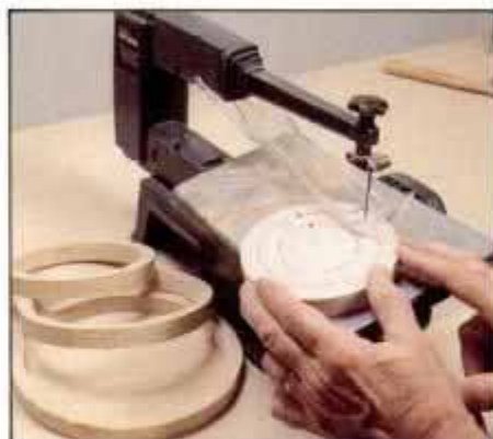
16 Tilt scroll saw table to about a 5^\circ angle to cut beveled rings. Use larger angle to reduce telescoping if kerf is too wide.
