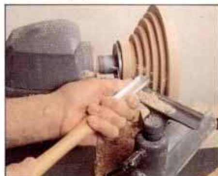
18 Mount work on lathe faceplate. Use sharp gouge to trim steps on bowl surface. Stop cutting when steps disappear.
