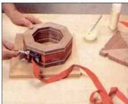
21 After carefully aligning parts, use band clamp to hold ring segments in place after glue is applied to mating surfaces.
