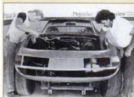
Front inner fenders anchor body to chassis along with header support rods that attach to front frame extension.
