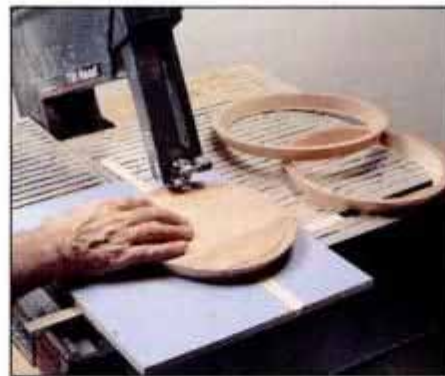
10 Circle jig guides 30° cut when making 7/16-in.-wide rings. Circles also can be drawn with a compass and cut freehand.
