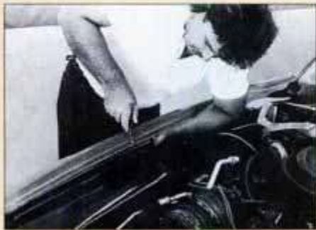
Inner fenders are held in place by self-tapping screws and later bonded. They also attach to the radiator support.
