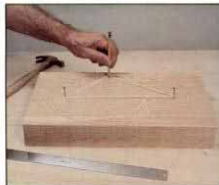
5 Lay out ellipse with two nails and string loop. Ellipse size and proportion are controlled by nail placement and string length.
