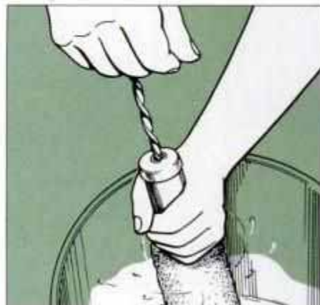
17 Spin dry a roller after you wash it. Hold it in a bucket and pump paint spinner handle. Spinner also works on brushes.
