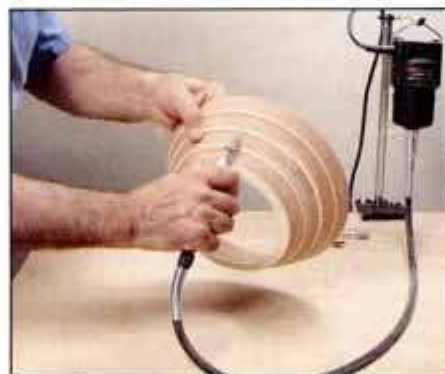
13 Level the inside and outside of bowl walls with rasp or flexible drive tool. Bottom is installed after smoothing.
