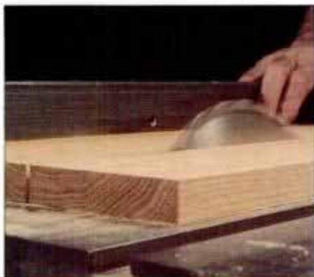
When ripping hardwood, blade stays cooler if it's raised at least 1 in. above stock. The saw guard is removed for photo clarity.
