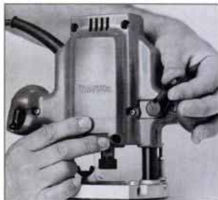
A lever is used to lock plunging action. P-C lever is spring loaded in the lock position. Elu incorporates lock in the right handle.
