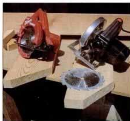
Portable saws with thin-kerf blades cut with much less effort. Rough diagonal cuts show evidence of blade wobble.
