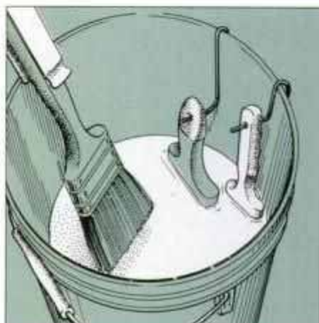
17 Suspend brushes in thinner at the end of the day. Keep the paint brushes off the bottom by using brush hooks or clips.
