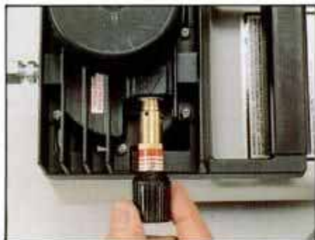
1 Adjust output pressure by turning the knob on top of compressor. Pressure is infinitely adjustable between 10 and 100 psi.
