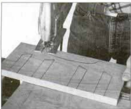
10 Lay out dadoes and curved cutout on stand base. Make curved cut with a jigsaw. Remove saw marks with rasp, then sand.
