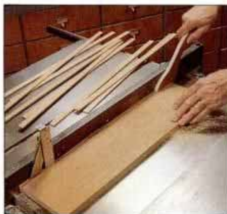
Ripping very thin strips for edge banding produces a slightly greater yield and less waste with a thin-kerf blade.
