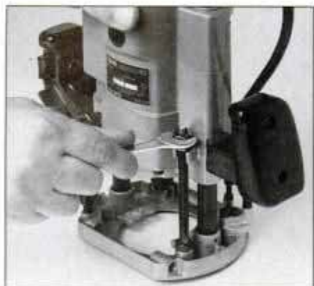
Set bit depth for edge trimming or router table work with threaded rod and nuts at back of Ryobi tool. Hitachi and P-C are similar.
