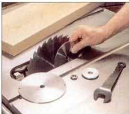
Blade stabilizers reduce vibration to help produce a finer cut. When cutting thick stock, a smaller diameter stabilizer is necessary.
