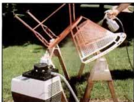
4 Air delivery was smooth and steady for spraying paint, even heavy-bodied materials such as rust-inhibitive primer.
