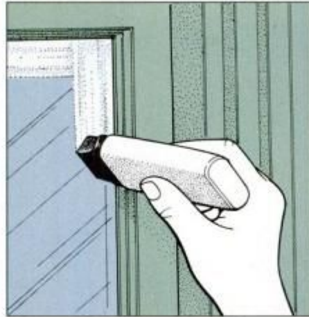
5 Rub sealant on glass before painting. Afterward, scrape the window clean with a retractable razor scraper.
