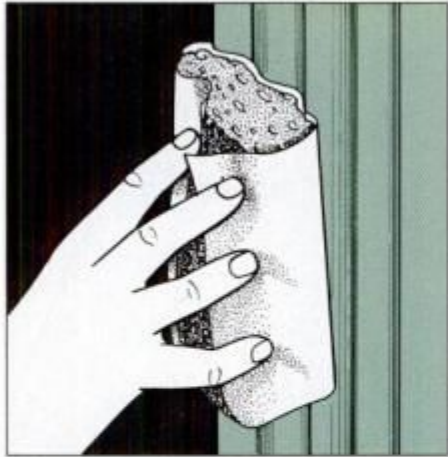
4 Wrap sandpaper around a sponge to sand curved areas, like window or door trim. Sponge takes on molding profile.
