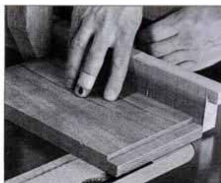
12 Rip a 6-in.-wide x 10\frac{11}{16} -in.-long piece and cut the tenons on both ends. From this, rip the stretcher and handle.
