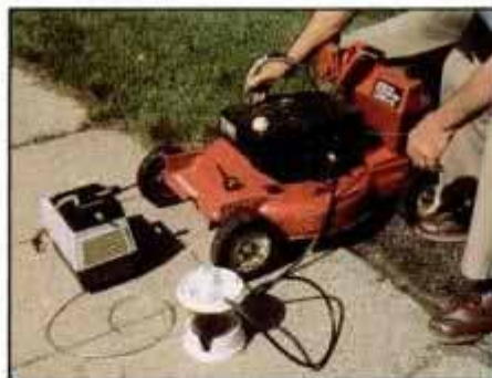
2 Oil-Vac is quick, easy and clean to use. Compressor draws vacuum through 40-ounce jar and sucks oil out of 4-cycle mower.
