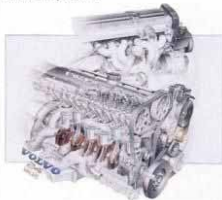
New aluminum alloy 24-valve dohc inline-Six is still one year away from U.S. debut.
