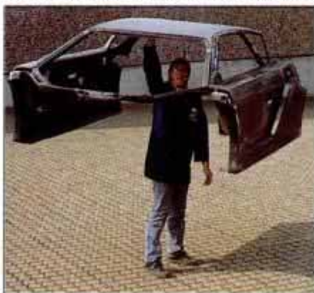
Zender Fact 4 carbon-fiber/aramid body shell weighs just 122 pounds.
