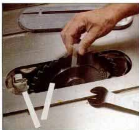
To help correct a blade that has a slight wobble, carefully positioned paper shims are placed between blade and stabilizer.
