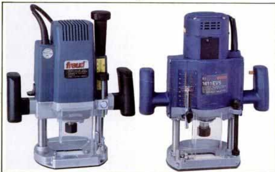
Heavy-duty plunge routers are offered by most manufacturers, and combine power and versatility. The Freud FT2000 (left) boasts 3½ horsepower, and the 3-horsepower Bosch 1611EVS (right) has electronic variable speed with soft start to reduce starting torque.
