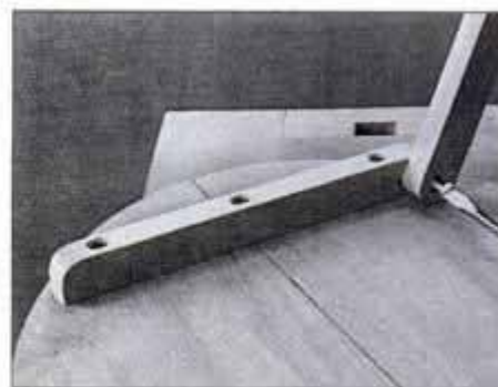
9 Attach the legs to the top with a machine screw. Place a washer between the leg and the cleat to reduce the friction.
