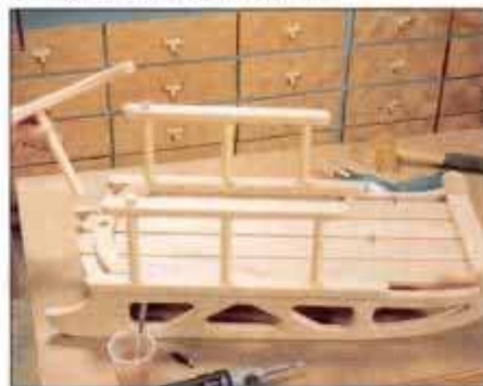
11 First assemble rails and dowels without glue to test fit the parts. Rear and side dowels are pinned to top rail.
