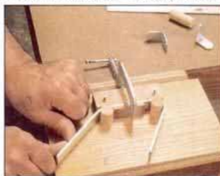
12 Clamp aluminum flat stock to jig. Stock should be centered to produce a symmetrical handle, then bent to shape.
