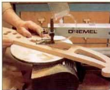
3 Bore holes in the runners to start the cutouts. Saw between holes with a scroll saw to drop out the waste.
