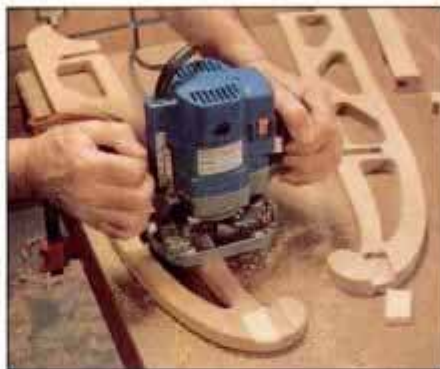
7 Ease corners with rounding-over bit. Place blocks in crossmember cutouts to prevent tearout as bit moves over edge.
