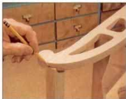
6 Fit crossmembers to runners without glue. Mark the runner radius on the front crossmember and plane down to the line.
