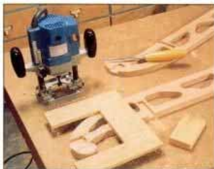
5 U-shaped plywood guides router to make the cutout for the front crossmember. Chisel the ends of the cutout square.
