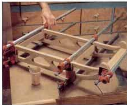
8 Using water-resistant glue, clamp the crossmembers to the runners. Measure the diagonals to check assembly for square.
