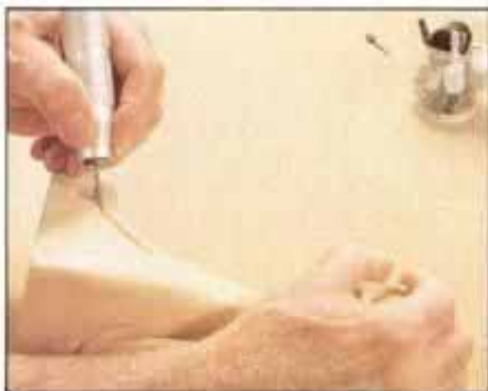
The tool carves delicate details using only a light touch. It derives its cutting power from speed, not pressure.
