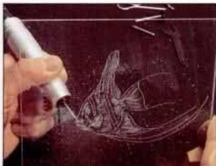
The variable-speed foot control permits low-speed cutting, a necessary feature to prevent burning when cutting plastics.
