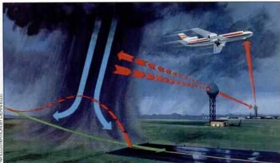
TDWR alerts tower to microburst on glide path, so controller can warn pilot away.
