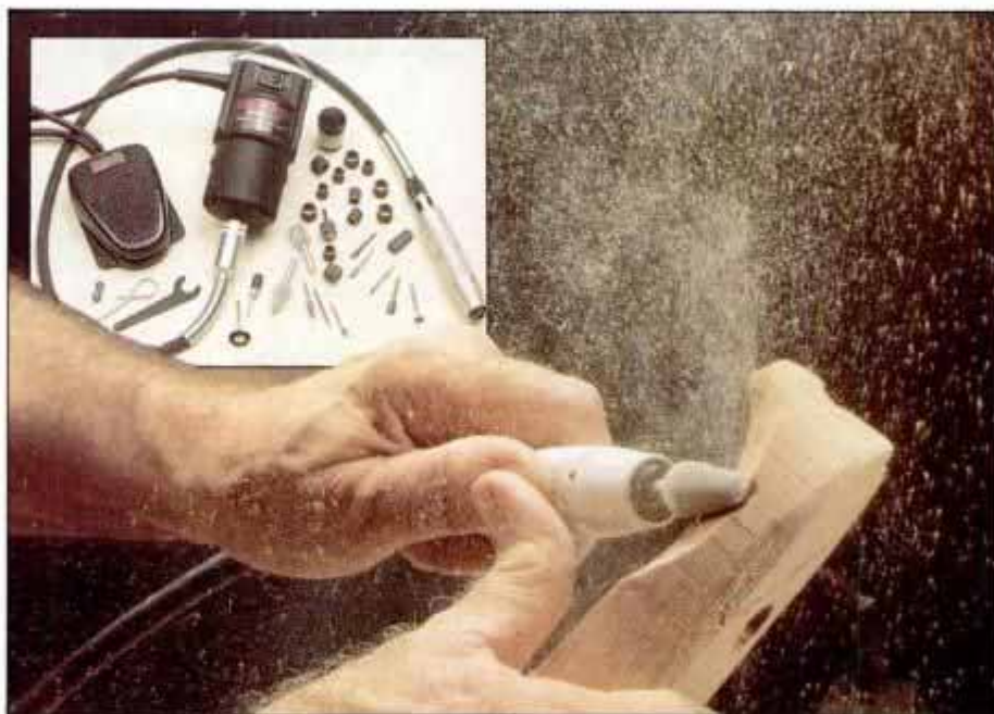
Flex Shaft Carving Kit includes motor, shaft, foot pedal control and bit assortment.
