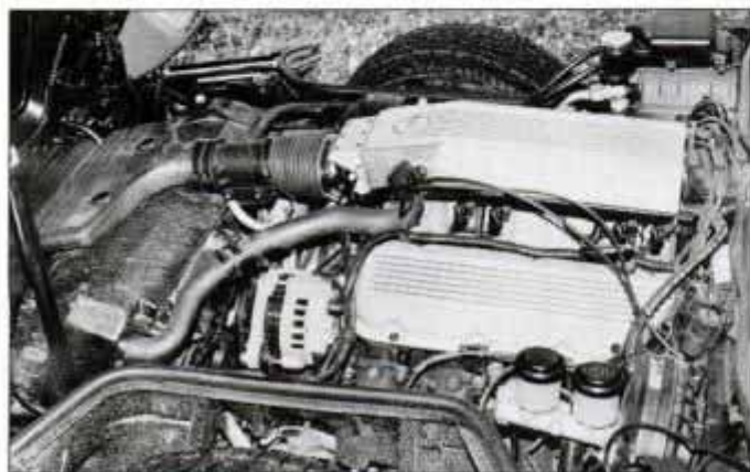
Chevy big block's custom injection system and modified exhaust.
