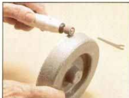
The sanding drum makes short work out of deburring even hard-to-grind metals. Here, the coarse drum deburrs cast iron.
