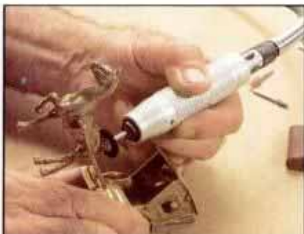
Polishing metal is a snap with the brush wheel loaded with polishing compound. Light pressure easily removes tarnish.
