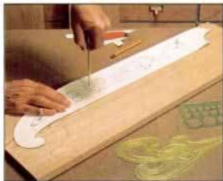
1 Tape a runner pattern to the stock. Mark the hole centers for the cutouts by poking an awl through the pattern.
