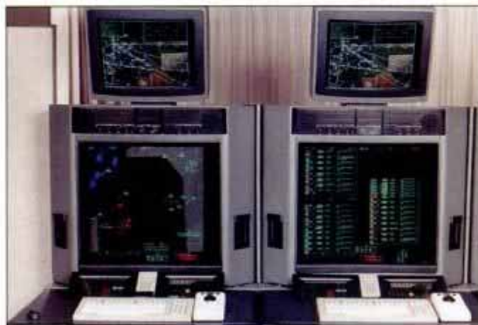
High-resolution consoles form the heart of the FAA's Advanced Automation System. Raytheon will install more than 5000 of them.
