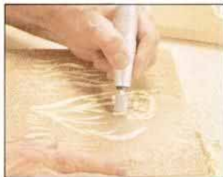
Even with large structured-tooth carbide cutter, turning at full speed, the tool is easily and precisely controlled while carving.
