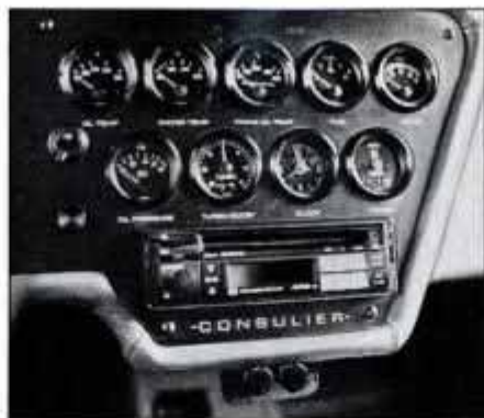
Aircraft-style gauge array in center console is long on info, short on readability.
