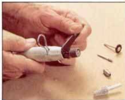
To change bits, insert pin to lock the motor shaft. Unlock collet nut with the wrench provided, insert new bit and tighten.
