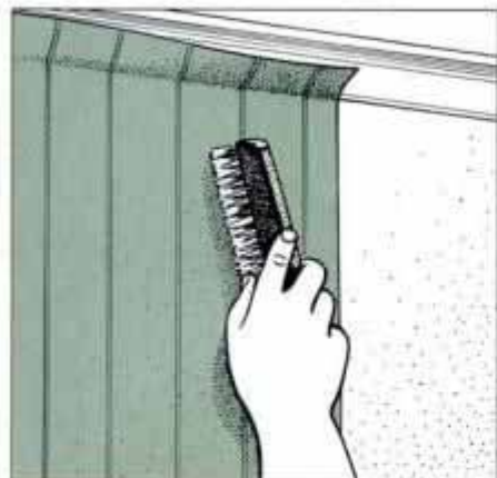
7 Align first strip with vertical layout line. Smooth strip with wallpaper brush, working out from its center to the edges.
