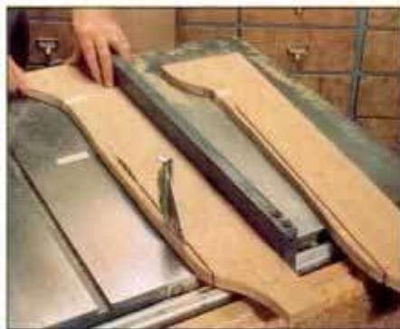
2 Make straight cuts on runner with the table saw. Attach tape to the workpiece and saw table to mark the end of the cut.
