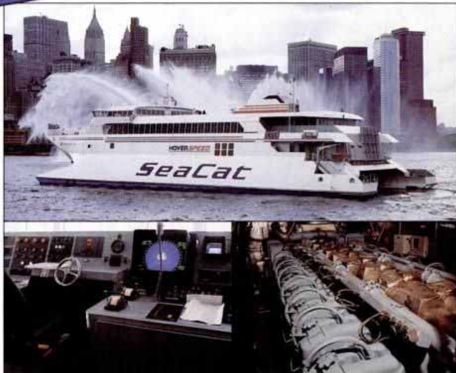
Great Britain, welcomed by fireboats in New York (top), has a race-car-size helm (above left), flanked on right by radar and throttles for 16-cylinder diesels (above right).
