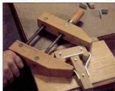
13 Nail block to jig and complete bend using parallel jaw clamp. Sand or file off sharp edges, prime and paint handle.
