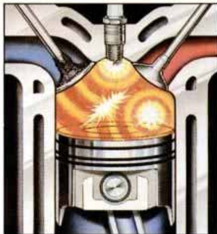
Independent flame fronts from premature ignition cause knock (above). To combat the problem, octane enhancers are used.
