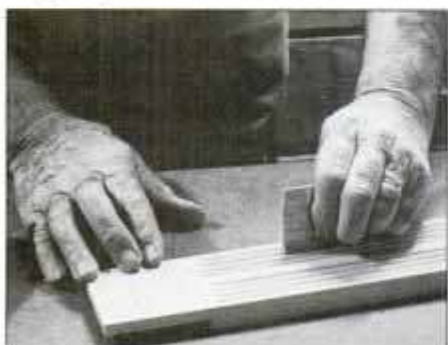
5 Lightly hand sand the beading with folded fine-grit sandpaper. Avoid rounding over the beading's crisp corners.
