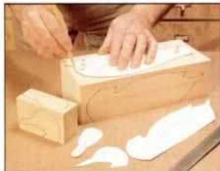
14 Mark top and side view of decoy body on the stock. Make sure both views are accurately aligned. Repeat for head blank.
