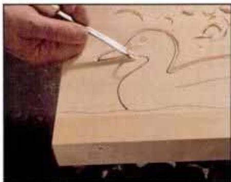
8 Begin relief carving by using the V-tool to outline the duck profile. Keep the cut in the waste area—about 1/8 in. from the line.
