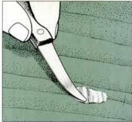
11 Reheat knife, wipe it clean with 4/0 steel wool and smooth the shellac patch.
