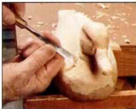
26 Install decoy head with glue and lagscrew. Use a gouge to blend the head with the body so the surfaces are continuous.
