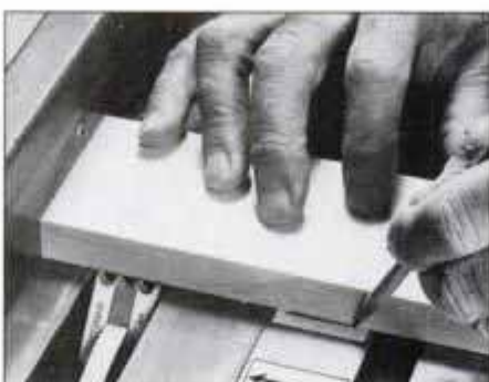
3 Apply tape to table saw bed to set up for beading cuts. Marks on tape indicate where beading cutter engages workpiece.
