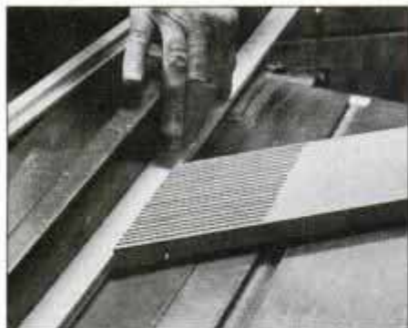
8 Cut rabbet in rail and stile trim with two cuts on table saw. Use a feather board to keep workpiece against the saw fence.
