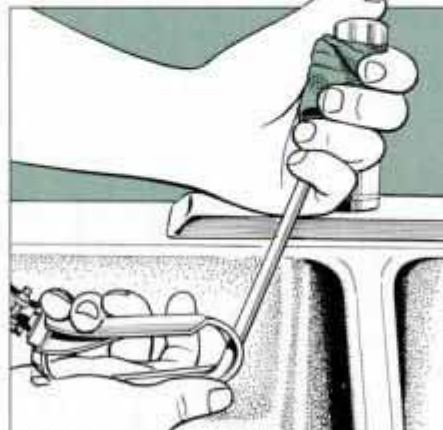
11 Open cold side and insert gun tip from air tank into spout. Seal with rag and shoot air, then repeat for hot side.
