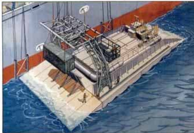
Gantry on pontoon platform snares cargo from container ship.
