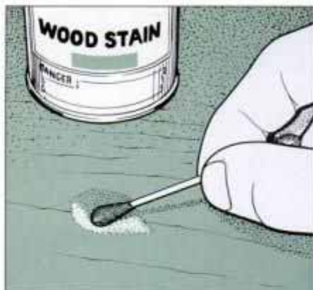
6 Once filler is dry and sanded level, apply wood stain with a cotton swab.
