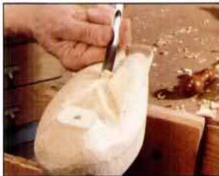
23 Use a straight gouge to shape the depression on decoy back. Note that neck joint has been shaped to match head.
