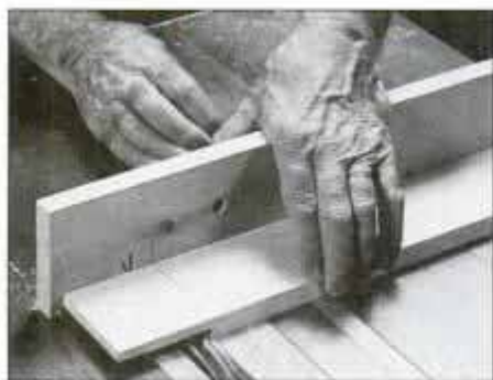
2 Cut the half-laps using a miter gauge and a dado head on the table saw. The blade height equals half the stock thickness.
