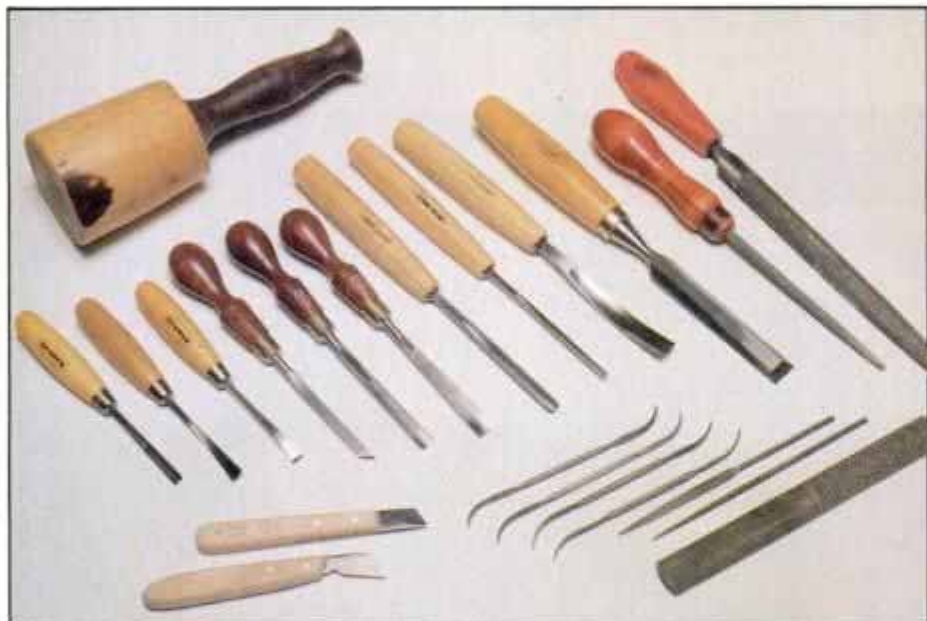
1 A simple carving kit includes straight and bent gouges, straight and skew chisels, a veiner, a V-tool and a mallet. Chip carving knives (bottom left) are used for decorative surface carving. Files and rasps smooth carved surfaces, and rifflers shape and smooth details.
