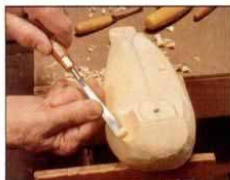
21 Use gouge in pivoting motion to form the concave shoulder curvature. Always follow grain direction of block.
