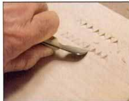
3 Six-cut triangle begins with three stop cuts made from the center of the triangle. Remove waste by cutting in from sides.
