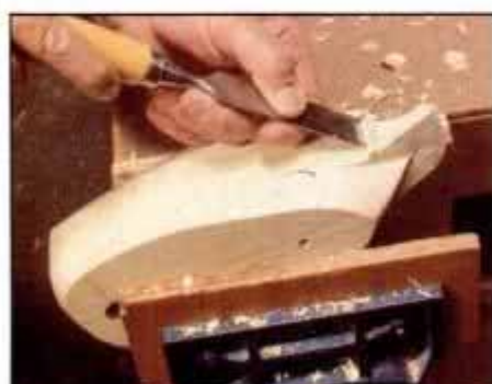
20 Use chisel with bevel up on convex curve. Pressure is applied with hand on handle. Hand on blade controls the cut.
