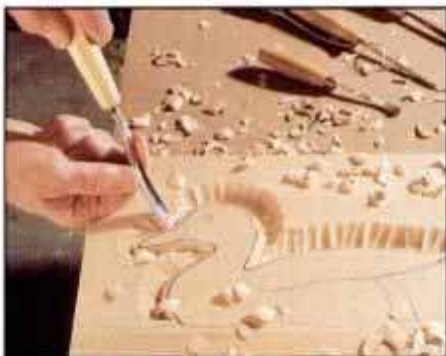
9 After making vertical cuts around the outline using straight gouges and chisels, remove waste with a gouge.
