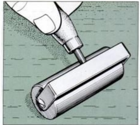
18 Press veneer down with roller and leave a weight on it until glue resets.
