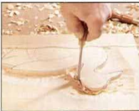
10 As work progresses, continue alternating between grounding cuts made with bent gouge and cuts that follow outline.
