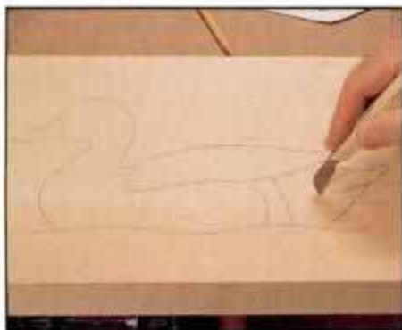
5 After laying out the duck profile, begin carving by holding the knife at 90° to make stop cuts that follow the outline.
