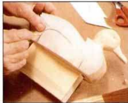
24 After preliminary body shaping, use a paper pattern to lay out wing-pocket shape symmetrically on sides of decoy.
