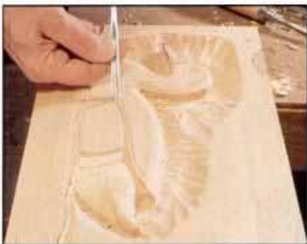
12 Use the V-tool to incise the separation between the wings. To clearly see contours of carving, light the work from a low angle.
