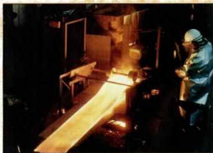
In direct-strip casting (top), steel strips fly off cooling wheel. In spray forming (below), atomized steel cools on substrate belt.
