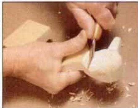
16 Fit the head blank to the head-holding jig and shape head by whittling. Note how thumbs are placed to help control cut.
