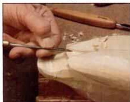
22 Use a skew chisel for cleaning out tight areas. Work is firmly secured in vise by a 2 \times 4 block screwed to the work.
