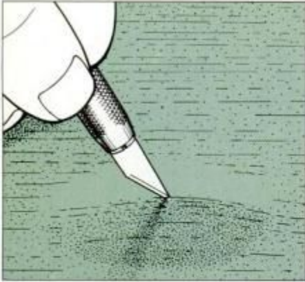
16 Slit the center of veneer blister with a razor knife. Make the slit along the grain.
