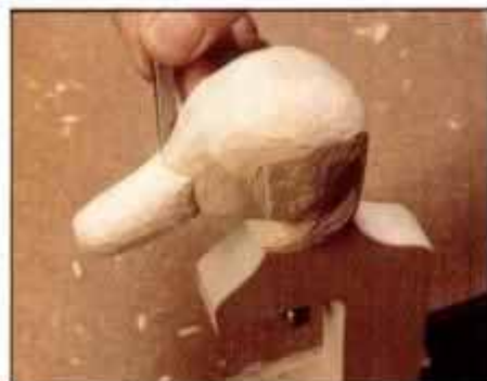
17 After preliminary shaping, install head-holding jig in vise and begin shaping the bill details with a small skew chisel.
