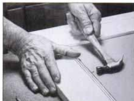
13 Place cardboard behind mirror. Nail cleats to rails and stiles. Lay hammer on cardboard and swing into the brads.
