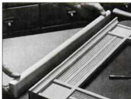
12 Glue and nail lower cornice molding to rail, then glue and nail on upper molding. Divide the cornice overhang equally.
