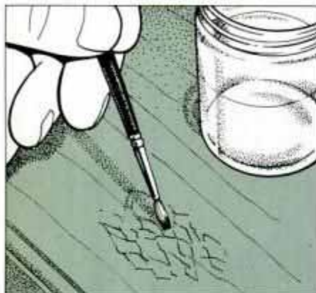
4 Apply solvent to an alligatored finish. Softened finish flows into the cracks.
