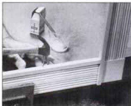
10 The stile trim pieces go on next. Hold the frame upright in a vise. Glue and nail the trim. Set and fill the nailheads.
