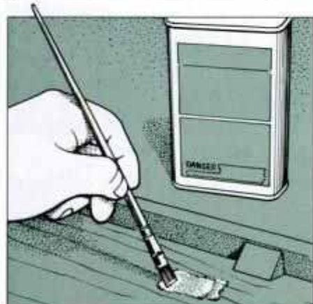
1 First identify the finish on furniture being repaired. Test it with solvent.
