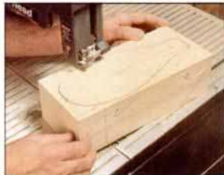
15 Band saw the side profile first. Replace the waste to reinstall the top view layout. Then, band saw to the top outline.
