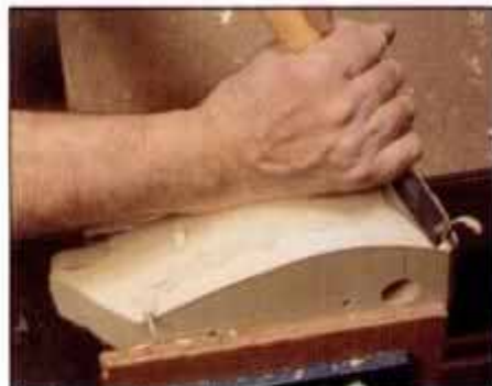
19 Begin rounding the body by making a series of chamfer cuts around the bottom. Use the mallet for heavy work only.
