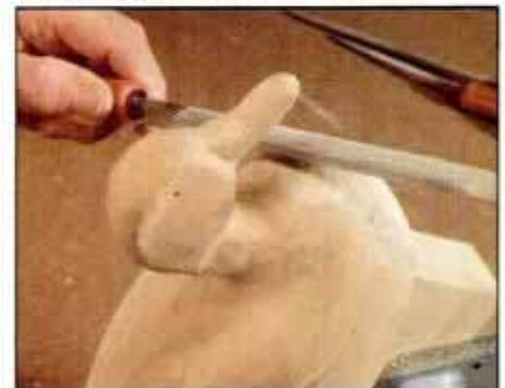
28 Use a flat file for smoothing convex areas, a half-round file for large concave surfaces and a round file for small curves.
