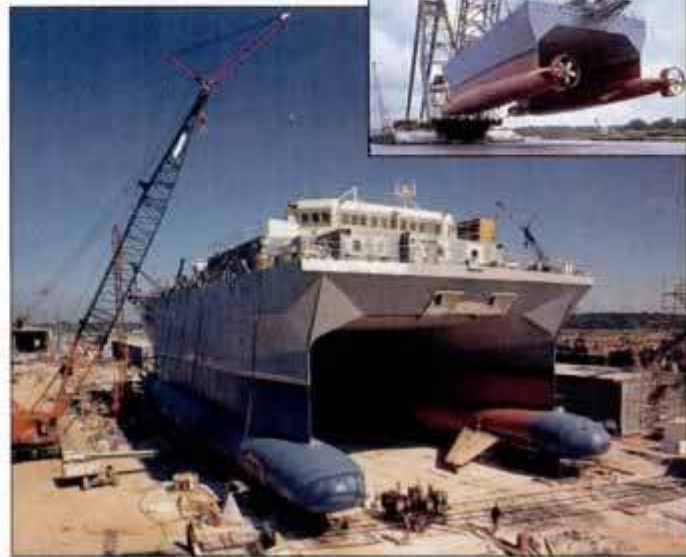
USNS Victorious is launched by shear-leg crane during christening.
