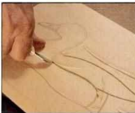
7 Hold the knife at 45° to the surface and cut along the second set of lines to remove wood and delineate the shape.
