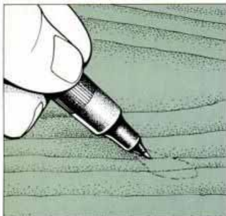
7 Draw graining on patch with a fine-tip pen. Soften sharp lines with a cotton swab.
