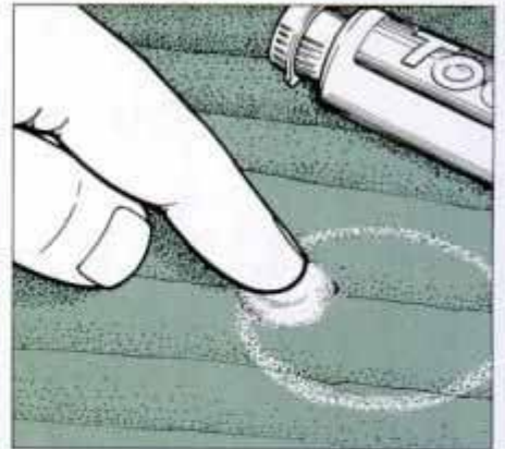
12 Gently rub on some toothpaste to remove white ring from shellacked surface.
