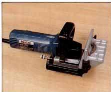
1 The Freud JS100 tool shows standard plate joiner configuration. Blade is gear-driven and motor has slide switch.
