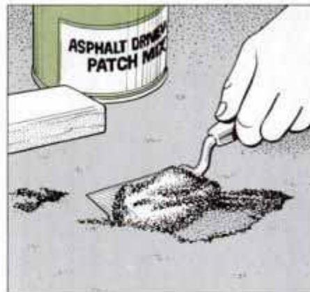
6 Mound patching compound in holes using a small trowel. Patch should be about 1/2 in. higher than the surrounding surface.
