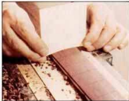
6 While hand planing the fingerboard camber, use a 7-in.-rad. template to gauge the arc. Then, sand the board smooth.
