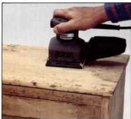
4 After the bleached wood is dry, finish sand all surfaces with 120-grit paper. Since bleach is in wood, be sure to wear respirator.
