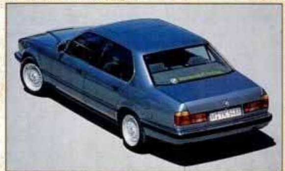
BMW's hydrogen-powered car is the most advanced one currently on the road. It carries fuel in high-density, liquefied form to extend range.
