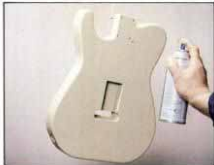
18 After priming guitar body, apply finish coats. Be sure to have adequate ventilation and observe manufacturer's precautions.
