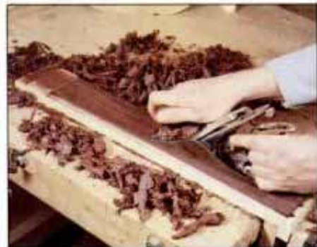
2 Use a sharp, finely set hand plane to joint and thickness fingerboard to \frac{1}{4} in. Long bench hook holds work in place.
