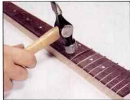
7 Install frets by first bending to tighter curve than board. Hammer ends in place and then tap from side to side to seat fret.
