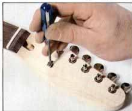
21 After fitting tuning machines, screw string retainer in place. This holds high strings down to bear tightly on nut.
