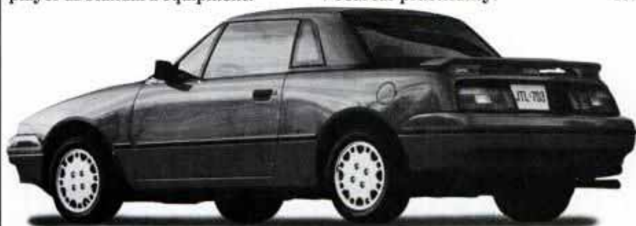
Capri's optional hardtop has glass side windows and a rear window defogger.
