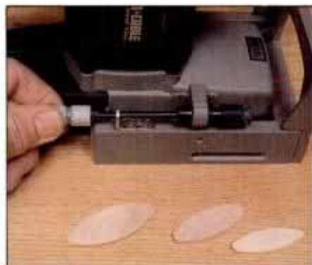
3 Adjustable depth-of-cut stop has three positions to suit the three plate sizes. Knurled knob permits fine-tuning.
