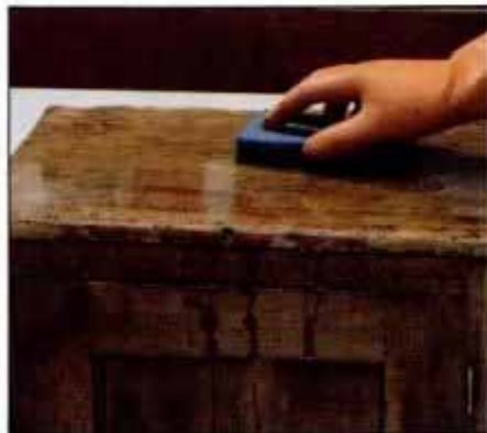
3 Use 2-part bleach, available at paint stores, to remove stains and discolorations apparent after stripping.
