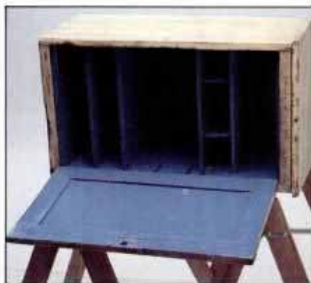
5 Because the interior was difficult to strip, we chose to paint it blue after wiping surfaces with a turpentine-dampened rag.
