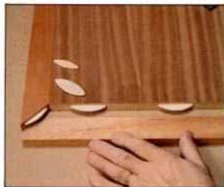
9 This mitered edgebanding uses two plate sizes: No. 10 plate for the narrow miter and No. 20 along the panel edges.
