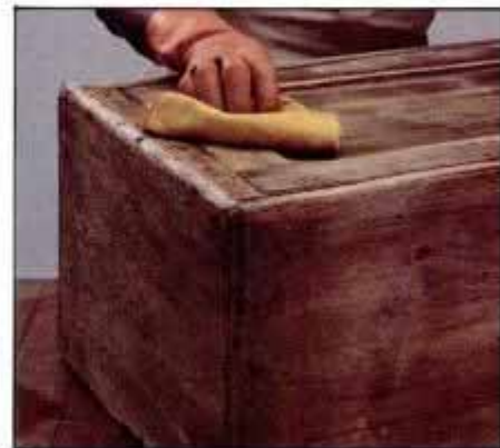
9 After the wax has dried for a few minutes, buff the entire surface with a soft, clean, lint-free cloth to produce a satin luster.
