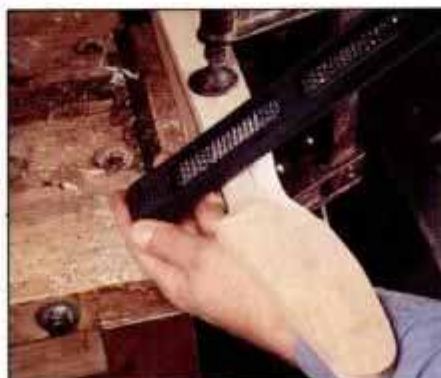
8 Use Surform tool to shape neck back near head and body joint. Finish between with spokeshave and sand smooth.
