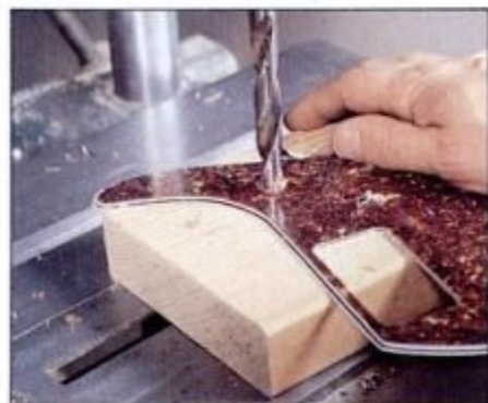
15 After cutting pickup holes, use drill press to bore control holes, pickup screw holes and pickguard mounting holes.
