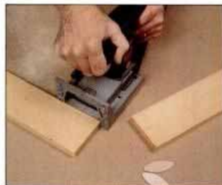
6 Align index mark on joiner faceplate with centerline of joint. Turn on power and push forward to make the slot.
