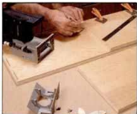
11 To join shelf to case side, first clamp shelf to side panel at shelf location. Then mark joint centers on both panels.
