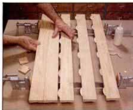
15 When edge gluing lumber, reference slots from best side of stock. Place slots 2 in. from end, and 4 to 12 in. in between.
