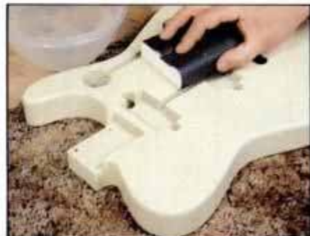
19 Wet sand final finish with 400- and then 600-grit paper to remove all imperfections. Then use polishing compound.
