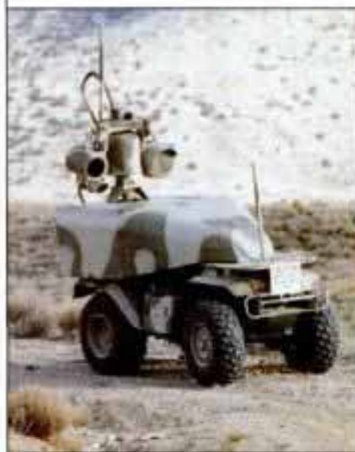
Telerobot ATV, with mast-mounted sensors (left), and fixed sensor stations (right) secure sensitive outdoor locales.
