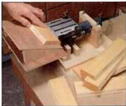
23 With appropriate shopmade bevel platform in place on joiner stand table, slots are cut for miter joints of any angle.
