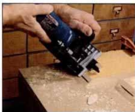
10 Edge mitering is done by setting the fence for 45°. Most tools register against the inside of the joint as shown here.
