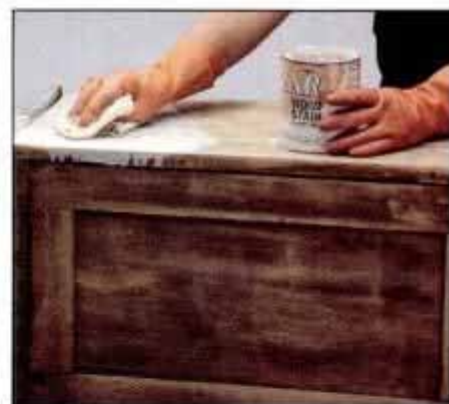
6 After applying thinned pine stain to color wood, white stain is applied and then wiped off to give whitewashed look.
