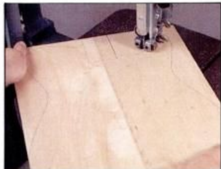
10 After laying out body shape and centerlines on 1 1/4-in.-thick basswood, saw to the outside of the line on the band saw.
