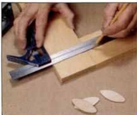
5 The first step in making a plate joint is to align mating pieces and mark the center of the plate joint slot on both pieces.
