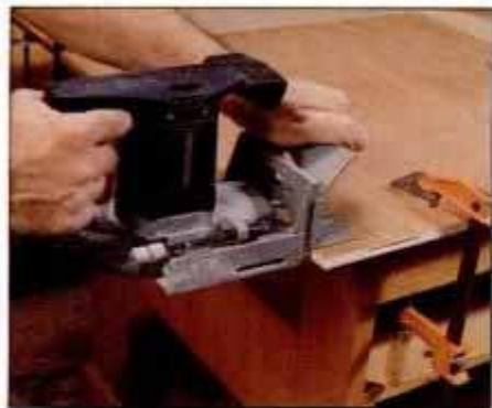
8 To position slot at center of thin stock, such as 1/2-in. plywood panel, install fence at correct distance from blade.
