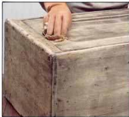
8 Additional surface protection and luster is achieved with a thin coat of paste wax. Apply with a rag or extra-fine steel wool pad.
