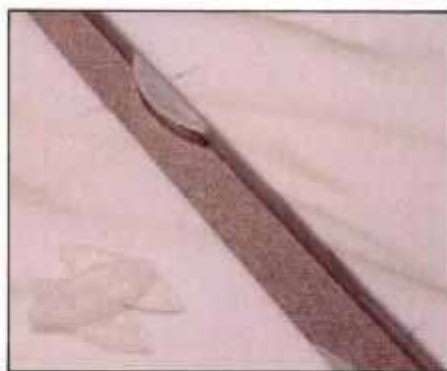
19 For aligning and stabilizing solid-surfacing materials, the plastic, translucent Lamello C20 plate is available.
