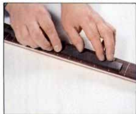
22 Lay a large file along the fingerboard and move it carefully along the length to level all frets to the same height.
