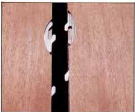
20 The Lamello aluminum KD fitting is inserted into No. 20-size slots. Fitting at top is shown on panel surface for clarity.
