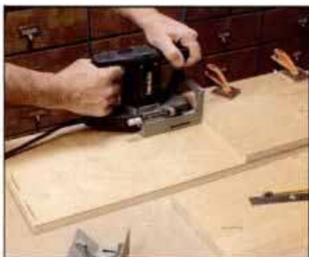
12 With base of tool held flat against cabinet side, align index mark with slot centers and cut all slots in shelf edge.
