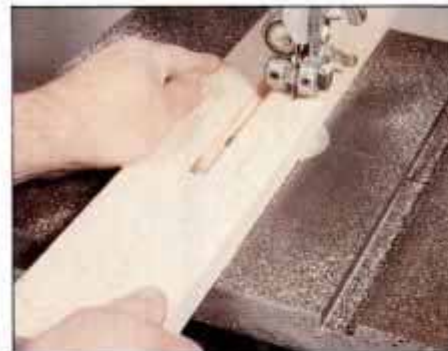
1 After routing the channel for the truss rod in \frac{3}{4} -in.-thick maple, lay out neck outline and band saw to outside of line.
