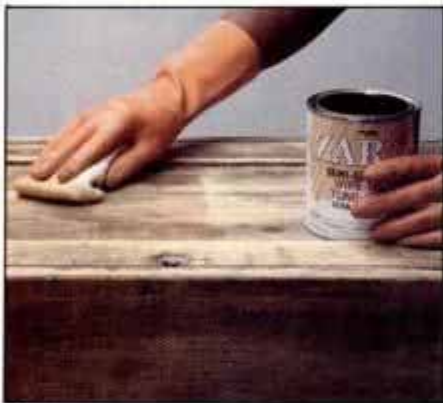
7 When the stain has dried for 24 hours, apply the tung-oil finish with a rag. Apply a second coat after buffing with steel wool.
