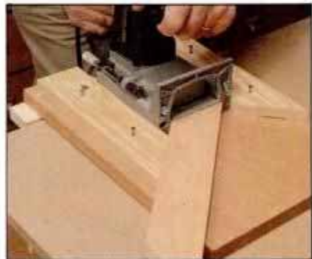
25 Platform jig consistently positions joiner and stock. A pair of projecting nail points in the base anchor workpiece.
