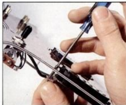
17 Mount the completely wired assembly in the pickguard. Pickup screws and springs allow adjustment of pickup height.
