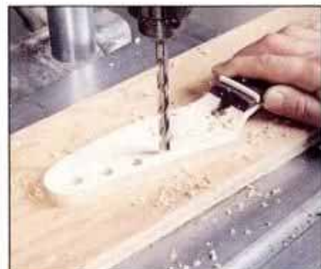
9 Carefully lay out spacing of holes for tuning machines and bore on drill press. Use backing board to eliminate tearout.
