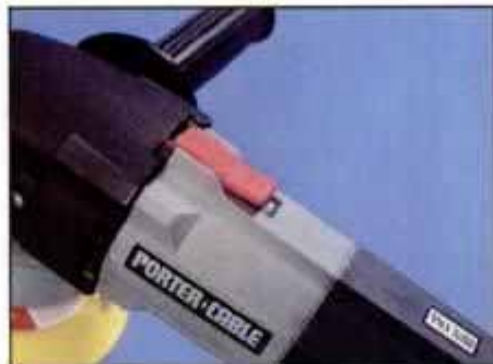
1 Slide switch forward to turn on power. Release it to turn off sander. Lock on power by pushing front of switch down.
