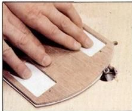
14 Mount router in router table and use chamfering bit with pilot to bevel edges of pickguard. Work against bit rotation.
