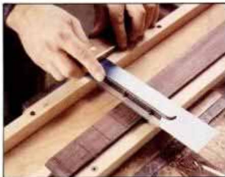
5 After laying out fret spacing, saw fret slots perpendicular to fingerboard centerline. Saw kerf must be .020 in. wide.
