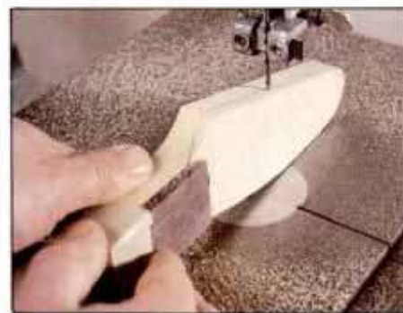
4 Shape head setback on band saw to bring head thickness to \frac{1}{2} in. Smooth sawn face with drum sander and by hand.
