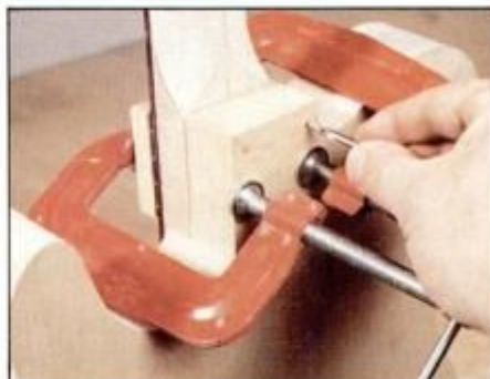
12 After boring screwholes through body, align and clamp neck in place and transfer pilot hole locations to neck.
