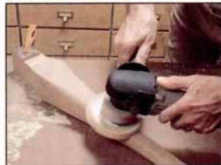
4 The accessory contour pad has slightly more flexible backing. Sander equipped with pad smooths a cabriole table leg.
