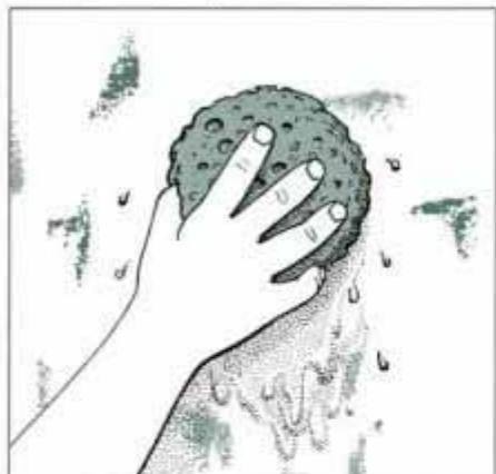
15 Wash glue residue and bits of paper off the wall using a solution of TSP and warm water, or use a household detergent.
