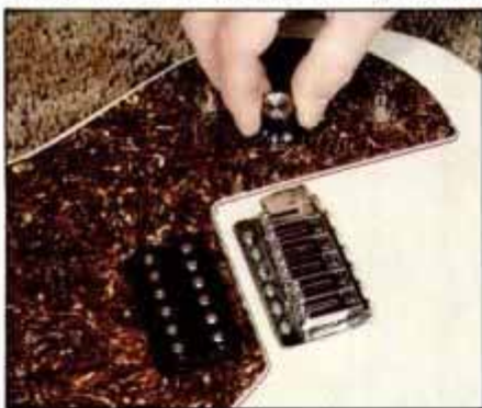
20 Install tremolo unit and wired pickguard assembly. Rotate controls clockwise and install knobs with No. 10 facing up.
