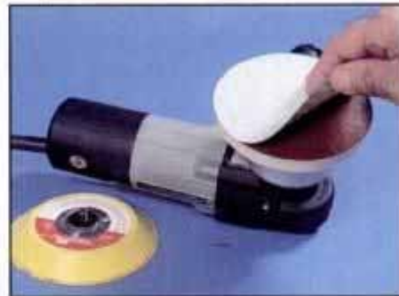
2 Abrasive discs are easily installed. Simply peel off their backing paper and stick them onto the padded disc.
