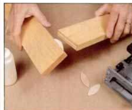
7 Apply glue to the slots and to the surfaces to be butted. Insert plate in one slot, join the second piece and clamp.
