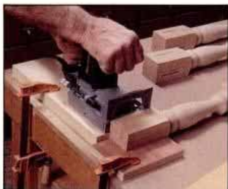
16 Offset joints can be made by supporting the tool on a spacer block to locate the slot. L-block holds work in place.
