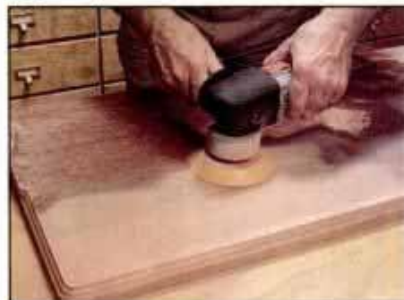
3 Sander proved to be versatile. Here it's used to remove a finish by sanding varnish coats off a mahogany surface.
