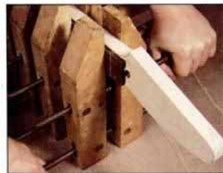
3 After installing truss rod in channel with epoxy, glue fingerboard to neck with carpenter's glue. Let glue dry overnight.
