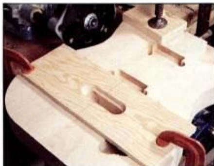
11 Plunge router with guide bushing follows plywood templates for cutting all body cavities. Shown is the tremolo slot.
