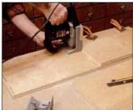
13 To cut corresponding slots in cabinet side, hold tool upright against shelf edge and align index mark with centers.
