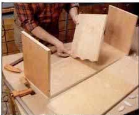
14 After all slots have been made, apply glue, insert plates and assemble. Check for accurate alignment before clamping.
