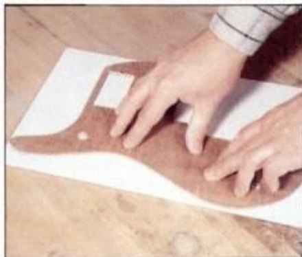
13 Use double-faced tape to attach pickguard template to pickguard blank. Then, band saw blank roughly to shape.
