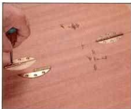
21 Lamello hinges are flush mounted in recesses milled with plate joiner. Hinge halves are detachable for easy installation.
