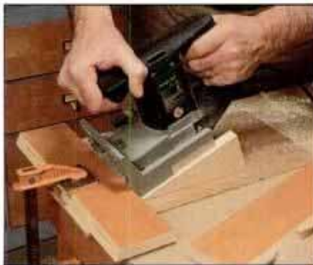
24 Bevel platform can also be used with handheld plate joiner for bevels other than 45°. Clamp stock to prevent shifting.
