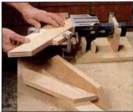
22 Bench-mounted joiner is ideal for small parts and repetitive jobs. Here, guideblock uniformly registers stock for miter joint.
