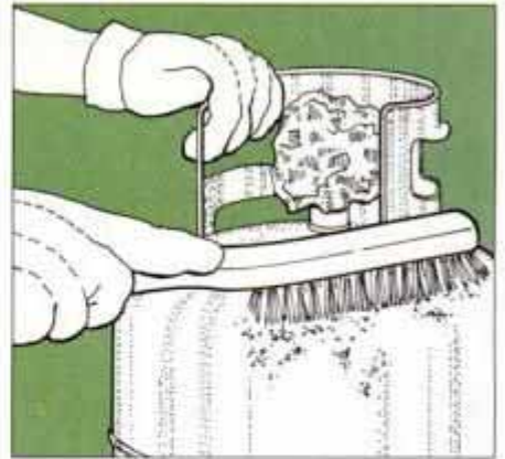
18 Cover gas tank valve with aluminum foil and remove loose paint with a wire brush. Scuff tank with fine-grit sandpaper.
