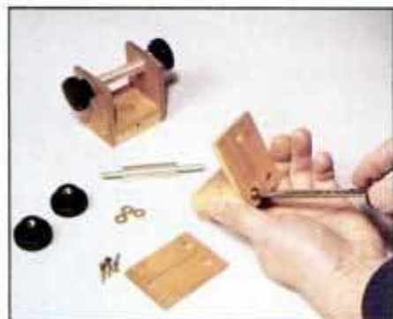
2 Focusing slides are assembled with brass screws and washers. Thread plastic knobs on focusing-rod ends and tighten.
