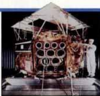
CRRES satellite undergoes checkout (above), before being launched into elliptical orbit gauged for maximum exposure to Van Allen radiation (right).
