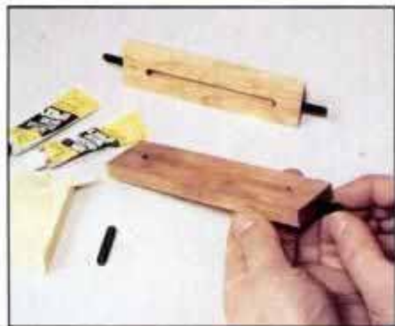
1 Begin assembly by using quick-setting epoxy to secure threaded studs in the shift bar ends. Let epoxy set for 8 hours.
