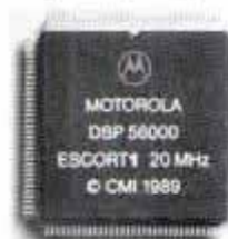
The heart of ESCORT's DSP circuitry is a custom version of the Motorola DSP 56000. This 20 MHz 24 bit parallel HCMOS processor is capable of 10.25 million instructions per second, and is also used in Steve Jobs' new $10,000 NeXT computer.
