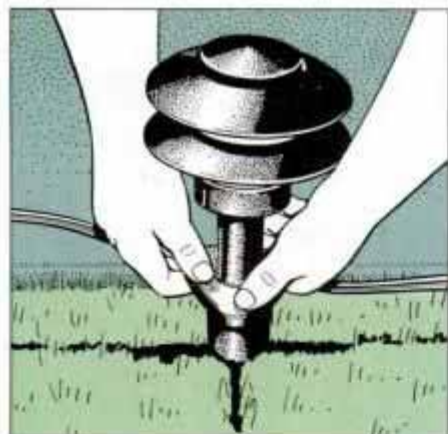
19 After making deep crosscut in sod, press stake into opening until its platform rests at ground level.
