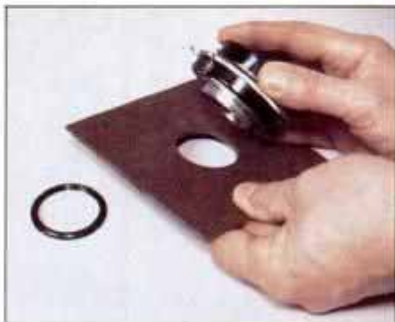
9 Use a holesaw to cut hole for lens in exact center of lensboard. Install lens in hole and secure with lens retaining ring.
