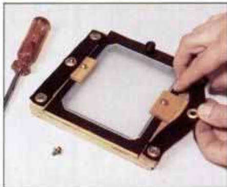
6 Screw elastic strips to film back. Lift strips and insert glass view screen. Secure view screen to elastic with brass screws.
