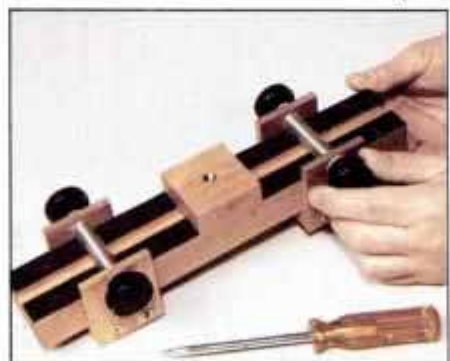
3 Install focusing slides on monorail so plastic-sheathed rods bear on abrasive strips. Adjust for smooth operation.
