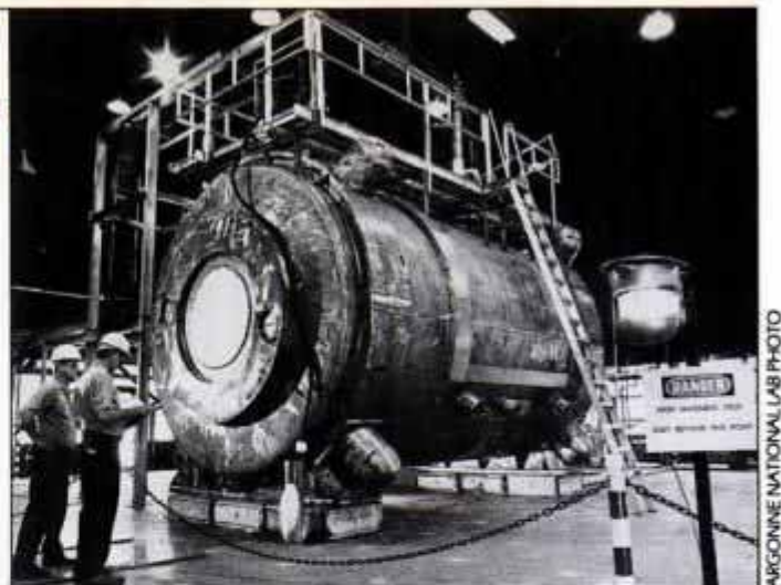
Argonne superconducting dipole (right) crisscrosses lines of magnetic flux and electric current to produce thrust (left).
