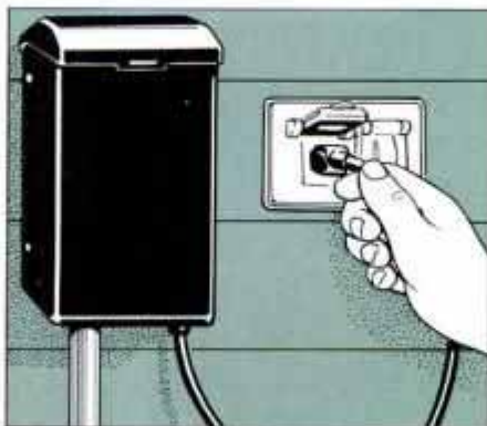
1 When using an outdoor receptacle, hang box at least 12 in. above ground. Protect cable to ground with conduit.
