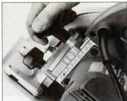
Adjust cut depth on drop-foot saws by loosening knob and sliding base up or down. Graduations on Bosch tool indicate depth of cut in inches or centimeters.
