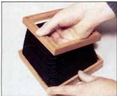
5 Use contact cement to join bellows to front and rear frame. Make sure parts are aligned properly before applying pressure.
