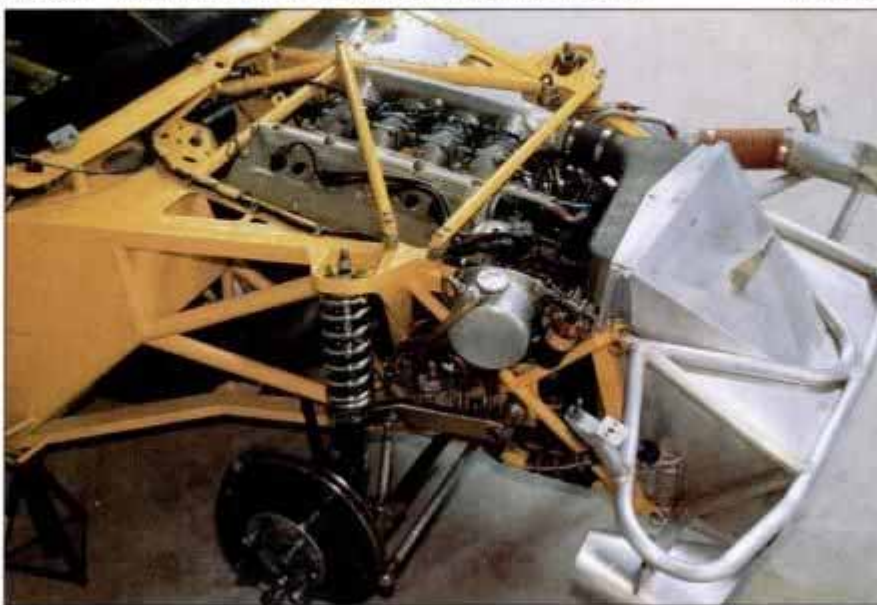
Dave Finch's steel spaceframe chassis has an aluminum front substructure.
