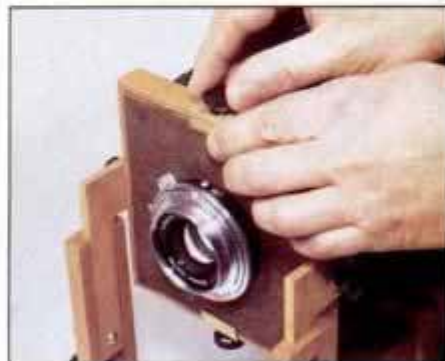
10 Brass clips at top and bottom of front frame hold lensboard in place. Secure the clips by tightening plastic knobs.
