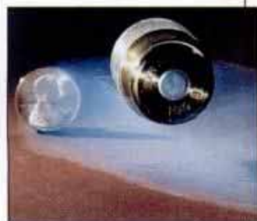
One gram of Livermore's smoke-like aerogel supports 100 grams.
