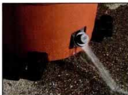
6 Unscrew the drain cap to drain the vacuum or flush out the tank with a garden hose. Its liquid capacity is 13 gallons.
