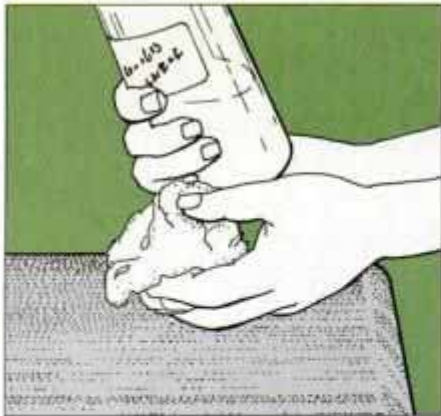
16 Degrease grill body by wiping it with a rag soaked with white vinegar. When the vinegar is dry, the grill is ready to paint.
