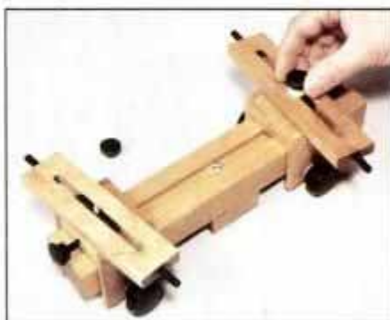
4 Assemble shift bars on focusing slides with appropriate hardware. Use supplied plastic washers under all knobs.
