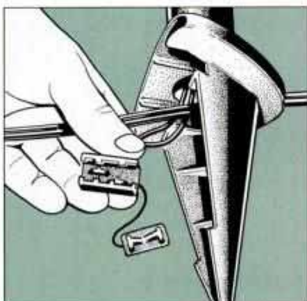
8 Feed cable through stake platform to the desired location. Then remove cover from cable clip to expose contact points.
