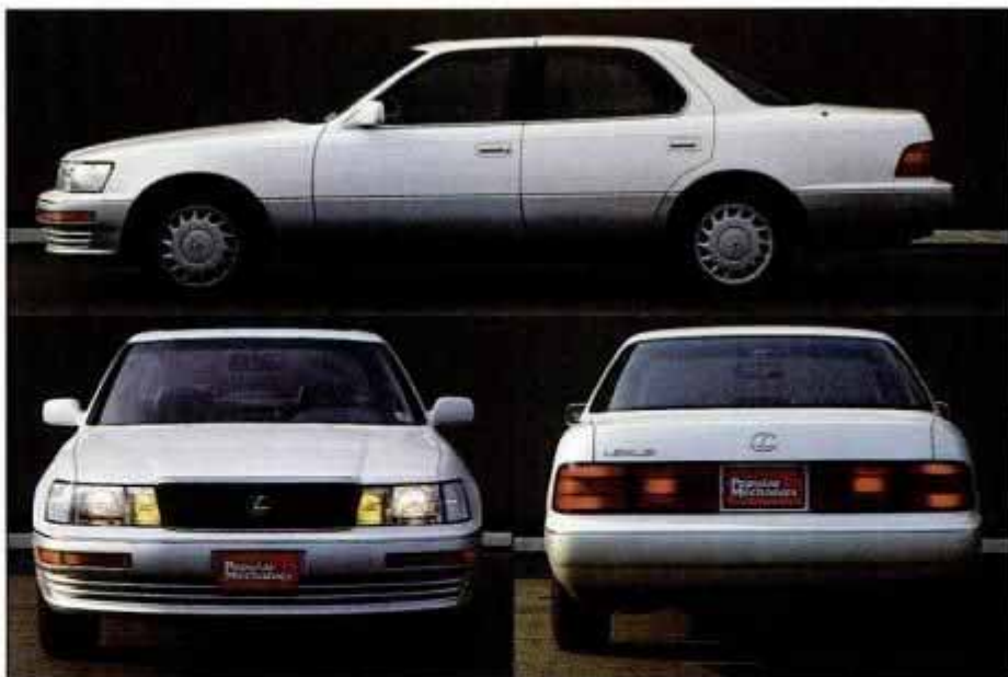
Although Toyota borrowed heavily from Mercedes in LS 400 design, 41.6 percent of owners cited styling as a best-liked feature. Wind tunnel development yielded excellent 0.29 Cd rating, contributing to exceptional interior quiet.
