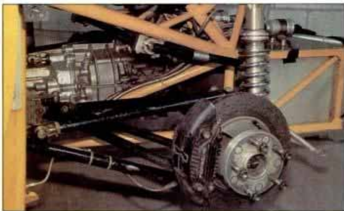
Semitrailing arm rear suspension mimics upper/lower control arms.
