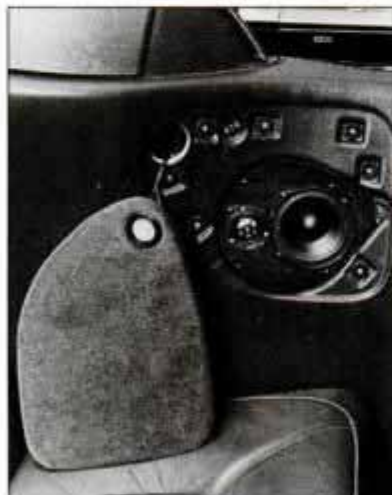
Rear speakers are hidden behind acoustically transparent grilles in this Saab 900 convertible belonging to P.D. Lazarus. Amplifiers and signal processors are installed in trunk under hinged floorboard.
