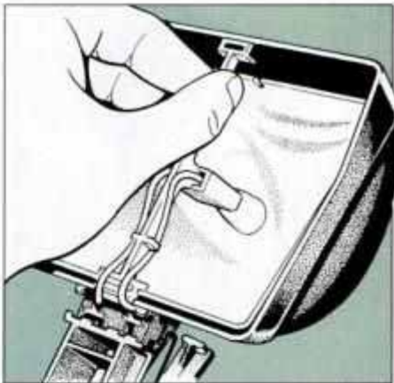
13 To install floodlights, feed wires through bridge and fasten bulb to center leg of bridge. Snap bridge onto lamp head.
