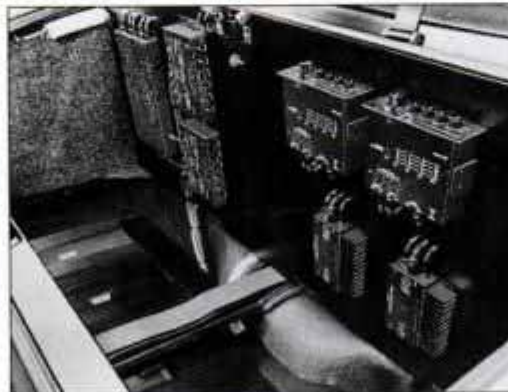
Rear speakers are hidden behind acoustically transparent grilles in this Saab 900 convertible belonging to P.D. Lazarus. Amplifiers and signal processors are installed in trunk under hinged floorboard.
