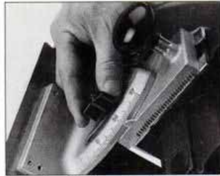
Loosen bevel knob to rotate base to desired cutting angle. This Skil saw is graduated in single degrees. Other tools may be graduated in 5° increments.
