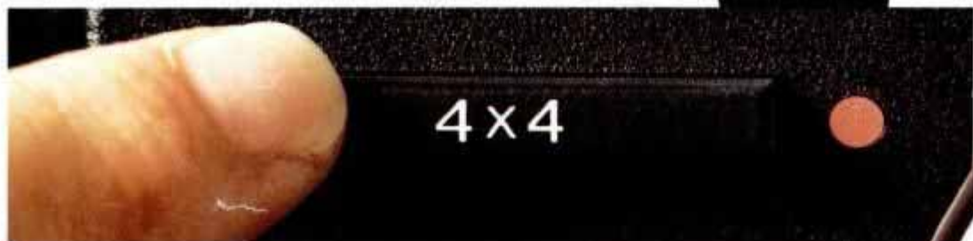
A Ford exclusive: Electronic pushbutton four-wheel drive system. Shift on-the-fly from 2WD to 4WD-High and back at the touch of a button at any speed. Standard on Ranger 4x4s.
