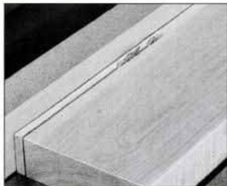
9 Rip slats slightly oversized from 1 \frac{3}{4} -in.-thick stock. Then plane them to finished thickness to remove the saw marks.
