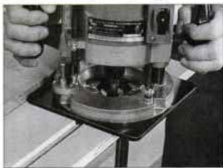
5 Cut a dado across the pedestal panel to accept plywood bottom. Clamp a fence across the panel to guide the router.
