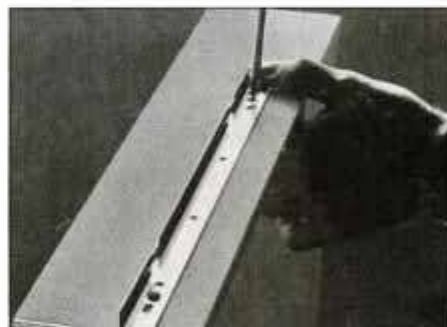
22 Assemble drawer box front, back and sides. Screw the drawer slide to side of box. Screw through slotted holes only.
