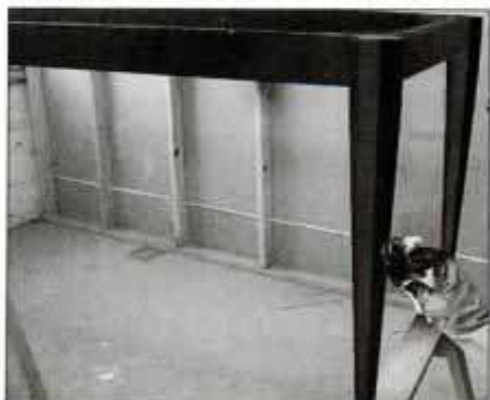
18 Apply the ebonizing stain with a rag, brush or by spray. Wear gloves and use organic filter cartridges in the respirator.
