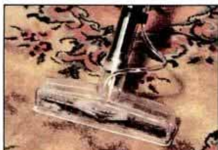
Carpet washing head circulates detergent in fibers while drawing dirty water into tank. After washing, suction dries carpet.
