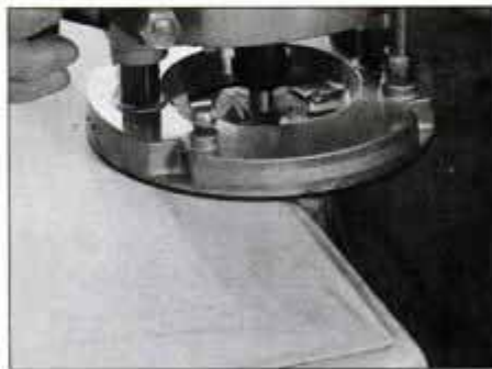
18 Use 5/8-in.-dia. rounding-over bit to mold corners of edge banding. Rout bottom edge first, then rout top edge.
