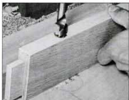
8 Use a \frac{3}{4} -in. multispur or Forstner bit in the drill press to bore recess for tabletop fasteners in apron's top edge.
