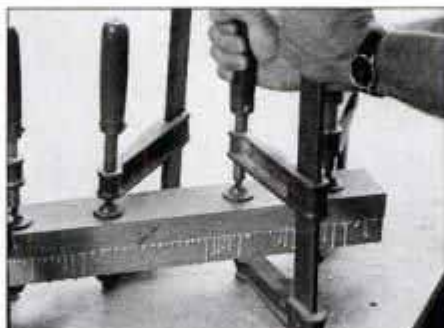
1 Glue up slightly oversize leg blanks. When the glue is dry, rip and crosscut the blanks to the finished dimension.
