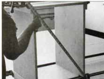
7 Clamp up assembly and measure diagonals to check for square. If measurements differ, shift clamps to achieve squareness.
