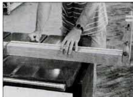
2 During crosscutting, butt legs against clamp or stopblock on miter gauge. This ensures the legs will be the same length.
