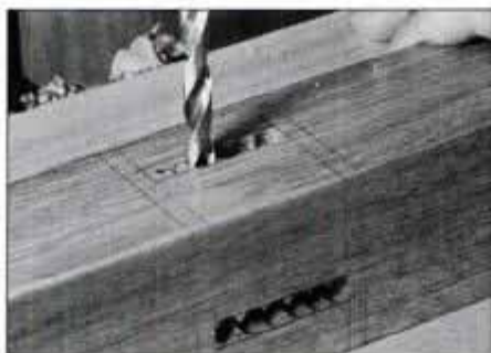
3 Mark the mortise position on legs and remove waste by boring overlapping holes with \frac{3}{8} -in.-dia. bit in drill press.
