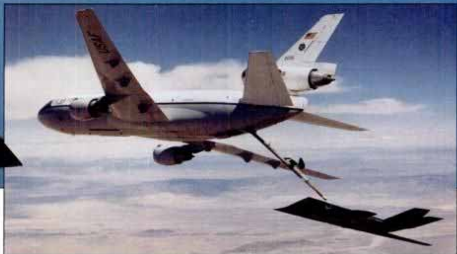
Looking different from every angle, the F-117A Stealth Fighter cools its jets through flat, shielded nozzles visible above. A pop-up receptacle facilitates in-flight refueling (right).
