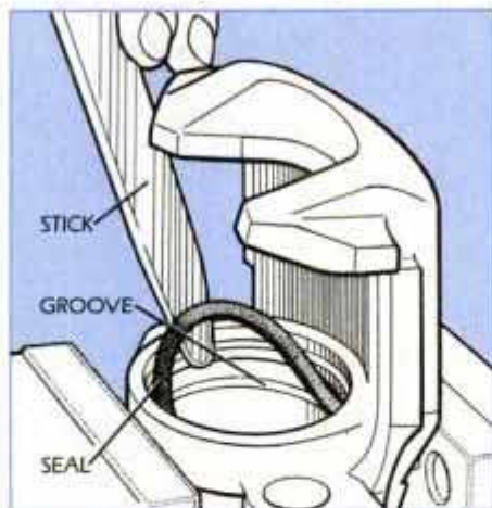
4 Use a plastic or wooden probe to lift the seal from its groove in the caliper bore.
