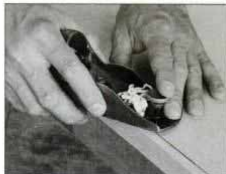
2 Plane edge band flush to the panel's edge with a sharp block plane. Be careful not to plane into the panel's face veneer.
