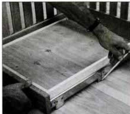
24 Position drawers over inverted desk top and mark position of mounting tabs. Attach drawers, and adjust as necessary.
