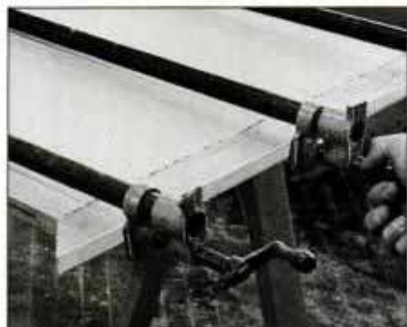
19 With top on sawhorses, use long pipe clamps to hold edge band to panel. Spread glue on joining plates and on edge band.
