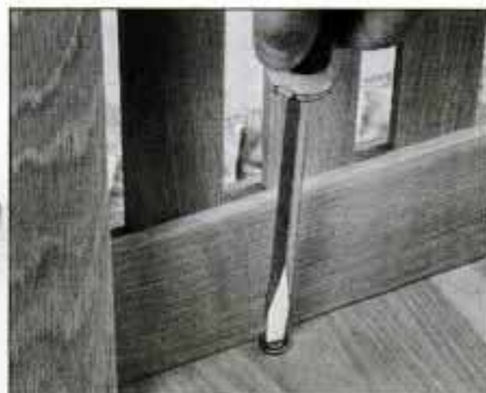
20 Screw tabletop fasteners to the apron edges. Then invert base on top, and attach, leaving 1 1/2-in. overhang on all sides.
