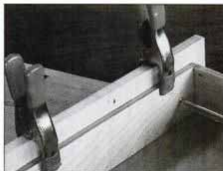
23 Clamp the finished drawer front to the drawer box. Attach the drawer front to the drawer box with a pair of screws.
