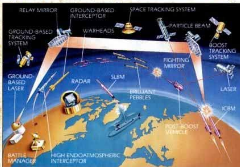
Phase I components of SDI (colored gold) will include only kinetic kill devices. Directed energy weapons, such as lasers, will be added later.
