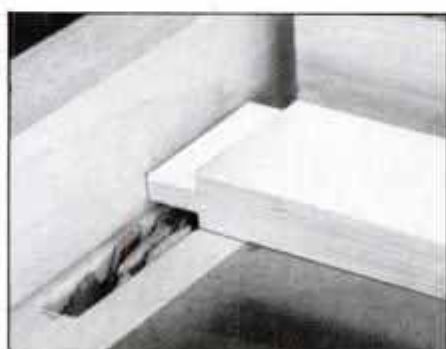
9 Cut tenon cheeks on aprons using dado blades in table saw. Butt apron against fence, and use miter gauge to guide cut.
