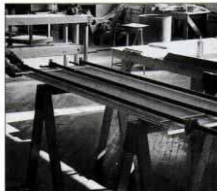
17 Clamp end edge bands in place first. Prevent clamps from coming in contact with glue by supporting them on strips.
