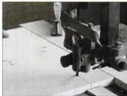
3 Saw out the notch for toeboard on the band saw. Fence and stop clamped to the saw table ensure precise, straight cut.
