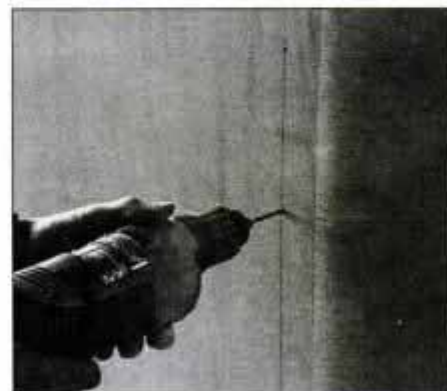
14 Bore pilot holes for screws that will attach modesty panel to pedestal. Be sure to bore the inside face of pedestal.
