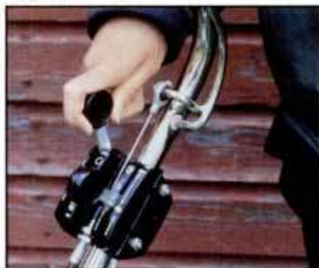
Dual control levers are located on right side of handle. Inside handle engages front-drive mechanism. Outside handle controls speed.
