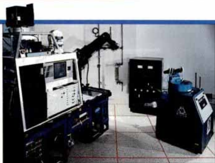
HERMIES III and smaller forerunner HERMIES II show off improved manipulators. Both think with high-speed parallel processors.
