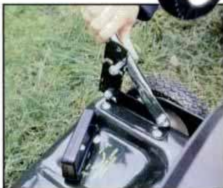
Handle has two height positions and can collapse over mower deck for storage or transport. Push spring-loaded bolt to change.
