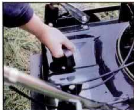
Mower deck height is easily adjusted by one D-handle mounted on rear of deck. Just turn handle, and all four wheels move at once.
