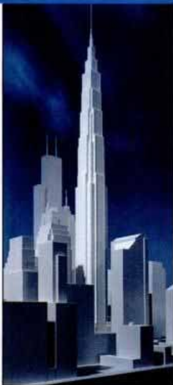
At 1914 ft., the Miglin-Beitler Tower will dwarf the Sears Tower. Tube-and-fins design will help tower stand up to the Windy City weather.
