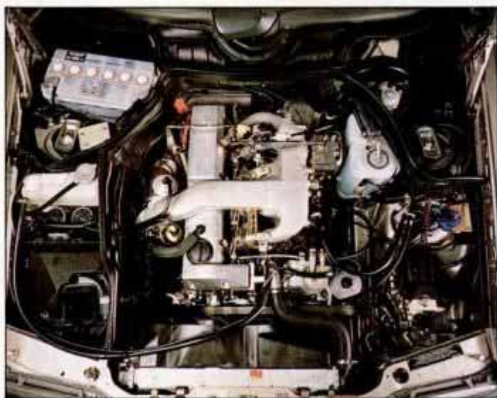
Back on the diesel track, Mercedes-Benz has introduced two new models—the 6-cylinder 350SDL Turbo and the 5-cylinder, 2.5-liter 300D Turbo (engine shown above). Redesigned prechamber improves combustion and reduces emissions.
