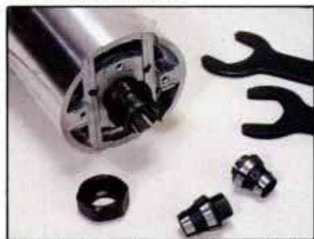
6 A pair of wrenches and 1/4-in.- and 1/2-in.-dia. split collets come with router. A 3/8-in.-dia. collet is sold as an accessory.
