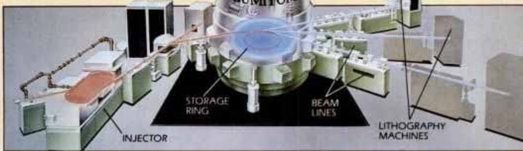
Sumitomo Heavy Industries' Aurora delivers beams radially to X-ray litho workstations.
