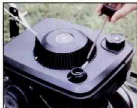
Engine crankcase oil fill tube is conveniently located on the top of the engine. Easy-to-read dipstick is attached to fill cap.
