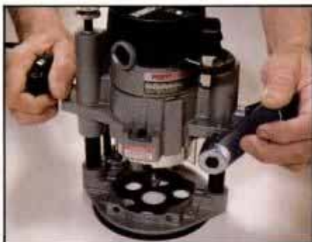
1 Pivot the lever down to lock the router in plunge position. Lever's location near handle makes for smooth and safe use.
