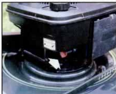
Fuel shutoff valve (arrow) should be turned off when mower is not in operation to keep fuel in carburetor instead of draining out.
