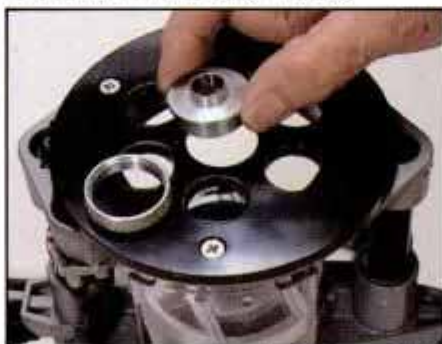
5 The router uses a standard Porter-Cable subbase, edge guide (not shown) and 2-piece template guide, being installed.
