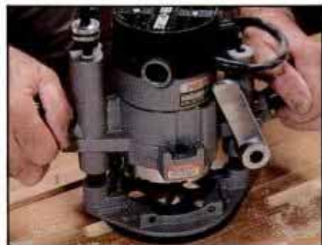
3 At the end of a plunge cut, the lever is pivoted up, and the router is switched off after the bit is safely retracted.
