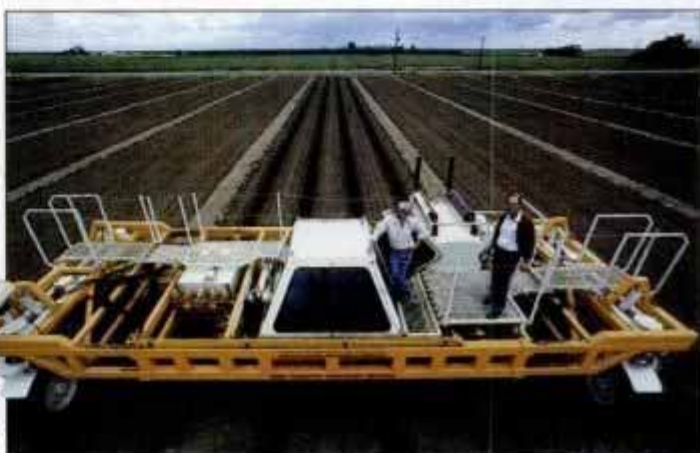
Ultrawide tractor, tested in San Joaquin Valley, boosts alfalfa yields by leaving soil loose and airy.
