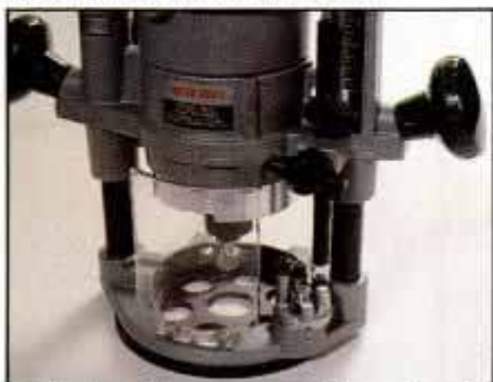
4 The 6-position turret and the adjustable rod control the depth of cut. The turret has three fixed and three adjustable stops.
