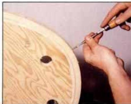
6 When stems have cooled, replace clamps with screws. Brass screws do less damage to cutting tools if they're accidentally struck.
