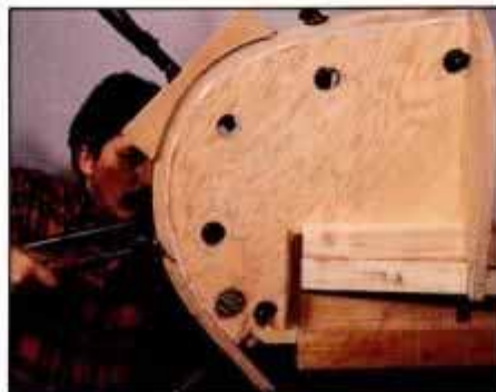
5 After steaming stem blanks, bend around mold. Clamps fit in holes and caul evens pressure on tight portion of curve.
