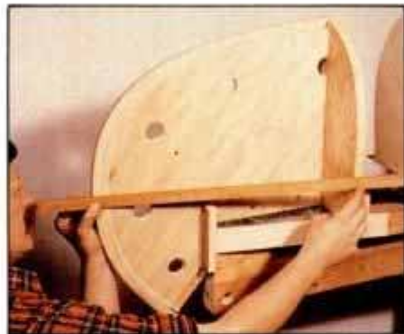
7 Use a fairing batten to determine stem bevel and check for mold alignment. Note rounding of stem end near first mold.
