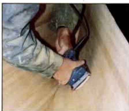
26 Inside of hull is smoothed by sanding. Start with disc sander and coarse paper. Finish with orbital sander and by hand.
