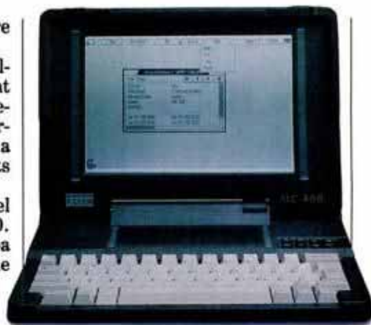
Psion's new MC600 laptop computer uses erasable flash memory IC cards rather than a traditional disk drive. List price for the MC600 is $2999.
