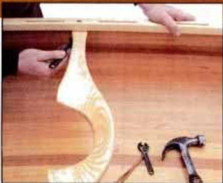
28 Carved yoke makes canoe easy to carry on shoulders. Secure to inwale at midships with bronze bolts, washers and nuts.
