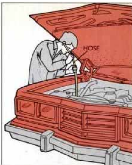
4 A piece of hose makes a good impromptu stethoscope for tracking engine noises.
