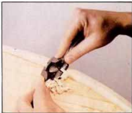
18 After removing false stem screws, trim the stem flush with the planking. Taper stem to meet hull at hull bottom.
