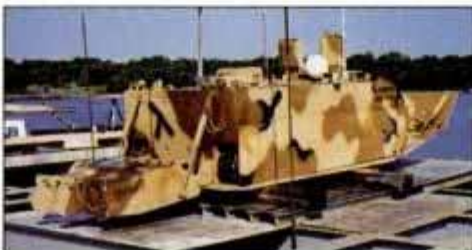
Artist's concept of future planing assault vehicle (above) is based on test bed (left) which recently hit 33.8 mph in Chesapeake Bay tests.
