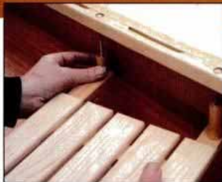
29 Use \frac{3}{4} -in. dowels with holes bored through centers as spacers to align seats parallel to bottom. Secure with bolts.
