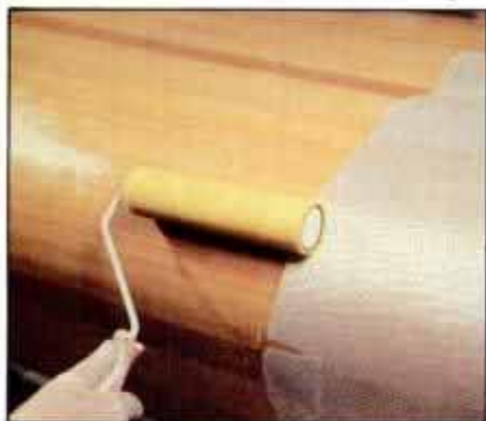
24 Mix 300-ml batches of epoxy resin at a time. Pour a small amount on the hull and work into the cloth with a foam roller.
