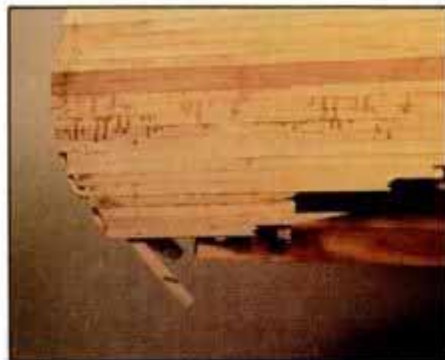
12 With the sides of the hull completed, move back to the bow areas and plank down to the sheer with short scrap strips.
