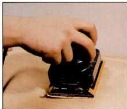
20 After planing, smooth the hull with an orbital sander. Follow by hand sanding with the grain until the hull is smooth.
