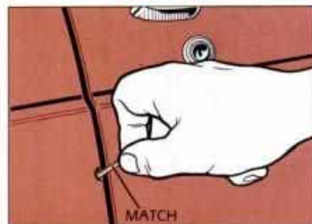
40 Repair chips by dabbing touchup paint into chip with a match or tiny brush.
