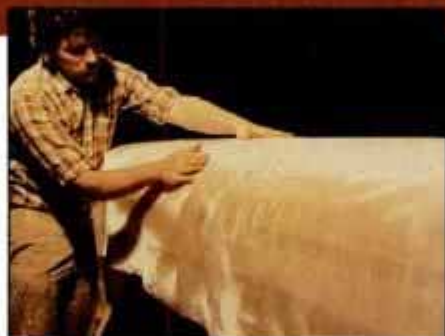
22 Lay a 60-in.-wide piece of cloth over the hull and cut it 1 ft. longer at each end. Smooth the cloth so it conforms to the hull.
