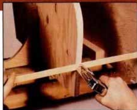
10 Staple the first strip to molds No. 4 through 8 at the sheer mark. Drop the strips about ¼ in. from straight at stems.
