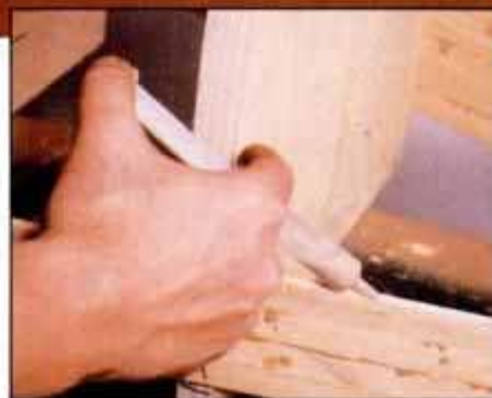
11 Apply glue to strip edge with syringe. Press next strip in place and staple. Alternate sides and epoxy strips at stems.
