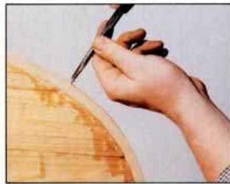
16 After bending false outer stem on separate mold, secure with epoxy and screws. Remove screws after epoxy cures.
