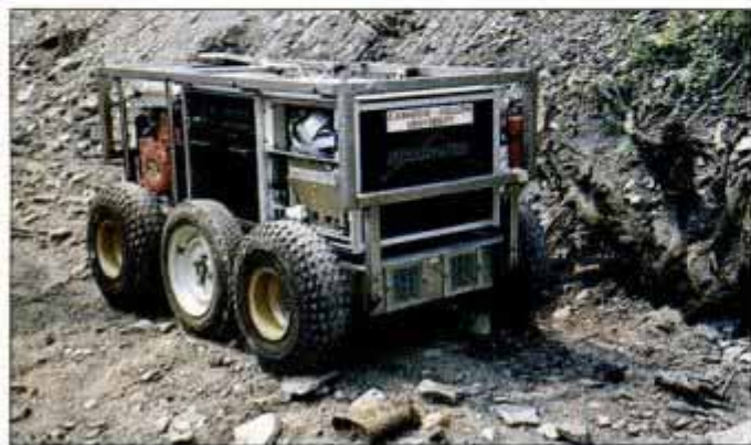
Six-wheeled robot (above) guides ground-penetrating radar over hazardous waste sites, producing image of barrel (top).
