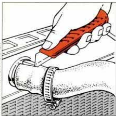
1B Slit a stubborn radiator hose to ease removal, but don't gouge tank connectors.
