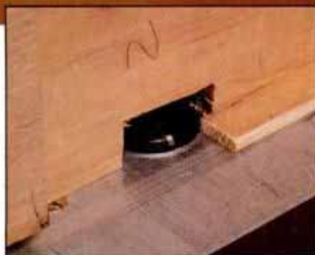
9 After ripping the ¼-in.-thick × ¾-in.-wide strips, shape the ¼-in.-dia. convex and concave edges on the router table.
