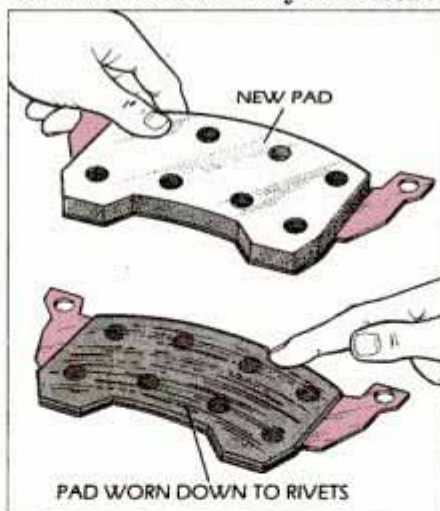
24B If your pads are riveted, you may have to remove them to gauge wear.
