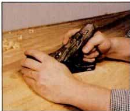
19 Smooth hull with a sharp hand plane. Work diagonally to remove ridges, dents and glue. Then plane with the grain.
