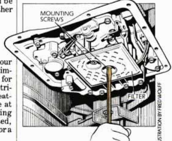
17A You'll find the transmission filter right under the pan, under the valve body.
