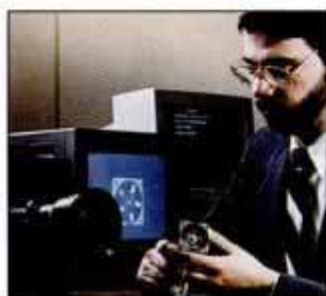
Battelle engineer holds rapidly spinning fan, frozen on high-speed video system behind him.
