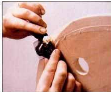
8 Bevel stem with spokeshave while continuing to check with fairing batten. Stop bevel about two-thirds of the way up.
