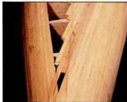
14 Complete one side of the hull, letting strips run over the centerline. Then, snap a chalkline along the center and cut to line.
