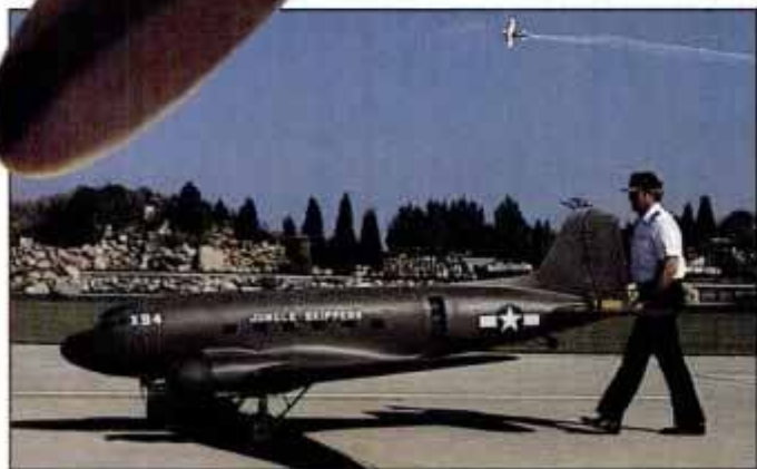
A 1/5-scale C-74 Skytrain is walked out of hangar with a load of tiny paratroopers. This giant, custom-made model has a 19-ft. wingspan.
