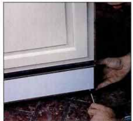
6 Reinstall front panel on dishwasher door, then remove lower access panel. Check owner's manual for proper method.
