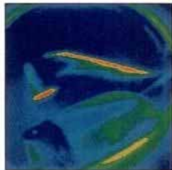
SILTS pod on stabilizer (above) produces false color images (right) showing hot-spot temperature of 1100° in red.
