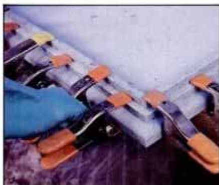
7 Underedge of countertop can be built-up to create different designs. Just join strips to top with fusion material.
