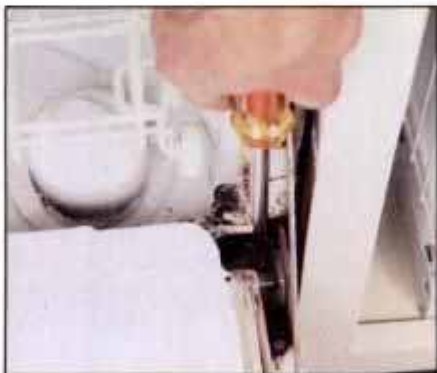
4 Remove screws that hold access panel in place. They were accessible from inside of our unit, once the door was opened.
