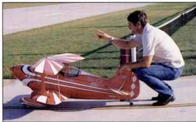
Pitts Special is ready to taxi out to the runway. The 1/5-scale aerobatic biplane model has a 68-in. wingspan and 1400 sq. in. of wing area.
