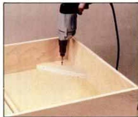
8 Cut corner gussets to size and glue to toe-kick assembly. Then center assembly on island bottom and attach with screws.
