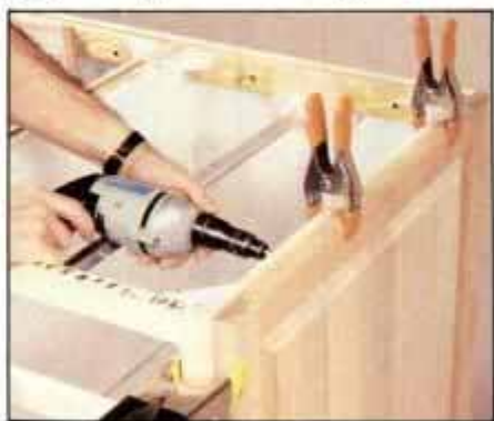
9 Order back and side panels from door and drawer front company. Then, attach by driving screws from inside the cabinet.
