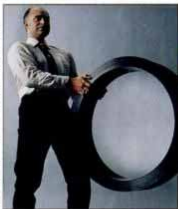
Navy's computer-guided Advanced Unmanned Search System (top) reaches 20,000 ft. with hull made at Oak Ridge (above). Composite sample (left) weighs 82 lbs., steel would weigh 429.
