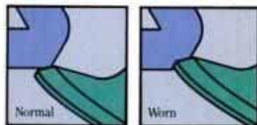
Unleaded gas allows valve seats in certain engines to wear away due to abrasion formerly prevented by lead. Valve Armor protects valves against this expensive damage.
