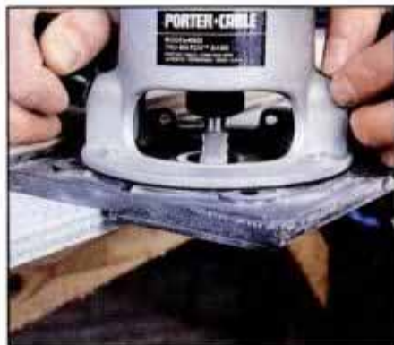
5 Cut seams with Tru-Match routing system. System produces wavy cut that is self-aligning and nearly invisible.
