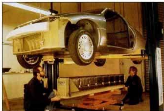
Fill 'er up. Impact's appetite is satisfied by 870 pounds of batteries.
