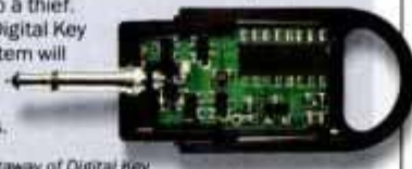
Actual size cutaway of Digital Key
