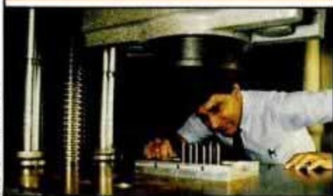
Engineer places sample of sine wave composite in screw jack testing machine to see how it would absorb energy in a crash.
