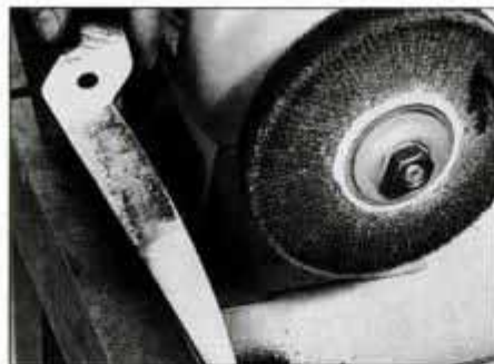
19 To remove tarnish on garden shears and other tools, use a fiber wheel. Always hold tool cutting edge away from wheel rotation.
