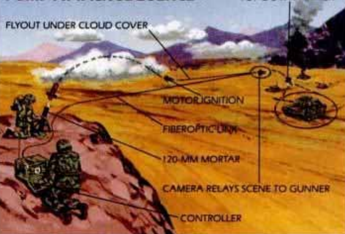
High-speed photograph shows FOMP projectile deploying control wings in flight tests. Illustration delineates path of shell from firing, to ignition of rocket for subcloud flyout, to terminal guidance toward selected target.
