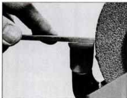
2 Position adjustable toolrest no more than ⅛ in. from wheel. Right-angle position shown produces a square ground edge.
