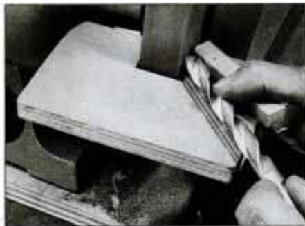
12 Finish sharpening bit by rotating bit clockwise 1/6 turn while shifting it to guidelines positioned at 47° to wheel side.
