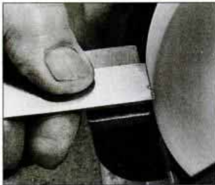
9 To regrind an overheated tool edge, set toolrest to 90°. Grind beyond discoloration. Then, reset toolrest and reshape bevel.
