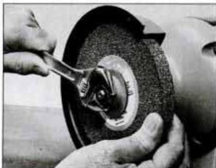
1 Tighten wheel mounting nuts with hand pressure on wheel—never overtighten. Keep washer and wheel face free of debris.
