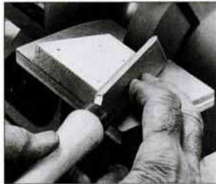
10 Sharpen flat-ground bevel of lathe skew chisel on side-grinding wheel. Jig keeps blade positioned for uniform bevel.
