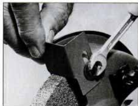
3 Adjust the spark deflectors to within ⅛ in. of the wheel to prevent sparks from flying out over the top of the wheel.
