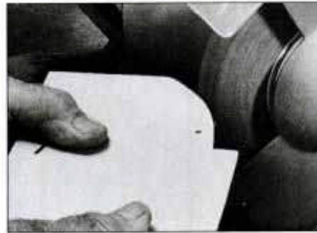
13 To smooth hacksaw marks in metal-working, first set toolrest to 90°. Support work on toolrest and feed against wheel.
