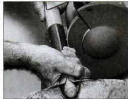
17 Riveted tools like this garden shovel can be disassembled for repair by grinding away the rivet heads with a coarse wheel.
