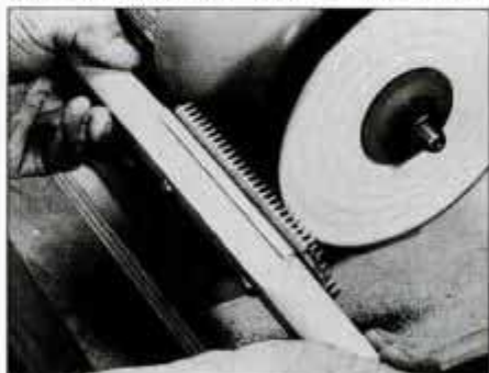
23 Wheel rake is used to dress the edge of cloth buffing wheels. It removes caked compound and trims frayed edges flush.
