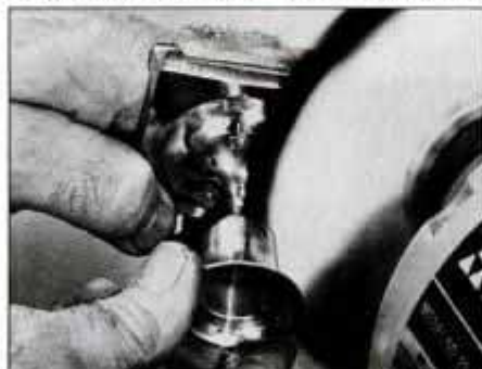
22 Use a loose cloth buffing wheel for reaching into confined areas. Jewelers rouge is appropriate for precious metals.
