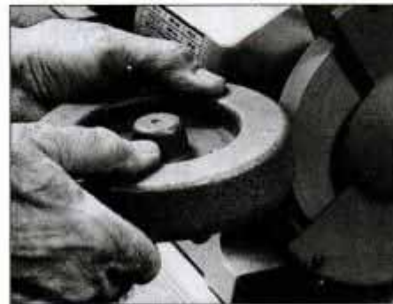
16 Silicon carbide is also recommended for grinding cast iron. Avoid heavy pressure that may overheat and damage wheel.
