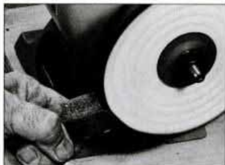
20 Prepare cloth wheel for buffing by pressing compound to wheel edge while grinder is running. Avoid heavy application.
