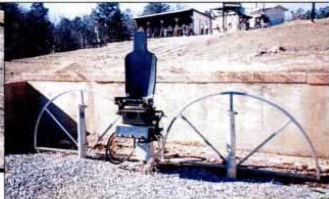
Steyr ACR prototype (above) fires flechettes in 3-round salvos. Sensors in arches next to pop-up target (right) trace paths of bullets that miss.
