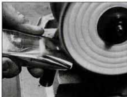
21 Use a cloth wheel loaded with white (pumice) compound to polish chrome. Always hold work to lower section of wheel.
