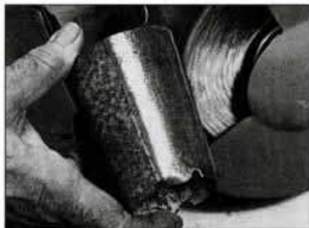
18 Use a coarse wire wheel to remove rust and scaling paint. Fine wire wheels mar less and produce a satin-like finish.
