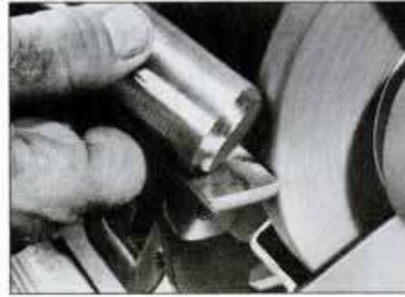
14 Bevel round stock by supporting it on a level toolrest and rotating the stock clockwise while moving across wheel face.
