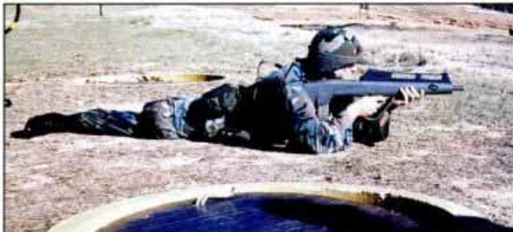
Steyr ACR prototype (above) fires flechettes in 3-round salvos. Sensors in arches next to pop-up target (right) trace paths of bullets that miss.
