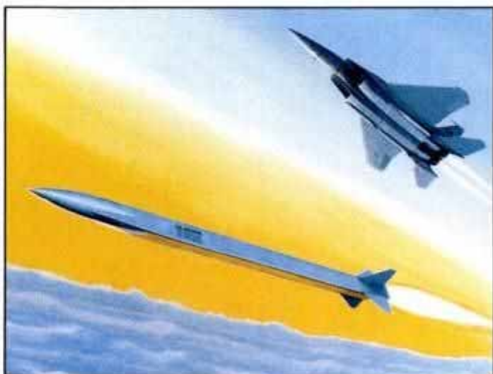
Concept of Have Dash II hypersonic missile shows asymmetrical flat-bottom design that permits bank-to-turn steering.
