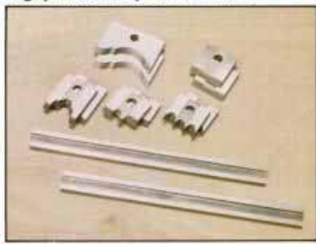
6 Among the available cutters are (top to bottom, left to right): picture frame, rabbet, clover, glue joint, three bead and planer.
