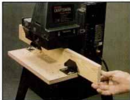
3 Guides bolted to the bedboard support stock for edge planing. The machine can edge plane stock up to \frac{1}{4} in. wide.
