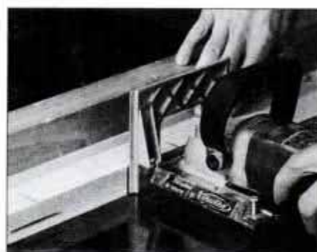
2 The saw table provides an excellent surface to cut slots for joining plates. The saw's fence supports the workpiece from behind.
