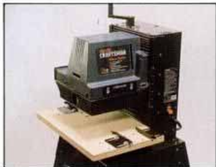
1 The crank, for positioning the cutterhead, and the ON/OFF switch are easily accessible from the machine's feed side.
