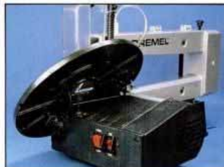
3 The 12-in.-dia. table tilts 45° left for bevel cutting. The ON/OFF and the HIGH/LOW speed switches are next to each other.
