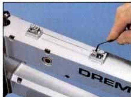
2 Built-in gauge on top of saw helps to accurately attach the adapters on the plain-end blades. Hex wrench tightens the adapters.
