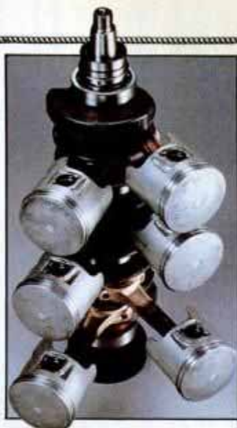
The 250-horse Yamaha V76X (left) features an offset crank (above) to adjust to 76° V and a cross-induction system (below) with six carburetors.
