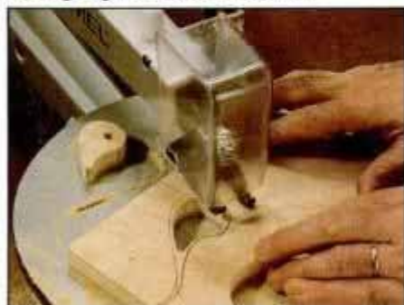
4 At high speed, a fine-tooth blade leaves smooth edges. The blade cuts plywood without splintering along the kerf's edge.
