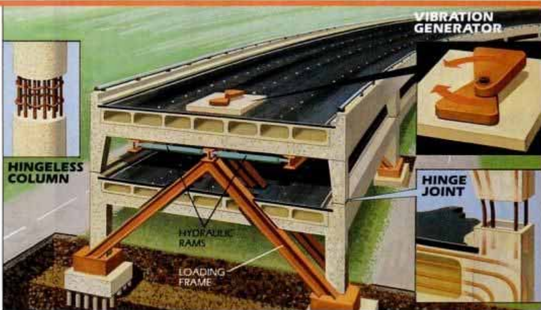
Newer columns (inset left) do without hinge joints (inset right) that failed in collapse of I-880.
