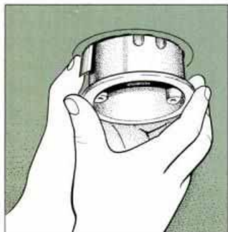
3 Compress bracket and push box into opening until bracket snaps past edge of drywall. Then tighten bracket screws.
