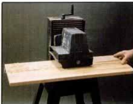
2 The 6-in.-wide cutters can surface boards up to 12 in. wide, in two passes, thanks to the unusual open-throat design.
