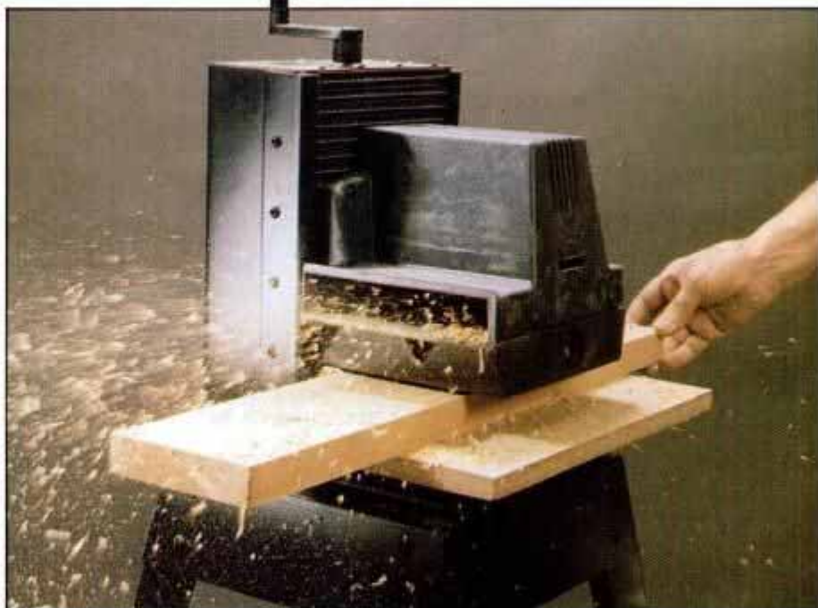
Planer/molder surfaces stock up to 12 in. wide, planes edges and cuts moldings.
