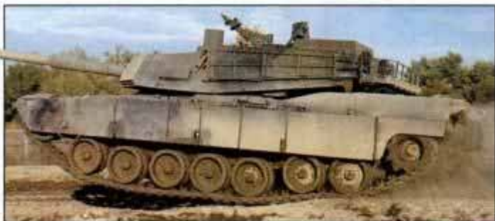
In-arm suspension in trials on M1 tank (left) replaces torsion bars that waste hull space and add weight (below left). Friction damper and gas spring (below right) are kept far apart.
