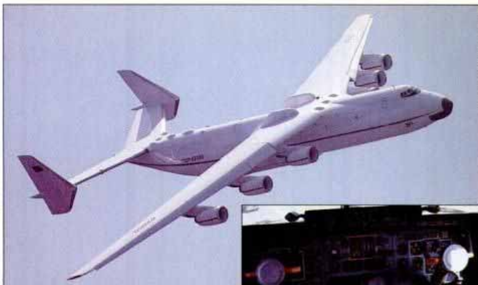
An-225's faired external attach points are arranged for a variety of loads. Cockpit (right) is similar to An-124's, except for extra throttles in the center to control the fifth and sixth engines.
