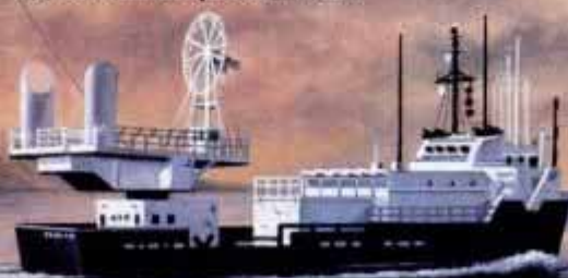
MOBILE AEROSTAT PLATFORM VESSEL Carries tether-handling and support equipment for radar balloon, along with communications gear, to dispatch data to interceptors and C 3 I.
