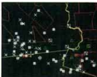
Radar symbology aids sorting at C 3 I West. An X indicates primary track only. Slash is civilian transponder. Box with slash is transponder and primary. Pound sign is coast track, meaning contact has been lost. And green triangle is military transponder.
