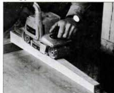
10 With the leg clamped to the workbench, use a belt sander or a hand plane to smooth away saw marks and refine profile.
