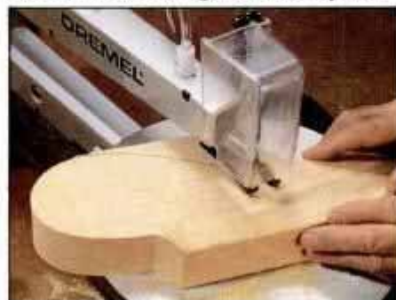
5 The Dremel saw cuts up to 2-in.-thick stock. Built-in blower, powered by saw's reciprocating motion, clears away sawdust.
