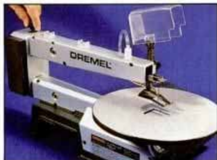
1 Blade tension is adjusted by turning the knob on the top frame. The blade guard pivots to give you access to the blade.
