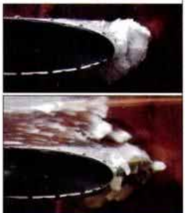
Boot on leading edge expands when current is applied. Wind-tunnel photos show effects on ice.
