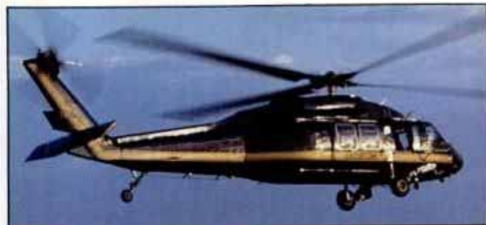
Customs Sikorsky Black Hawk with tail stabilator down for low speed.
