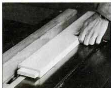
13 Using the dado blades in the table saw, cut groove in apron's back. Groove receives wood buttons that attach top to base.
