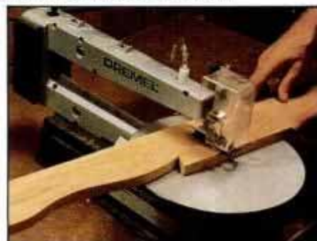
6 The blade is mounted sideways to saw long workpieces. Sturdy construction helps the saw handle large workpieces.
