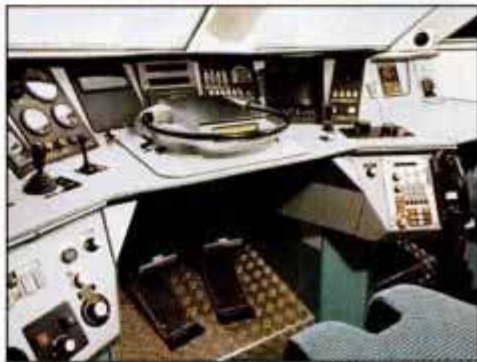
Looking like the Citroën of trains, the ergonomics of the TGV's cab (left) are peculiar but effective. Panel features keyboard and display tied to self-diagnostic system, and to digital public-address system that gives info on LCDs in passenger cars.
