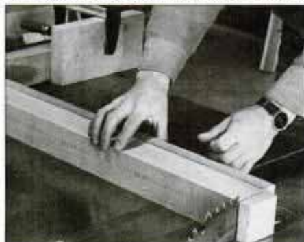
5 Crosscut 2\frac{1}{2} -in.-sq. leg blanks. A stopblock clamped to the fence ensures the legs will be cut to the same length.
