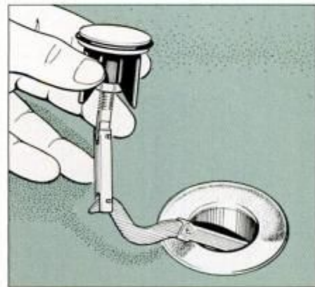
3 To remove hair, or plunge a tub with pop-up tripwaste mechanism, gain access to drain line by lifting out pop-up arm.
