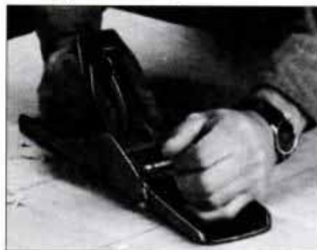
4 Clamp the top to the workbench and use a sharp plane to smooth and flatten the surface. Plane diagonally and with the grain.
