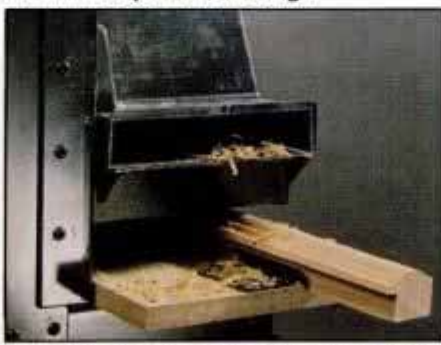
5 In two separate operations, the planer/molder cuts the rabbet and shapes the face of stock to make a picture frame molding.
