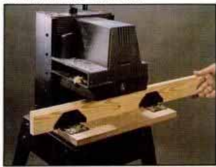
4 Molding cutters are substituted for the planer knives to shape a board's edge. Moldings can also be cut on the stock's face.
