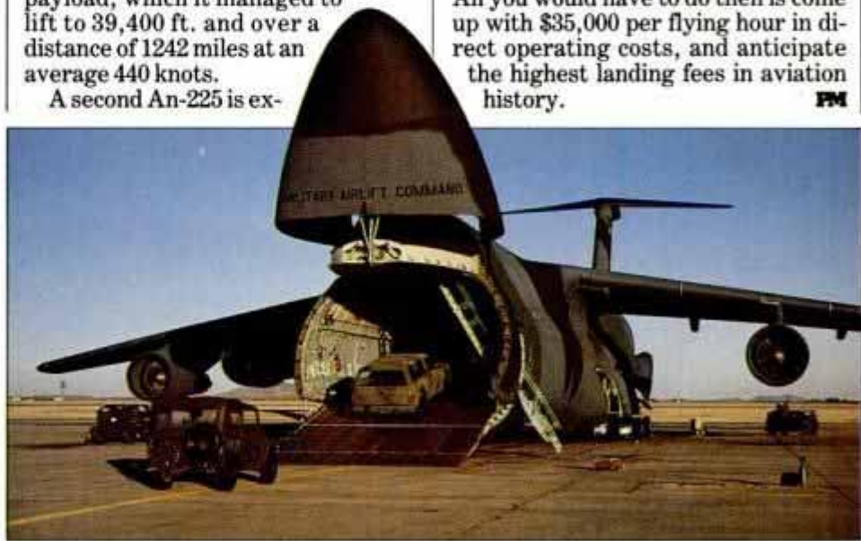
Largely digital instrumentation in C-5B Galaxy is less austere than Antonov's. Yawning C-5 can carry 16 three-quarter-ton trucks, six Apache attack helicopters, or a pair of M1 Abrams main battle tanks.
