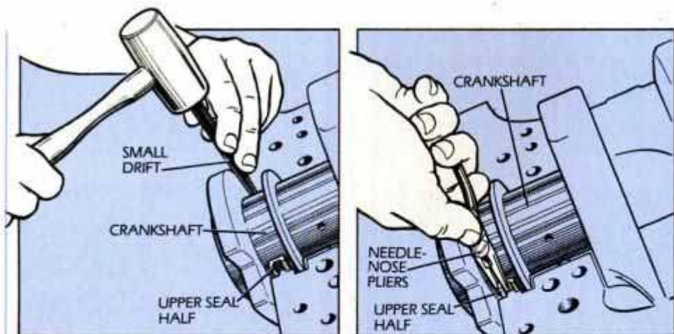
5 Tap the rear main bearing seal into the block (left), then tug on the protruding edge with needle-nose pliers while turning the crank to spin it out (right).
