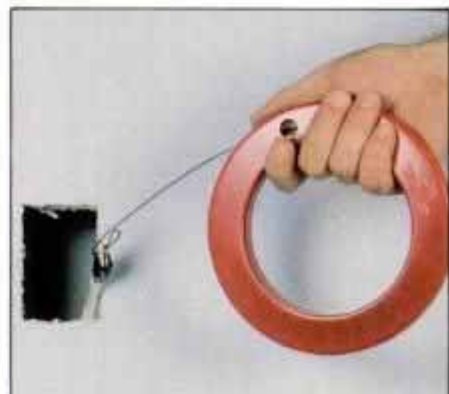
4 Fish tape makes running new wire in enclosed spaces much easier. Just cut opening in wall and feed tape into another opening where new cable is accessible. Then hook cable on end of tape and pull back.
