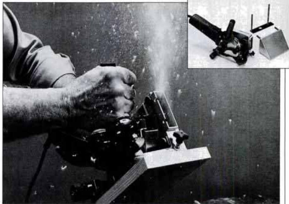
Black & Decker's Elu 3380 plate joiner comes with fence and miter guide (inset).
