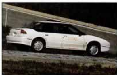
Evolution of Saturn's glass post styling can be seen in this series of shots, taken over several months during prototype development. Glass wraps around A- and C-pillars to provide airy, open feeling.
