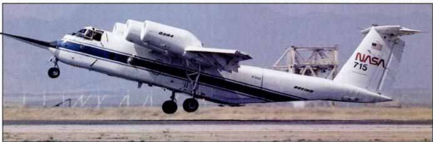
NASA's OSRA research craft will be fitted with a jump-strut nosegear for flight tests at Ames Research Center this fall.
