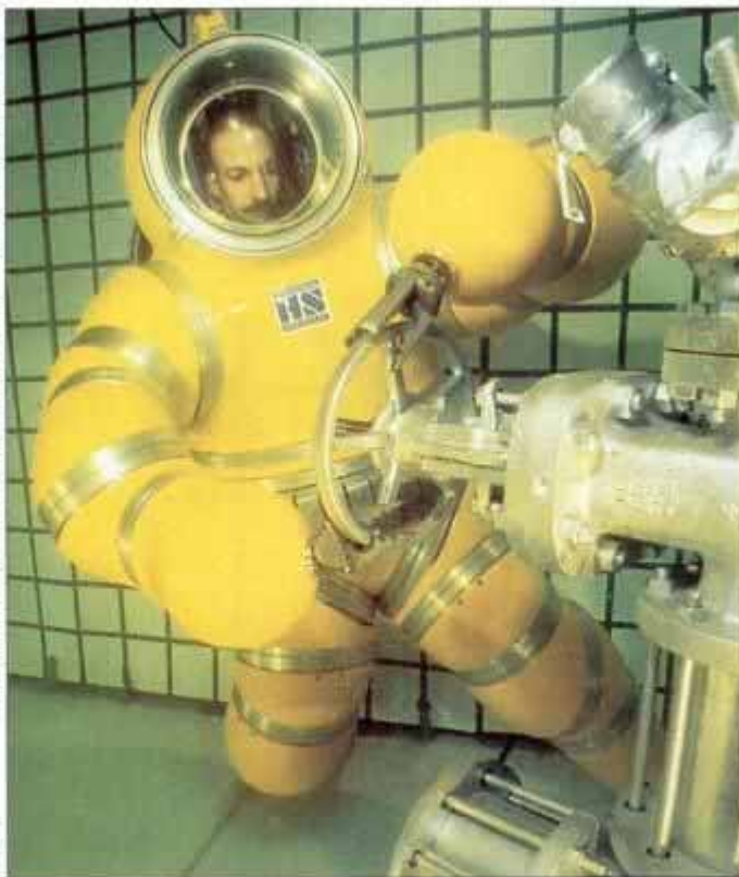
Under pressure: Divers (top) breathe hydrogen mix while working more than 1700 ft. down. The Newtsuit (above) represents another approach, keeping the diver at sea-level pressure, while preserving much of his dexterity.
