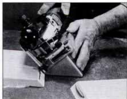
4 Use the miter guide to cut box miter slots. The blade is off-center on the mitered face so it won't break out back of stock.
