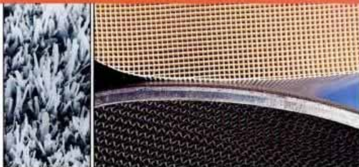
Metallic whiskers shown in micrograph (left) secure catalysts to metal monolith, shown below conventional ceramic (right).
