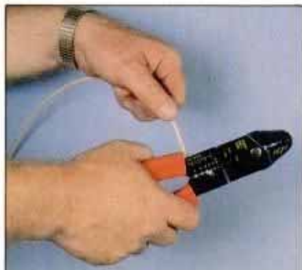
3 Multi-tool cuts cable and strips insulation from wire. To use, just insert wire into proper gauge slot and squeeze the handles together. Then twist tool around wire and pull off insulation.
