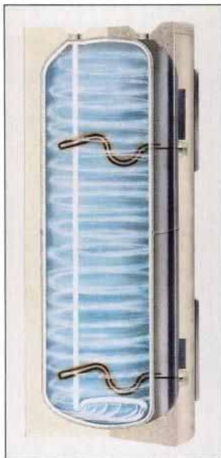
New water heater has just one welded seam around middle of tank and baked-on plastic coating inside to prevent rust. This design also eliminates need for anode.
