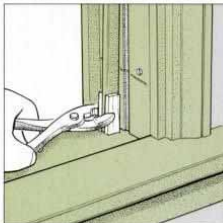
11 Use pliers to pull the parting strip out of its groove so you can remove upper sash. Protective wood strips prevent damage.
