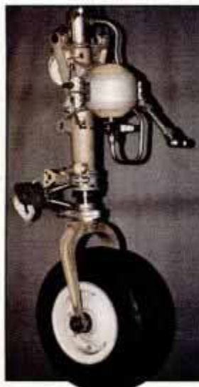
NASA's OSRA research craft will be fitted with a jump-strut nosegear for flight tests at Ames Research Center this fall.
