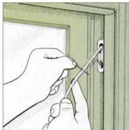
9 Pull on cord until sash weight hits pulley, then slip nail through cord. This keeps sash from being pulled back into jamb.
