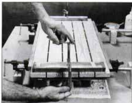
2 Place panel on clamps between clamping pads and tighten slightly. Then lightly clamp cross supports on both sides of each end.
