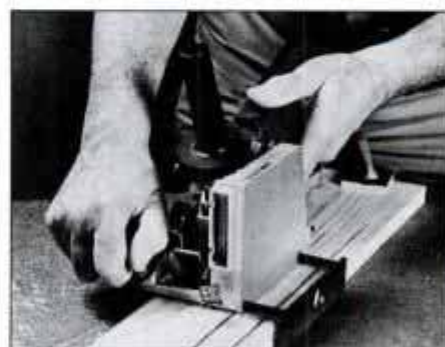
6 In an operation similar to cutting a row of slots, the joiner is held down and pushed forward to cut spline grooves.
