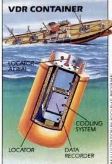
Sealed in its protective vessel, VDR floats free of a wreck, carrying answers for investigators.
