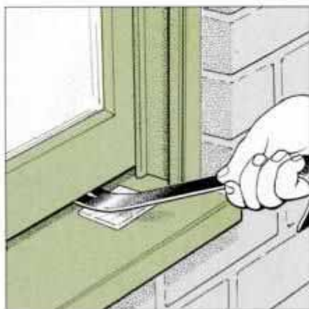
2 Move outside and force a pry bar between the sash and sill and pry up the sash. Scrap wood pad protects sill.
