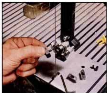
Remove metal guide blocks from saw and replace with plastic blocks. Blade will form its own seat in blocks to prevent twisting.
