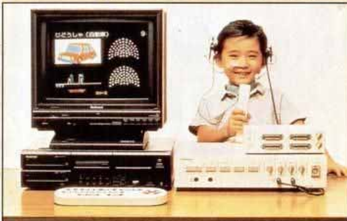
Speech trainer shows graphics in response to headgear sensor input.
