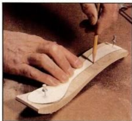
3 After cutting the side profile, trace plan view on spoon blank. Keep pattern tight against curve as you trace.
