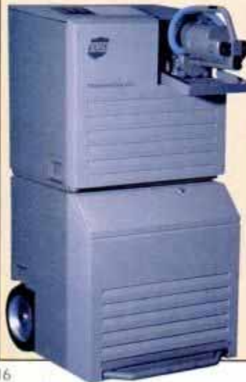
Handheld collector (above) sucks up 2 liters of air per second, then is inserted in Thermedics analyzer (left).
