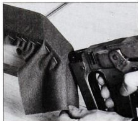
28 At corner pockets, finish stapling cloth over the rail by driving two staples, just beyond cushion facing, into rail end.
