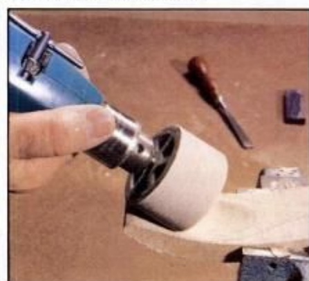
5 Smooth away carving marks with sanding drum in electric drill. Move drum over bowl from front to back.
