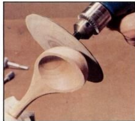
9 As with spoon, shape back of ladle with sanding disc. Cushion ladle handle in vise with foam or piece of cloth.
