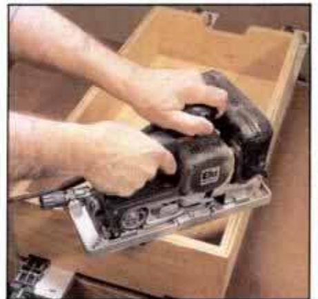
5 Sanding frame keeps sander level to prevent gouging on broad surfaces or spans two edges, as with drawer top.
