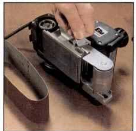
2 To change belts, lift lever on sander's side to retract front roller and release tension on belt. Then slide belt off.
