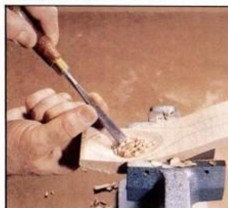
4 Hollow the spoon bowl using a fishtail (shallow curve) gouge. Push gouge from bowl's rim to its center.
