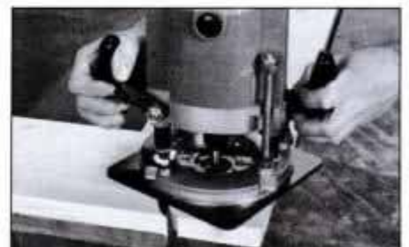
2 Cut away liner at corner and side pockets. Use either a sabre saw or a straight bit and ball-bearing pilot in router.
