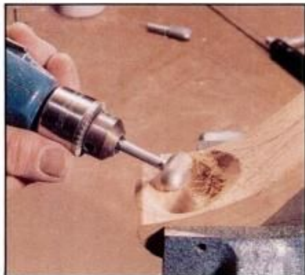
8 Use a rotary file in electric drill to hollow ladle bowl. Make arcing passes, moving file right to left to counter file's spin.
