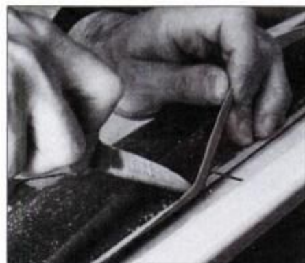
26 Trim off cloth that extends beyond feather strip using a sharp knife. Trim on cushion side (waste side) of strip.
