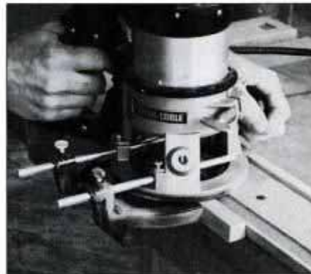
21 Clamp rail liner to bench top. Cut shape on edge of rail cap. Ebony rail sights have been glued in and sanded flush.
