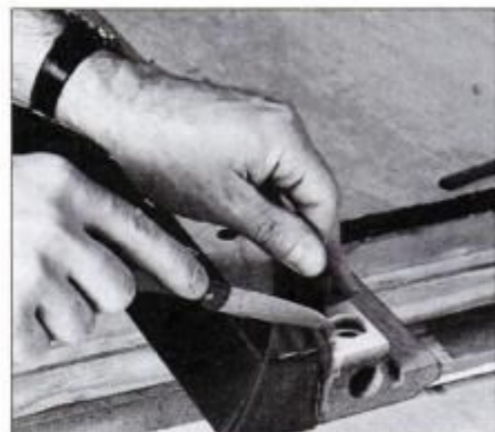
29 At the side pockets, fold cloth over rail end and staple under rail. Trim cloth with knife, leaving ¼ in. beyond staples.
