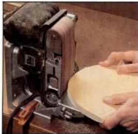
3 Unscrew front handle and bolt sander to cast-aluminum stand to convert it to benchtop sander. Table tilts to 45°.
