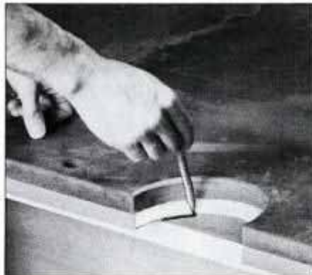
14 Lay slates on frame and trace pocket cutouts and rail bolt holes. Remove slates and mark setback cutting line.
