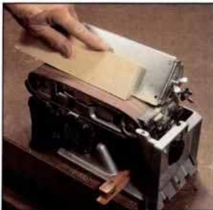
4 Sander and stand can be tipped over and clamped to bench. Sander table is repositioned to serve as tilting fence.
