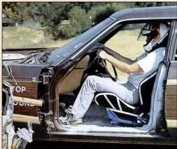
Safety seat, demonstrated here in 45-mph crash without seatbelt, leans back to keep driver's head and chest from contacting the wind-screen or the steering column.
