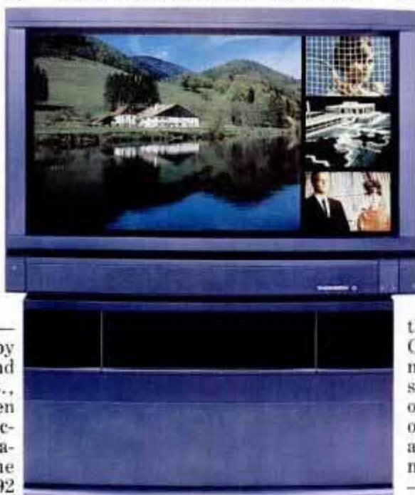
Ready for HDTV: Thomson's 16-to-9 format TV with 34-in. widescreen tube debuts in Europe next fall. It also can display four regular TV shows, as above.
