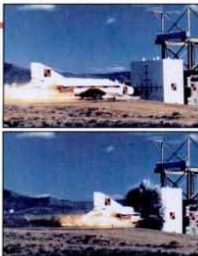
Footage shows Phantom's split-second demise. Plane disintegrated completely, except for small sheared-off sections of tail and wingtip.
