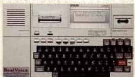
Realvoice laptop provides speech impaired with voice, print and LCD outputs.
