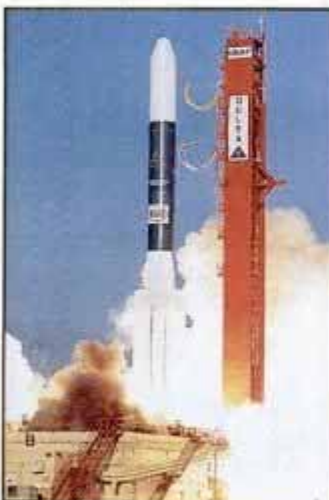
Delta II bearing Marcopolo 1 departs Cape Canaveral. Six of nine solid rockets fire for liftoff.
