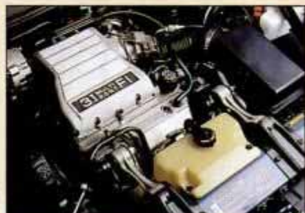
GM-10 platform and Euro suspension make Lumina an agile slalom performer. Dashboard seems borrowed from another era. Port-injected 3.1 V6 gives good jump off the line.
