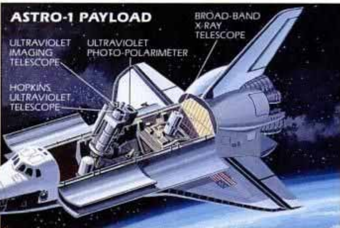
Astro-1 correlates data from X-ray and ultraviolet instruments.
