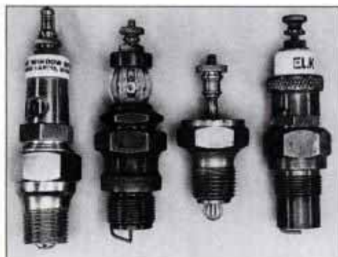
"Visible" plugs had small windows that allowed observers to locate dead cylinders at a glance.
