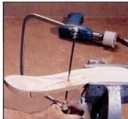
6 Cut spoon's plan profile by sawing toward blank's center. Switch the blank end for end in vise to finish cut.
