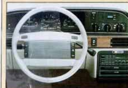
Taurus handling conveyed sense of solidity to test crew. Instrumentation is new for 1990, as is driver's airbag and knee bolster. Vulcan 3.0 V6 gave Taurus acceleration honors.
