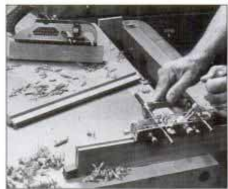
12 After cutting lid panel tongues with rabbet plane, use combination plane to cut matching grooves in capping pieces.
