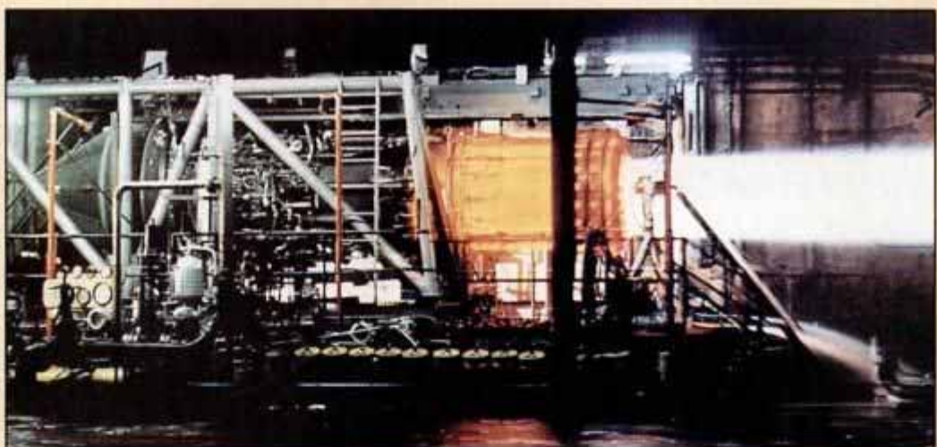
Instrumented-technology demonstrator engine is fired up to test IHPTET components.
