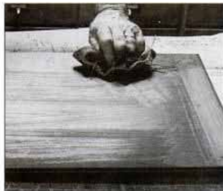
3 When filler dries and dulls, wipe away excess with burlap. Work across grain to fill pores and then wipe with grain.
