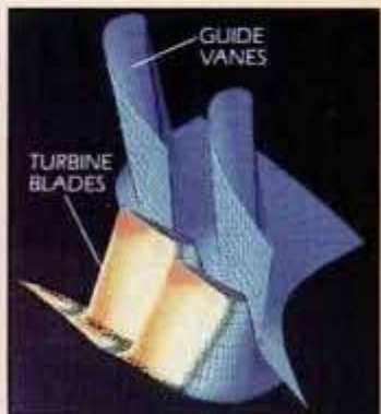
Computer model tests aerothermodynamics. Pressures are highest in blue, lowest in orange.
