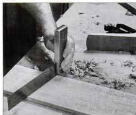
7 Check the surface frequently for flatness. After planing diagonals, plane with the grain and finish with smooth plane.
