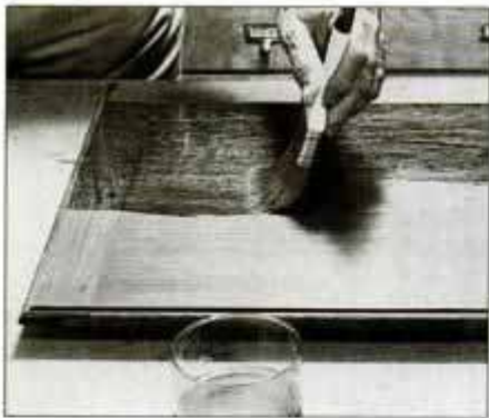
4 Thin, wash coat of shellac is used after stain and filler to seal surfaces. Lightly sand when dry. Also, shellac unexposed areas.
