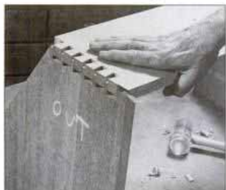
9 Test fit dovetails. Joint should require only light tapping to bring pieces together. Trim where necessary with sharp chisel.
