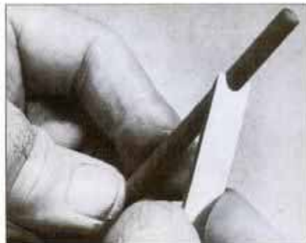
17 Hone concave edge of beading cutter with round slip stone. Periodically hone back of cutter to keep profile sharp.
