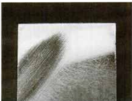
9 Closeup view of chisel-back surface illustrates factory grinding marks that have been honed away at the tool's edge.
