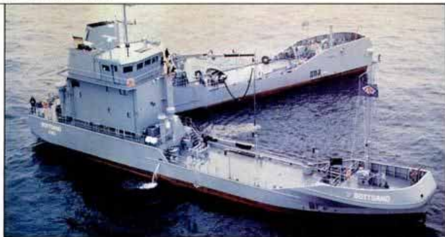
In oil-recovery mode, the hull of the oil-recovery vessel Bottsland gaps into a V to funnel oil toward ORAS equipment, which will separate it from water.
