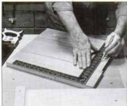
13 A large steel square is used to mark crosscutting lines square to edge. Lines indicate exact finished length of piece.
