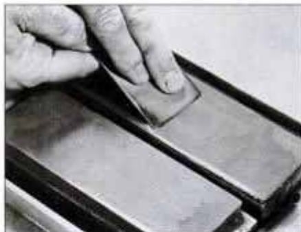
11 Firmly hold tool with both hands while passing over entire surface to help distribute wear. Maintain consistent angle.
