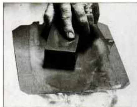
3 Water stones must be frequently trued for a straight honed edge. Use waterproof abrasive paper and water on flat surface.
