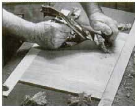
1 After the glue has dried on the edge-joined bottom panels, hand plane both surfaces so the panel is uniformly 1/4 in. thick.
