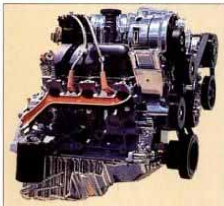
Ford's new 4.0-liter V6 brings much-needed muscle to both Ranger and Bronco II lineups.
