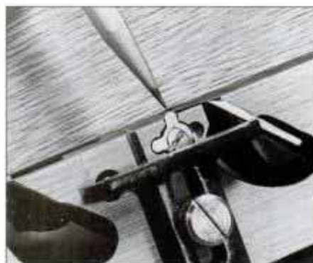
1 Closeup shows spur in position for cross-grain cutting. Rabbet plane (shown) has single spur, combination plane has two.
