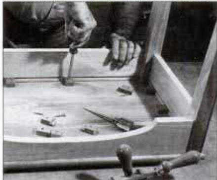
4 Bore the holes in the base for securing the buttons. Install buttons to ensure that components fit properly and then remove.
