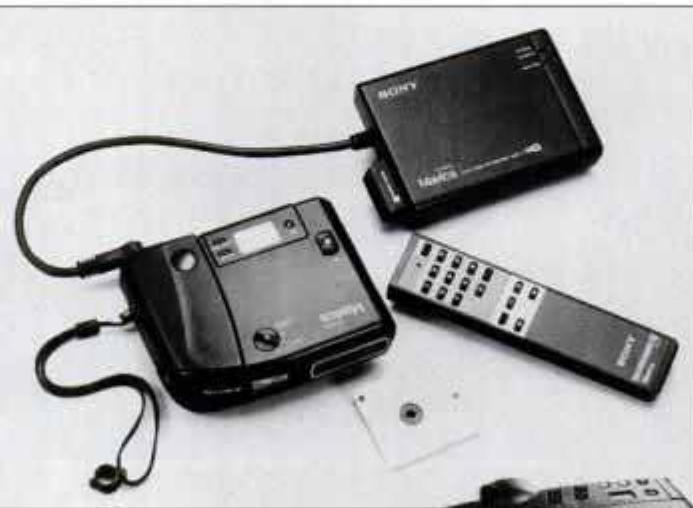
New, all-electronic still video cameras from Sony (above) and Canon (right) record images on magnetic disks instead of film. The images are displayed directly on a TV monitor—no developing is required.
