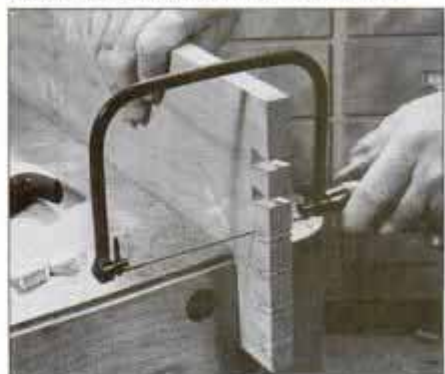
6 Remove most of the remaining waste with a coping saw. Don't cut too close to base line to avoid overcutting.
