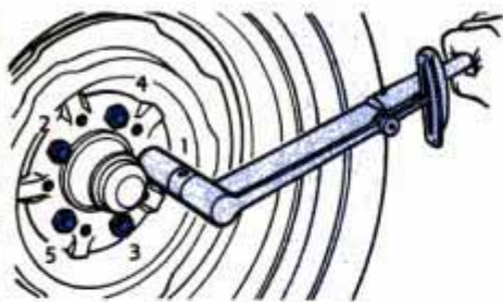
3 Torque wheels in an alternating pattern to avoid wheel or hub distortion. Check your owner's manual for the correct torque spec.
