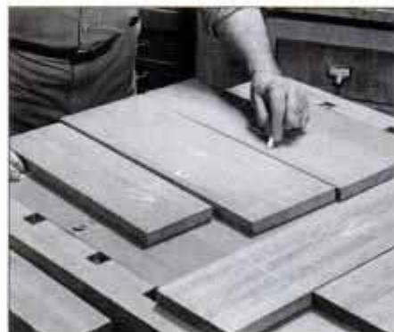
9 Wide panels are made by edge gluing narrower boards. Plan to assemble panels with grain of each board in same direction.
