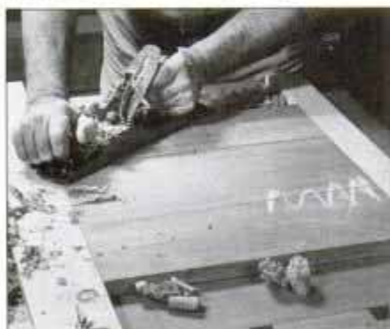
16 Fine diagonal cuts remove excess where necessary. When first side is true, flip panel over and plane other side parallel.
