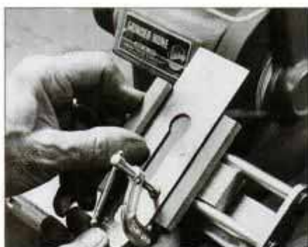
7 Adjust tool rest to bevel angle and slowly advance blade toward wheel. Keep blade moving and cool edge in water.
