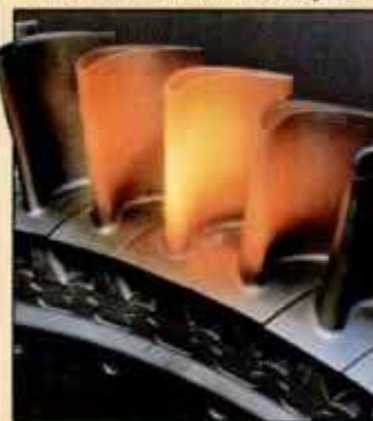
The turbine blades (above), each one a single crystal of alloy, are latest materials technology. Burner (right) tests future alloys.
