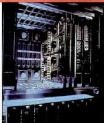
ES-1 circuitry (above) has up to 128 computational units. In flow diagram (right), units shunt commands from green instruction area into blue floating point and red integer areas for processing. Data from main memory is prefetched into high-speed cache memory, and even higher speed register memory, so processors aren't kept waiting.
