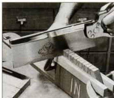
2 Clamp guide strips to the board, aligned with base line, to act as depth stops. Make cuts on waste side of line.
