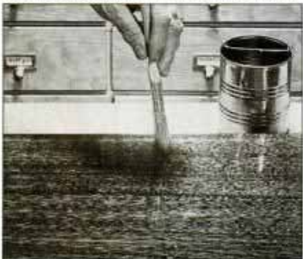
7 After wiping brush slowly across wire, hold it vertically and stroke lightly with grain, barely touching surface.
