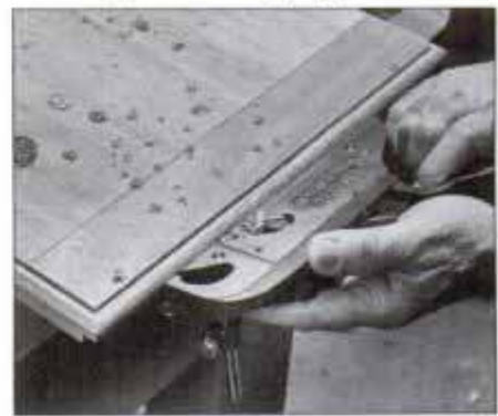
15 Finish lid by planing quarter round. Start with 1/8-in.-deep rabbet. Chamfer uniformly and progressively round corner.
