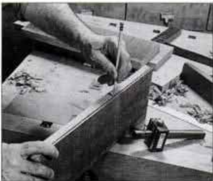
5 Sharp pencil makes scribed line visible. To remove remaining stock quickly, use rounded cutter adjusted for coarse cut.
