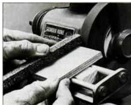
1 Dress grinding wheel flat with a silicon-carbide dressing stick. Use a coarse (60-grit) wheel for shaping bevels.
