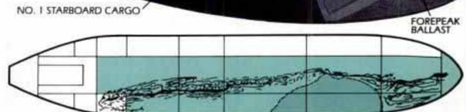
Initial grounding left a gash running from the Valdez's forepeak to her starboard slop tank. The 11 colored tanks were all holed. Darkened area was caved in when she came to rest.
