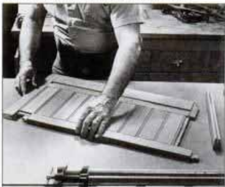
2 Dry assemble the back first to check for good fits and proper panel spacing. Then, apply glue to frame joints and clamp.
