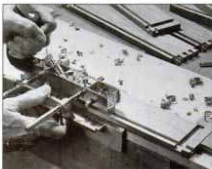
5 Cut grooves with combination plane. Start with drawer fronts aligning groove with dovetail cavity. Then, groove sides.
