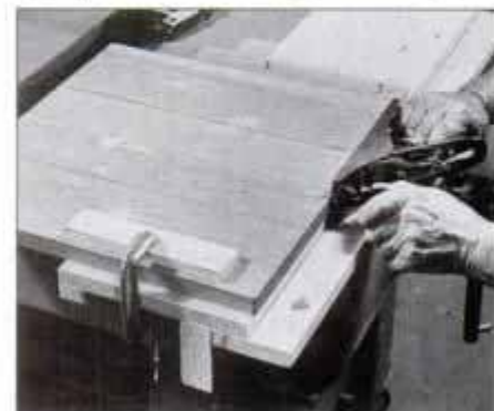
18 A shooting board makes end grain trimming simple. Note small chamfer on end which keeps end grain from splitting.
