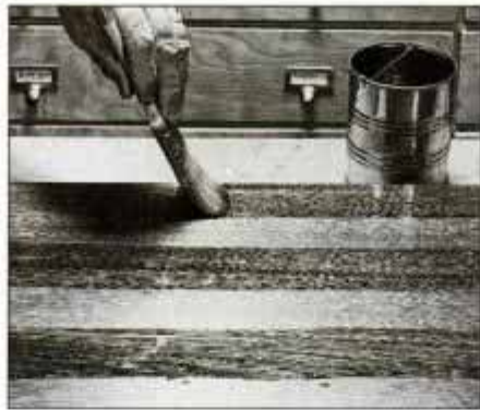
5 Apply varnish with grain in stripes about one brush width apart. Brush slowly to flow varnish on with minimal bubbling.
