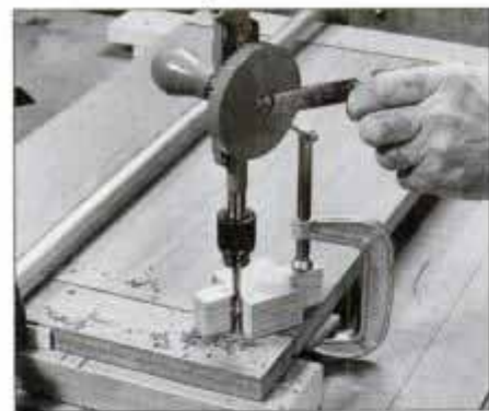
13 Clamp end capping pieces tightly to panel and bore holes for pins. Boring guide helps keep bit square to work surface.
