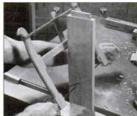
17 Lay out front apron curve and saw to line with a bow saw. Remove saw marks with sandpaper and curved sanding block.
