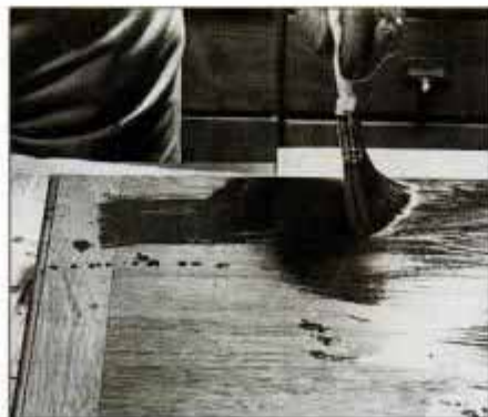
2 Paste wood filler is applied with stiff brush in direction of grain. Japan color is added to filler to match color of stain.
