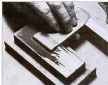
20 Hone the cap-iron end to a straight, sharp, knife-like edge so it fits tightly against the back of the plane iron.
