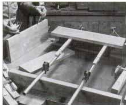
11 Set pipe clamps on 2x4s and apply glue to board edges. Prepare four straight pieces for clamping across panel ends.
