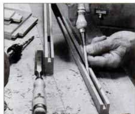
9 Use a sharp, 1/4-in. chisel to remove remaining waste from mortises. Note that width of mortise is determined by groove.
