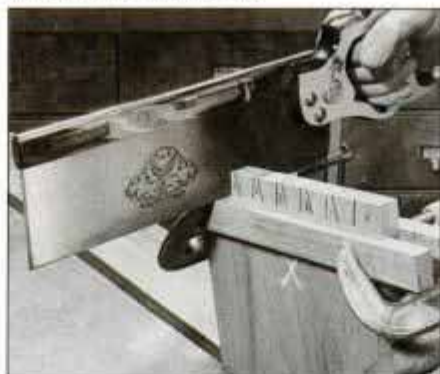
5 After marking cutlines, use a backsaw to cut to waste side of line. Tilting board in vise allows saw to be held vertically.
