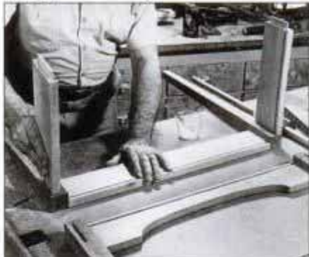
3 Test fit leg mortise-and-tenon joints. Use pipe clamps to glue assembly together and check for square by measuring diagonals.
