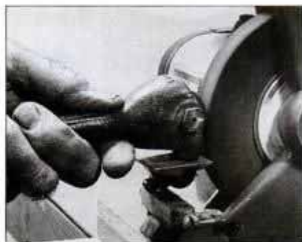
2 A clogged or glazed grinding wheel will generate too much heat and cut poorly. Open pores with star wheel dresser.
