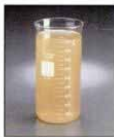
Deposits removed using water alone
