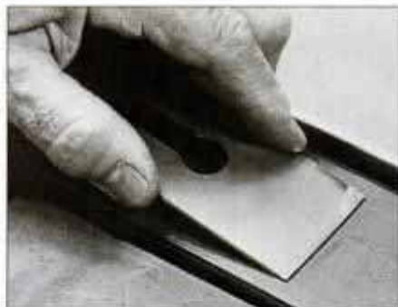
10 Begin honing hollow-ground bevel by lifting blade until heel and toe contact stone for the correct honing angle.
