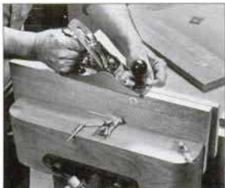
10 Joint mating edges by folding adjacent boards together and planing both at once. Plane a perfectly straight edge.
