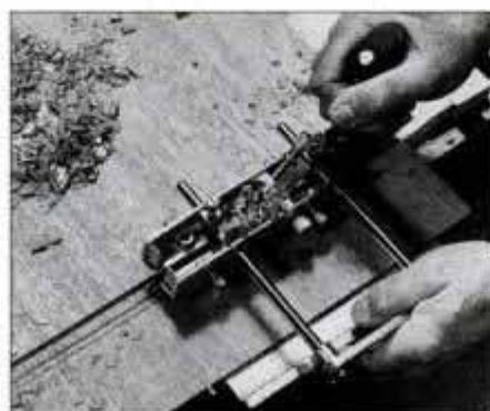
2 Cut dado using combination plane with spurs set for cross-grain work. Fence guides cut. Wide cuts may require two passes.
