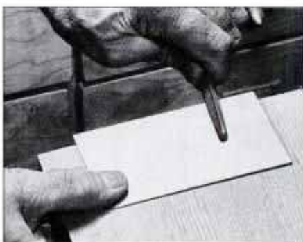
26 To create cutting hook on scraper, begin by holding scraper firmly on the bench edge and drawing burnisher across face.
