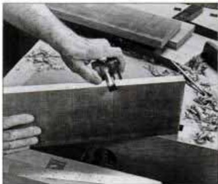
4 After planing edges square to completed face, use a marking gauge to scribe finished thickness on both edges of the board.
