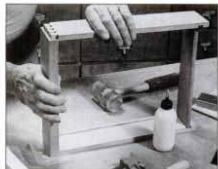
6 Apply glue to the dovetail joints and back dado. Then clamp the front, sides and back square and install bottom panel.
