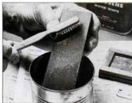
4 Use a stiff brush and kerosene to clean and rejuvenate clogged or glazed oil stones for faster and easier honing.
