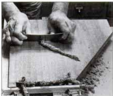
1 A properly sharpened scraper does an excellent job of smoothing surfaces and removing slight ridges left by planing.
