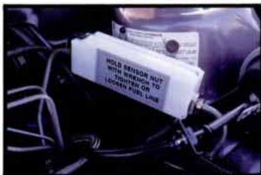
Under the hoods of the cars tested are all the familiar components, plus a fuel-line sensor to measure the proportion of methanol to gasoline fed to the engine. Sensor data allow engine computer to adjust to mixture.
