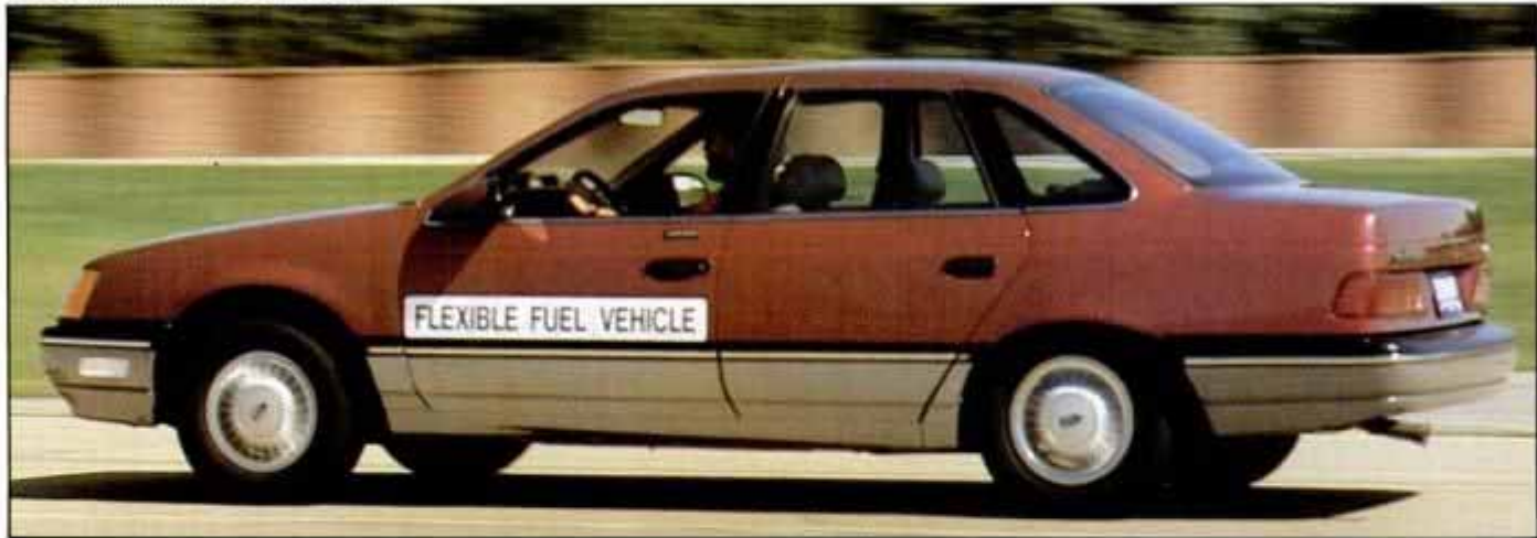
FFV Taurus was slower than gas-powered Taurus, although tests show 6-hp gain to 162 hp using 85-percent methanol/15-percent gasoline.
