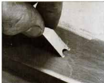
16 Sharpen beading cutters of combination plane by first gently honing flat sections. Then, hone back of cutter smooth.
