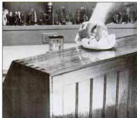
9 After polishing with rottenstone and water, apply paste wax. Let wax dry for 20 minutes, then buff with a soft cloth.
