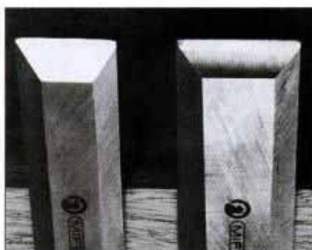
8 Flat-ground bevel (left) compared to hollow-ground. Note uniform grinding and concave surface of hollow grinding.
