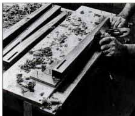
19 Use shooting board to plane the taper smooth. Place \frac{1}{2} -in.-thick strip under plane to center plane on stock.
