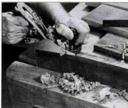
2 Plane both edges of each board straight and relatively square. Longer jack plane trues the rough, irregular edges quickly.
