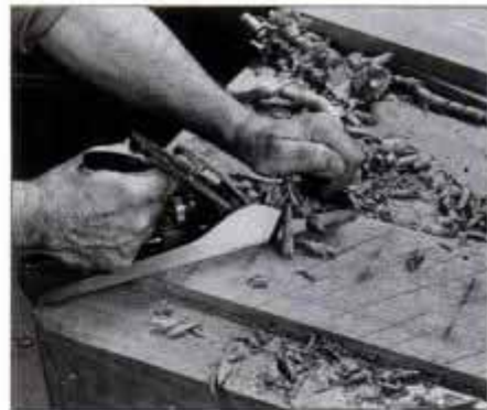
6 Begin second surface by planing diagonally starting at one corner and working across. Then, plane opposite diagonal.
