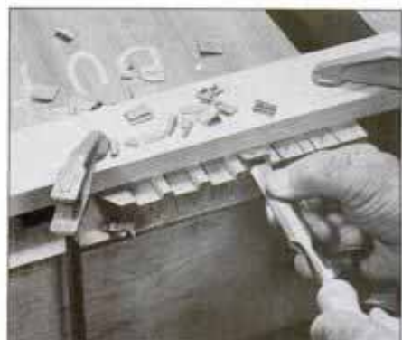
3 Remove dovetail waste gradually. Use a chisel to chop vertically from above and then horizontally from the board end.
