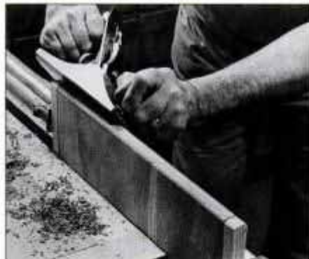
5 Plane rounded base edge on end grain first. Scrap stock clamped at ends prevents splintering. Then, plane long grain edges.
