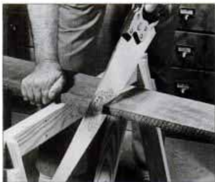
1 Mark the rough lumber and cut with a sharp crosscut saw. Cut each piece square and oversize to allow for trimming.
