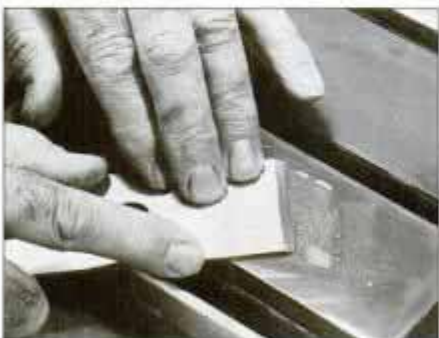
12 After removing wire edge by honing back on coarser stone, hone bevel and back on polishing stone for mirror finish.
