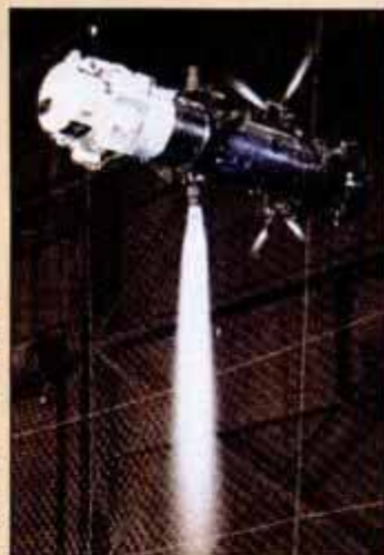
A recent SDIO experiment tested Brilliant Pebbles' stability in full-thrust mode.
