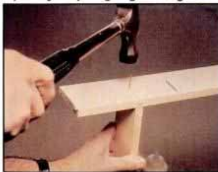
14 Assemble drawer with glue and nails. Check diagonals for square and adjust as necessary. Sand front before attaching.
