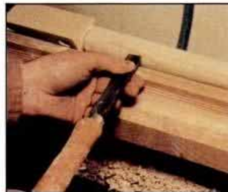
6 Use ¾-in. or 1-in. gouge to turn tapered portion of legs. Use ⅜-in. gouge to shape small cove at top of leg.
