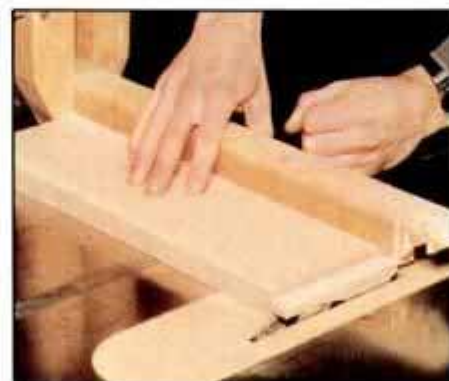
8 Cut tenon on table saw using dado blades and miter gauge. Parallel jaw clamp acts as stop for positioning workpiece.
