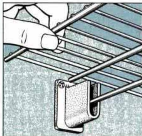
5 Pivot shelf away from back wall and place side-wall bracket over end of rail. Level shelf and screw bracket to wall.
