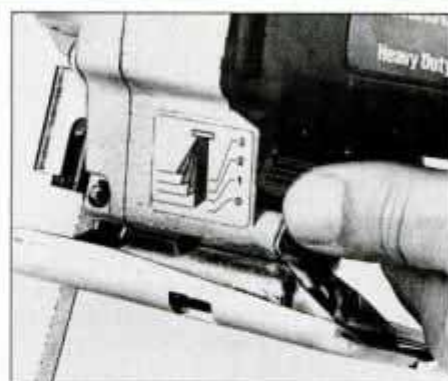
Black & Decker orbital adjustment lever is mounted behind housing and pivots at center. It can be operated from either side.
