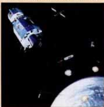
Brilliant Pebbles deploys from its life jacket and homes in on ICBMs picked up by an orbiting BSTS satellite (right).
