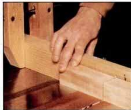
5 Cut ⅜-in.-deep kerf around leg blanks to prevent chip-out when turning. Extend miter gauge with scrap piece.
