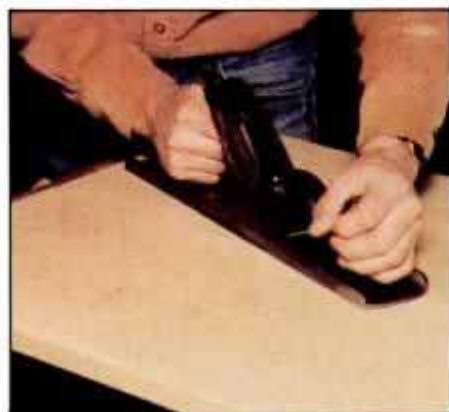
2 Use a sharp bench plane to smooth and flatten panel's top. First, plane diagonally across the panel, then with the grain.
