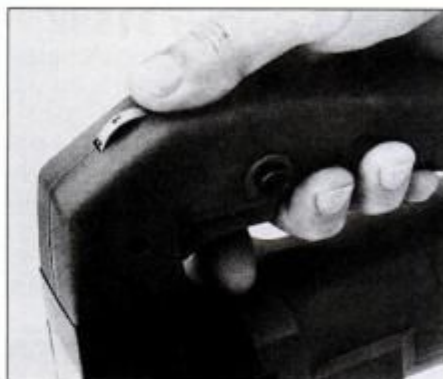
Trigger on saws with separate speed dial simply acts as ON/OFF switch. Cutting speed can only be varied by adjusting dial.
