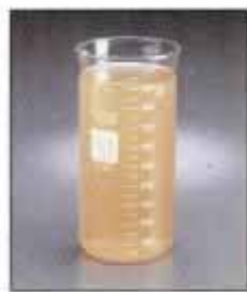
Deposits removed using water alone
