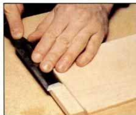
9 Remove ridges left from dado blades by carefully pushing chisel across tenon. Hold chisel flat against workpiece.
