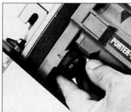
Porter-Cable sabre saw features orbit selection dial behind housing. Ryobi control is similar but mounted in housing.
