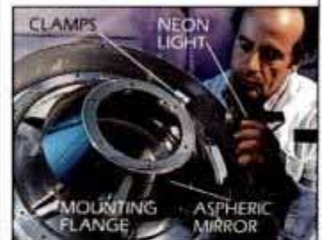
Machinist checks aspheric, grazing-incidence UV mirror.
