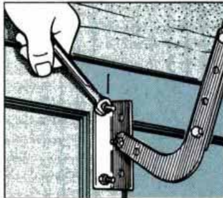
20 Fasten bracket with carriage bolts. Bore bolt-shank clearance holes through door and insert two bolts from outside.
