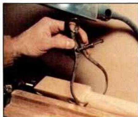
7 Check large and small diameters with calipers. Smooth leg progressively with 100-, 120- and 220-grit sandpaper.
