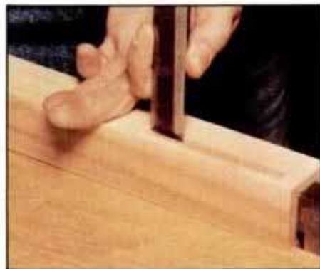
4 Pare walls of mortise flat with chisel, working carefully to mortise lines. If tenon is too tight, pare it, not mortise.
