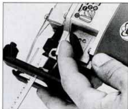
Side-mounted, 4-position orbital adjustment lever is common to Makita, Hitachi, Bosch, Freud and AEG tools tested.
