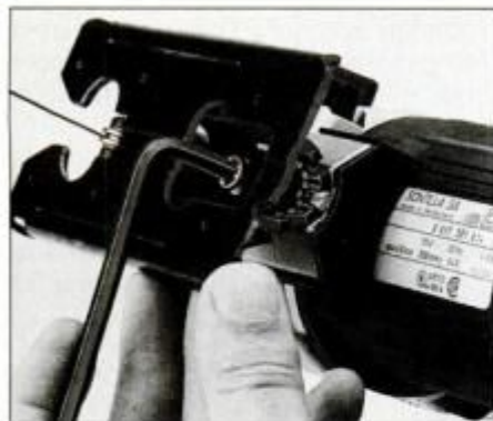
Loosening screw unlocks base to adjust for bevels. AEG, Freud and Bosch (shown) feature notches that engage at common angles.
