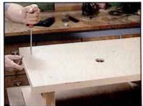
9 Countersink the screw holes in the top, and drive the screws through into the base side panels and hardwood cross supports.
