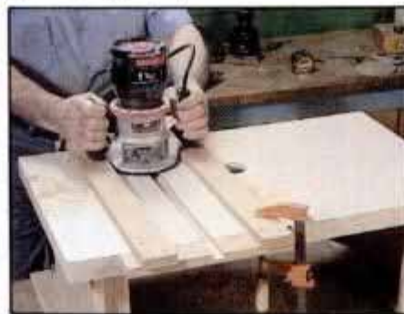
11 After excess laminate is trimmed off, cut the miter gauge slot in top. Guide the router between the two fences clamped to top.
