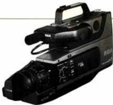
RCA's CC360 Pro-Edit Super VHS camcorder has built-in editing for home video movies.
