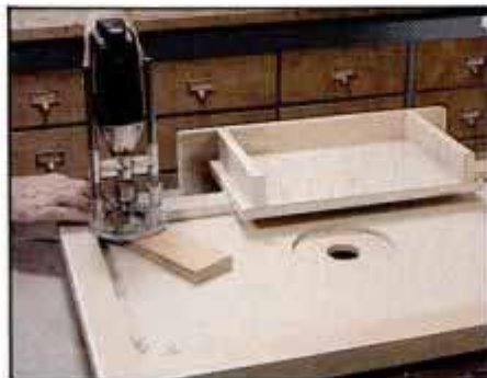
8 Bore screw holes in top from underneath. Gain clearance in the corners for the drill guide by supporting it on wood block.
