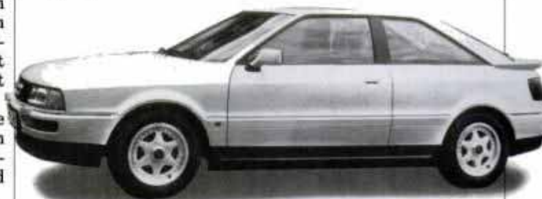
Audi Coupe Quattro's new Five gets four valves per cylinder.
