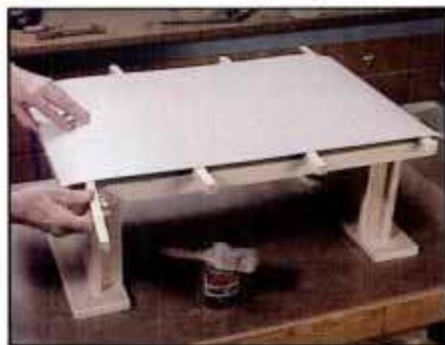
10 Move laminate into place, resting it on sticks. Starting at one end, remove one stick at a time until the sheet rests on top.
