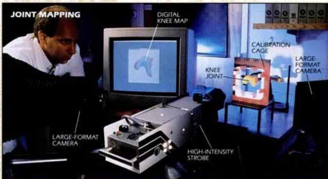
Strobe illuminates joint surface to make the photograph that will later be digitized into computer map.
