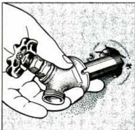
3 With water line cut, simply pull out old sillcock and length of pipe attached to it.
