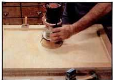
2 Cut the outline of the recess that will seat the router's base using a template, straight bit and accessory template guide.
