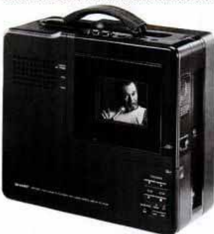
Video to go: Sharp's VC-V540U combines a VCR and 5-in. color screen, runs on AC/DC.
