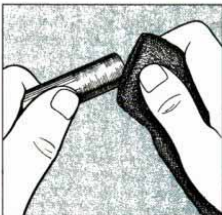
4 Prepare supply line for soldering by polishing away tarnish with steel wool.
