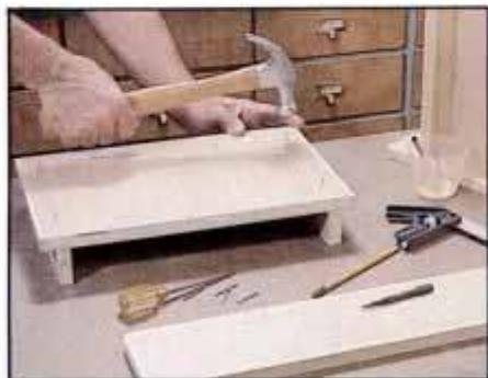
7 To construct base, glue and nail uprights to side panels, then attach feet. Trim the base edges with hardwood edge strips.
