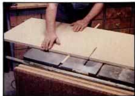
1 Begin router table's construction by ripping and crosscutting particleboard for top. Here, the miter gauge guides the cut.
