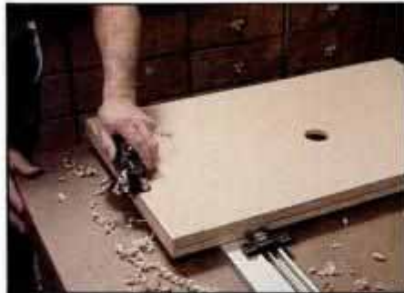
5 Cut wood edging strips slightly wider than thickness of top. Apply ends first, then trim flush using the block plane.
