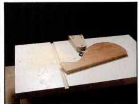
12 Bit safety shield is used during router operations with fence removed. For edge shaping, use router bit with ball-bearing pilot.
