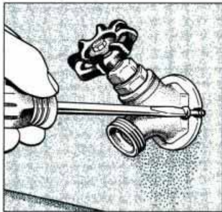
2 Remove the old sillcock from outside, by unscrewing two flange screws from siding.
