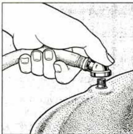
7 If tank is waterlogged, add air through snifter valve. Use compressed air, bicycle pump or drain tank completely and refill.
