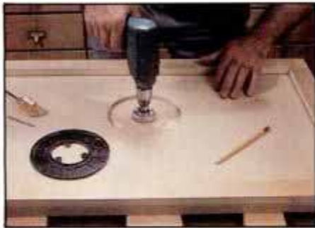
4 Bore through the center of recess for router bit clearance hole. Guide the 2-in. holesaw by boring the pilot hole first.
