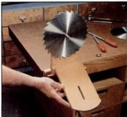
4 Secure shopmade clamp in bench vise. Clamp grips the blade close to the teeth to prevent chattering. This version is suitable for blades that are from 4 to 12 in. dia.
