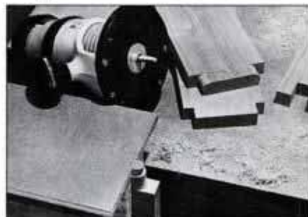
19 Use a template and a router with guide bushing to round edges of tenons to fit routed mortises. Or round tenons by hand.
