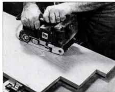
3 After the glue has dried, use a belt sander to smooth both sides of each top piece. Finish smoothing with orbital pad sander.
