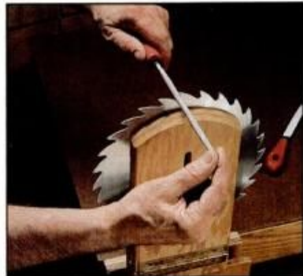
5 To deepen gullets, rotate the round file slightly as it is stroked forward. Do not rock the file and be sure to use the same number of smooth, even strokes per gullet.
