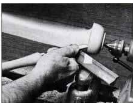
14 Turn inside concave area above foot on offset center. Use round-nose turning tool. Stay safely away from knee area.
