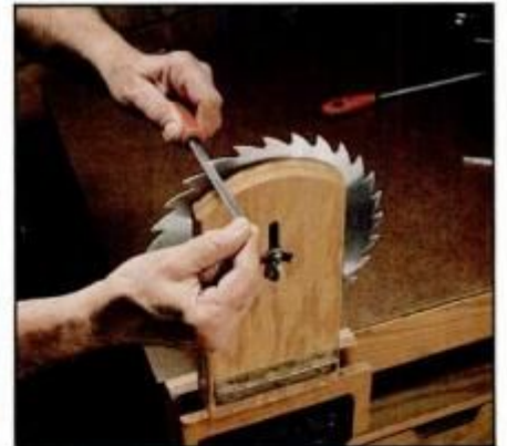
6 File the faces of rip teeth only when reshaping is required. A mill file with one round—or ground-off—edge facing down should be stroked straight across.
