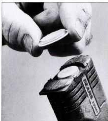
Slide adhesive-backed plastic disc onto heating element on the end of the electric applicator. Heat softens adhesive so the disc will bond to the wall's surface.
