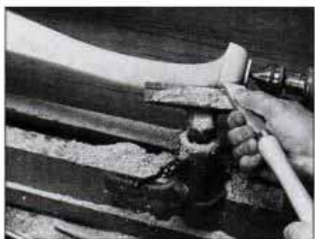
13 Mount leg in lathe on actual stock centers. Turn convex foot section to profile shown. Also, begin to round back of ankle.
