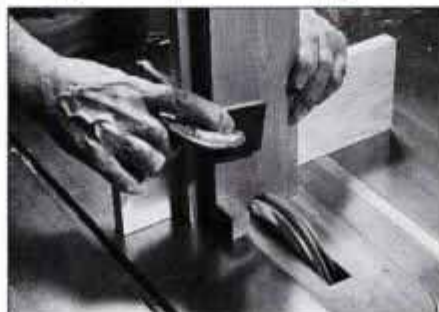
18 Shift aprons over the guide pin, clamp and cut. Third pass requires scrap block behind top apron to prevent tearout.
