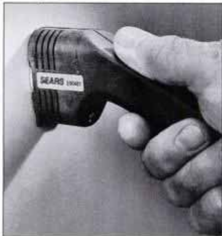
Position disc on wall surface and hold steadily in place for 5 to 15 seconds. Time varies depending on the type of wall surface.
