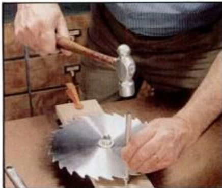
7 Set blade after shaping but before sharpening the teeth. Place tooth on beveled bolt-head anvil, then strike with drift punch to bend only the tip of the tooth.
