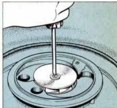
3 Remove screw that holds impeller in place. Then lift impeller off pump shaft and set it aside so it won't be damaged.
