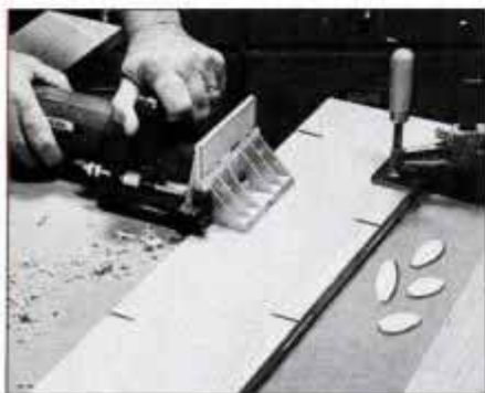
1 We used a plate joiner and No. 20 plates to join the tabletop pieces. Place plates 6 in. apart and locate to miss finished edge.
