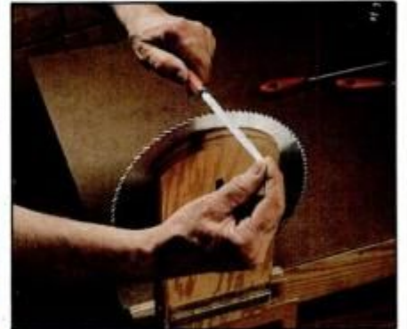
9 File crosscut teeth until one-half the jointing flat disappears. Then reverse the blade in clamp and file the alternate teeth to remove the remainder of each flat.
