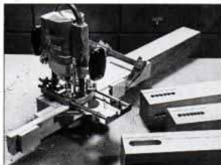
11 Rout mortises 13/16 in. deep. Preboring 1/2-in. holes makes job easier. Note two swinging legs have only one mortise each.
