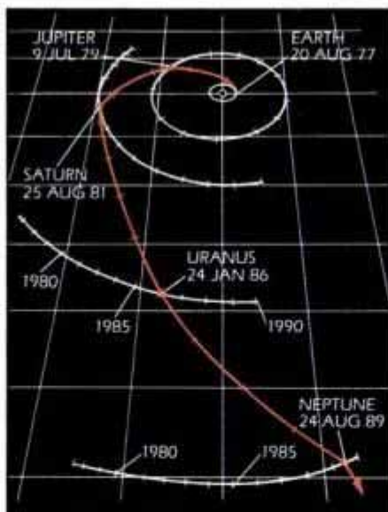
A unique alignment of the four outer planets has given Voyager 2 a crucial gravity assist on the journey to Neptune.
