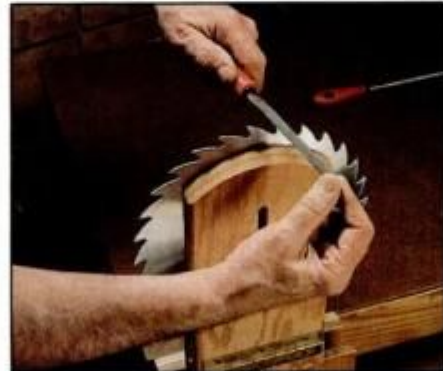
8 File the tops of rip saw teeth straight across until the flats resulting from jointing just vanish. The original top bevel clearance angle must be maintained.
