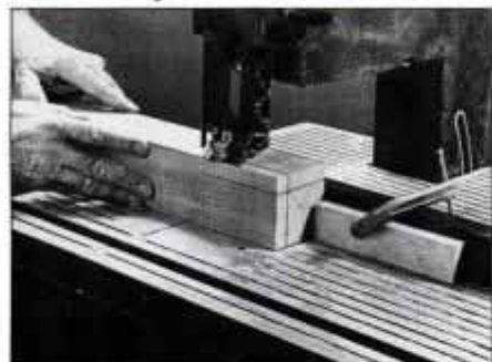
10 Band saw 4-in.-deep cuts, 1 in. from the surface of 3/4-in.-sq. leg blanks. These cuts form leg cheeks on adjacent sides.
