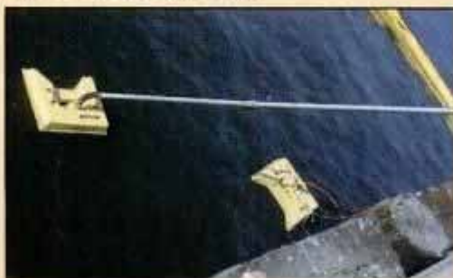
Surface skimmers pick up oil contained by surface booms and pump it to interim storage tank.
