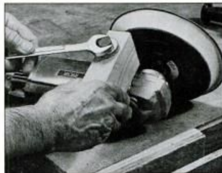
To convert a disc sander to a stationary tool, first remove side handle and install a short block of 2x4. Secure block with a long bolt.
