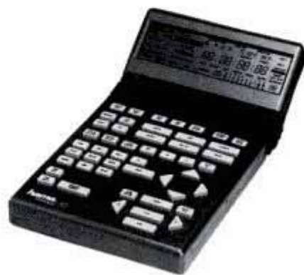
Hama's Video Cut 10 is a compact editing device for use with 8mm format camcorders.
