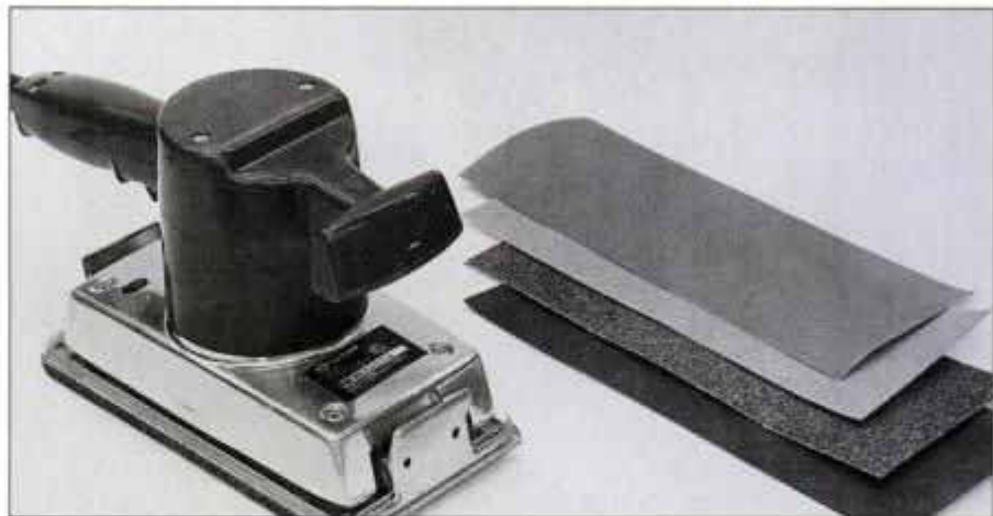
Orbital finishing sander accepts ½-sheet of standard 9 × 11-in. sandpaper. Shown, is a standard model, but sanders that come with dust collection bags are available, too.
