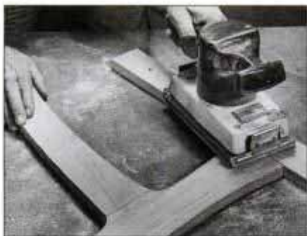
Circular motion of orbital sander makes it ideal for sanding across right-angle joints. There's little chance of cross-grain scratches.
