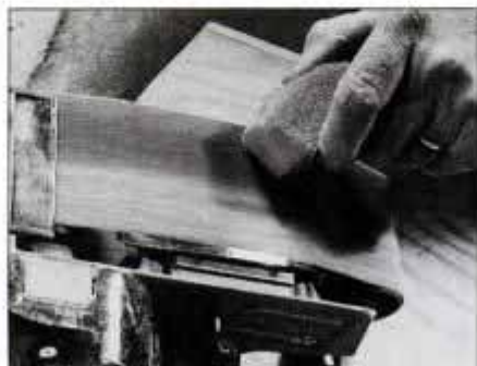
Extend life of abrasive belts by cleaning with a rubber cleaning stick. Hold stick against the running belt to remove wood dust.
