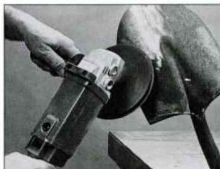
A disc sander is a quick and easy way to remove rust from metal surfaces. Always wear eye protection when using a disc sander.
