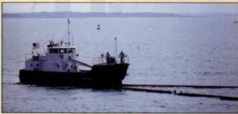
For widely dispersed spills, the skimmer Delbay can be fitted with floating booms (above) pulled by tender boats (not shown). The booms funnel oil toward an opening in Delbay's bow (left), where a conveyor belt carries it into the hold. An oil storage barge supplements the skimmer's capacity.
