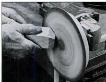
Clamp 2x4 block in a vise to hold sander upright. Use a foam-backed abrasive pad to provide a flat sanding surface.
