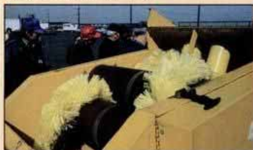
Wringing machine cleans a chain of oleophilic "pompoms", which can be reused.
