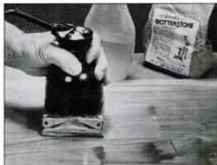
When fitted with an optional rubbing pad, palm sander can be used to polish a finished surface using rottenstone and water or oil.
