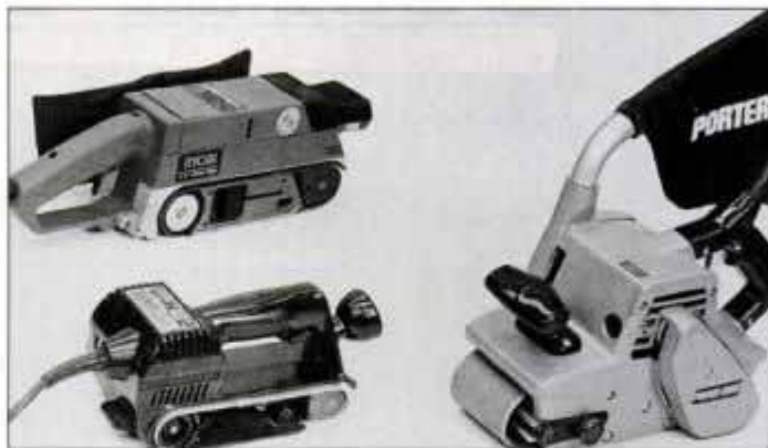
Three popular belt sanders: Ryobi 3 × 21-in. (upper left), Porter-Cable 3 × 24-in. (right), and 2½ × 16-in. Skill Sandcat (lower left).
