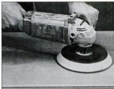
Thick foam-backed abrasive pad allows fine sanding with 120-grit or finer sandpaper. Note that unlike a disc, pad is flat on surface.
