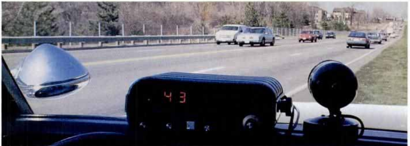
Traffic radar doesn't say which car is being clocked, it merely flashes a number. The radar operator must then try to determine which vehicle produced the reading.
