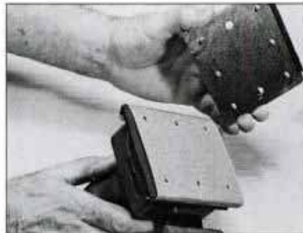
Dustless palm sander comes with spiked metal plate for punching holes in sandpaper. Wood dust is sucked through pad, into bag.
