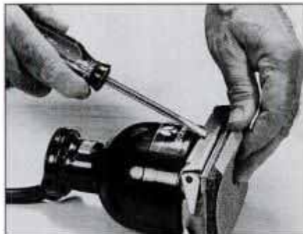
Paper clamps differ from sander to sander. Clamp on Porter-Cable sander is lifted with a slotted screwdriver to accept sandpaper.
