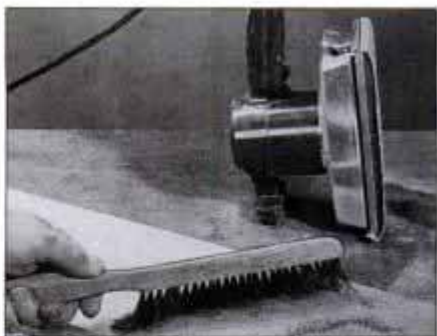
After switching to a finer-grit sandpaper, be sure to sweep the work surface clean. Abrasive-grit leftovers could scratch the surface.
