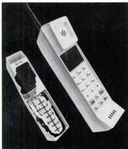
Cutaway of cellular phone (above) shows Duracell's hybrid battery. It uses flat zinc/air cells (below) to power phone in standby mode, recharge the NiCd battery used for transmitting and eliminate AC recharging.
