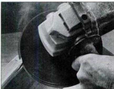
Be careful when maneuvering the sander. The edge of the disc can easily slice into the work, as shown. Keep the sander moving.
