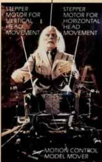
FACE CONTAINING RC SERVOS AND VACUUM BLADDERS
