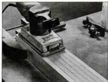
Gang sanding saves time when edge sanding. Two outside boards are scrap boards that prevent rounding inner workpieces.
