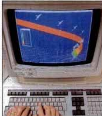
Ribbon's change in color shows increasing dynamic pressure on hypervelocity plane.
