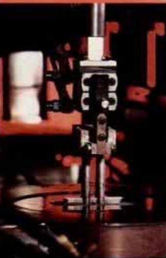
Robot arm inserts cold-pressed preform in PTM after heating in furnace.
