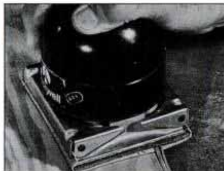
Advancing with the open side of sander can cause edge of abrasive paper to catch on splinters, as shown. Rotate sander 90°.
