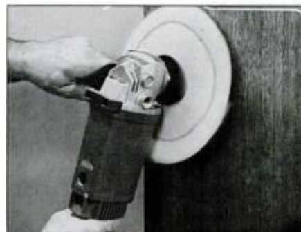
A lamb's wool bonnet is used for polishing jobs. Apply paste wax with a damp cloth, let dry and then buff with sander at low speed.
