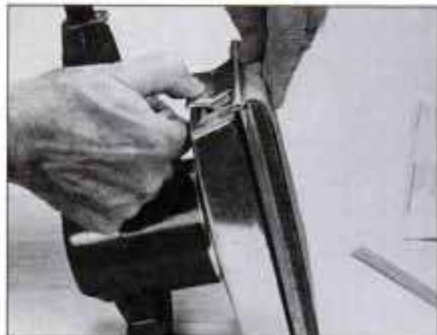
Spring-loaded clamps hold the sandpaper. Be sure to pull the paper tight. Loose, floppy paper reduces the sander's effectiveness.
