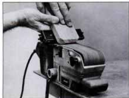
Flat-top sander can be clamped to workbench for use as a stationary tool. Ryobi offers this attachment for sanding bevels.
