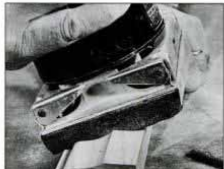
To sand contoured, irregular-shaped surfaces, install a thick, sponge rubber pad on sander. Soft pad contours to shape of work.
