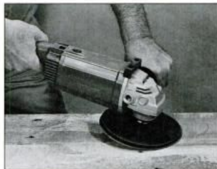
For rough sanding, like removing paint, press down so one-third of disc makes contact. Keep handle low to avoid gouging.
