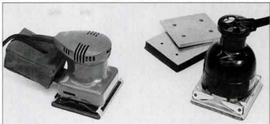
Orbital palm sanders accept a ¼-sheet of sandpaper and are designed for fine, finish sanding. Makita model (left) has dust bag. At right, is the popular Porter-Cable Speed-Bloc sander.
