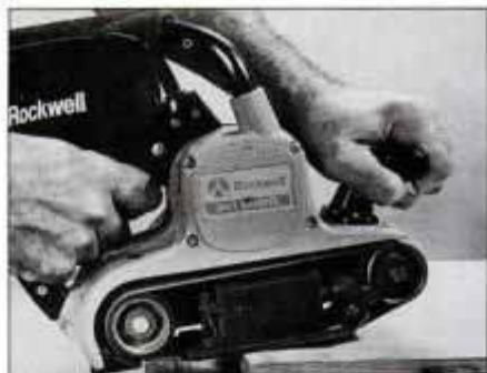
Avoid this common mistake. Keep the sander flat on the work. Tilting sander, as shown, will round over the board's end.
