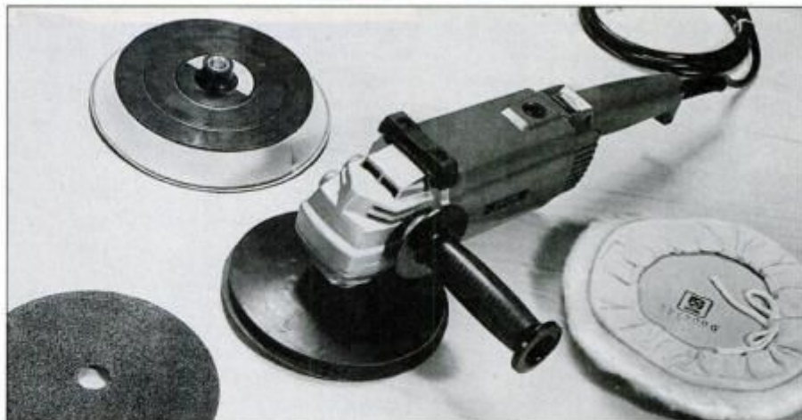
Disc sander is fitted with a rubber backing pad for use with abrasive disc (bottom left) or polishing bonnet (right). Thick foam rubber abrasive pad (upper left) permits full-face sanding.
