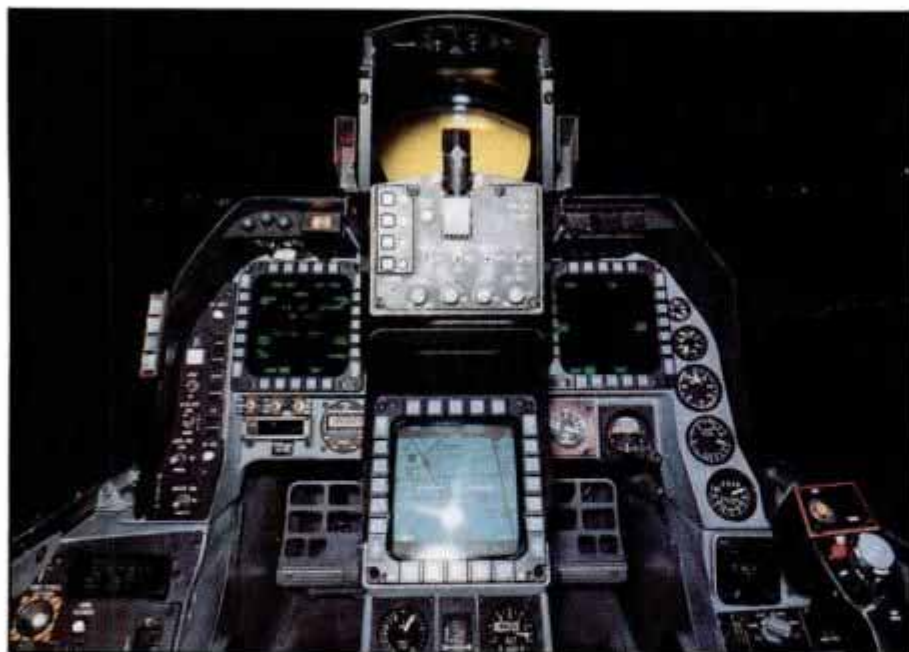
The F-16's front office includes wide-view heads-up display and multiple CRT screens that offer the pilot instant updates on navigation, engine performance or weapons status. The F-16's bubble canopy (left) affords almost 360° sightlines.
