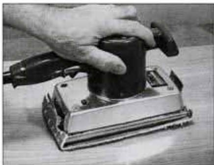
Cover sander's pad with a double layer of terry cloth and buff paste wax on furniture. Use a clean section of cloth for final buffing.
