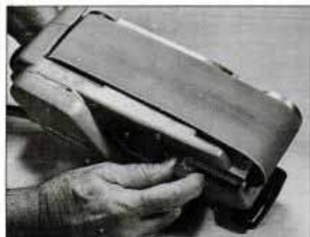
Most sanders have belt-tracking knob near the front roller. Turn the knob, while the sander is running, until the belt is centered.
