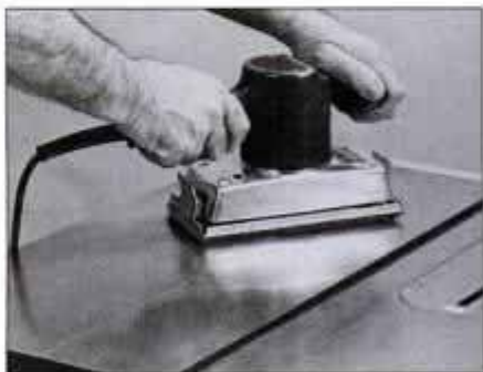
Polish metal with 600-grit silicone-carbide abrasive paper. To remove rust stains, apply mineral oil first, then polish the surface.
