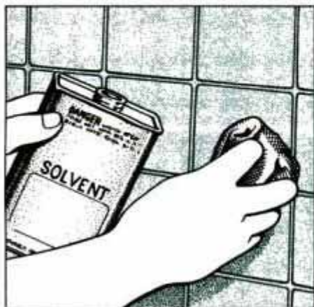
1 To install adhesive-backed holders on ceramic tile, first clean off all the residue from the surface using denatured alcohol.
