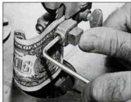
Use a dollar bill as a spacer when installing guide blocks. Slip bill on each side of blade. Push in block until it lightly touches the bill.
