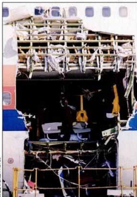
A crippled United Flight 811 rests safely on the Honolulu tarmac following the presumed inflight failure of its forward cargo door (right).
