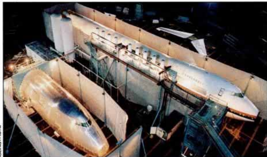
Flight-cycle testing at Boeing hopes to spot pressurization anomalies.
