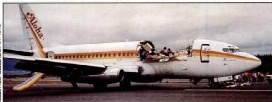
Prelude: The Aloha Boeing 737 on the ground in Maui after its midflight breakup.
