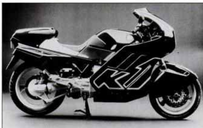
BMW's K1 (above) challenges Japanese superbikes with 16-valve head and 100 hp. Honda's Pacific Coast PC800 (below) is sheathed in ABS plastic and has liquid-cooled V-Twin, shaft drive.
