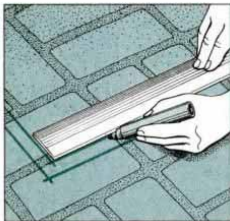
8 Use a water-soluble felt-tipped pen to mark cutting lines on flooring. Mark rough cutlines 1/2 in. outside finish cutlines.
