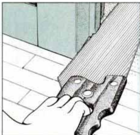
2 Where required, trim casing and doorstop with a sharp handsaw so new underlayment and flooring can fit in neatly.
