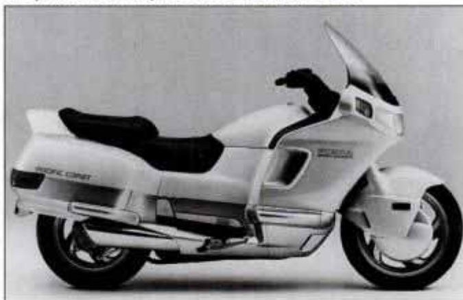
BMW's K1 (above) challenges Japanese superbikes with 16-valve head and 100 hp. Honda's Pacific Coast PC800 (below) is sheathed in ABS plastic and has liquid-cooled V-Twin, shaft drive.
