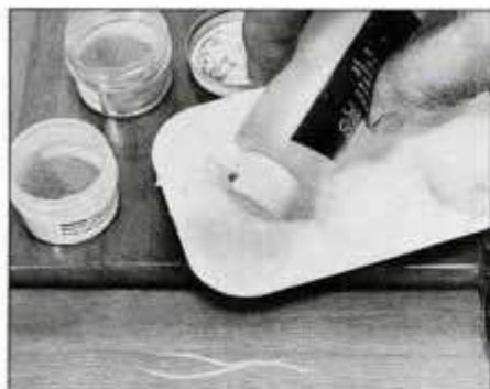
The first step is to add liquid mixer to a well in the plastic mixing tray. For most minor scratches, you'll need only a few drops.
