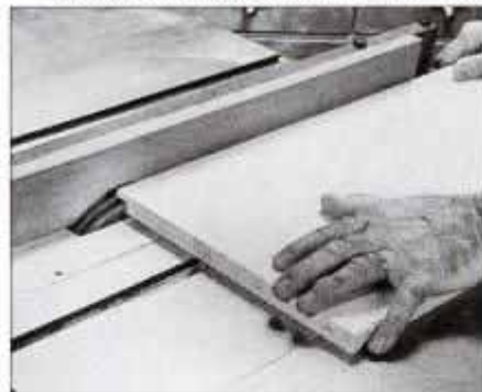
When cutting rabbets with a dado blade, attach an auxiliary wood fence to the rip fence. Note that blade is partially hidden by wood.
