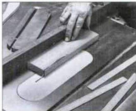
When ripping thin strips, replace standard table insert with a plywood one. Raise blade through plywood to form the narrow slot.
