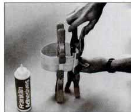
8 Once the veneer has dried, slip it off the mold, apply glue to overlapping section, and secure it with a few spring clamps.
