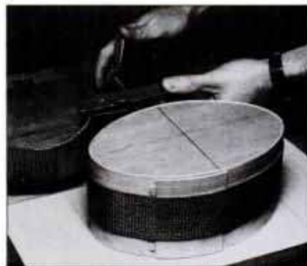
7 Secure wet veneer to plywood mold with a web or band clamp. Place scrap veneer over fingers to help prevent splitting.
