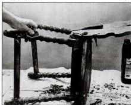
To remove the stripper and softened paint from turned legs and other irregular-shaped surfaces, scrub with a 3M stripping pad.
