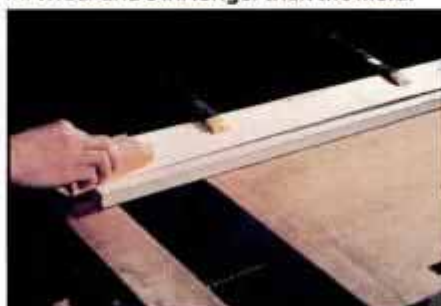
5 Use 100-grit sandpaper and a wood block to sand a taper on end of veneer.
