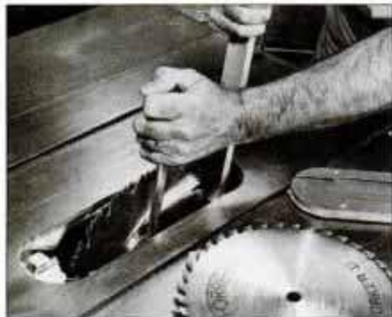
To change blades, first unplug the power cord. Then, use a wood stick to hold blade as you remove the arbor nut with a wrench.
