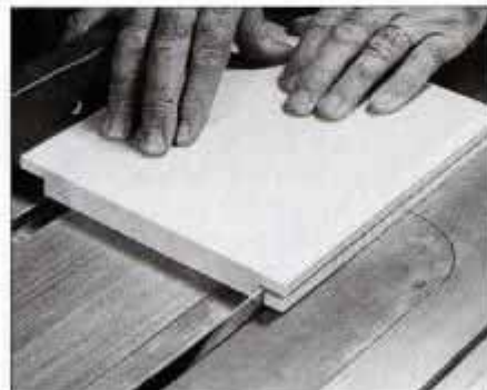
Readjust blade height and fence position for second cut. Pass work between blade and fence to prevent kickback of cutoff strip.
