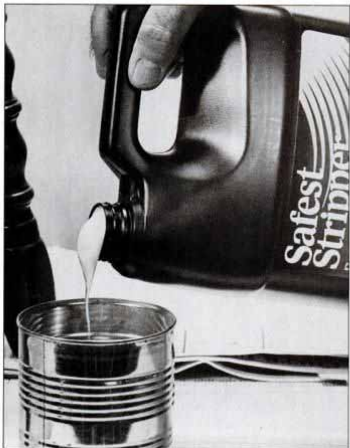
Paint and varnish remover is formulated as a slow-pour, semipaste. This pancake-batter consistency permits the stripper to adhere to vertical surfaces without running. Apply it from a clean metal can.
