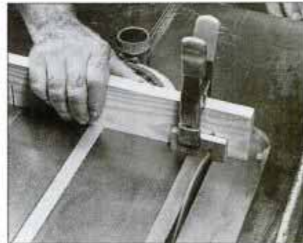
Never take chances when crosscutting small pieces. Use a spring clamp to hold work to miter gauge fence. Keep your fingers away.
