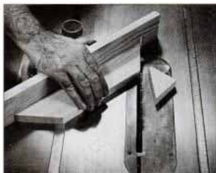
This shows cutting a 45° miter with miter gauge set in the closed position. Note wood fence attached to miter gauge for support.
