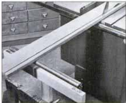
Long stock must be supported. Make a simple T-shaped frame with roller. Clamp frame to sawhorse so roller is even with saw table.
