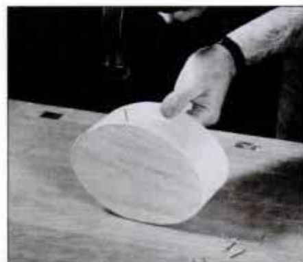
9 Bore 1/16-in.-dia. pilot holes to prevent splitting the veneer. Then, fasten pine box bottom with 1/2-in. brass escutcheon pins.
