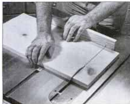
For crosscutting a wide board, one hand holds the work against the miter gauge fence while the other pushes forward.
