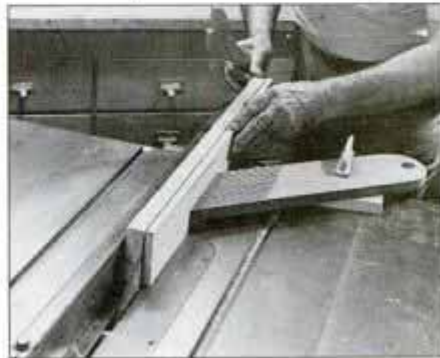
Here, a featherboard holds work for resawing—that is, cutting thick boards into thin ones. Cut featherboard on band saw.
