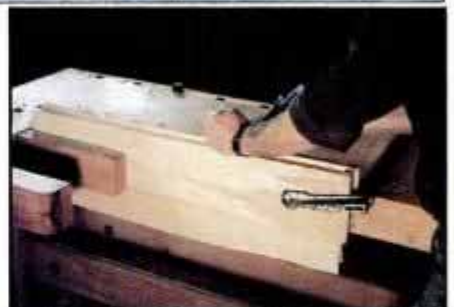
3 Clamp box-side veneers between 3/4-in.-thick boards. Allow uneven edge to protrude 3/8 in. Then, plane edges straight.
