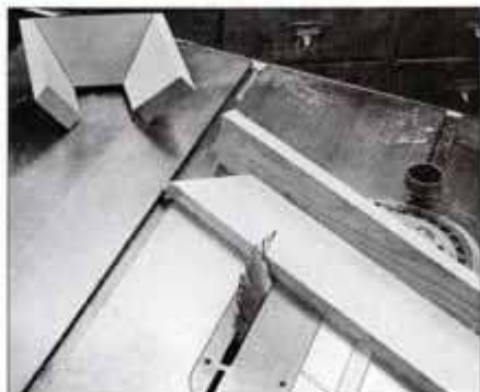
Here's the setup for a typical compound angle cut. Tilt the saw blade and angle miter gauge to create both a bevel and miter cut.
