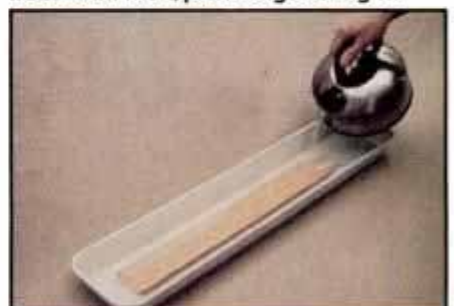
6 To soften veneer, place it in a long tray and soak it in boiling water for 4 minutes.
