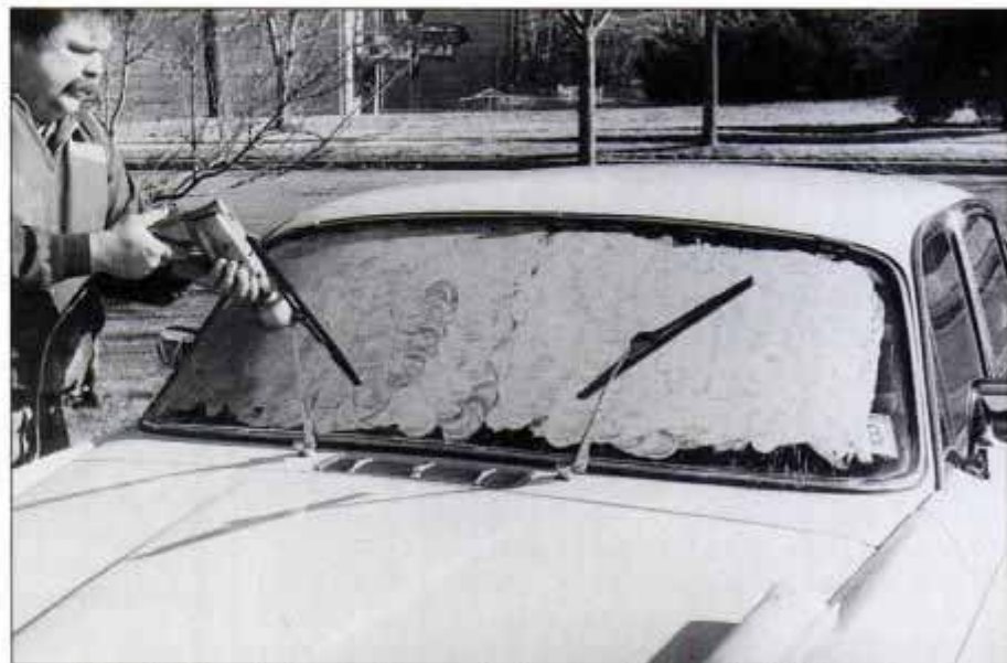
Felt polishing wheel and oxide powder slurry can buff out windshield scratches.
