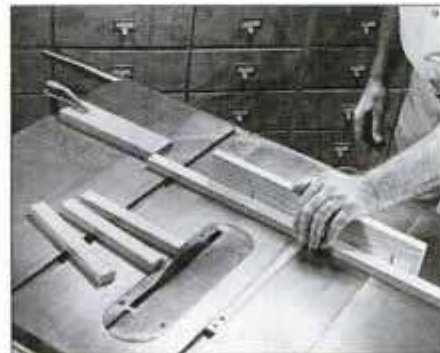
A stop block clamped to the saw table allows for identical repetitive cuts. Butt the work against block and advance the miter gauge.
