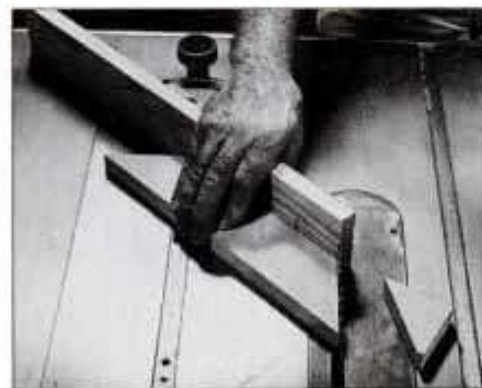
Here, miter gauge is in the open position and is set back from blade. When mitering a wide board, the miter gauge will be off saw table.
