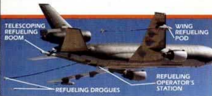
McDonnell Douglas KC-10 with all fueling hoses deployed.
