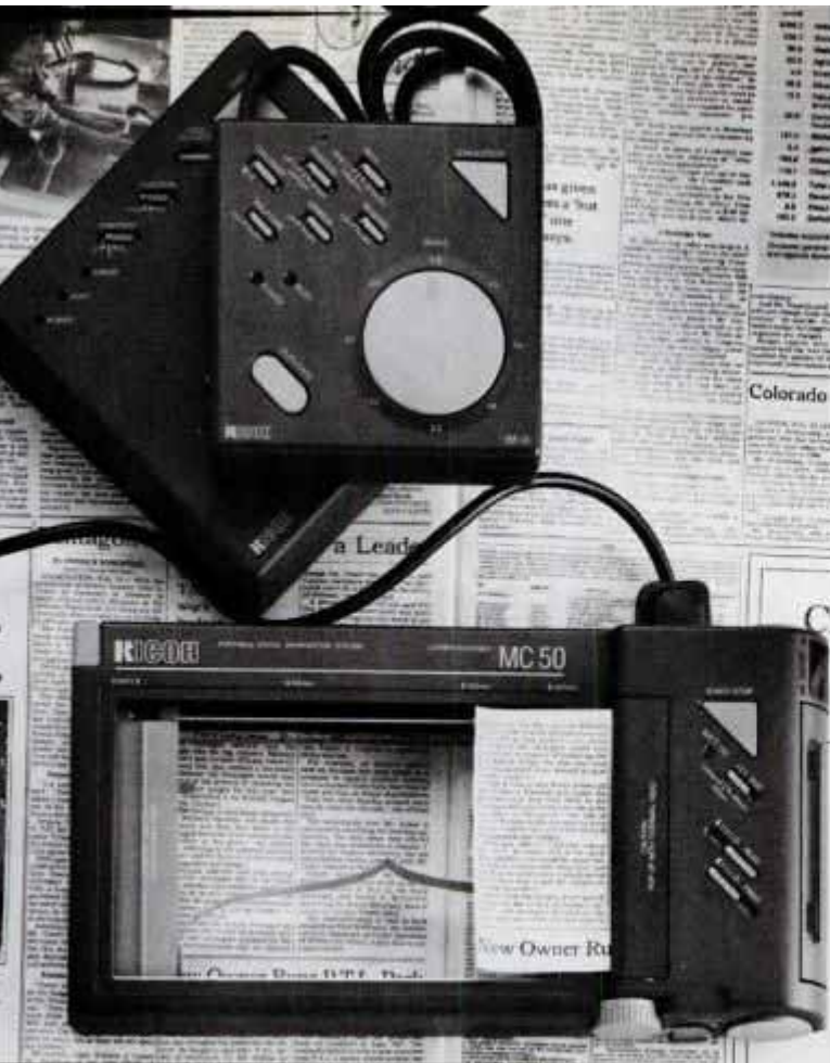
MC50 thermal copier is the scanning module of Ricoh's Portable Copier/Digitizer System. Other modules (top) enable system to fax documents or feed them to a computer.
