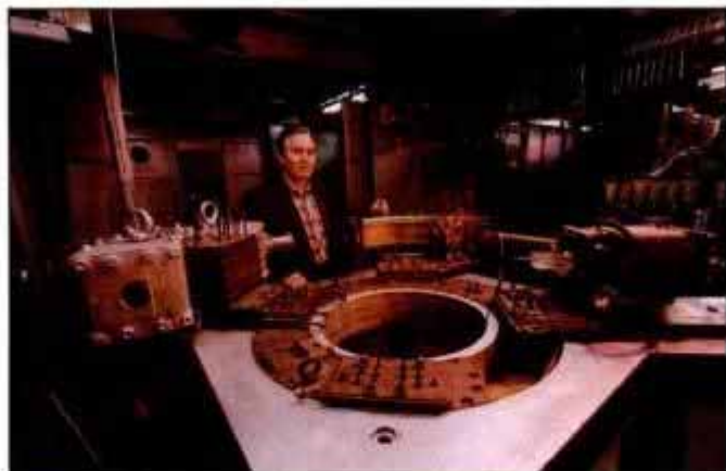
The Big Electron Beam [above] will be used to inject short-pulse electrons in the world's largest linear accelerator. Aside from high-energy particle experiments, Soviet researchers are studying industrial/medical uses of accelerator technology, including the 1.8-meter proton cancer therapy ring (below).
