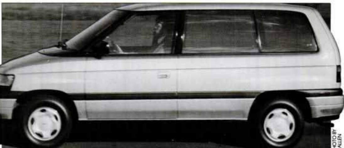
Mazda MPV: New multipurpose van that puts V6 power to the rear wheels and can tow 4300 pounds.
