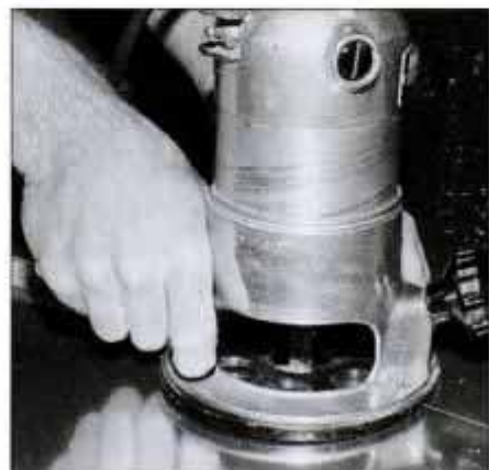
5 A router is the best tool for rough cutting laminate. Align cut mark on panel with edge of bench and cut with straight pilot bit.
