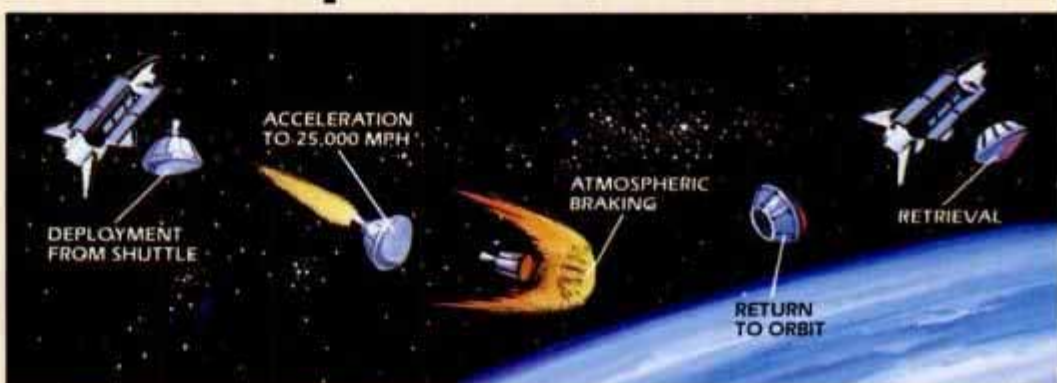
Aerobrake vehicle tests atmospheric deceleration.
