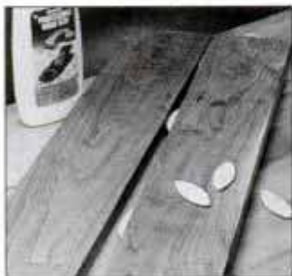
After cutting slots in workpieces, football-shaped biscuits join boards. Hardwood biscuits are made of compressed beech.
