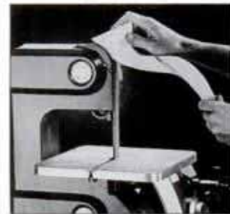
Sander has the upper wheel exposed so that it can be used for contour sanding. Apply light pressure to avoid clogging belt.
