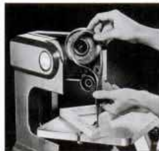
For internal sanding—smoothing inside a cutout—remove sanding belt from top wheel and pass through cutout in work.
