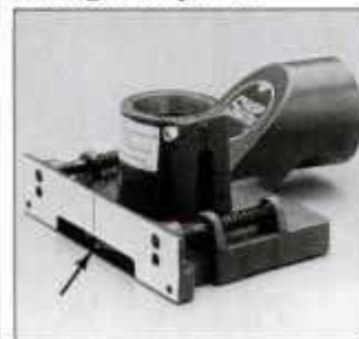
Here's the biscuit joiner removed from the Mark V tool. A 4-in.-dia. blade is concealed behind slot (arrow) in fence.
