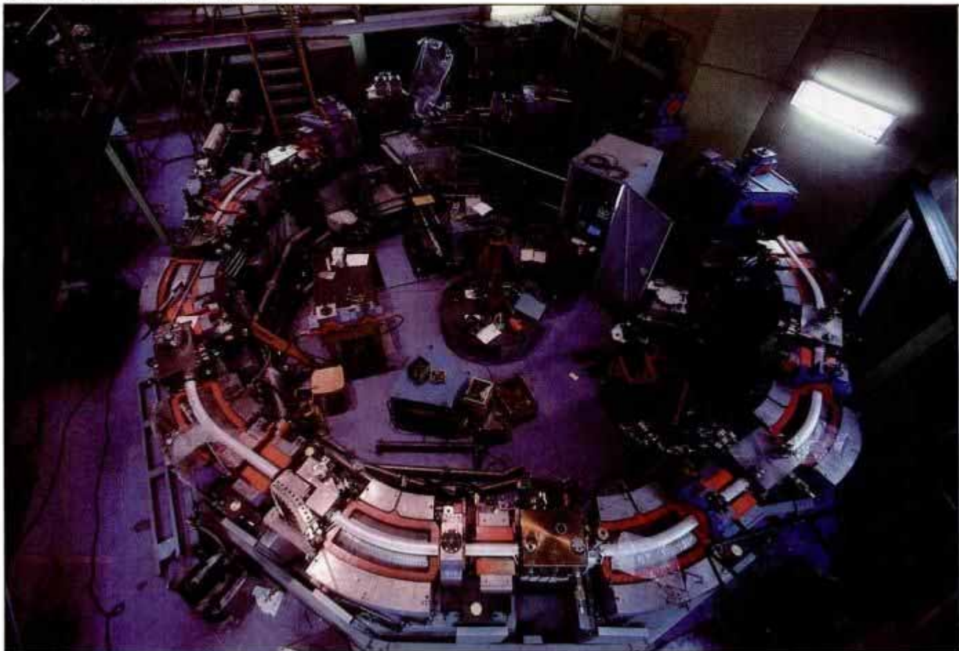
The Big Electron Beam [above] will be used to inject short-pulse electrons in the world's largest linear accelerator. Aside from high-energy particle experiments, Soviet researchers are studying industrial/medical uses of accelerator technology, including the 1.8-meter proton cancer therapy ring (below).
