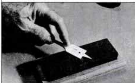
Any wire edge (burr) that results from sharpening, can be removed on a flat sharpening stone. Lay bit flat on stone and rub lightly.
