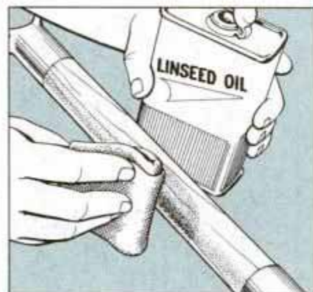
14 Using a cloth, rub boiled linseed oil into the handle to make the wood weather resistant. Repeat this treatment annually.
