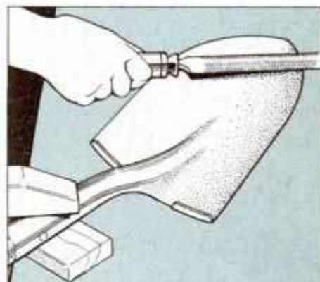
3 Clamp shovel to a bench, for sharpening. Start with double-cut file to reestablish bevel. Sharpen edge with a single-cut file.
