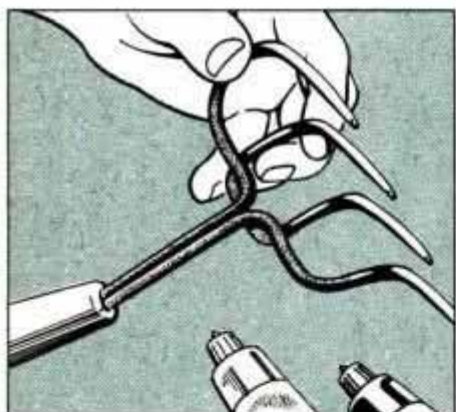
19 Secure the loose head of a cultivator by filling socket with epoxy adhesive. Five-minute epoxy is ideal for quick repairs.
