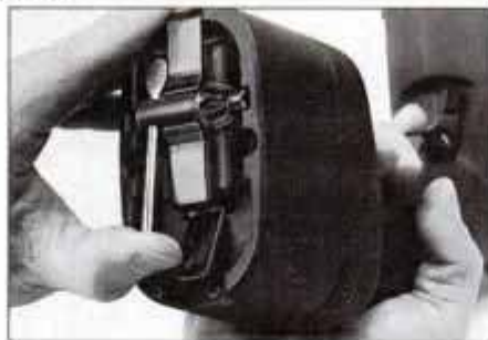
The chuck key for the Porter-Cable tool is held securely in the metal battery strap. It's easy to remove but more difficult to replace.
