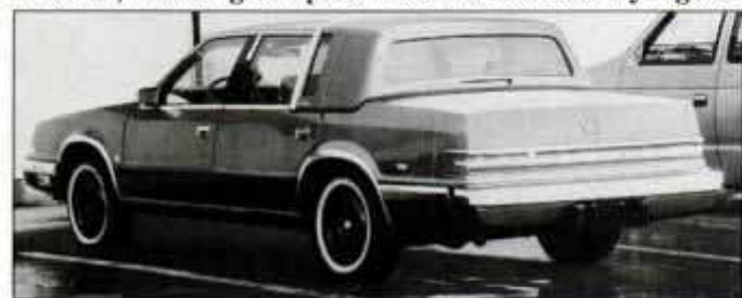
Chrysler Imperial rides on stretched New Yorker chassis.
