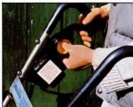
Motor has three speeds with switch conveniently located below throttle handle. Adjust speed based on soil conditions.
