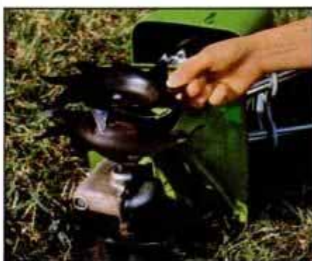
To remove a tine for maintenance or replacement, simply pull out the lock pin, then lift off the tine assembly from the driveshaft.
