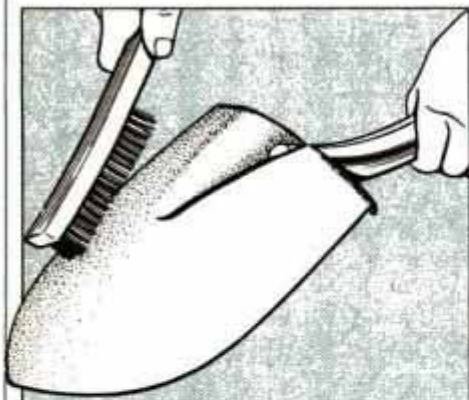
1 Extend the useful life of tools by removing rust immediately. Use a wire brush or steel wool to expose clean, bare metal.
