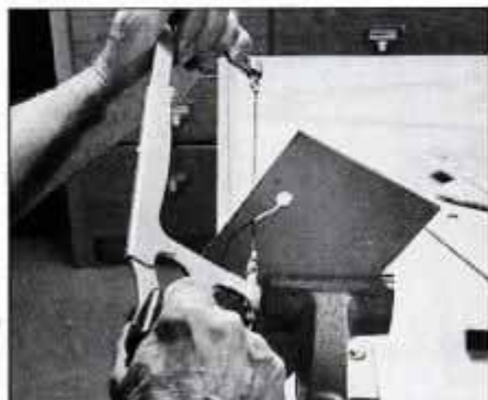
Rod saw is excellent for making irregular-shaped cuts in tile, glass, marble and hardened steel, as shown. Fits standard hacksaw.
