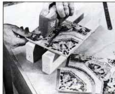
Grit-Edge sabre saw blades cut ceramic tile easily for perfect-fit installations. Blades cut most masonry and abrasive materials.
