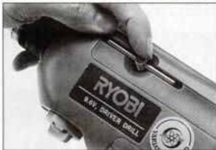
The socket for the Ryobi chuck key makes key removal difficult. The Bosch drill uses a similar design but removal is easier.
