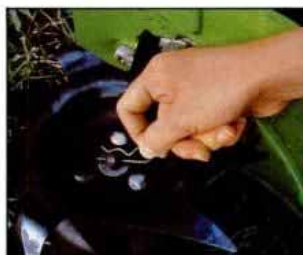
Tiller comes equipped with two steel tine assemblies. Tines are attached to a horizontally aligned driveshaft with simple lock pins.
