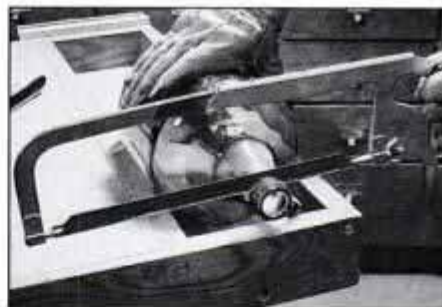
Cutting glass, in this case a wine jug, would be impossible with a conventional blade. Grit-Edge blade cuts without slipping.
