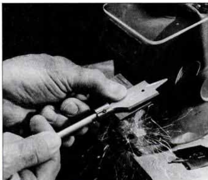
Sharpen spade bits on bench grinder quickly and accurately. Adjust angle of tool rest to match original bevel angle of bit's cutting edges.
