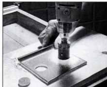
To cut round holes in tile, slate, brick, clay pipe and steel, try a Grit-Edge hole saw. Available in sizes from 3/4 in. to 4 1/2 in. dia.
