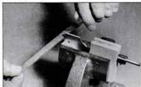
Use a file to sharpen bit's starting point, too. Hold file at same angle as point's original bevel. Make light strokes on each side.
