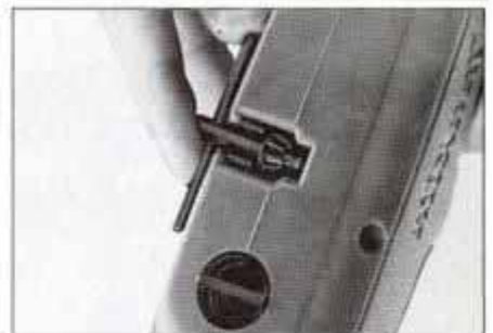
Makita and Milwaukee both feature a clip that holds the chuck key shank securely. Removal and replacement are simple.
