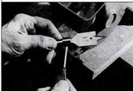
Attach a depth-stop collar to bit's shank. Collar butts against tool rest to control amount of metal removed from the cutting edges.
