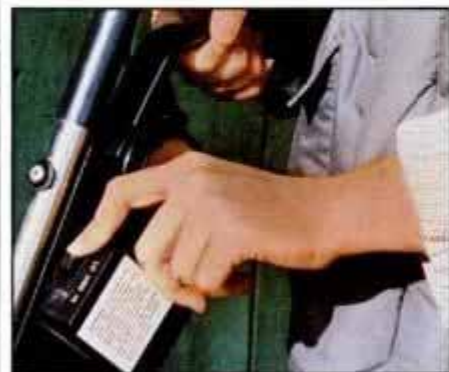
To engage throttle, push in yellow SAFETY SWITCH button and pull back on throttle handle. Release handle and tiller stops.
