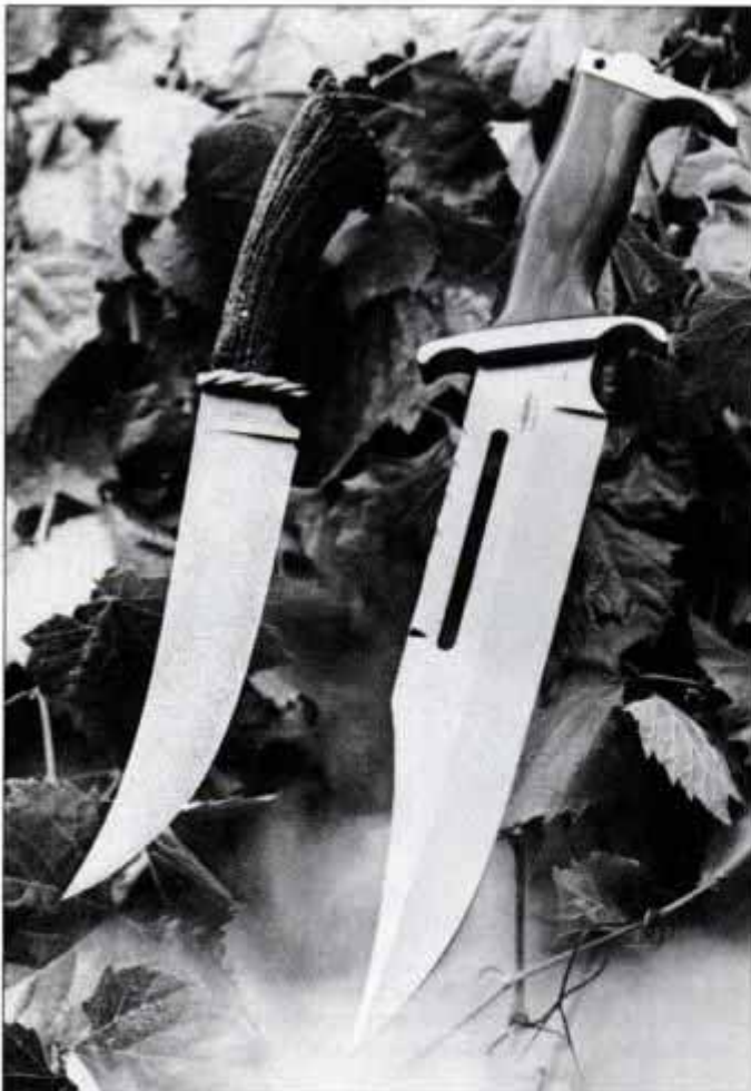
Rambo III (right) has a heavy 18-in. tool-steel blade, while the Persian Bowie has an ornate carbon-steel blade known as Damascus steel.
