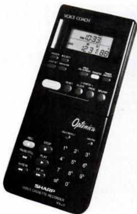
Sharp's Voice Coach remote control gives you vocal instructions for VCR programming.
