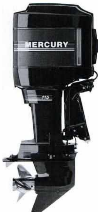
Merc equipped the 115 with a new smart carburetion system, Concept 2+2, which restricts fuel flow to 2 cylinders at low rpm.
