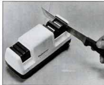
Stage three: final honing for a razor's edge. Make a few slow strokes over disc followed by a few fast strokes to polish edge.
