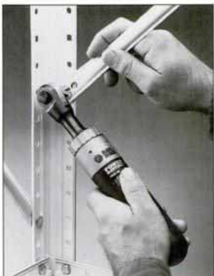
Touch of a button spins off nuts quickly. Power Ratchet is useful in tight spots where there's little room to swing the handle.
