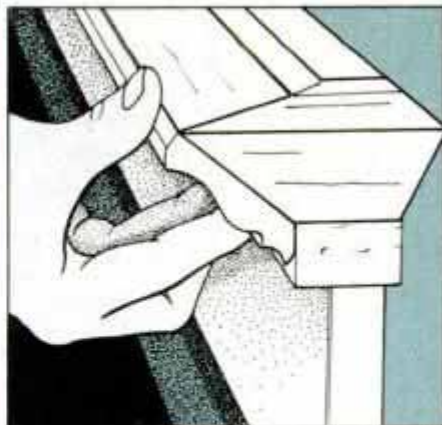
15 With one end of crown molding cut, hold in place and mark opposite end for trimming. Nail with 4d finishing nails.
