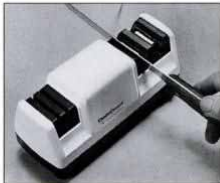
Stage two: sharpening slots. Magnets hold knife at the correct angle. Lift the handle at end of stroke to sharpen the blade tip.
