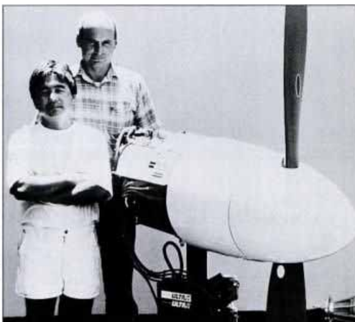
Aero rotary, with builders Ryusuki Oku and Jim Mederer. Engine exposed (right) shows components in 18-in.-dia. package.
