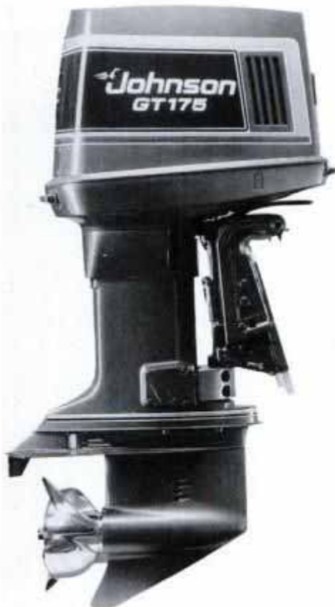
The Johnson GT 175 is a dedicated bass motor, with fuel and oil injection, QuikStart and S.L.O.W.
