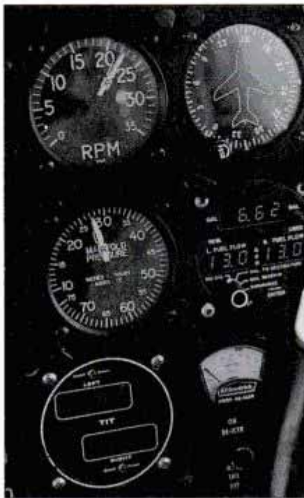
Digital gauge at bottom shows turbocharger inlet temperature for both engines. One mid-right shows fuel burn for each engine of 13 gph, and Loran-based mpg of 6.62.
