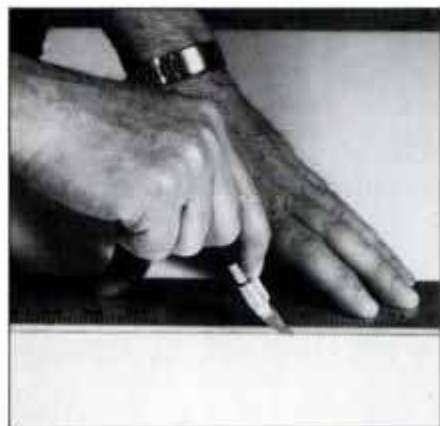
1 Trim mat board to size with a knife and straightedge held by spring clamps. Cut \frac{1}{8} in. less than inside frame size.
