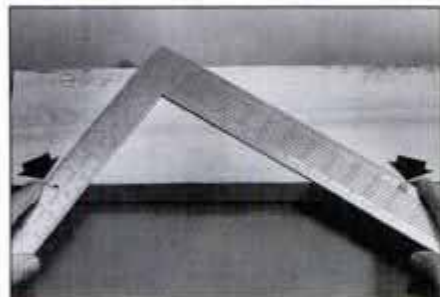
4 To establish plumb cut at top of rafter, align 8-in. mark on tongue and 12-in. mark on body with same edge of rafter board.
