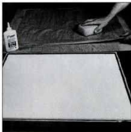
7 Moisten kraft paper, run thin bead of glue on rear edge of frame, then flip over frame and press down onto paper.
