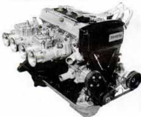
Toyota's 16-valve twin-cam 1.6-liter Four is the new power in Formula Atlantic.
