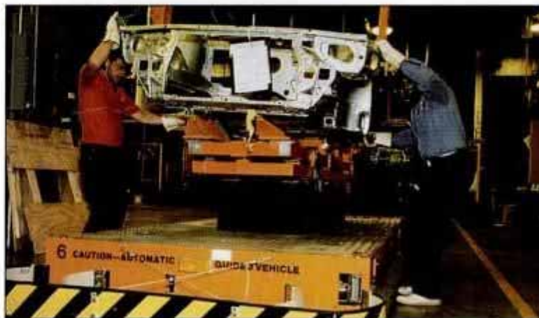
Reattas ride AGVs several times during assembly.
