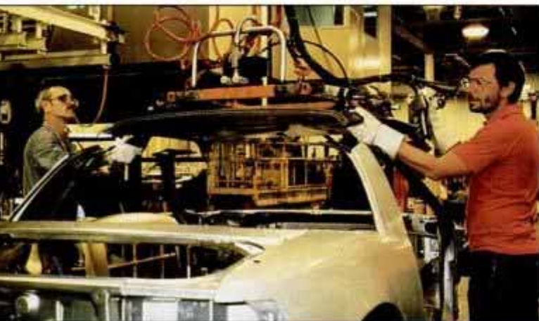
Roof panel is held up by suction until lowered into place.
