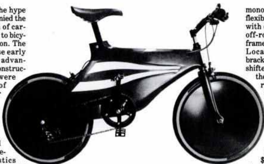
Carbon-fiber monocoque frame from SSDG is strong, aero smart.
