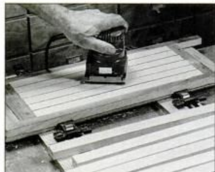
4 Place side frame pieces on flat board and clamp for gang sanding. Wood strips between stock and clamps protect stock.
