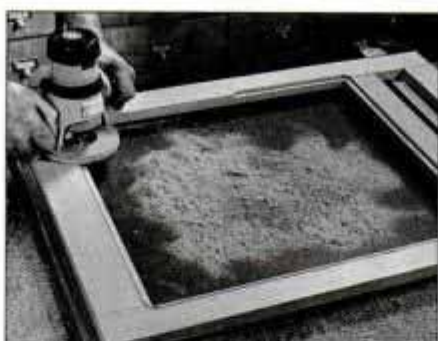
12 After seat frame is assembled, use a 3/8-in. rabbeting bit to rout the 1/4-in.-deep rabbet that holds the plywood seat.
