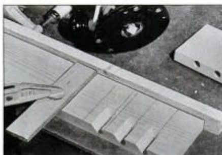
9 V-groove bit routs slope on forward edge of slots. Clamp strip squarely to guide router. Strip at edge limits router travel.
