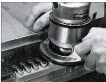
Template allows router to cut tricky half-blind dovetail joints. Router is equipped with guide bushing and dovetail bit.
