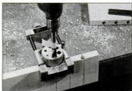
8 The angled slots are started by boring ½-in.-dia. holes near face of arm stock. Use a brad-point drill bit for the best results.
