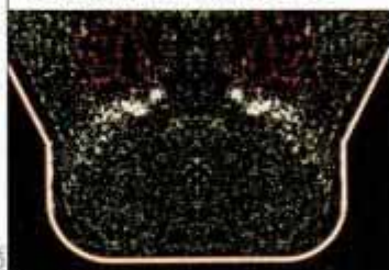
Ignition as piston nears top.
