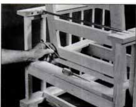
15 Secure hinges to back first. Then, insert rod and place back in position. Carefully mark hinge screw locations on seat frame.
