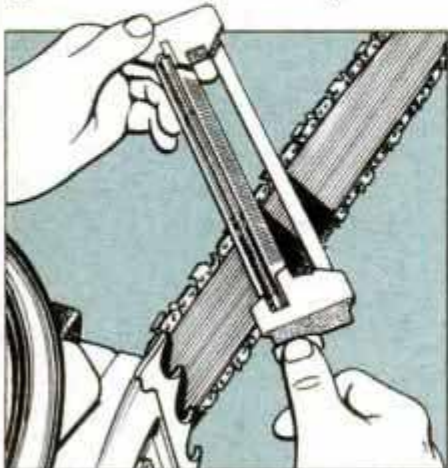
12 Reinstall the bar, chain, plate and housing, then tighten chain. Sharpen teeth with a combination file guide.
