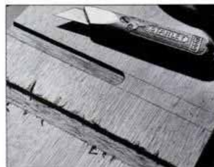
Cross-grain routing can splinter the veneer of some plywood. To prevent this, scribe the cut's borders with a knife before routing.
