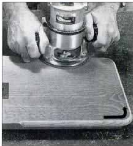
For best control and safest working conditions, advance router against rotation of bit. This means counterclockwise, as shown.
