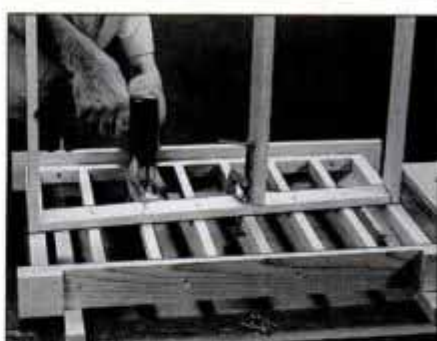
13 Clamp seat box frame to side and bore and countersink pilot holes. Holes at each end are bored at an angle to reach frame.
