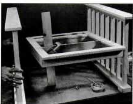
14 Use scrap stock clamped to box frame for supporting seat assembly when aligning other side. Secure with screws.
