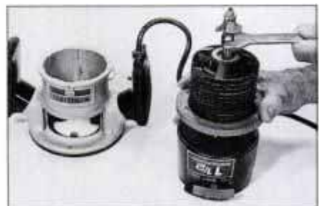
This Sears router has two convenient features: a stand-up, flat-top housing and a shaft-lock button for 1-wrench bit changes.
