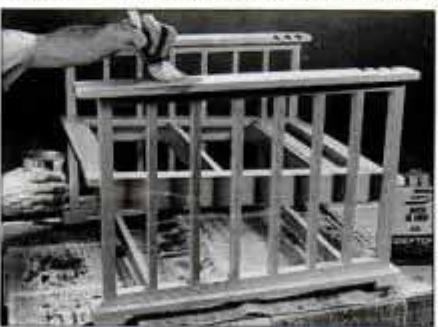
16 Two coats of Danish Oil Finish are applied for a clear durable finish. For extra protection, apply a last coat of varnish.
