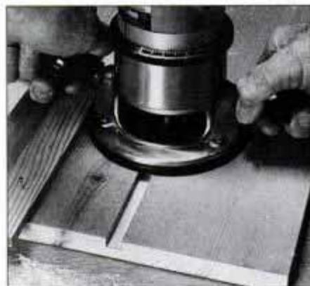
Guide router against straightedged board that's nailed to workpiece. Allow guide to overhang work to support router at start.
