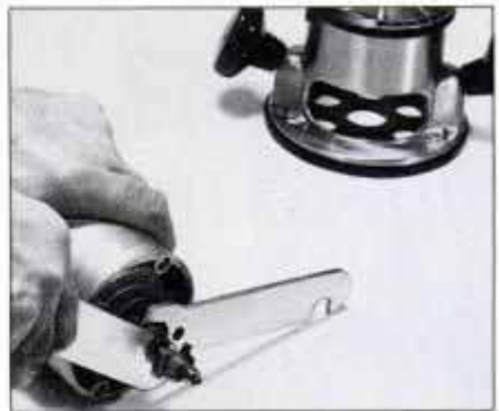
Some routers require two wrenches for bit changes. Place one wrench on the shaft and tighten chuck with the other wrench.
