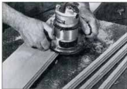
Here's a safe, easy way to rout decorative moldings. Shape the edge of a wide board and then rip the narrow molding from it.
