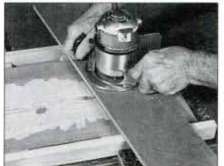
This simple setup turns a router into a surface planer. Router is attached to board that spans the workpiece on two wood rails.
