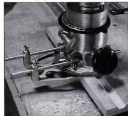
Edge guide accessory mounts on two steel rods that clamp to the router's base. Guide rides against work's edge to control cutter.
