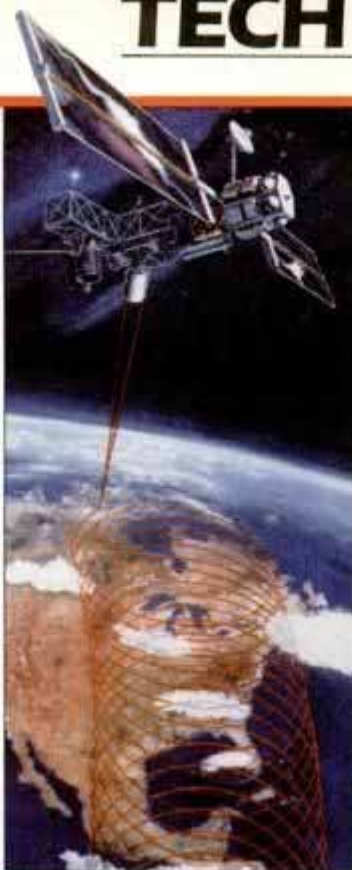
Lidar uses circular tracking pattern to obtain wind data from ground up to 40,000 ft.
