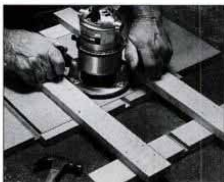
Clamp or tack-nail the jig and workpiece to the bench and make the first pass. Scrap strip is in place to prevent splintering as bit exits.
