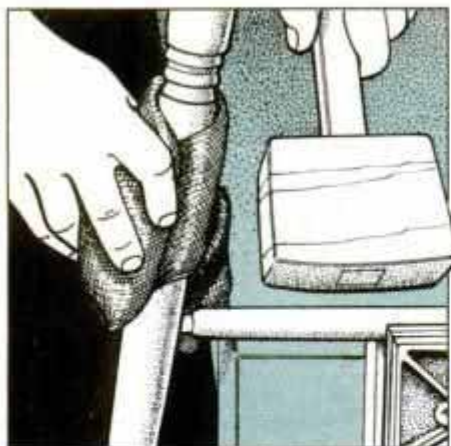
2 If joint is loose but won't easily come apart, place rung in vise and knock joint apart. Cloth protects leg from marring.
