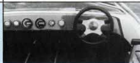
Instruments are angled to driver and easy to read, but throttle is tight against seat.
