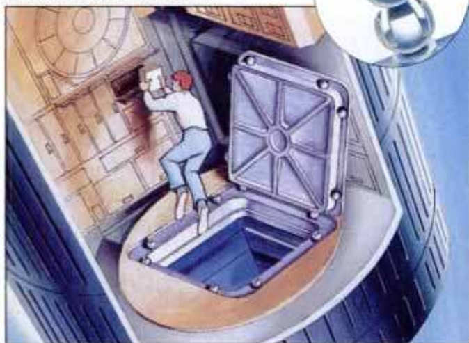
Four-way door, for Space Shuttle, opens regardless of orientation.
