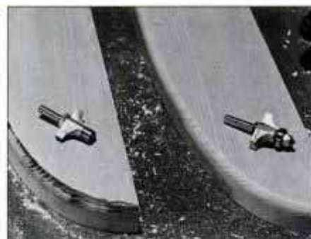
A dull bit (left) will burn the work and put undue strain on the router's motor. Carbide-tipped bit (right) stays sharper longer.
