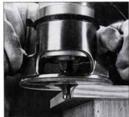
For precise control of edge shaping, use a ball-bearing piloted bit. Bearing rolls along uncut portion of edge to control the cutter.
