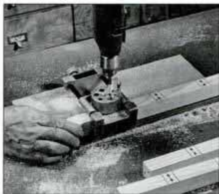
3 Align doweling jig at each spindle location and bore \frac{1}{4} -in.-dia. \times \frac{1}{16} -in.-deep holes. Tape on bit indicates boring depth.
