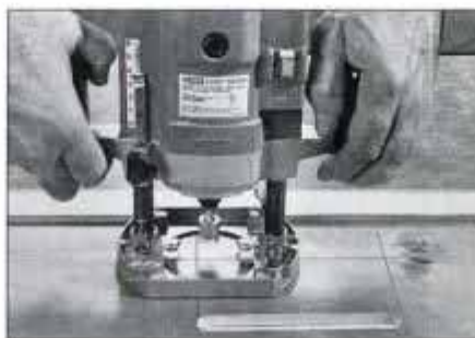
Plunge routers are especially useful for cutting stopped dados and slots, as shown. Router is mounted on a spring-loaded base.
