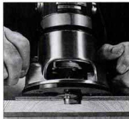
Guide bushing protrudes from subbase and rides against ¼-in. plywood template. Bit extends below bushing to shape the work.
