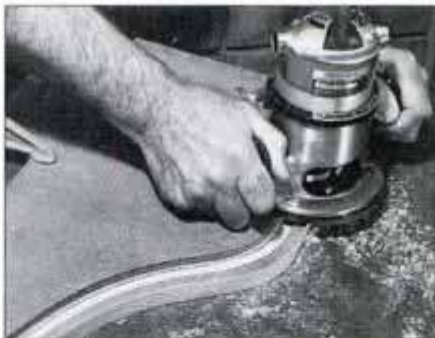
Guide bushing rides along a hardboard template to cut a groove for rolltop desk. Another tough job made easy with a router.
