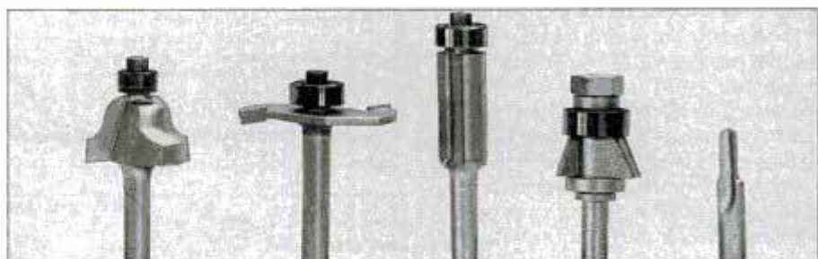
First four bits shown above have ball-bearing pilots. They are: Roman ogee, slotting, flush trimming bit and bevel trimming bit. The last bit shown is a high-speed steel veining bit.
