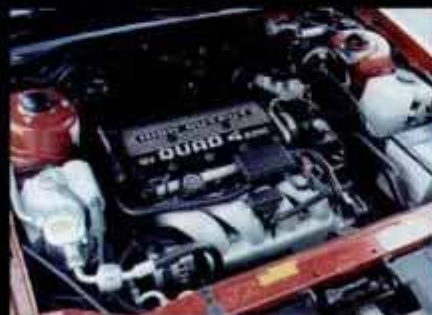
Deck spoiler distinguishes H.O. Calais. New cylinder head helps bump hp to 185.
