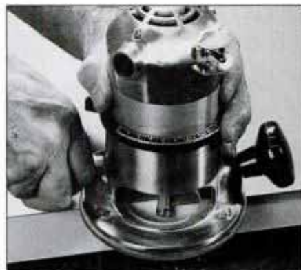
To trim overhanging plastic laminate, use a carbide-tipped flush-trimming bit. Be sure to keep the ball-bearing clean and lubricated.
