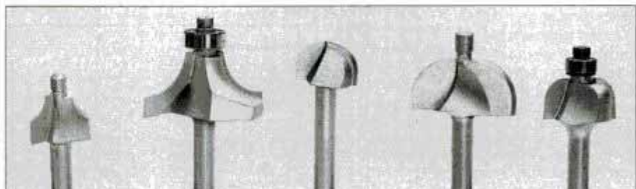
This set of bits includes (left to right): solid piloted beading bit, rounding over with ball-bearing pilot, core box and two cove bits. One cove has a solid pilot, the other a ball-bearing pilot.
