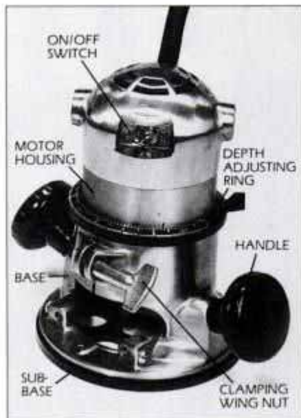
Here's a good, general-purpose router: The Porter-Cable model No. 100. Wingnut locks the base on motor to set the depth of cut.
