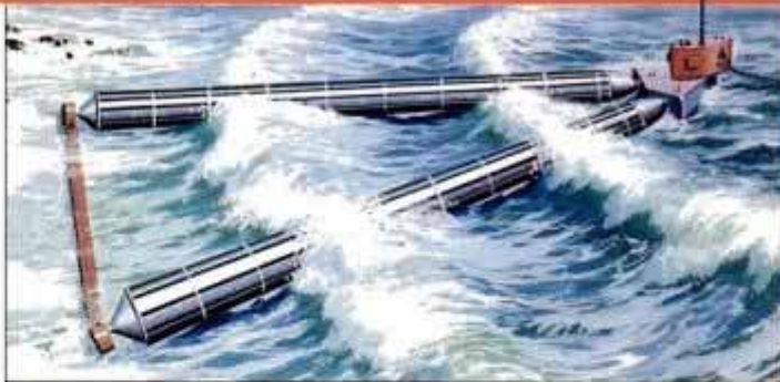
Booms rotate as waves move along axis.
