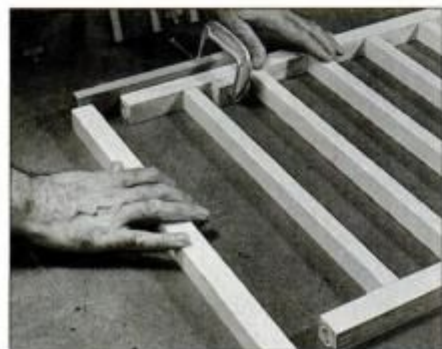
6 Use dowel centers for locating dowel holes in vertical frame pieces. Stock clamped to frame ensures alignment.
