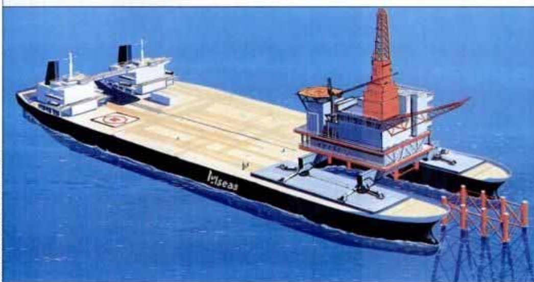
Rig straddles bows, ready for deployment on support platform, even in inclement weather.
