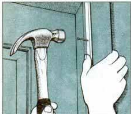
1 If the door opening is a little too wide for the door, fasten a thin wood strip to the inside of the door jamb with finishing nails.
