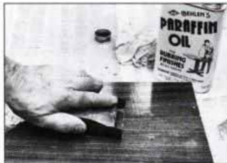
Paraffin oil is a popular lubricant for sanding, especially when working on shellac.
