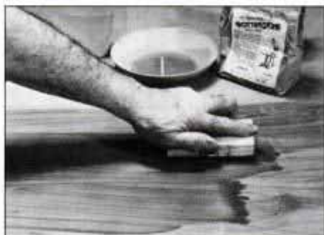
Polish finish with a wood block that has a piece of short-nap carpeting glued to it.
