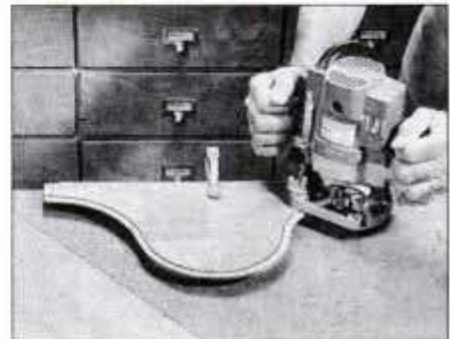
3 Rout a 1/8-in.-deep rabbet into the curved, inside edge of the front and back. Use a ball-bearing piloted 3/8-in. rabbeting bit.
