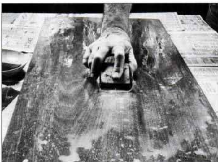
Use special waterproof abrasive paper to sand between coats of a finish. As a lubricant, use water, paraffin oil or mineral oil.
