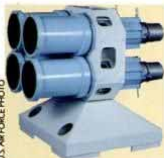
Four clustered telescopes have 16 times the resolution.
