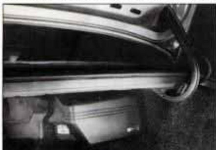
Ford/JBL subwoofer gets punch from its 10-liter enclosure, concealed in trunk.
