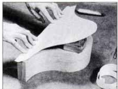
9 Remove backing on edge of veneer. Prop up veneer with a tape measure, align it exactly and peel off remainder of backing.
