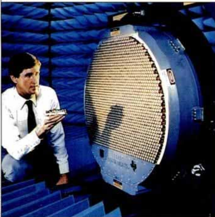
Solid-state phased-array radar aperture is tested in anechoic chamber. Aperture combines transmitter and receiver functions.
