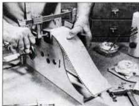
5 Secure the top between the front and back with several short bar clamps. Be sure that the top fits tightly into the rabbet joint.
