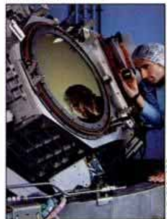
Zinc selenide viewing port of LWIR sensor.
