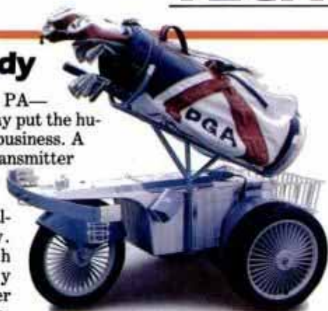
Rear-wheel-driven caddy follows short-wave radio transmitter on golfer's belt.
