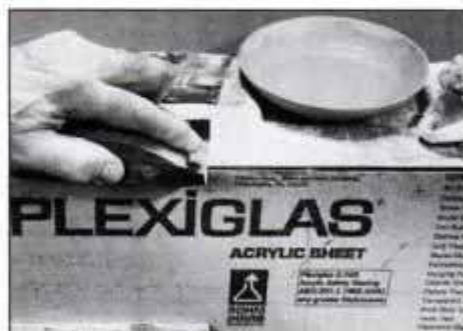
Form a supersmooth, highly polished edge on acrylic with wet abrasive paper.
