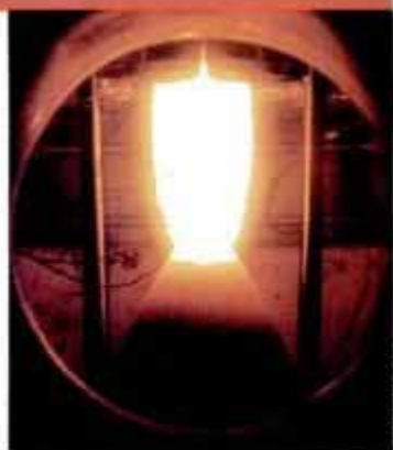
Red-hot rhenium chamber torture-tested in vacuum chamber.
