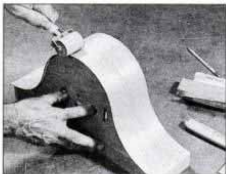
8 To ensure a strong bond, press down the veneer with a veneer roller. Then, trim off the excess veneer with a sharp utility knife.
