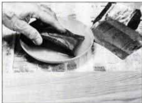
Use a rubber sanding block and rinse off the paper frequently in the lubricant.
