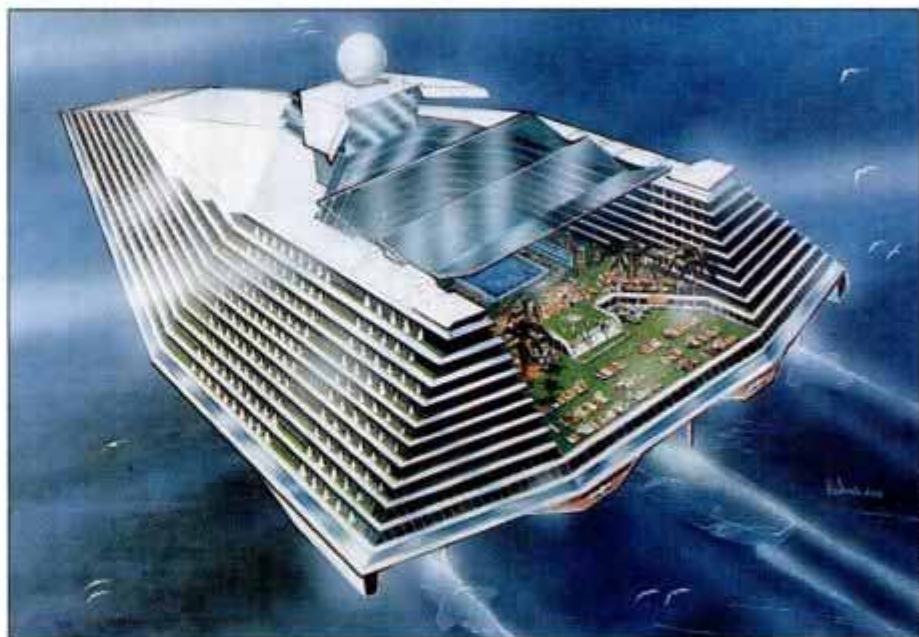
A trimaran SWATH concept permits additional space amidships for recreation.
