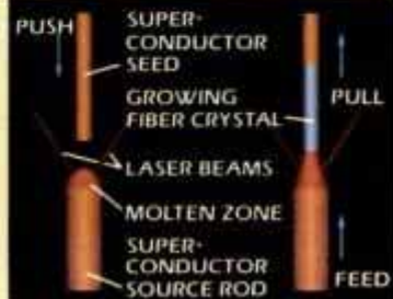
Inside pedestal-growth chamber (above) curved reflector focuses laser beam on all sides of hot spot. Process (below) involves pulling fiber away while feeding more source material into molten zone.
