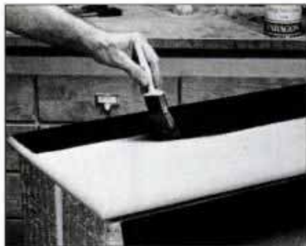
4 After priming the top for marbleizing, apply a coat of alkyd semigloss black paint. Masking protects the rest of the chest.
