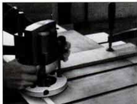
1 Cut case partitions to size, then lay out shelf locations on both. Use router and straightedge guide to cut shelf dados.
