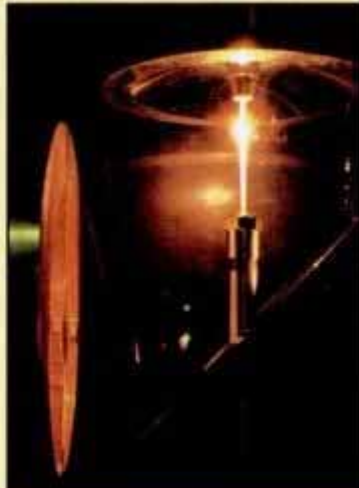
Inside pedestal-growth chamber (above) curved reflector focuses laser beam on all sides of hot spot. Process (below) involves pulling fiber away while feeding more source material into molten zone.
