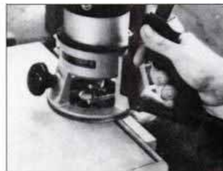
9 Rout spline dado in case sides using \frac{1}{4} -in. straight bit and router edge guide. Stop dado 1\frac{1}{2} in. behind front edge.
