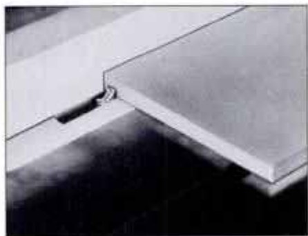
14 Readjust table saw fence and cut 1/4-in. groove in drawer sides, fronts and backs to receive drawer bottom panel.
