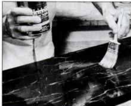
8 When the marbleizing is done, apply four coats of gloss varnish. If dissatisfied, wipe off the glaze and start again.
