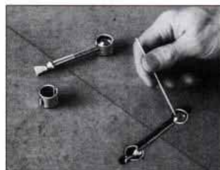
18 Use tight-joint fasteners and unglued spline to join both halves of bed platform. This joint is easily disassembled for moving.
