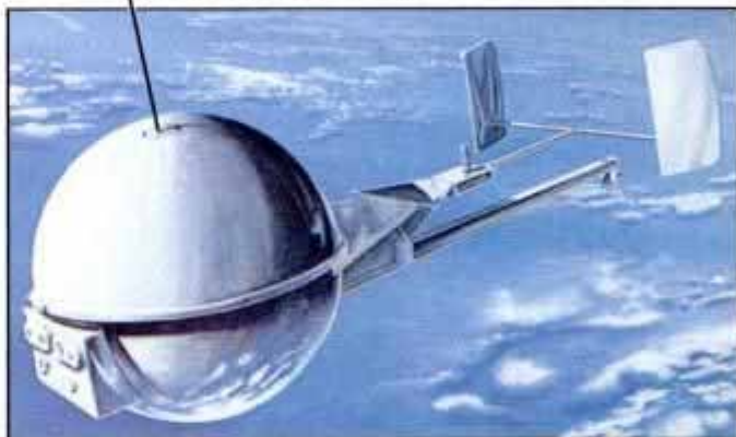
Tethered satellite's tail booms will house scientific instruments.
