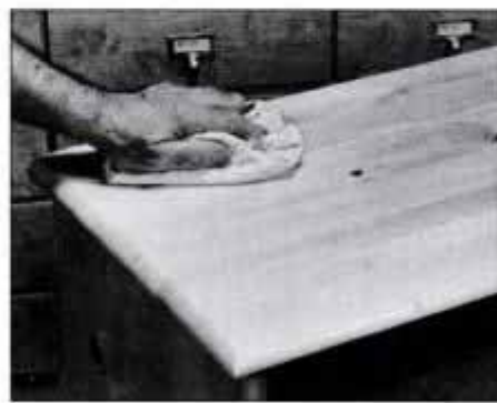
18 After final coat has dried, rub down cabinet with polishing compound. This softens the harsh gloss of the lacquer.
