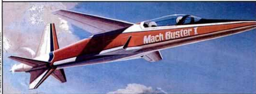
Mach Buster I features tail-pusher prop and high stubby wings to maximize lift-to-drag ratio.
