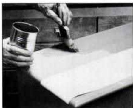
11 To create the look of two book-matched solid oak boards, mask half of the top before applying glaze coat.
