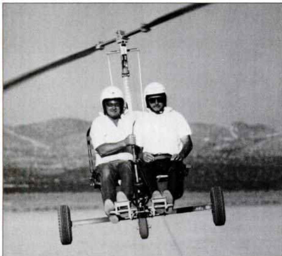
A towed unpowered machine gives beginning pilots first clues in gyro dynamics.
