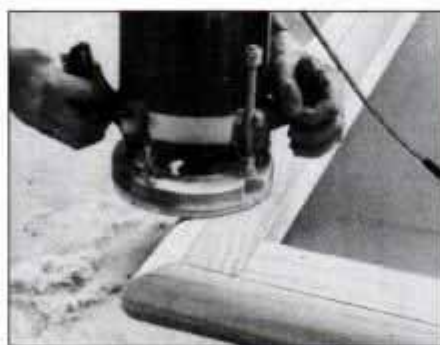
17 Attach edge banding and support strips to platforms, then rout radius on bottom edge first. Turn over and rout top edge.
