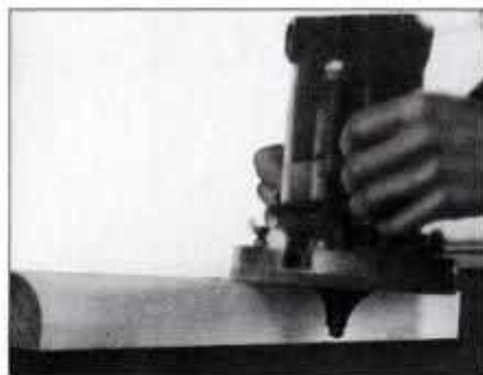
5 Glue and clamp poplar to case top and let dry. Then shape poplar edge by routing with \frac{1}{4} -in.-rad. rounding-over bit.
