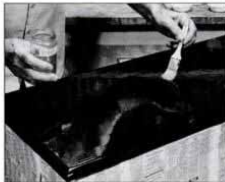
5 After painting the top black, apply a coat of shellac to produce a smooth surface. Then, apply a coat of clear glaze.
