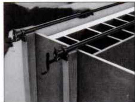
6 Glue and clamp top shelf and case bottom to partition assembly. Use cauls under clamp jaws to distribute clamping pressure.
