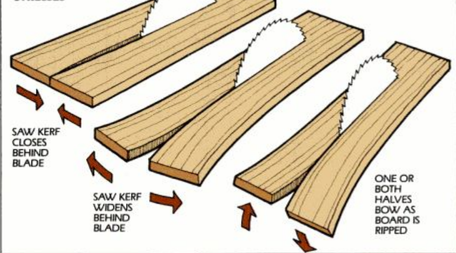
5 Cutting or planing boards with stresses can change the shape of the wood. It's wise to leave enough stock so the board can be rejointed after ripping. When planing, remove stock from each face equally. Binding (left) is typical of casehardened wood.
