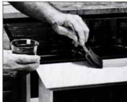
9 Wood-Sheen stain and finish can be applied with a soft cloth or foam pad. We applied two coats for desired luster.
