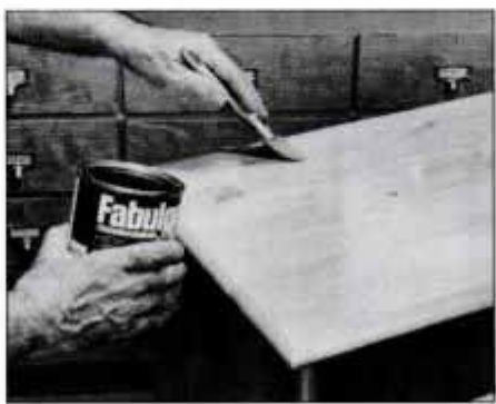
17 For a lustrous high-gloss natural finish, use three coats of brushing lacquer. Sand between coats with 220-grit sandpaper.
