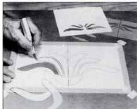
1 Mylar film is taped over drawing and cut with a razor-sharp knife to make stencil. Errors can be taped with transparent tape.
