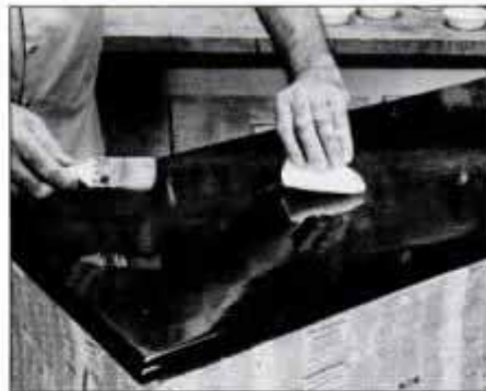
6 Add traces of white with a 2-in. brush to the glazed surface. Use a cloth wetted with clear glaze to soften white areas.
