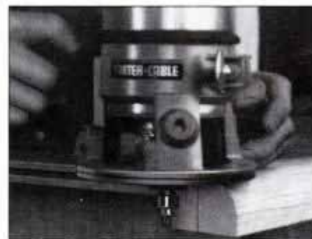
6 Rout spline groove on both ends of case top using a slotting cutter. Stop grooves 1\frac{1}{2} in. behind front of edge banding.
