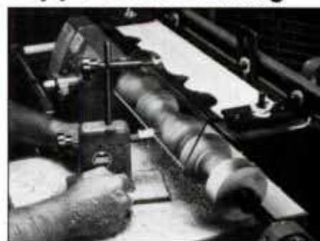
Lathe duplicator turns exact replicas quickly, easily. Here it's shown following a flat template as the cutter slides on the worktable.
