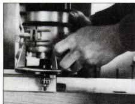
4 Cut poplar edge banding to size, then clamp securely to bench. Cut spline groove in edge using slotting cutter and router.
