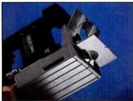
Bottomside-view of plate joiner shows carbide-tipped blade and adjustable fence. Knurled knob at left controls depth of cut.
