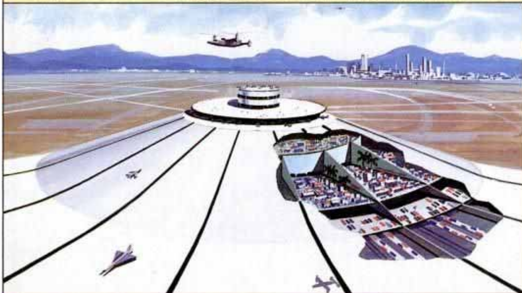
Subsurface highways would feed parking lot, hotels and convention center under Starry's radial airport.
