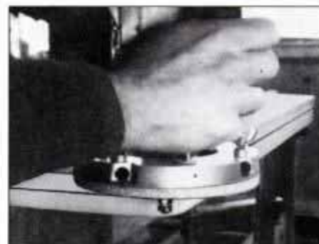
3 Align case side over template and clamp both to bench. Rout side flush to template using \frac{1}{4} -in. straight bit and pilot guide.
