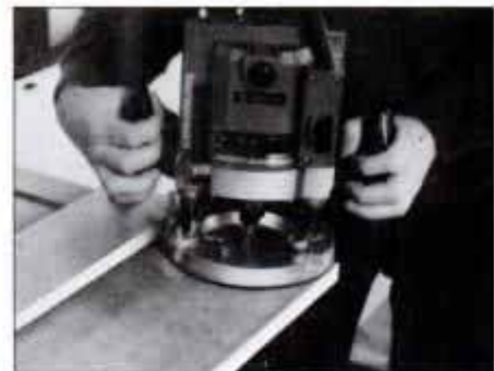
3 Again using a router and straightedge guide, cut dados in case bottom and top shelf to house the case partitions.
