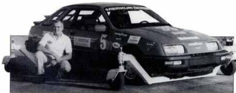
Outrigger-equipped Skid Car has become a fixture in the Bondurant driving school.
