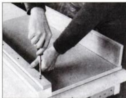
5 Glue and clamp wall cleat and edge banding to top panel. Rout profile on edge banding and attach doorstop to bottom edge.
