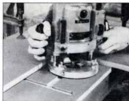
2 On case No. 1, lay out and rout additional dadoes to house the cubby drawer assembly. Use a straightedge to guide the router.
