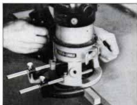
10 Glue and clamp poplar edge banding to front of headboard top. Let dry, then rout rabbet in back edge of top for case back.
