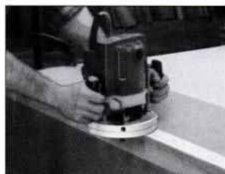
12 Rout radius on top corner of headboard edge banding with \frac{1}{4} -in.-rad. rounding-over bit. When done, sand profile smooth.
