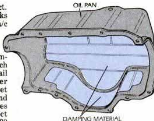
6 Even the steel oil pan benefits from added sound-deadening material.
