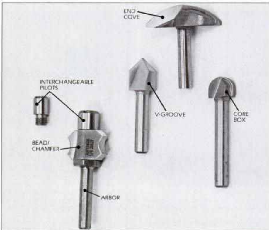
Router-bit set features four cutters that are used in different combinations to produce a wide variety of crown-molding shapes. End-cape and core-box router bits are carbide-tipped.
