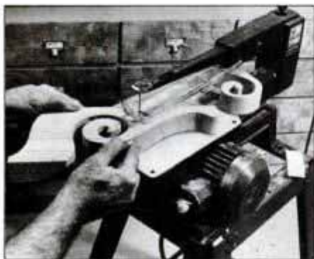
Direct-drive, ball-bearing motor powers the saw blade at 1700 spm to produce smooth cuts even in 2-in.-thick stock, as shown.
