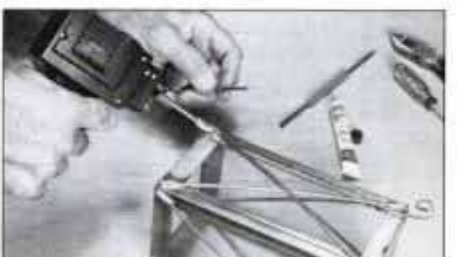
The heavy-duty, 60-watt tip worked well on repairing this brass lantern. Use this large tip for metal repair and stained-glass work.
