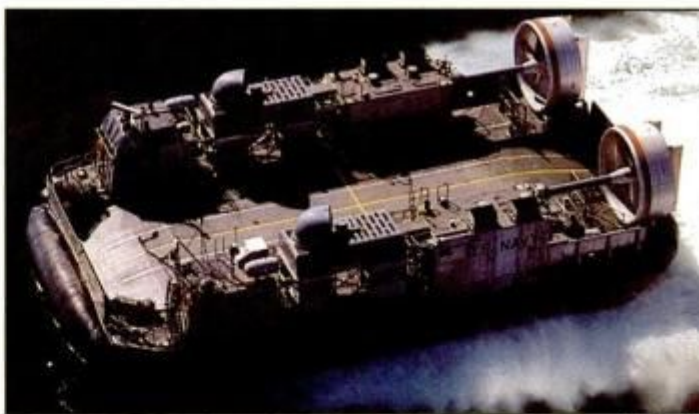
Navy's LCAC shuttles troops and cargo from ship to shore and inland.
