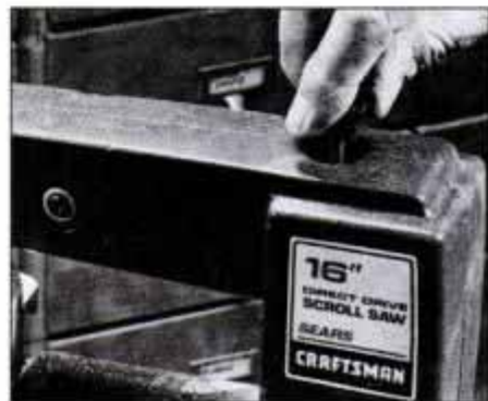
Blade tension is adjusted by turning knob located on top of the saw arm. A larger knob would provide a more comfortable grip.
