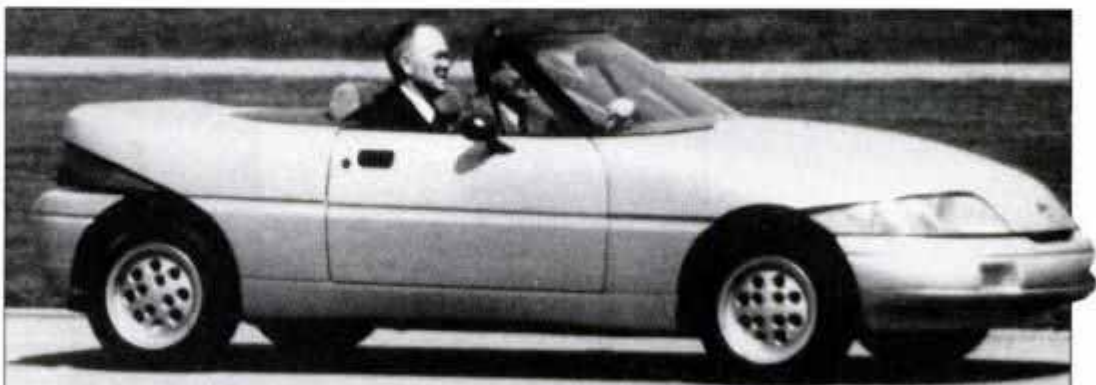
Plastic roadster is Ford's rolling test bed for fabrication of car bodies without the use of steel.
