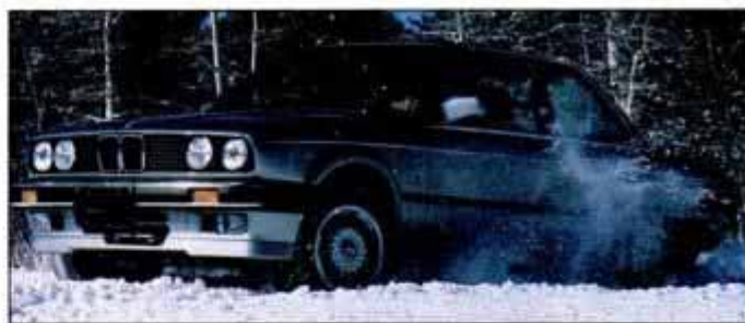
BMW 325iX is a full-time 4wd with a 37/63 front/rear torque split.
