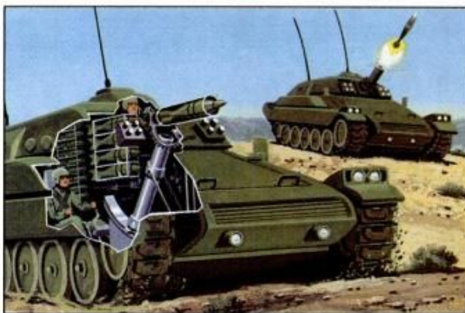
Automatic loader will feed tipped-muzzle mortar in 2-man vehicle.
