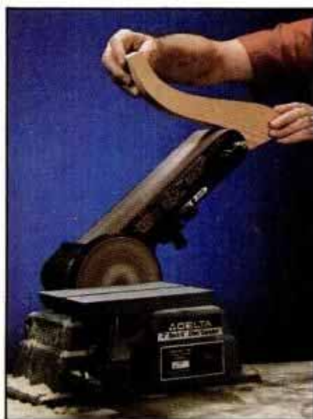
Sanding contours freehand is easy with the belt locked at an angle—about 45°. Work the piece over the rounded end of the arm.
