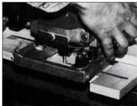
2 After assembling frames, rout a \frac{1}{4} -in.-deep groove 2 in. up from the bottom of each frame. Use a \frac{3}{8} -in.-dia. straight bit.
