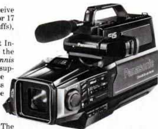
Electronic image-stabilization lens in camcorders eliminates jitters from home movies.
