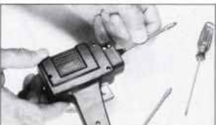
A screwdriver is all that's needed to change tips. Use the standard tip for most electrical work and do-it-yourself hobby/crafts kits.
