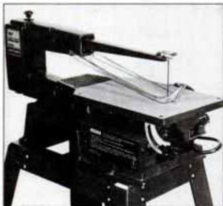
Benchtop scroll saw has a 16-in.-deep throat. The 5-in.-long blade is shielded by a clear plastic guard. Steel leg stand is optional.
