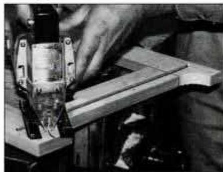
3 Lay out the 1\frac{1}{16} -in.-rad. arcs for the legs and cut with a sabre saw. Work from inside of frames and use a fine cutting blade.
