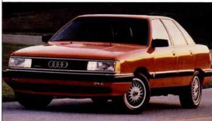
Audi 200 Turbo Quattro for '89 uses a 50/50 front/rear torque split.
