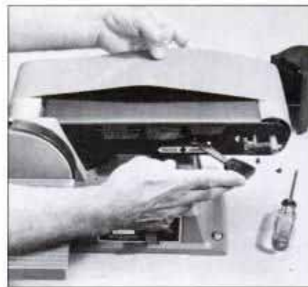
Convenient tension-release lever makes changing sanding belts quick and easy. Sander accepts 4-in.-wide × 36-in. belts.
