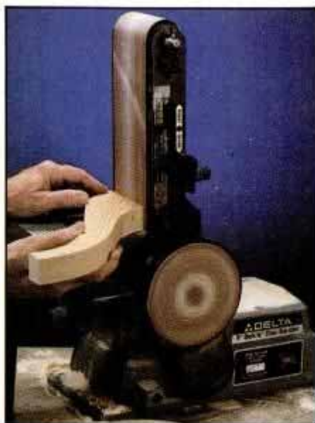
Position sanding-belt arm vertically to sand square ends. Check belt-to-table alignment with a square to ensure that it's exactly 90°.
