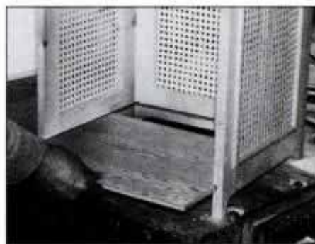
8 After assembling two sides to the back frame, slide \frac{3}{8} -in.-thick plywood bottom panel in place. Then, secure front frame.
