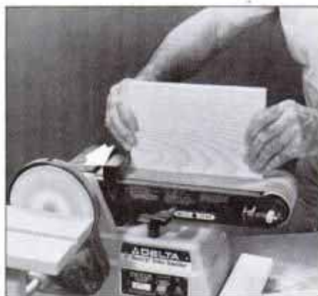
Install backstop (arrow) when sanding with belt in the horizontal position. It supports workpiece and offers much greater control.
