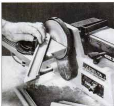
Worktable comes with a miter gauge for sanding precise angles. Worktable can be used with disc, as shown, or with the belt.
