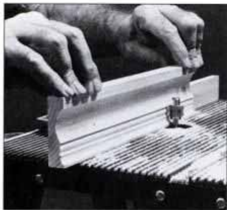
3 For the third cut, install the bead-and-chamfer bit and adjust the cutting height to a midway point between the first two cuts.
