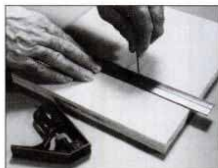
On most combination squares, blade can be removed from handle for use as a straight-edge rule. Use the scribe as a scratch awl.
