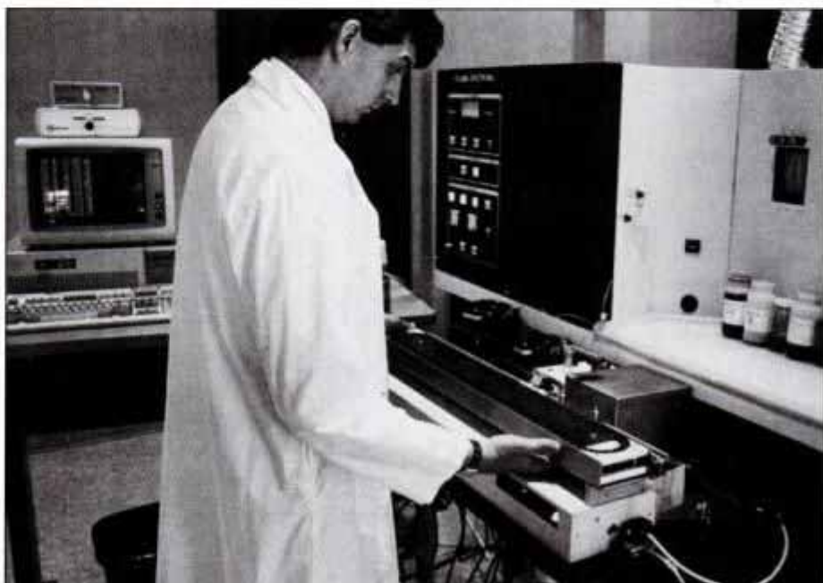
This $165,000 emissions spectrophotometer automatically checks tray of 100 oil samples and gives concentrations of contaminants in parts-per-million in 30 seconds per sample.
