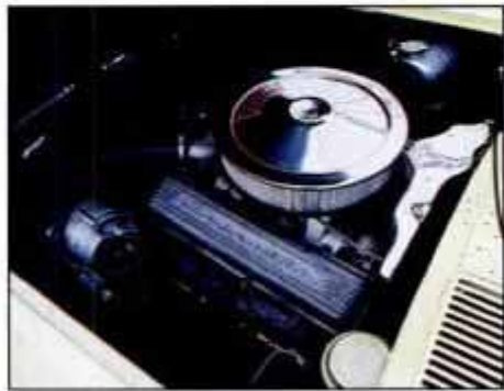
Ed Fischer's 1966 roadster is propelled by a 327-cu.-in., small-block V8 rated at 350 hp (SAE gross) and 360 lb.-ft. of torque. Narrow tires hampered the car's handling.
