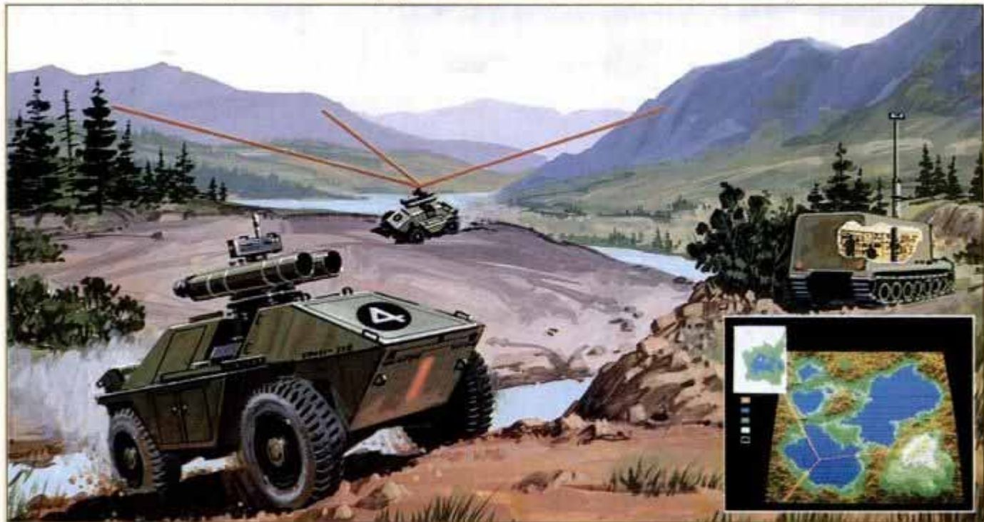
Vehicles controlled by mother tank (right) check laser rangefinder distances against digital terrain map (inset).
