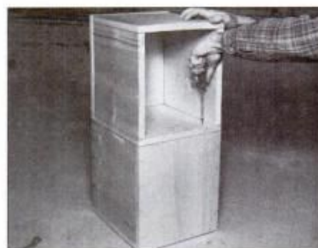
8 Fasten adjacent modules together with 1\frac{1}{4} -in. No. 8 fh screws. Notice the orientation of the openings as shown on drawing.
