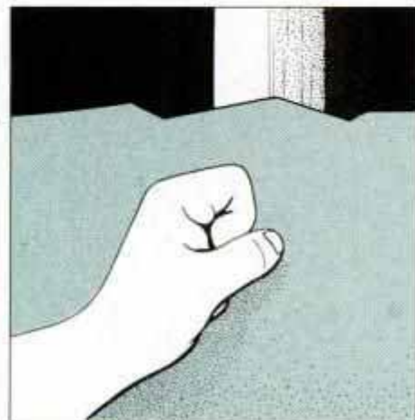
2 Using your knuckles, lightly tap along a wall and listen for a change in sound. A solid thud will be heard over a stud.
