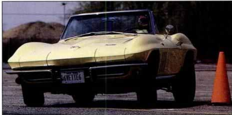
Ed Fischer's 1966 roadster is propelled by a 327-cu.-in., small-block V8 rated at 350 hp (SAE gross) and 360 lb.-ft. of torque. Narrow tires hampered the car's handling.
