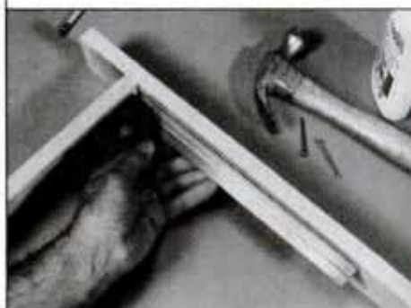
Use a combination square to check for square inside corners. Lock the blade so that its end is flush with the edge of the handle.
