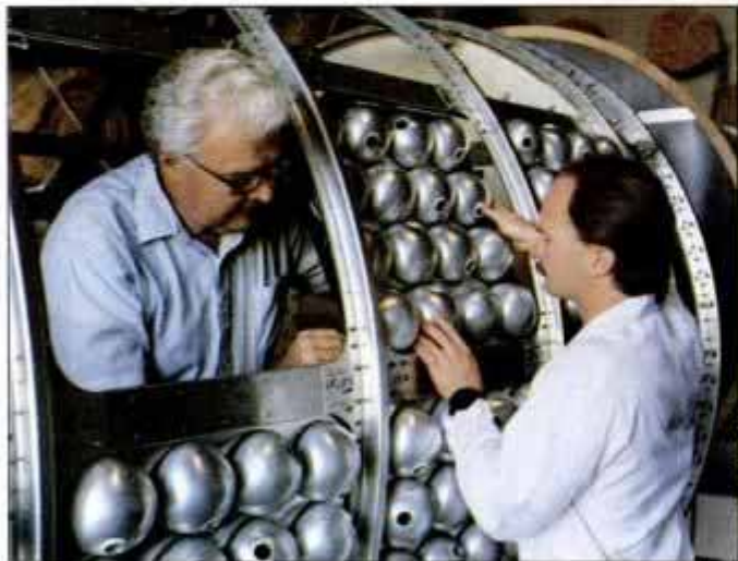
Series of 225 Hz resonators flew in propfan-modified test plane.
