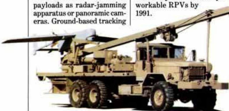
Skyeye is launched from truck-mounted catapult. Air vehicle has 20-ft. wingspan and packs fuel in wing bladders for 10-hour flight.
