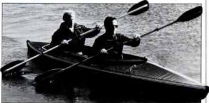
The Pisces folding, touring kayak can be assembled in 15 minutes.
