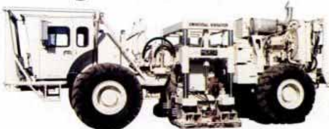
Vibrator's internal piston slams housing to create seismic waves.
