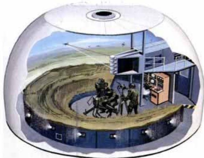
Slide projectors cast terrain background inside simulator dome.
