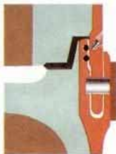
Challenger's offending SRB joint was a simple tang-and-clevis design.
