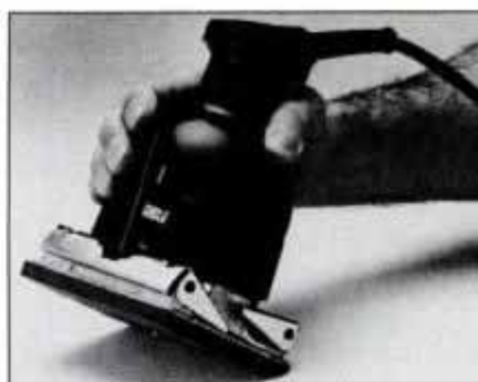
The Porter-Cable clamping mechanism requires a special tool. It's also easy to operate with an ordinary flat-tipped screwdriver.
