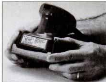
The twin-arm clamp design is opened by pushing the arms up and forward. Clamp is locked open for paper insertion.
