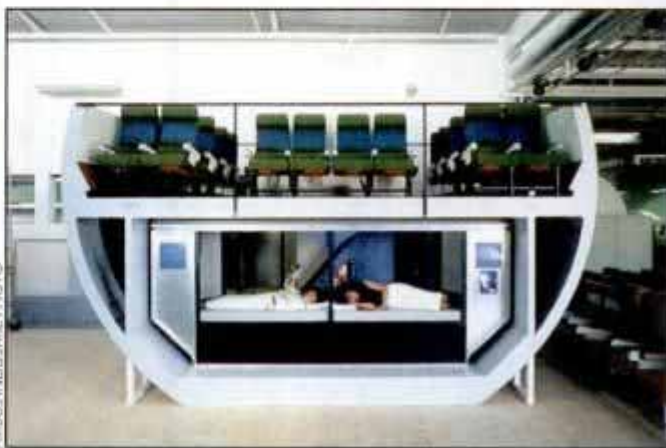
Airbus A340 model shows subcabin crew rest area.
