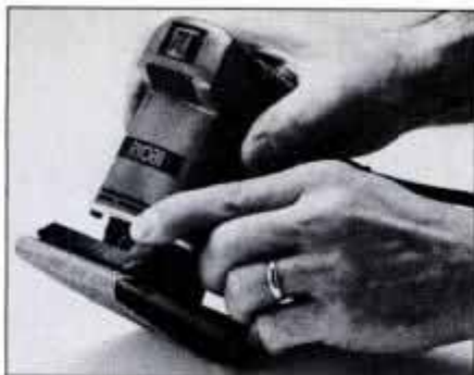
The most straightforward clamp is found on the Ryobi S-500A. Simply pressing the single lever-arm opens the spring-loaded clamp.
