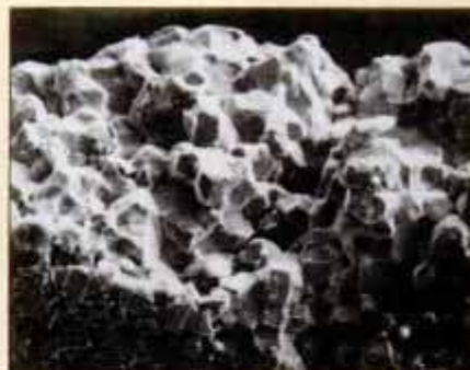
The 500X micrograph of an airframe crack (left) reveals transgranular, or cross-grain, fracture pattern of mechanical fatigue. Striations represent cycles of fatigue, and striation density is a gauge of airworthiness. The 170X micrograph of a failed aircraft component (right) shows a rougher intergranular, or between-grain, fracture pattern indicating corrosion.
