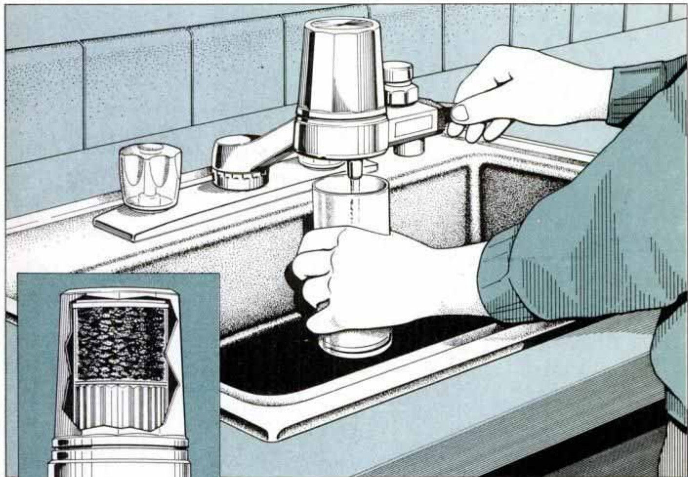
1 One of the most common types of filters uses a replaceable activated-charcoal cartridge (inset). This unit mounts to spout and can be bypassed when filtered water is unnecessary.
