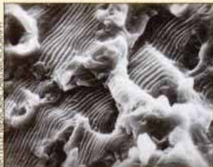
The 500X micrograph of an airframe crack (left) reveals transgranular, or cross-grain, fracture pattern of mechanical fatigue. Striations represent cycles of fatigue, and striation density is a gauge of airworthiness. The 170X micrograph of a failed aircraft component (right) shows a rougher intergranular, or between-grain, fracture pattern indicating corrosion.
