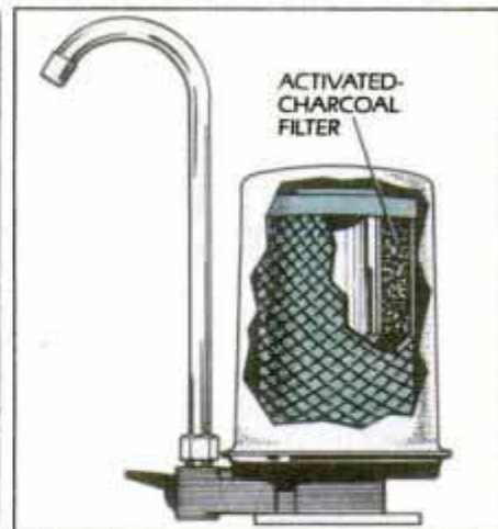
4 Countertop charcoal filters are connected to cold-water pipe. Replace elements as recommended by manufacturer.
