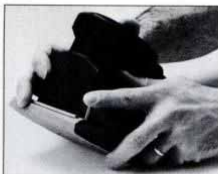
B & D 7445 uses a single-arm design. Spring tension holds clamp open. Pressing lever down forces clamp down on sandpaper.
