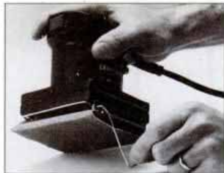
The bent-wire system utilizes the spring tension of the wire to hold the paper. One lever on each side controls clamping at each end.
