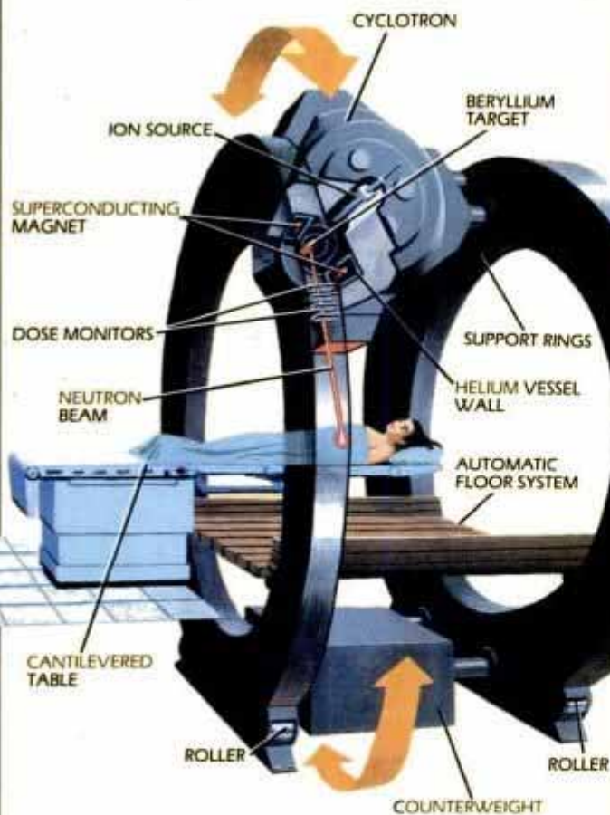
Cyclotron rotates so healthy tissue is spared the full dose.
