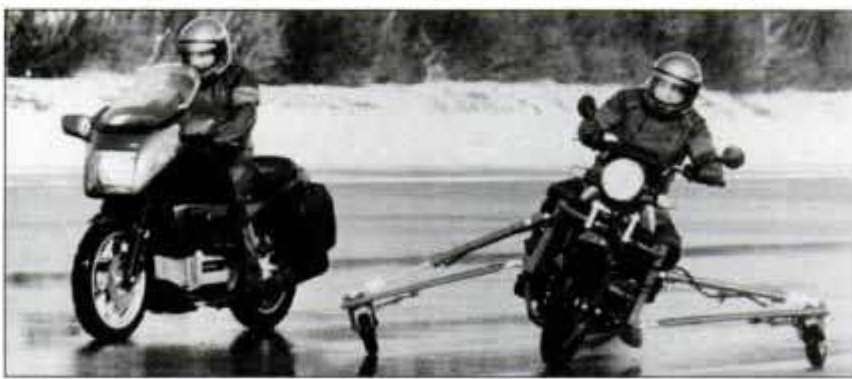
ABS-equipped BMW (left) stops safely, while conventional skids.
