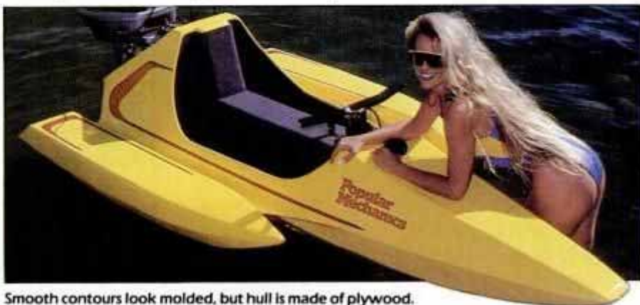
Smooth contours look molded, but hull is made of plywood.
