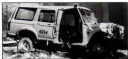
Bronco II 4-door proto after crash testing.
