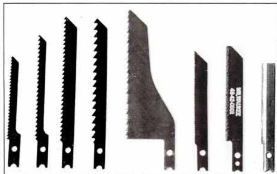
Here's a sampling of sabre saw blades, (l to r), 14-tpi scrolling, 12-tpi scrolling, 10-tpi taper ground, 6-tpi rough cut, 10-tpi flush cut, 24-tpi metal cutting, carbide grit and knife-edge.
