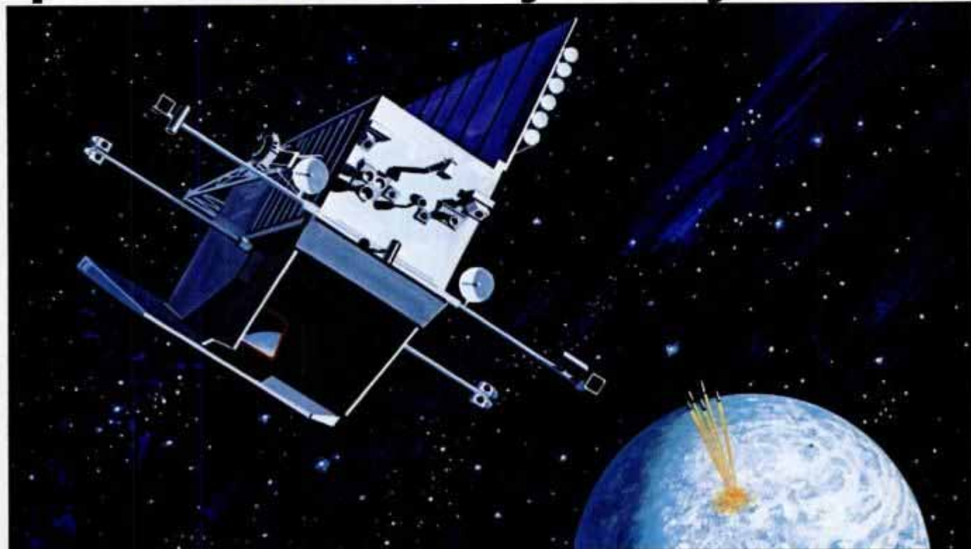
Above, Lockheed-conceived BSTS craft detects heat of ICBMs' liftoff plumes. Mirror in recess guides infrared radiation to concealed array of charge-coupled devices. Functions of external devices are classified. Delta-launched experimental module (left) contains both active and passive sensors, including laser detection and ranging (ladar).
