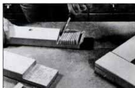
Using a chisel, break out the waste and scrape the joint smooth. Assembled half-lap, shown at right, forms a clean, strong joint.
