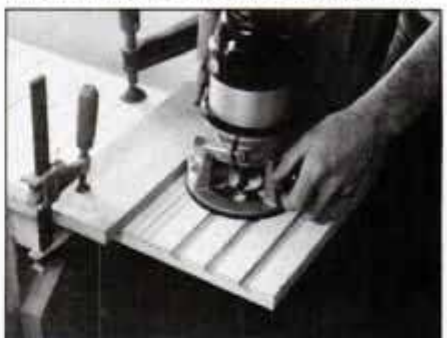
15 Begin the dentil molding by routing \frac{1}{2} -in.-wide dadoes across 1x12 stock. Board clamped to work guides router.
