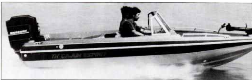
Tucked-under engine makes boat jump on plane, but plow water like a barge unless corrected.
