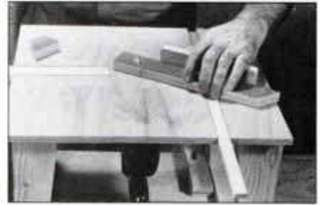
Execute square and angled crosscuts with a miter gauge. Gauge slides in a 5/16-in.-deep x 3/4-in.-wide slot that's routed in the tabletop.
