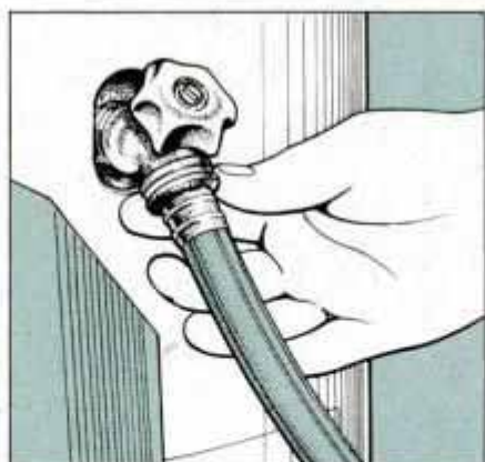
2 Attach a garden hose to the drain valve. Open the T&P valve or the hot-water taps in your house and drain the tank.
