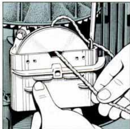
10 With spring tensioned, pass rope through housing, under clip and through hole in pulley. Knot end and pull snugly.
