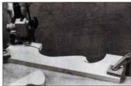
Cut out sharp inside corners in stages. First saw into the corner, back out the blade and then come back and make the finishing cuts.
