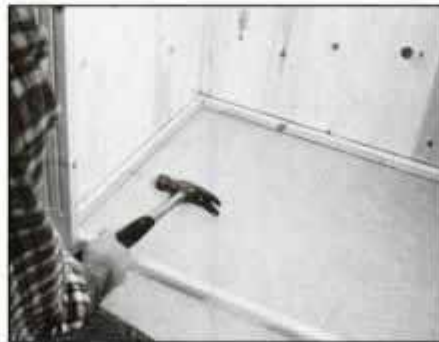
8 After nailing \frac{3}{4} -in.-sq. strips across cart front, nail strips around bottom edge of sides and back to support bottom panel.
