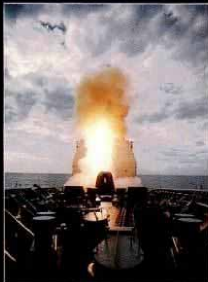
A vertical launch Standard surface-to-air missile aboard contemporary cruiser Lake Champlain leaves magazine in less than a second.
