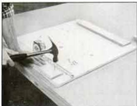
4 Select the best face of side and back panels and nail cleats in place. Don't use glue to avoid cracking or warping of the panel.
