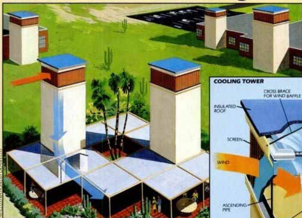
Hot air enters cooling tower (red arrow), cools and sinks (blue arrow). Detail of tower top (below) shows pump system recycling water to keep pads wet.
