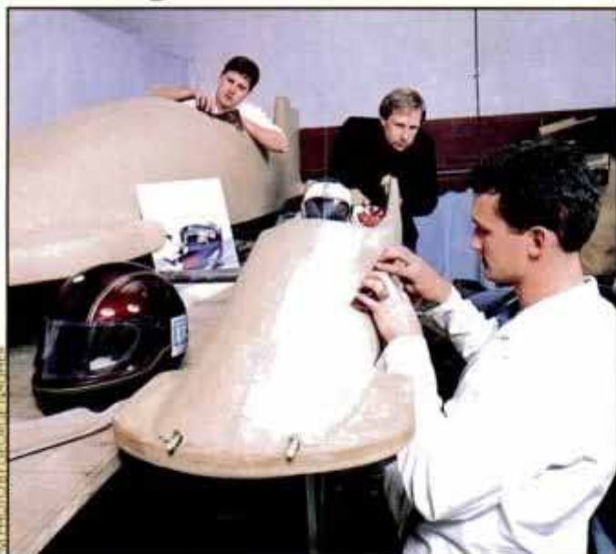
Airflow Sciences engineers craft sled model from clay.
