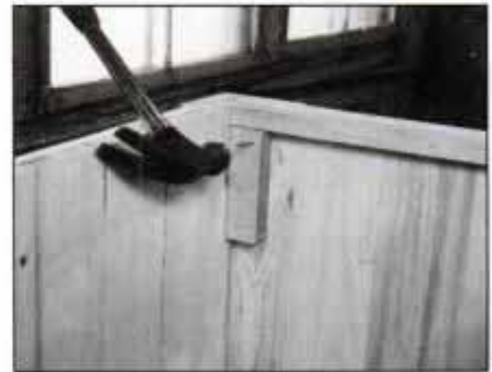
9 Glue and nail \frac{3}{4} -in.-sq. strip to upper back edge. Then secure the corner blocks with 3d finishing nails and glue.
