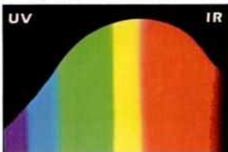
Composite sunglasses (above) with two different temple earpieces and lenses, illustrate a variety of sport-tech elements. Curve of visible light (left) shows relative strength of colors allowed through sunglass lenses. Mid-chart colors are easiest to distinguish, so they're transmitted in greater strength. UV light, on left, and infrared, on right, are kept to a minimum.
