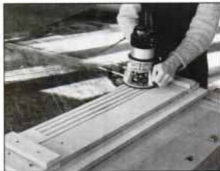
5 Leg fluting jig holds leg pieces in place and limits router travel. Use a \frac{3}{8} -in.-dia. corebox bit and router edge guide.
