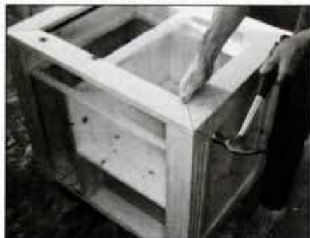
13 After cutting 1x4 cap pieces to length, nail in place on cart. Use glue and nail through each joint with finishing nails.
