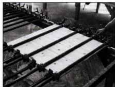
1 Edge-glue 1x4 boards for panels. Alternate clamps above and below. Be sure panels lie flat when clamps are tightened.
