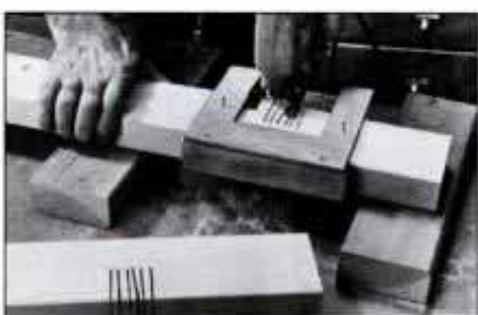
Form edge half-lap joints with this U-shaped jig. The jig guides the saw for the two outside cuts. Interior kerfs are made freehand.
