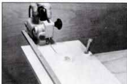
A straight wood strip, tack-nailed in place, ensures straight cuts. Note that strip extends beyond board to align saw at start of cut.
