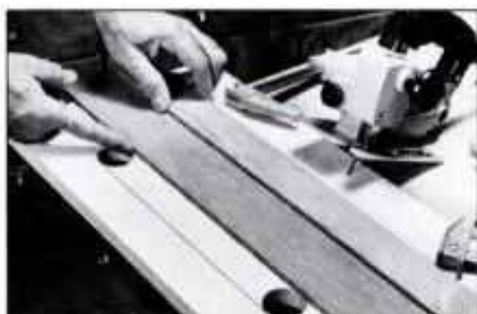
Customized-cutting guide requires no measuring. Simply place edge of guide on the line of cut. Saw blade will cut along guide edge.
