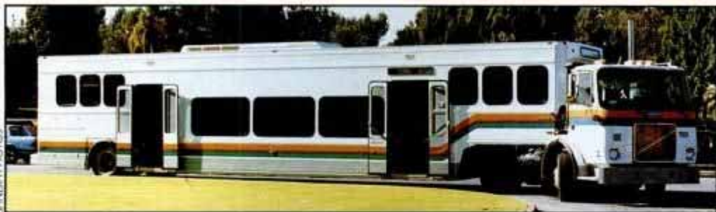
SuperBus negotiates curves more easily than conventional bus. Drivers like front-engine feel.
