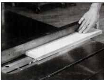
17 After cutting drawer components to size, cut \frac{1}{4} \times \frac{1}{4} -in. groove in sides and front with dado blade mounted in table saw.
