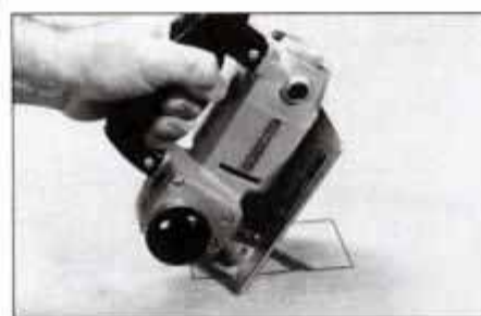
To make a plunge cut in the center of a board, tilt saw on its nose, start motor and then slowly lower the rear end of the tool.
