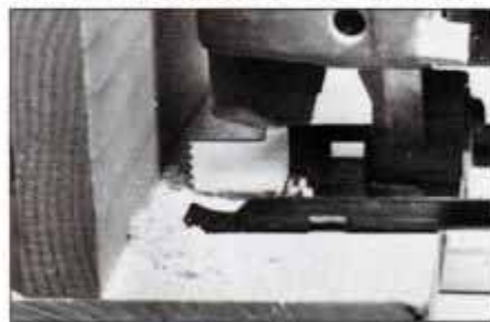
A flush-cut saw blade allows the saw to cut right up to a perpendicular surface. It's best to start the cut with a standard saw blade.
