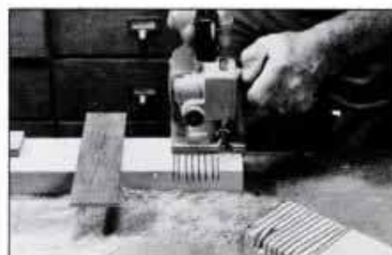
Cut end half-lap joints with a short blade. Wood plate under saw's base controls depth of cut. Strip nailed to work guides first cut.
