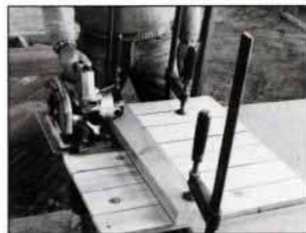
3 Mark panels to exact size for cutting. Clamp each panel to the worktable and use a straight board to guide the saw.
