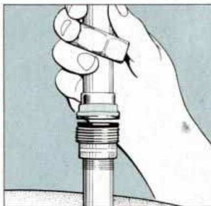
6 This dielectric union uses a rubber washer and a plastic insert to keep the brass upper half from contacting the iron half.
