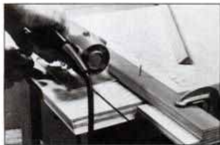
Some saws have a tilting base to cut bevels. Use a straight board to guide saw. Block clamped to guide supports saw at the start.
