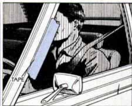
Wind flutter in trim can be located by temporarily taping down suspect pieces.
