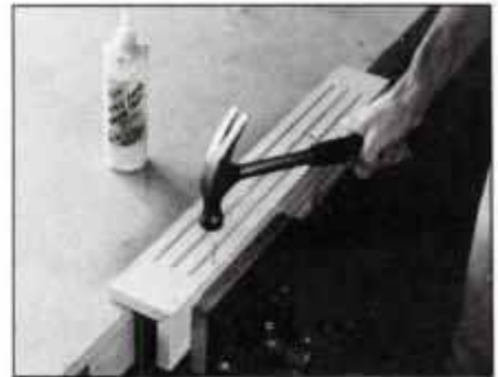
6 After ripping a 45° bevel on one edge of each leg piece, apply glue and nail pairs together with 4d finishing nails.
