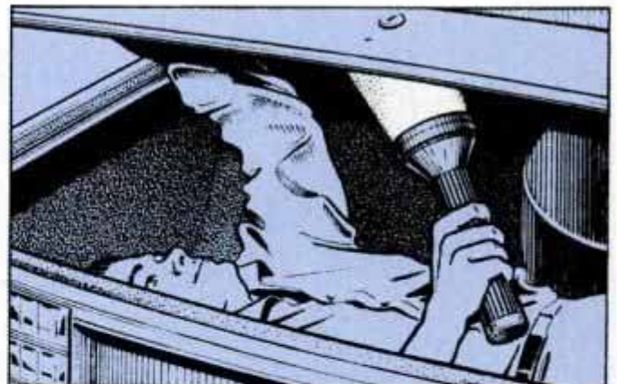
You, or a volunteer may have to get into the trunk to pinpoint leaks.
