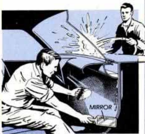
A mirror and a flashlight will come in handy for restricted areas like the dash.
