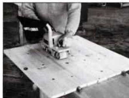
2 After glue has cured, scrape off excess and belt-sand panels smooth. Keep the sander moving with even pressure.
