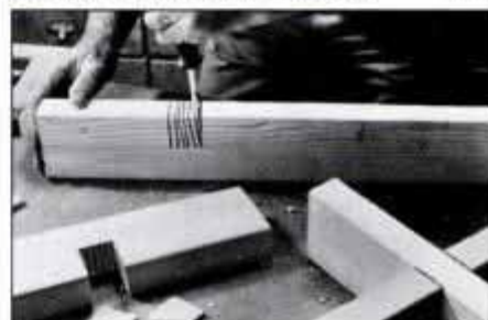
Break out the waste with a chisel. The two parts lock together and form a clean, invisible joint, as shown in the right foreground.
