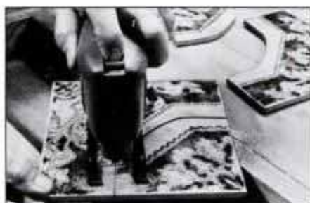
A tungsten-carbide-grit blade will cut ceramic tile, slate and other very hard, abrasive materials. Apply slow, steady pressure.
