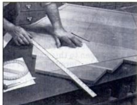
6 Make a cardboard template of the 108° corner angle to aid in laying out the table outline on the underside of the tabletop.
