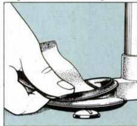
11 Before installing new ball or flapper, sand valve seat flush with fine sandpaper. To avoid damage, use light touch.
