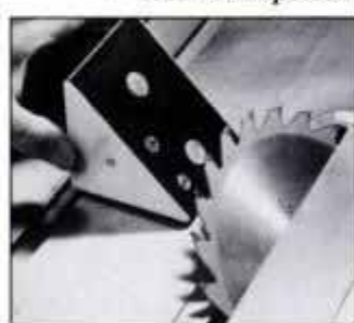
Two additional probes are utilized for checking 45° surfaces. Be sure that tool is disconnected from outlet before testing.
