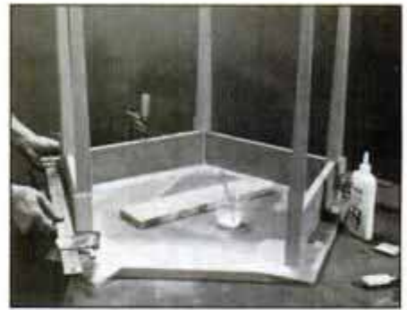
15 After adding the connecting rail, glue and clamp the fourth rail and last leg to the assembly. Finally, add the remaining rail.
