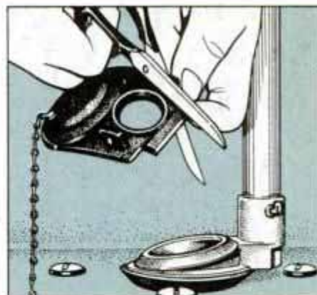
7 If replacing flapper on a flush valve that has no side pegs, slip collar over the tube. If pegs are present then cut off collar.
