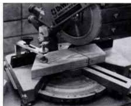
Accessory holddown clamp, attached to the left fence, is necessary when cutting workpieces too short to hold safely by hand.
