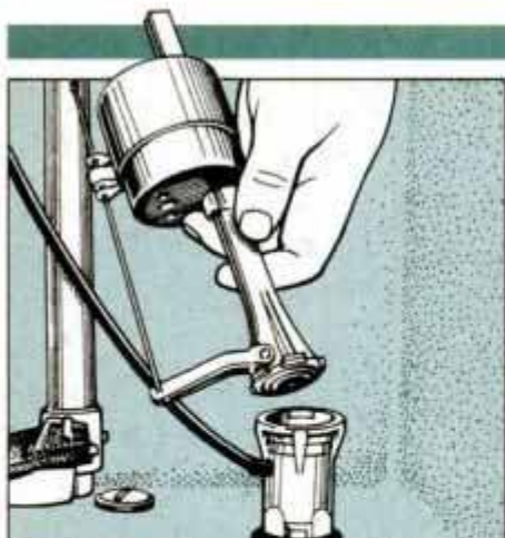
22 If sediment is a problem, a Fluidmaster ballcock replacement makes sense. It comes apart easily for cleaning.
