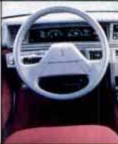
Cutlass Supreme combines look of analog instruments with vacuum fluorescent technology, for attractive solution to analog versus digital.
