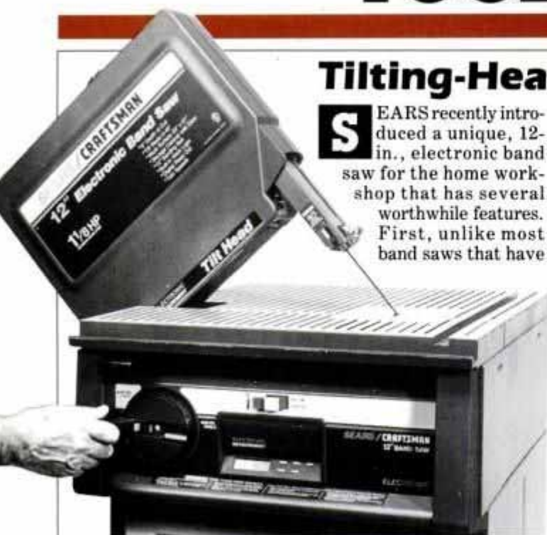
Band saw features a tilting head for bevel cutting. Release bevel lock and turn hand crank to desired angle. LCD reads out bevel angle.
