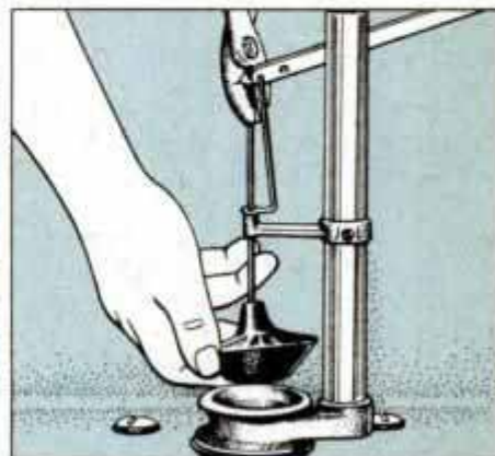
9 To remove a defective tank ball, hold the lift wire with pliers and unthread the ball. Old, brittle rubber will often tear.
