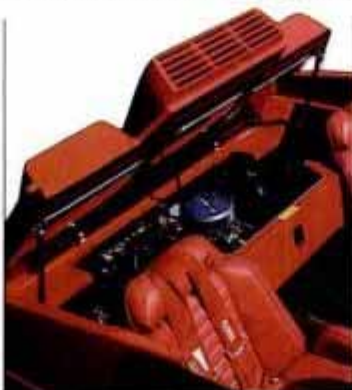
Under functional intake is 351-cu.-in. block bored to 403 cu. in.
