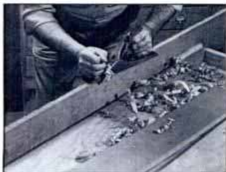
1 Plane one edge of each tabletop board straight and square before ripping. Use the longest plane you have for best results.
