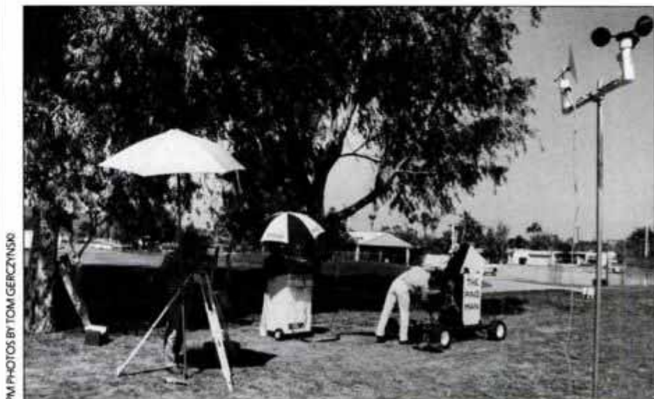
Karsten engineers use laser theodolite and meteorological instruments to test Ping irons.
