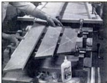
5 Assemble top in two stages. Lightly clamp flat, sturdy cauls across joints with wax paper between cauls and tabletop.
