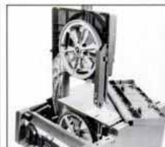
To change blades, remove upper wheel guard and front section of the worktable. The saw accepts 80-in. blades up to ½ in. wide.
