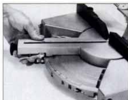
Slotted miter arm pivots left and right for miters up to 45°. Nine positive stops ensure accuracy for the most frequently cut miters.
