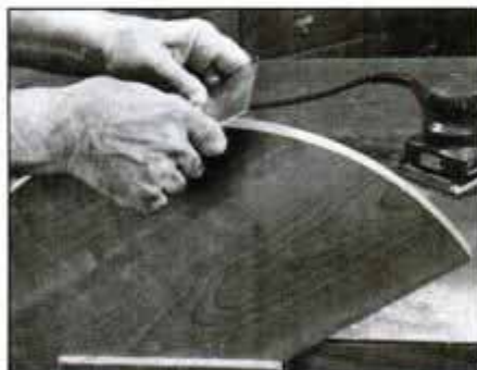
4 Clean up the rough-sawn edge with a cabinet scraper. Finish by sanding with a palm sander or with sandpaper and block.
