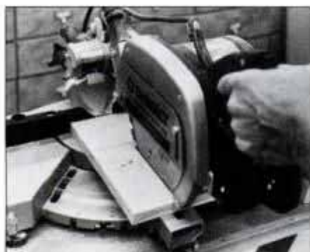
To crosscut a wide board, first pull the handle to extend saw head. Then, start the saw, lower it and push back toward the fence.
