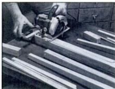
11 A T-shaped right-angle guide aids in cutting legs squarely to length. Clamp two legs together and cut in one pass.
