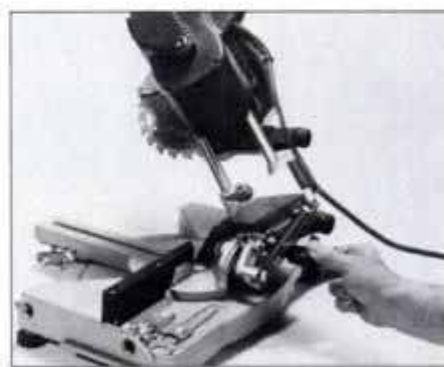
Adjust the bevel angle of the saw by adjusting the bevel lock knob. Note that the saw head is mounted on two parallel steel rods.
