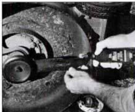
Compact size permits sharpening lawnmower blades without removing blade. Be sure to disconnect sparkplug wire first.
