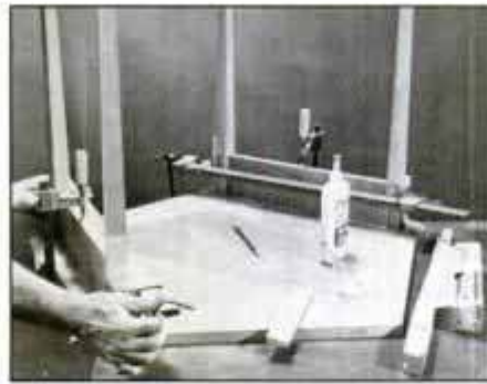
14 Glue two opposing leg assemblies first, using marked side of top as a guide. Use wax paper to keep excess glue off the top.
