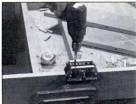
4 Keep the same side of doweling jig on working face of each board to ensure good alignment. Tape on bit acts as depth gauge.
