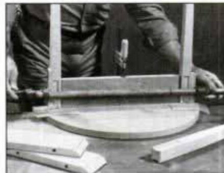
5 Assemble the rear rail and two legs with glue and clamp until dry. Use a layout drawn on underside of top as a guide.
