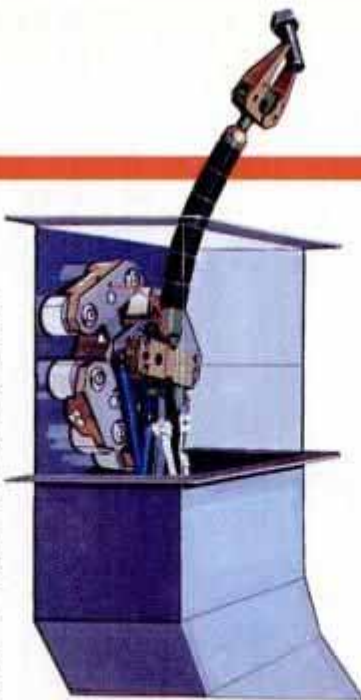
Crab can walk with up to 6.6 lbs. in its mechanical gripper.
