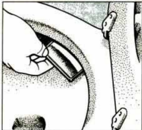
2 A dirty bowl usually means poor water flow from rim openings. To check clogged openings, hold mirror under rim.
