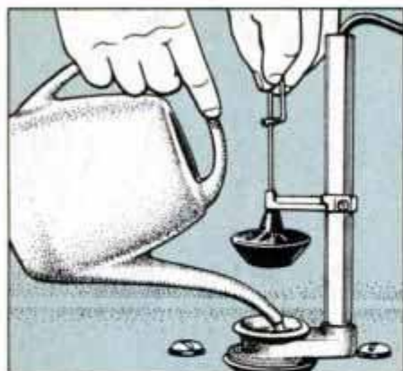
5 To clear congested rim holes, pour a 50/50 mixture of warm water and vinegar into the flush valve. Then ream holes with wire.
