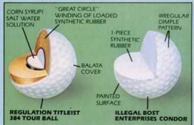
Makers claim that smaller size and added weight may give the 1-piece nonconforming ball (right) added performance.
