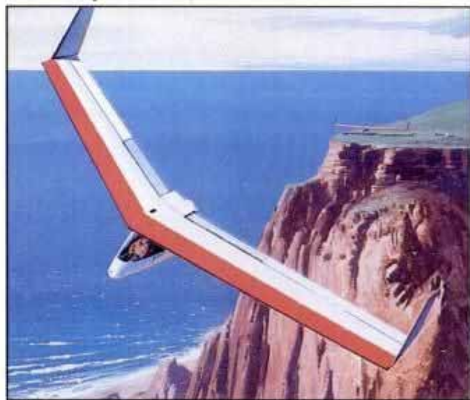
SWIFT's 35-ft. wingspan translates into a 23:1 lift-to-drag ratio.
