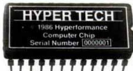
Electronic Control Module is usually under dash or behind kick panel. PROM is easily replaced: High-performance chip plugs in.
