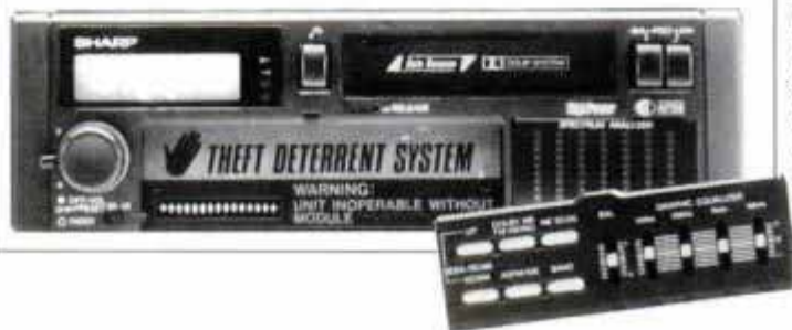
Technics' SL-P990 (above) is one of the first CD players with improved, 18-bit sampling. Sharp RG-F816 (below) deters car stereo thieves with pop-out module.
