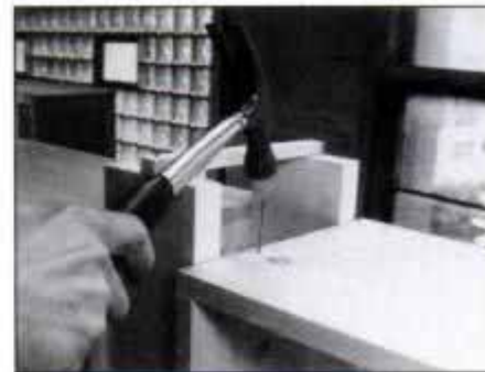
9 You'll need to remove the long spacers from upright tops when nailing the top shelves. Then, remove the short spacers.
