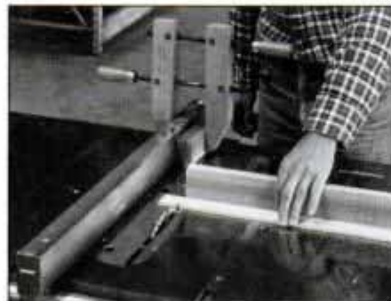
17 The decorative blocks are crosscut from \frac{1}{4} -in.-thick stock to 1\frac{1}{2} -in. squares. Use a stop block for accurate cuts.
