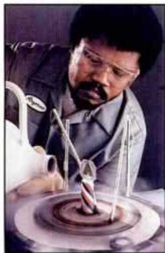
Argonne technician chills motor with liquid nitrogen.
