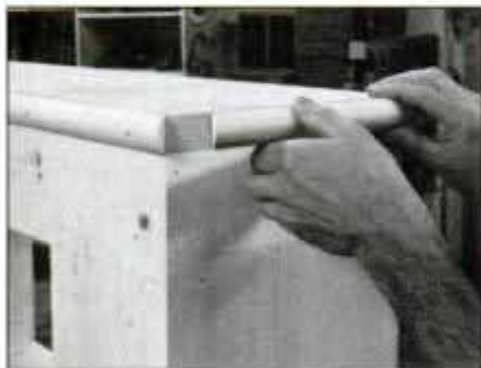
16 After marking and cutting miters, install with finishing nails and glue. Install long pieces first and cut short lengths to fit.
