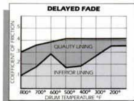
Some products begin recovery from fade, then the coefficient of friction plunges again.
