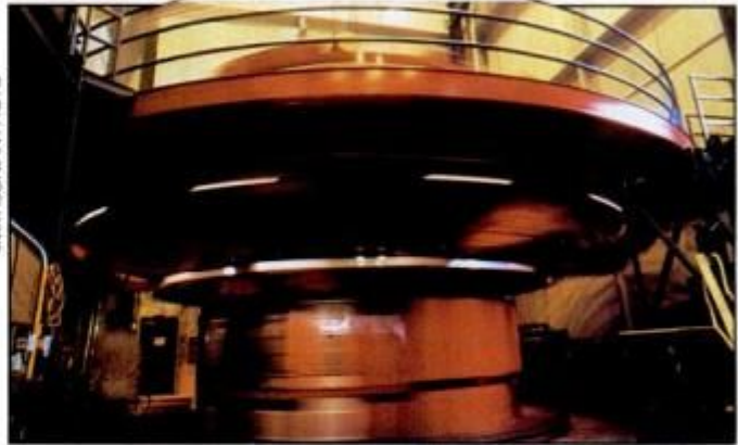
Furnace does 10 rpm for 24 hours at 1100 to 2000° F.
