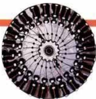
Electromagnets on plate bottom are simply bolts wound with copper wire.
