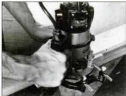
13 Make the molding with your router and rounding-over bit. Use a \frac{3}{8} -in.-rad. bit for the shelf trim and \frac{9}{16} -in. bit for the top.
