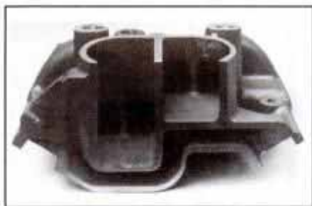
Cutaway of a high-performance manifold: The passage under the plenum is for exhaust heat, which is needed to maintain driveability in cold-weather conditions.
