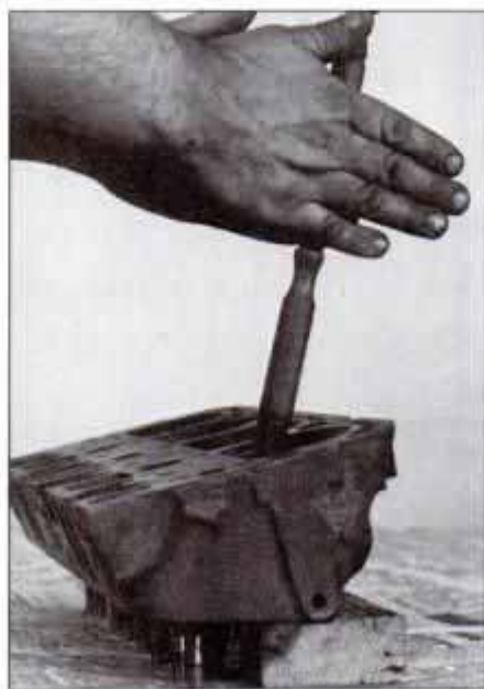
Valve lapping requires polished technique.
