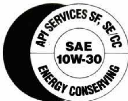
On every oil container you will find the API service rating and SAE viscosity rating.
