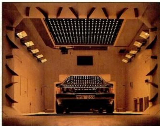
Saab tunnel ranges from -85° to 185° F with up to 95% humidity.
