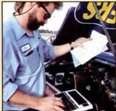
A laptop computer quickly alters the program of the engine management system.
