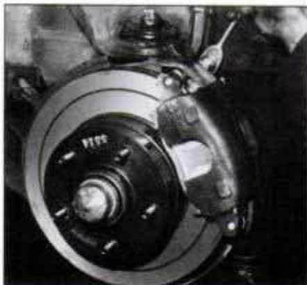
Don't forget to check and, if necessary, resurface rotors or drums. Proper surface finish is important to prevent brake squeal.
