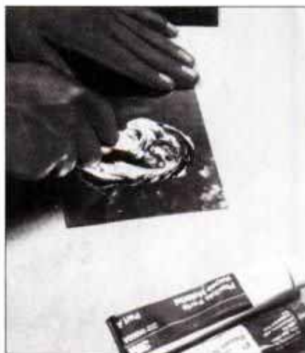
Mix equal parts of the flexible parts repair material on a nonporous surface.
