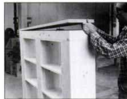
12 The top is cut to exact size from \frac{3}{4} pine stock. Make sure its edges are flush with the top trim before installing.
