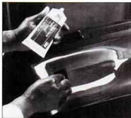
Smooth pinholes or uneven areas with some flexible parts putty and a body squeegee.
