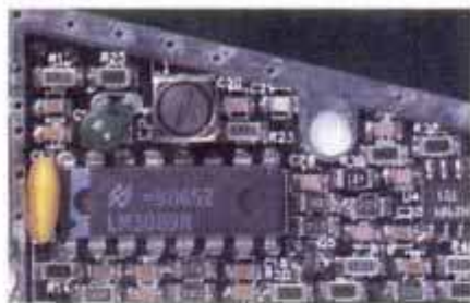
The EXPRESS 3 utilizes surface mount components
