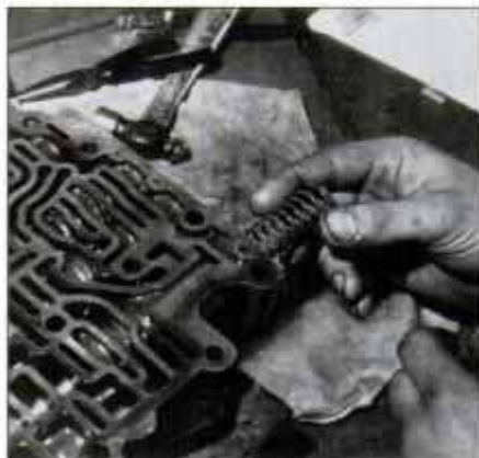
Control-valve springs provided with kit are installed in the valve body.
