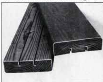
14 Special 2x6 Dura-Pine decking has rounded top edges and dual kerfs cut in the bottom surface to reduce cupping.
