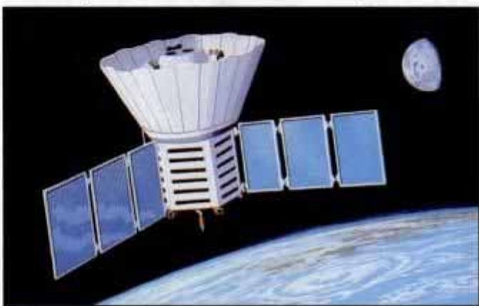
Skirt shields COBE's instruments from radiation sources.
