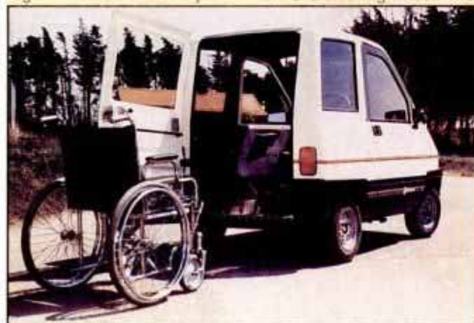
Handimobile minicar accommodates wheelchair by lowering floor.
