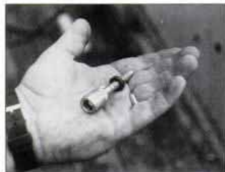
9 Here's a closeup view of a Jamb-Jack. Lagscrew shank is driven into studs and cylindrical head threads into door jamb.
