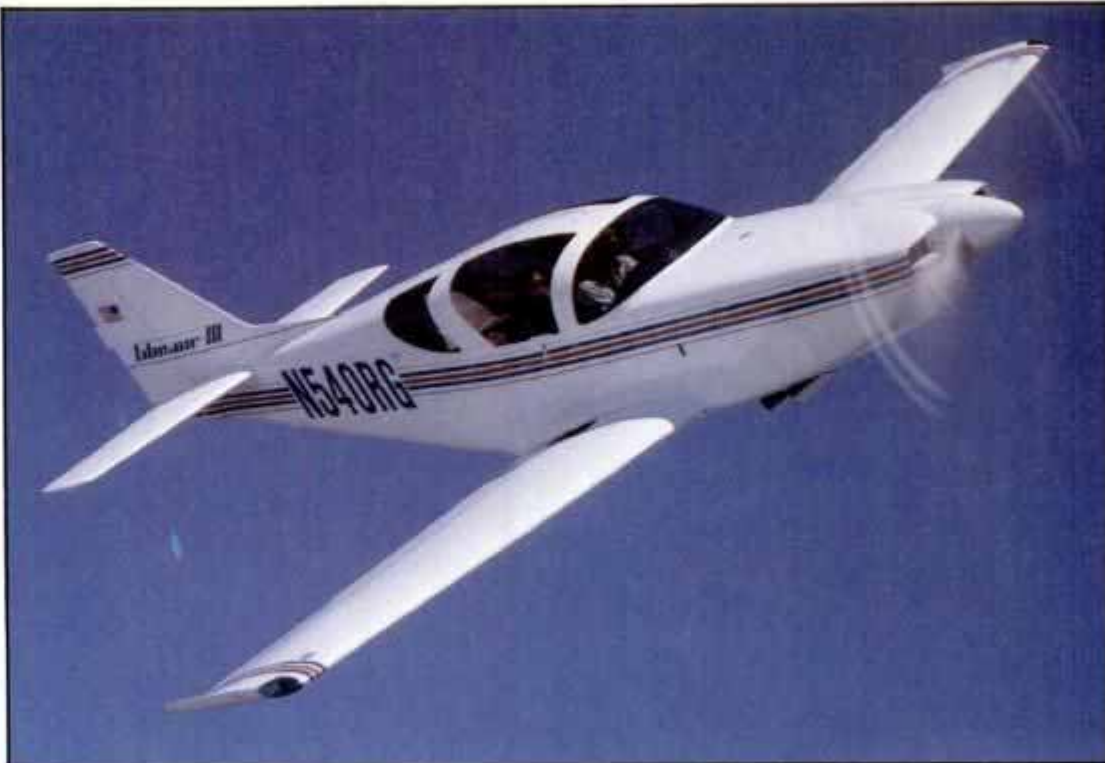
Two emerging standards: The all-composite Glasair III (top), considered the dean of the homebuilt trade, hits 270 plus. The Wheeler Express (left) also takes aim at the general aviation market with 195-mph, 4-place performance.
