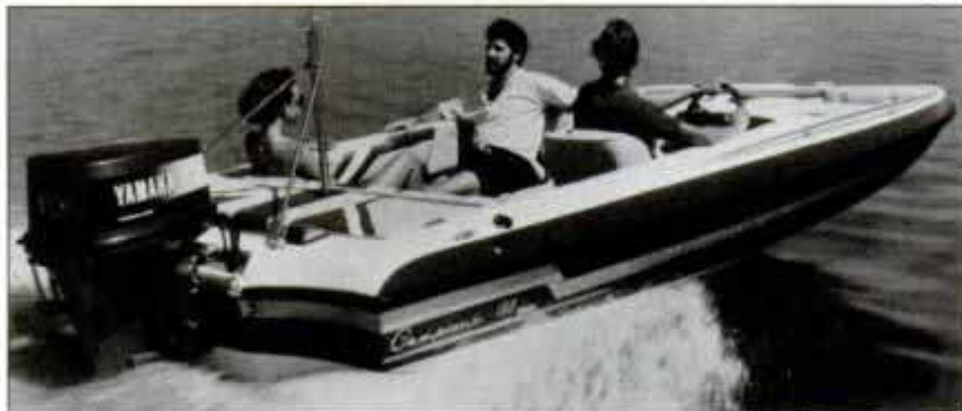
Yamaha's '88 130-hp V4 outboard is a harbinger of bigger things to come.
