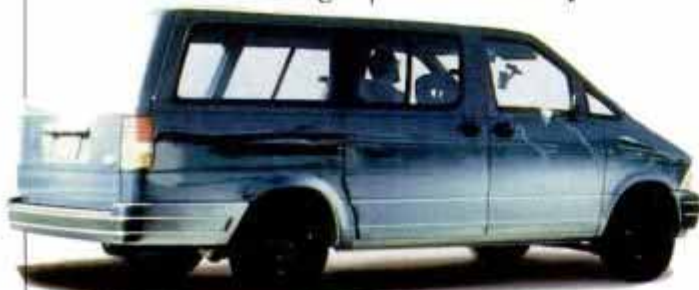
Ford's Aerostar for '89 has 18 in. grafted on behind rear axle.
