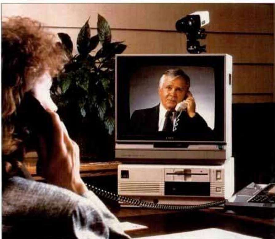
The U.V. Communicator sends full-color motion video over regular phone lines.
