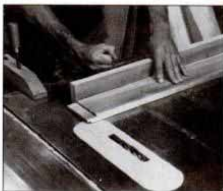
7 Cut tenons for the face frame and doors with a dado blade mounted in table saw. Hand screw clamp acts as stop block.
