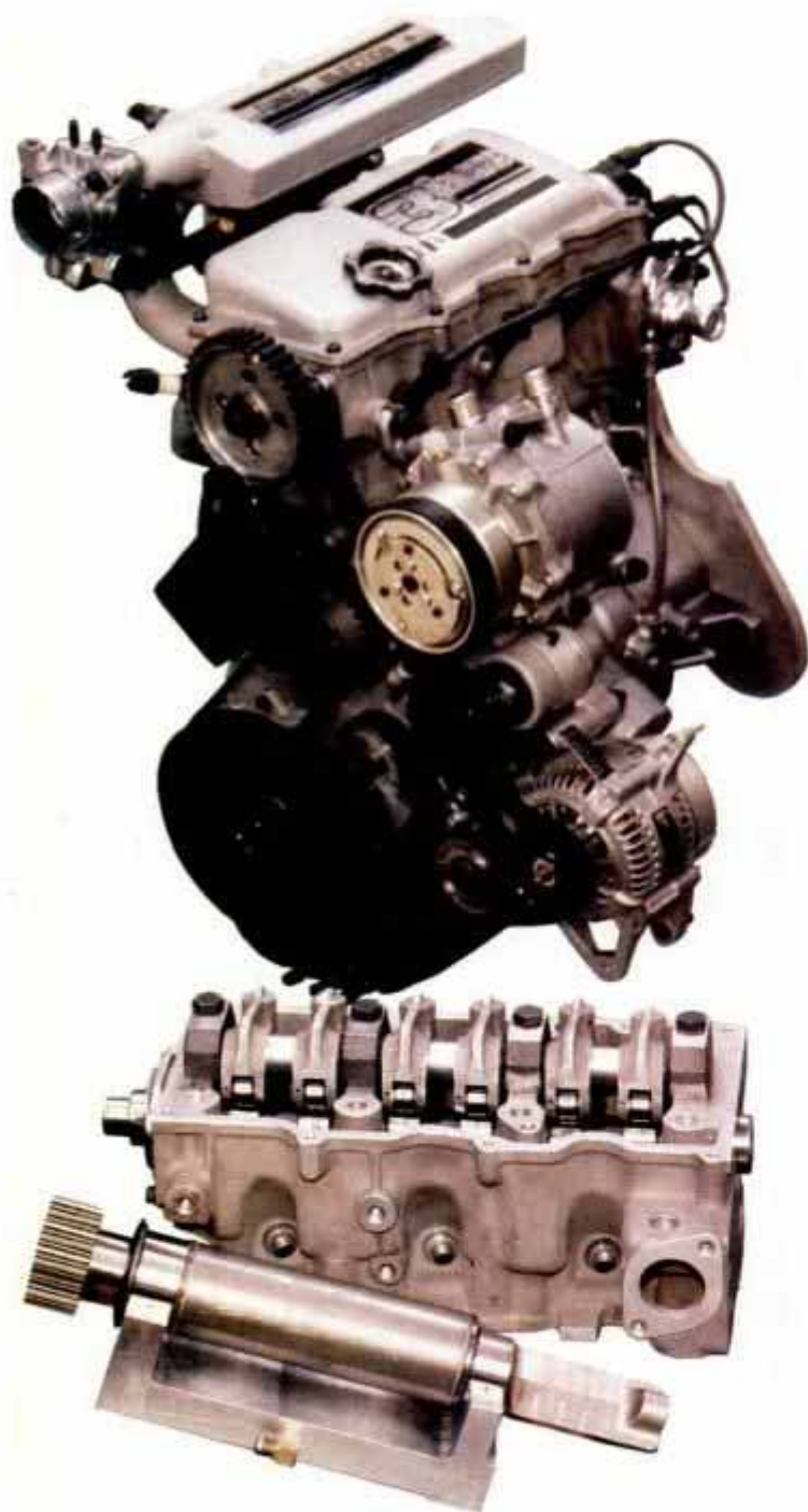
Concept 90 3-cylinder engine by Chrysler, developed for an as-yet unannounced car, uses sleeveless aluminum block, counterbalance shafts, cam low in head for hood clearance.
