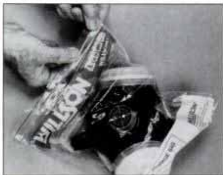
Store respirator in a tightly sealed plastic bag and keep it in a dry, cool place. Direct sunlight will promote rapid deterioration.
