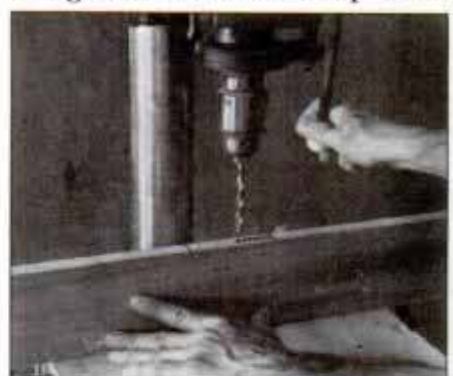
8 Begin the mortises in the face frame by removing most of the waste on the drill press. Use a sharp chisel to finish mortise.
