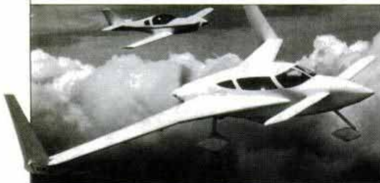
Velocity 4-placer is an all-composite design.
