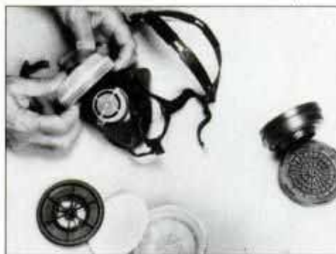
Here the cartridges are removed and just the filters are installed. The filters provide protection from dust only, not harmful vapors.
