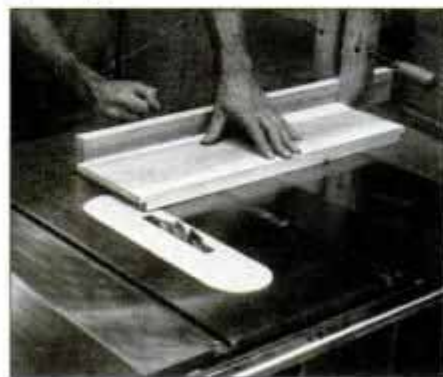
15 The rabbets for the drawer fronts, and other drawer joints, are cut with dado blade. Assemble with glue and 1-in. brads.
