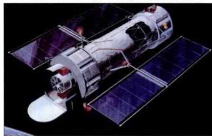
X-rays can't pierce our atmosphere, so AXAF will work 320 miles up.
