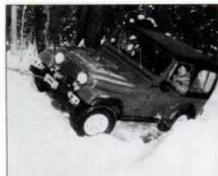
Step 3: With cable anchored to nearby tree (broad nylon-web belt protects trunk), winch and 4-wheel drive had us out, 1-2-3.
