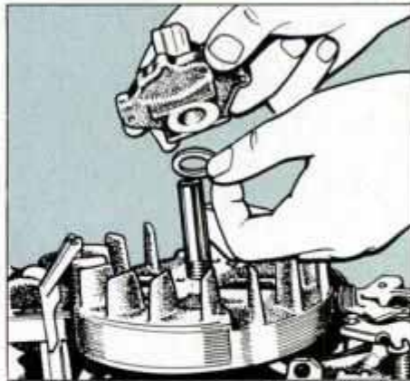
6 Once loosened, lift off the starter clutch and washer. Then, loosen the flywheel nut but leave it in place to protect threads.
