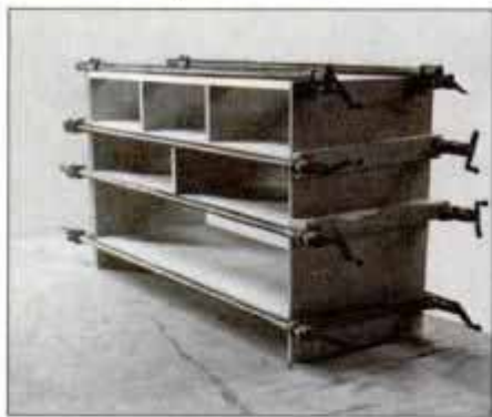
6 The assembled lower case is clamped until the glue sets. Cauls over each joint maintain even pressure along the joint.
