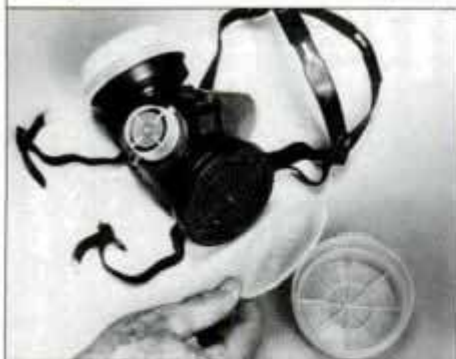
Install the appropriate cartridges for a specific contaminant. Note that respirator houses a dust filter and an air-purifying cartridge.
