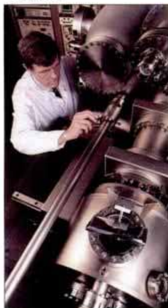
Molecular-beam epitaxy for mixing semiconductors.
