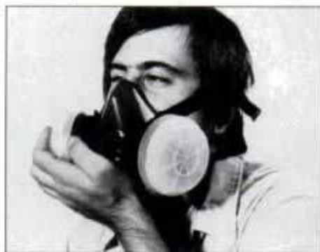
Make a positive pressure test to ensure a snug fit. Hold palm against valve and exhale. No air should leak from around respirator.
