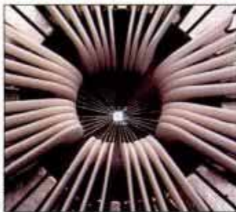
Testing apparatus dwarfs chip (left) that contains ultratiny transistors (above), enlarged 10,000 times.
