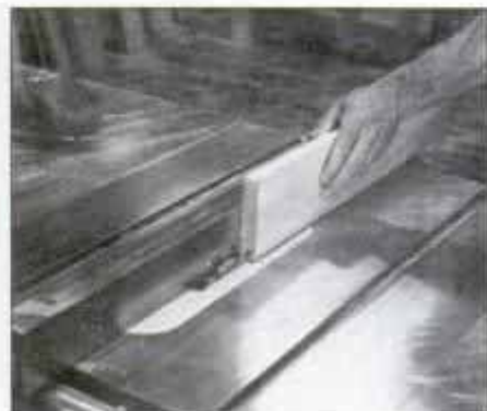
11 Door stile groove is cut on table saw with dado blade. This groove houses panel and acts as mortise for rail tenons.
