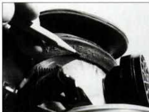
Inspect respirator periodically for signs of wear or damage. Any respirator that's dried out and cracked, as shown, should be discarded.
