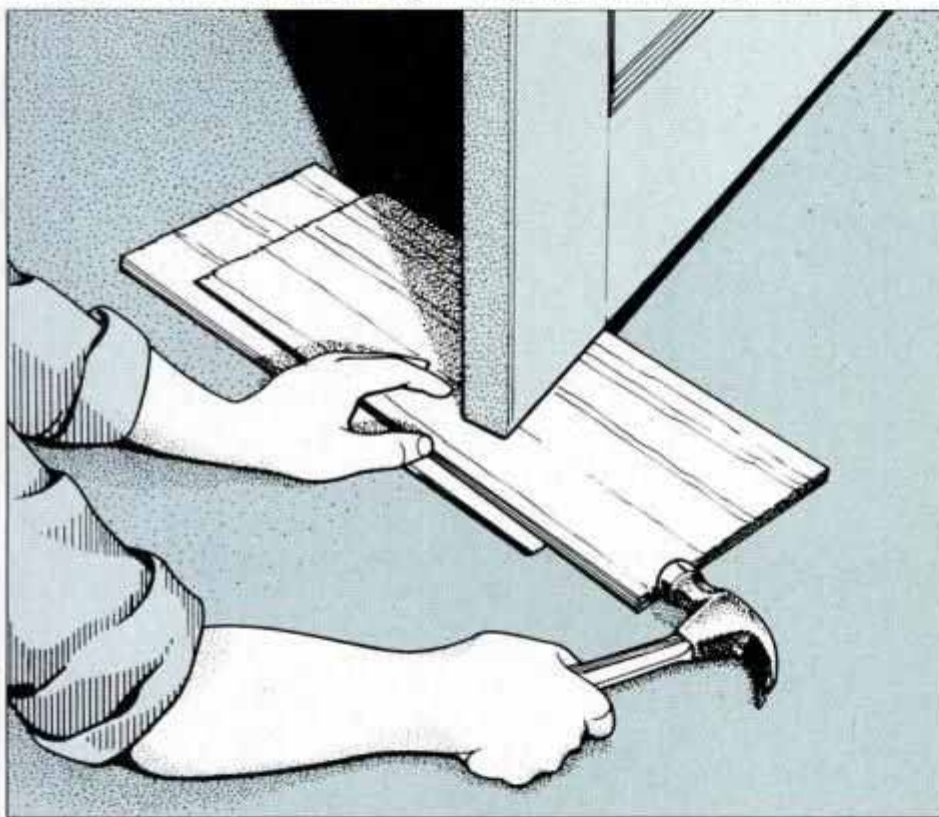
Before removing any of the hinges, place two opposing tapered wooden shingles under the door. Then, take the door weight off the hinges by tapping the shingles together.
