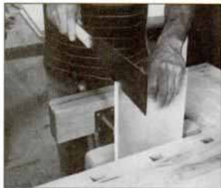
4 Panels that fit in stopped dados are notched on their front edge. Use a fine backsaw or Japanese saw to make this cut.
