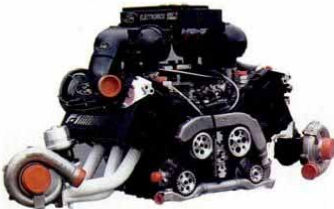
Twin-turbo Formula One Ford engine squeezes nearly 1000 hp from 1.5 liters of displacement, and uses modified EEC IV computer fuel/ignition management system developed for passenger car use.
