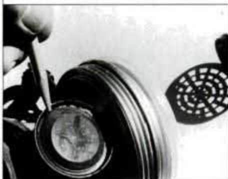
Check respirator fittings for dust buildup. Dust accumulation, shown around the valve, allows contaminated air to enter face mask.
