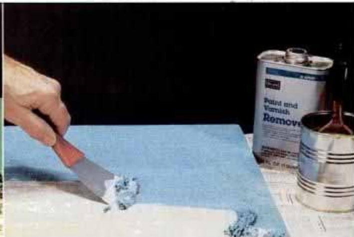
Chemical strippers are easy to use but can be very costly for big jobs.
