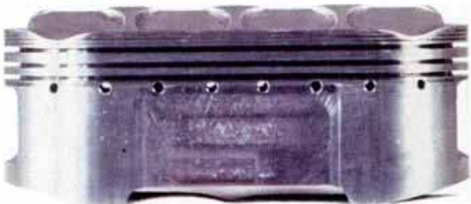
Oval-piston Honda racing engine is the ultimate in multivalve technology. The 4-cylinder, 8-valve, twin-plug motor was intended to circumvent rules prohibiting V8 motorcycle engines.
