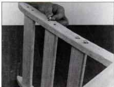
12 Use a plug cutter to make the 1/2-in.-dia. plugs. Glue in place and trim flush with a sharp chisel and fine sandpaper.
