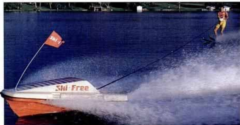
Here's the perfect solution for die-hard waterskiers who can't find a driver, copilot or even a boat to pursue their favorite sport. Ski-Free is a skier-controlled, jet-powered personal watercraft that can pull you all day on 3 gallons of gas. Controls are located in a yoke with a throttle trigger on the left and steering response on the right. This 210-pound, personal ski machine, which costs about $4500, has a deadman switch that shuts down the 40-horsepower engine if you drop the controls. Available by late spring.
