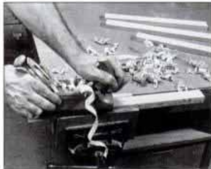
2 A sharp, finely set hand plane makes quick work of dressing the rough-sawn edges. Be sure to follow the grain direction.
