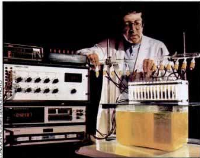
Microbes "burn" sugar to power this prototype fuel cell.
