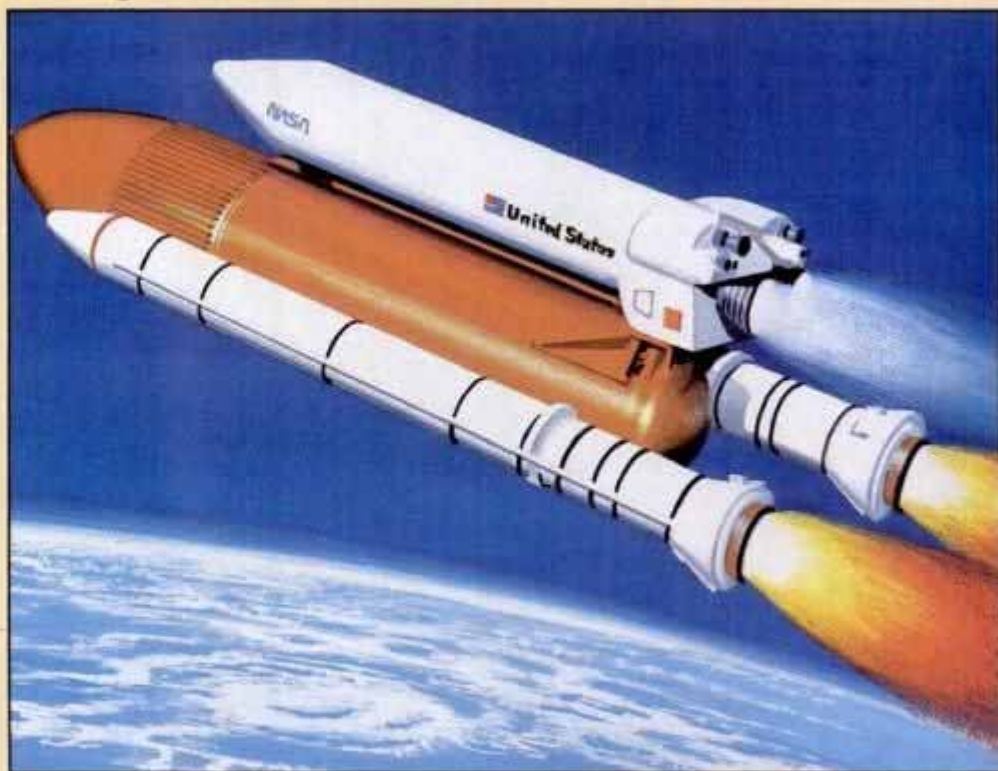
Shuttle-C could put payloads up to 150,000 pounds in orbit.
