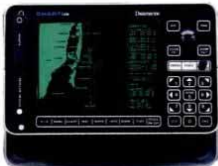
Navigation takes a big step forward with the Datamarine 7000 Chartlink, which translates loran and SatNav information onto visual charts. For $2595, you can measure distance and bearing between points, plus plot your course on an overview of the waters you're navigating.
