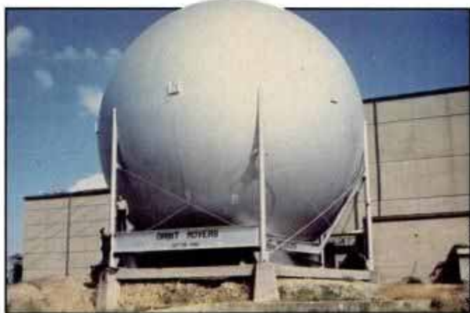
Huge vacuum chamber will clear air out of LHMELE laser cavity.
