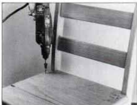
14 After clamping the front and rear units together, lay the seat in position and bore the holes for fastening the seat.
