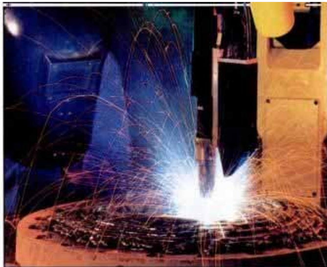
A 600-amp torch guided by robot vision system.
