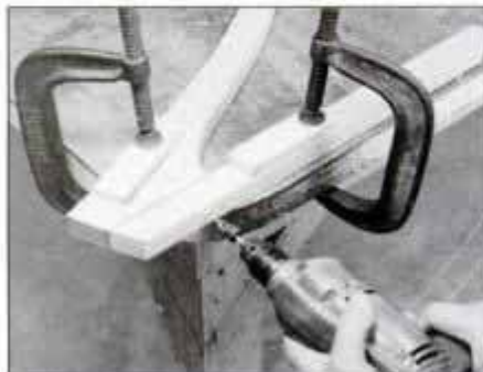
7 Clamp each side assembly to a corner of the worktable and mark and bore the plug, shank and pilot holes for the screws.
