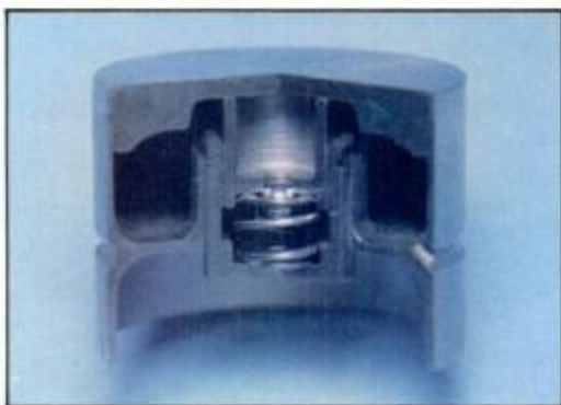
The aluminum-alloy head (above) has subtle aerodynamic shaping in combustion chambers, room for water passage between exhaust seats. Tidy hydraulic lifter (right, top) is only 35 mm in diameter, has close-tolerance fit to bores in cam carrier. Iron insert in alloy cam carrier (right, middle) prevents clearance change with temperature variations. The 1-into-4 equal-length intake manifold (right, bottom) is fabricated from thin-wall alloy tubing which is welded to cast flanges.
