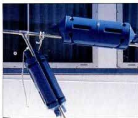
Molded-in grooves that allow new Ocean Fenders to clip directly to stanchions and rails are a clever feature. They interlock easily to form bumper boards and come in many sizes and colors. Prices for the fenders range from $23 to $95.
