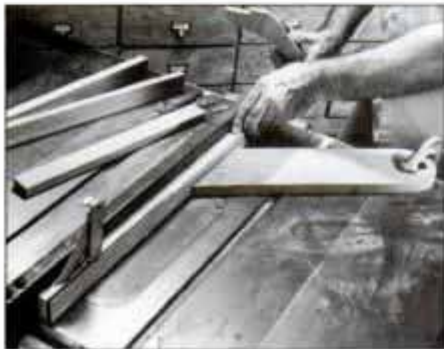
1 After trimming to width, resaw the stock to slightly greater than 5/8 in. To safely rip thin stock, use a splitter and featherboard.
