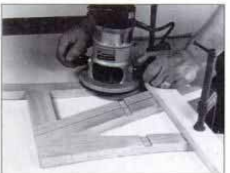
9 Mark the lines for the dadoes that house the steps. Using a straightedge guide, rout the \frac{1}{8} -in.-deep \times \frac{3}{8} -in.-wide dadoes.
