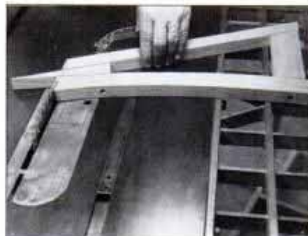
8 The rear side bottom is trimmed after assembly. Use the table saw with miter gauge set to the angle taken from the layout.
