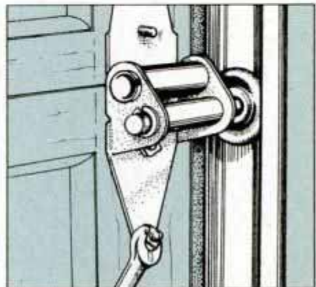
2 Severely clogged rollers must be removed from door by backing off retaining nuts. Be sure to remove one roller at a time.
