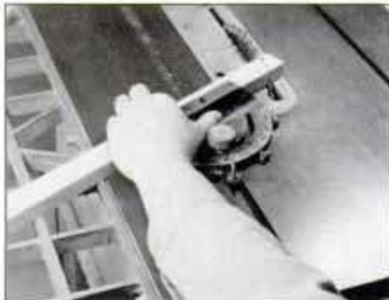
4 The trim angle for the middle support pieces is copied from the layout and transferred to the miter gauge for cutting.
