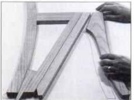
6 When all the side pieces are cut, place them on the full-size layout and check for fit. Trim components where necessary.
